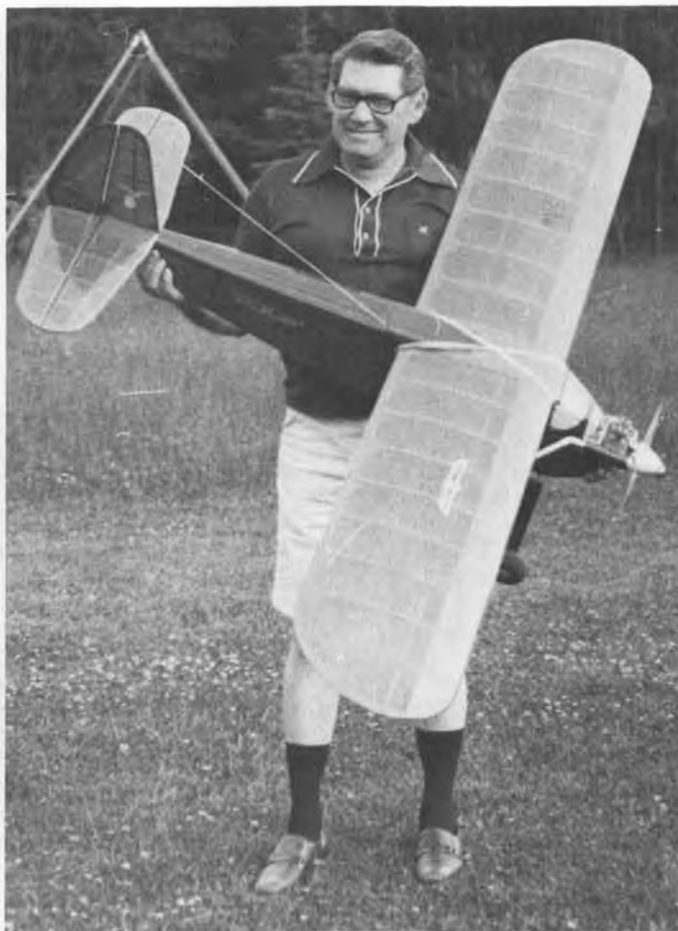
George shows the topside of TORC. Long tail moment assures stability.
