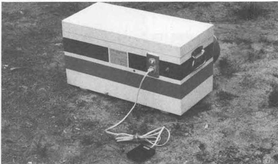
The winch box, ready for the flight line. Foot switch is shown hooked up and ready for use. Pedal stores in box when not in use.
