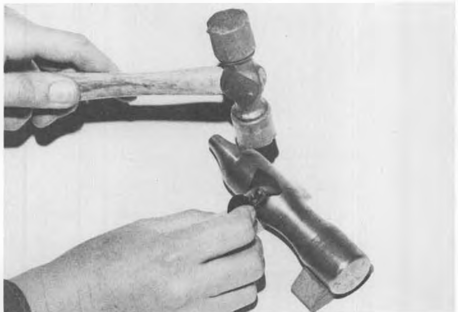
Dial-a-Prop has the mandrels for cupping blades. They are also useful for straightening bent blades. See text.
