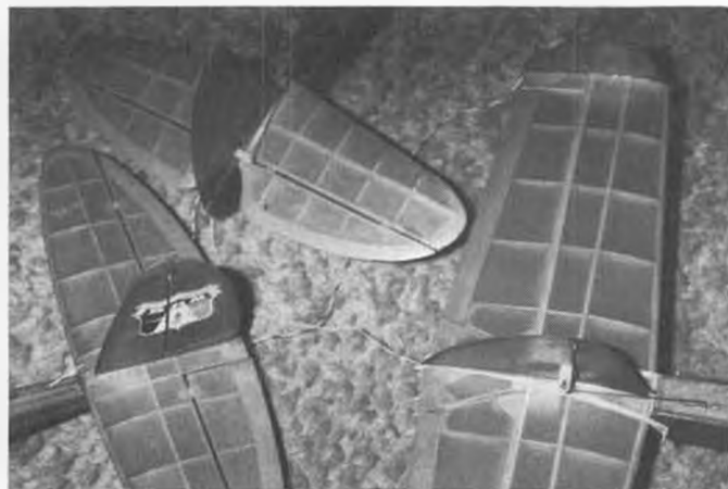
Typical control surface details. Control areas must be adequate and not interfere with each other.
