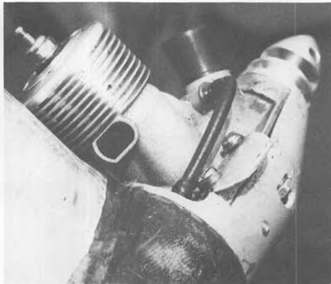
The split rear exhaust is an interesting . . . and practical feature of the Russian engine. Clears leading edge of wing, also wing pylon on F/F.
