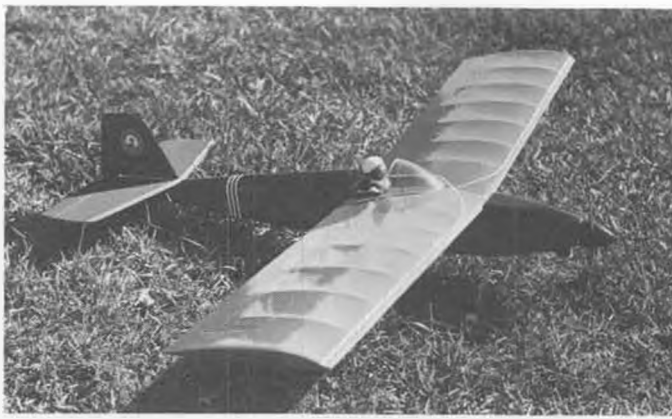
The author's S-Tee is a shoulder wing version of the Cox Q-Tee. It uses 2-channel R/C. Original is Lee Renaud design.
