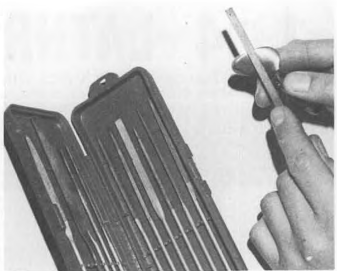
A good set of jeweler's files is used for sharpening the leading edge.
