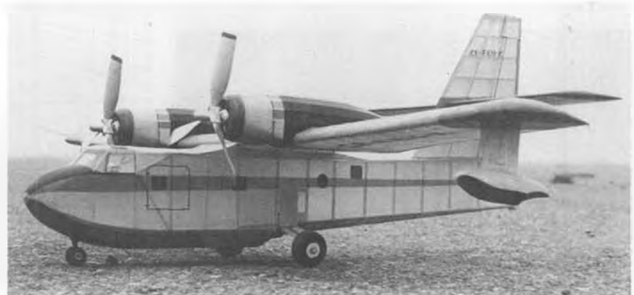
Walt Mooney's Canadair CL 125 had rubber power in nacelles, which limited flights to about 20 seconds. Excellent performance otherwise. Interesting R/C scale possibilities, no?
