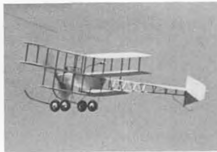
Bill Warner's CO 2 Avro 4 is all sheet balsa construction. Foam wheels.
