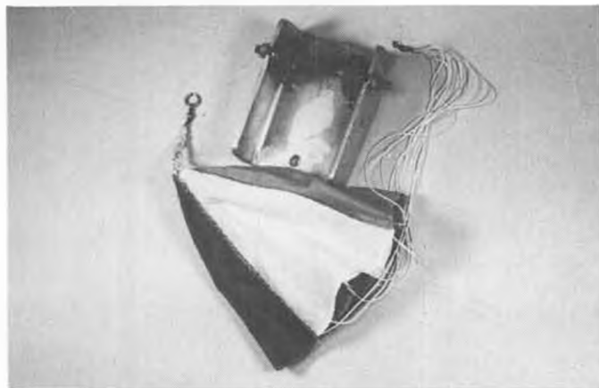
Parachute and turn-around are stored in box. Turn-around is made of channel stock and bicycle hub.
