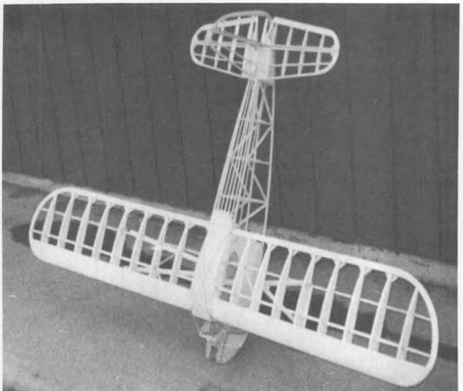
No, the framework is not showing the normal landing attitude of TORC! Structure is simple, light, and strong.
