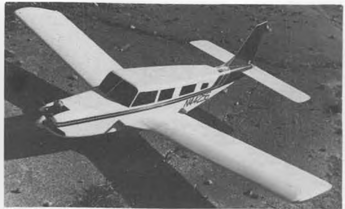
R/C Sport Scale 1/2A Piper Cherokee Lance from Superior Flying Models, has R/C rudder and elevator controls.
