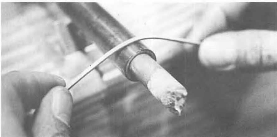
Hot soldering iron is used to bend bamboo. Keep bamboo strip moving to prevent scorching. Proctor kits are about the only place you'll find bent bamboo in modern model construction.
