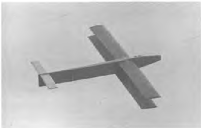
Chet Herbert's experimental bi-sailplane uses pivoted wings as the only control. Very sensitive.
