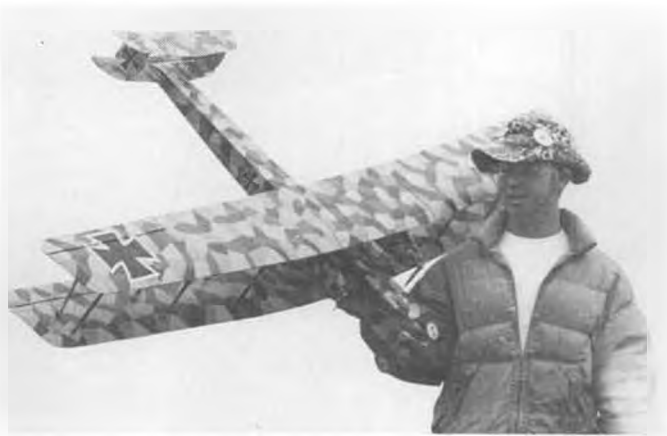
Bill Stroman's Zeppelin "Staaken" with four Astro Flight .020 electric motors. Pendulum controls for stable flight.
