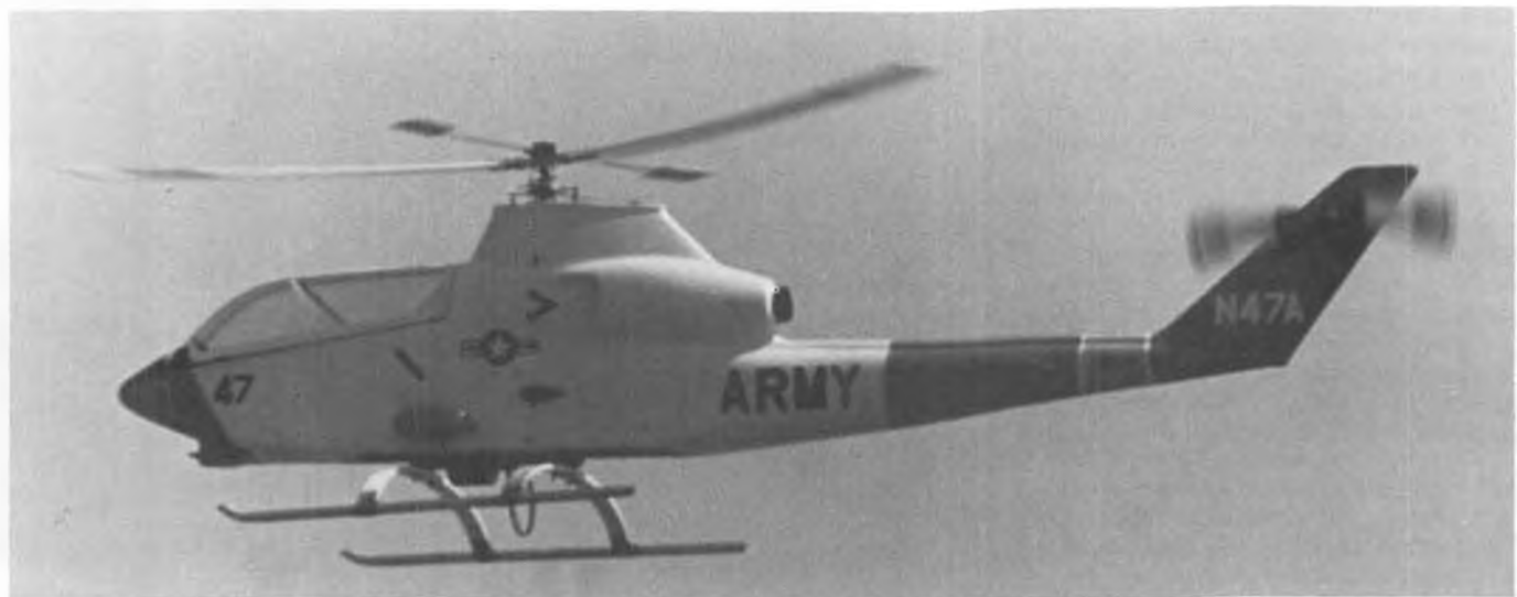
An eight-year-old Schluter Cobra, being flown by Dick Tristao. Twelve pounds flying weight, OS .60FSR power, MRC single-stick radio, and K&B Super Poxy finish. Cobra has logged over 700 hours of flying time.
