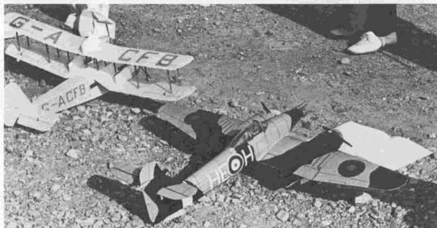
Westland Whirlwind from a Cleveland kit, by Chuck West. Uses two Cox TD .020's. Had problems with inconsistent engine runs.
