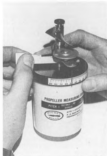
Measuring blades to check for equal cupping.
