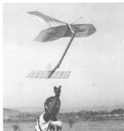
Darryl Stevens' Cat I and II record holding ornithopter. Model has 4 flapping wings, and 600 sq. in. area.
