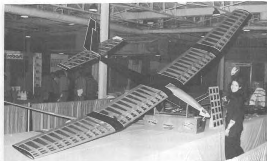
Powered glider built by Bill Goff, Texarkana, Texas, has 20 foot span, weighs 25 pounds, and is powered by ST .46 engine. Debbie Dilworth provides size comparison.
