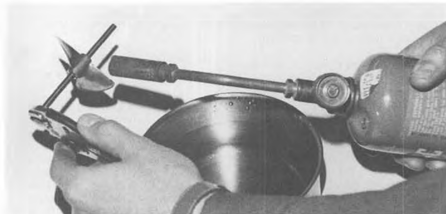
Heating a prop with propane torch is part of softening treatment so that blades may be cupped and sharpened.
