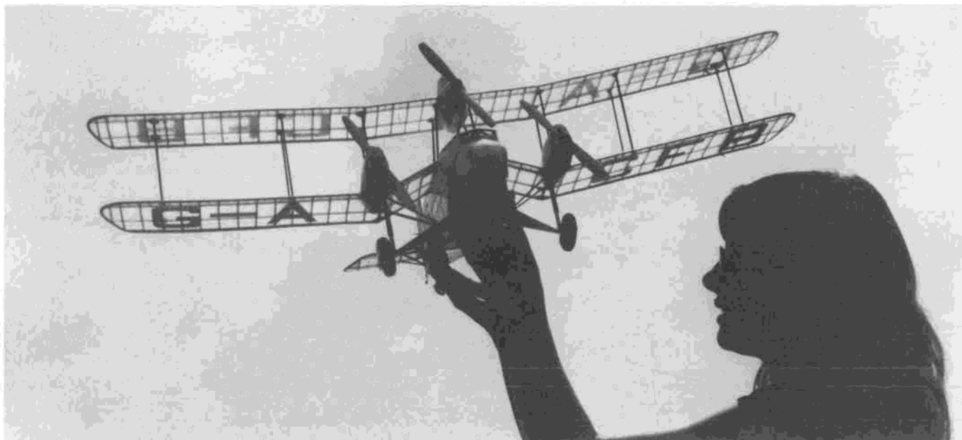
Bill Warner's Airspeed Ferry AS-4 has three first place trophies to its credit. It's powered by three Astro .010 electric motors and weighs 14 oz. with four 3/4 length nickel-cadmiums. Features interior detail, opening door, working landing gear oleos. Held by wife Phyllis.
