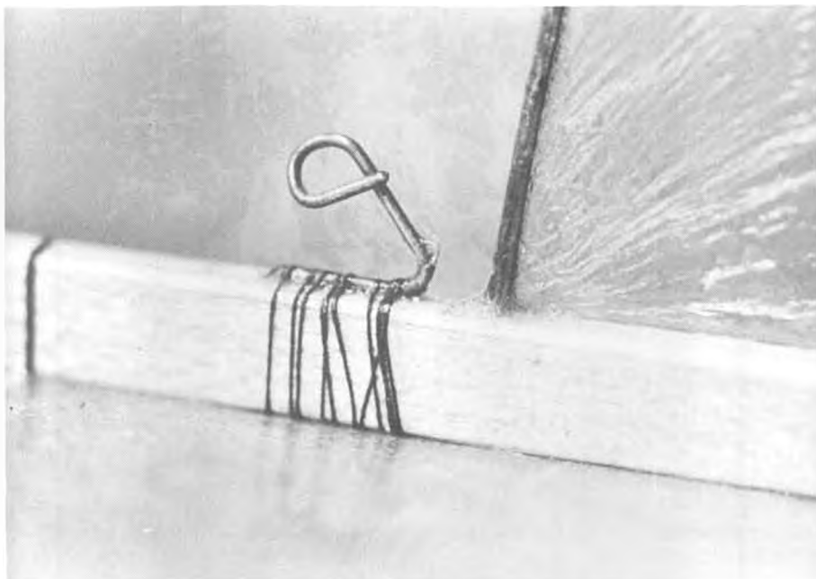
"S" hook will not walk or climb off this simple rear hook. Model is wound from the rear.
