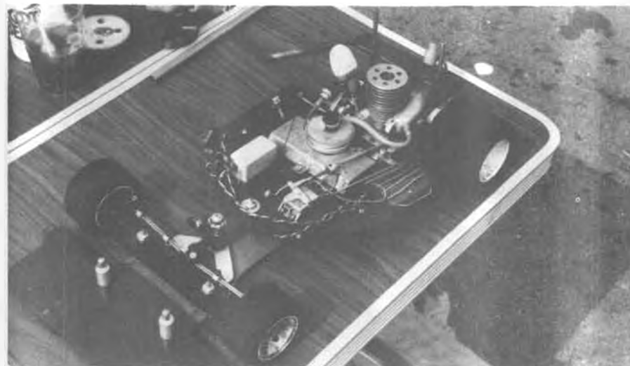
Gary Kyes' car will probably have battery and receiver moved forward to compensate for extra weight of 80 db muffler.
