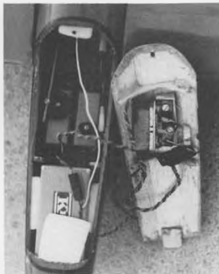
Radio installation. Switch is mounted in canopy, saves room in the fuselage.
