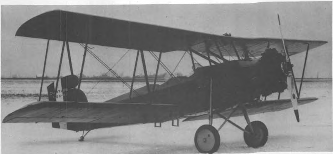
The 9-cylinder J-5 Whirlwind was phased out at the end of the first production run of Fledglings. Later Fledglings were equipped with the new 7-cylinder J-6 Whirlwind. Shown above is an N2C-2 with a J-6 installed. Howard Brooks photo.
