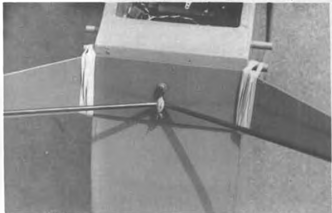
To get a stiffer landing gear, Tom Laurie added a spreader. Rubber bands at center provide some "give", if needed.
