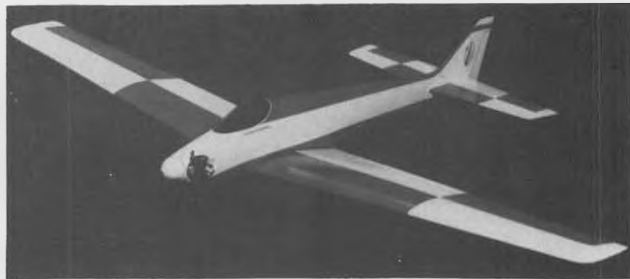
J&M Glascraft's "Fun X", 1/2A pattern and sport model. Features foam wing cores and glass fuselage.
