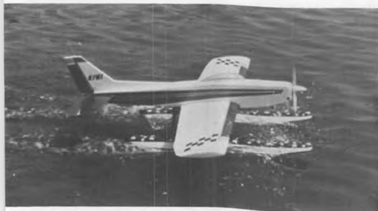
Above and below: Hank Pohlmann gets his feet wet launching the Kiwi, which takes to water like a duck on a pair of 33" Gee Bee floats. Lower right: Jim Duda's Kiwi has a sharp red, white and blue color scheme. Cables from the nose gear steering bracket operate a water rudder on one float.
