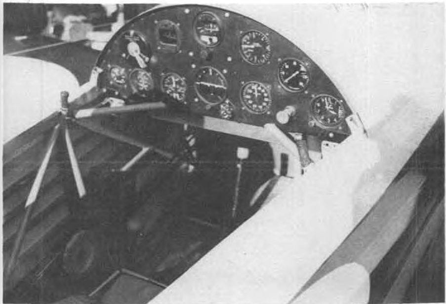
Cockpit of the Gee Bee. Rather cramped for space, but well instrumented. Fuel gauge is mounted on top of the fuselage, between the cowl and canopy (see other photos).
