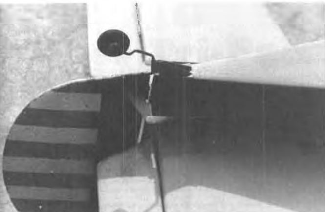
Tail wheel and rudder hook-up details. Tom's tail wheel bracket is bent from sheet aluminum, but a nylon one would be OK.
