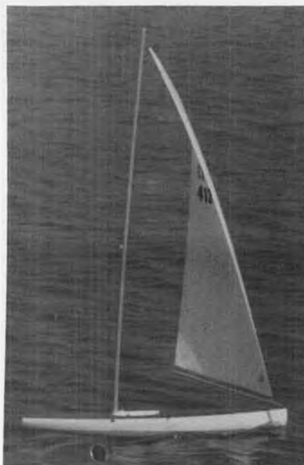
Insufficient leech tension has allowed a 90° twist to develop on this reach. Mast bend is again slacking the jibstay.
