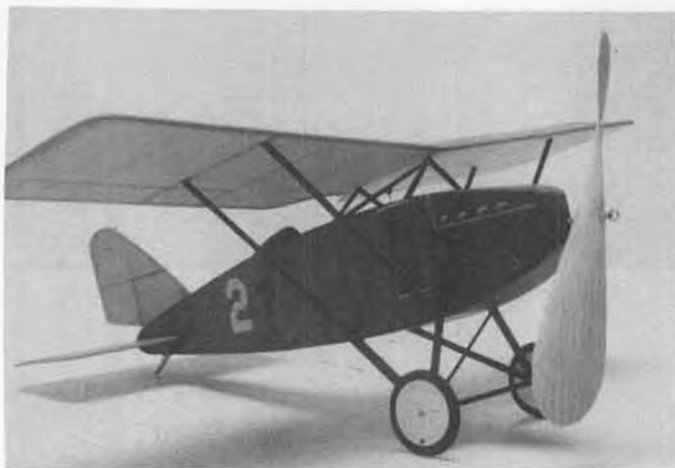
Laminated prop adds the finishing touch to the author's nicely-build Waterman Racer peanut. Also increases performance.
