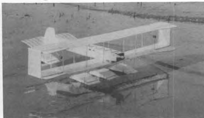
Bill's 1911 Voisin had CG too far forward at Flightmasters R.O.W., has since been trimmed and flies great (like all of Bill's models).
