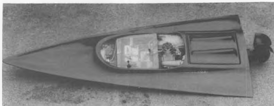
The Cobra Jet is reminiscent of Ed Fisher's "Northwind" delta hull boat. Comes completely assembled, all that's required is to install a radio.
