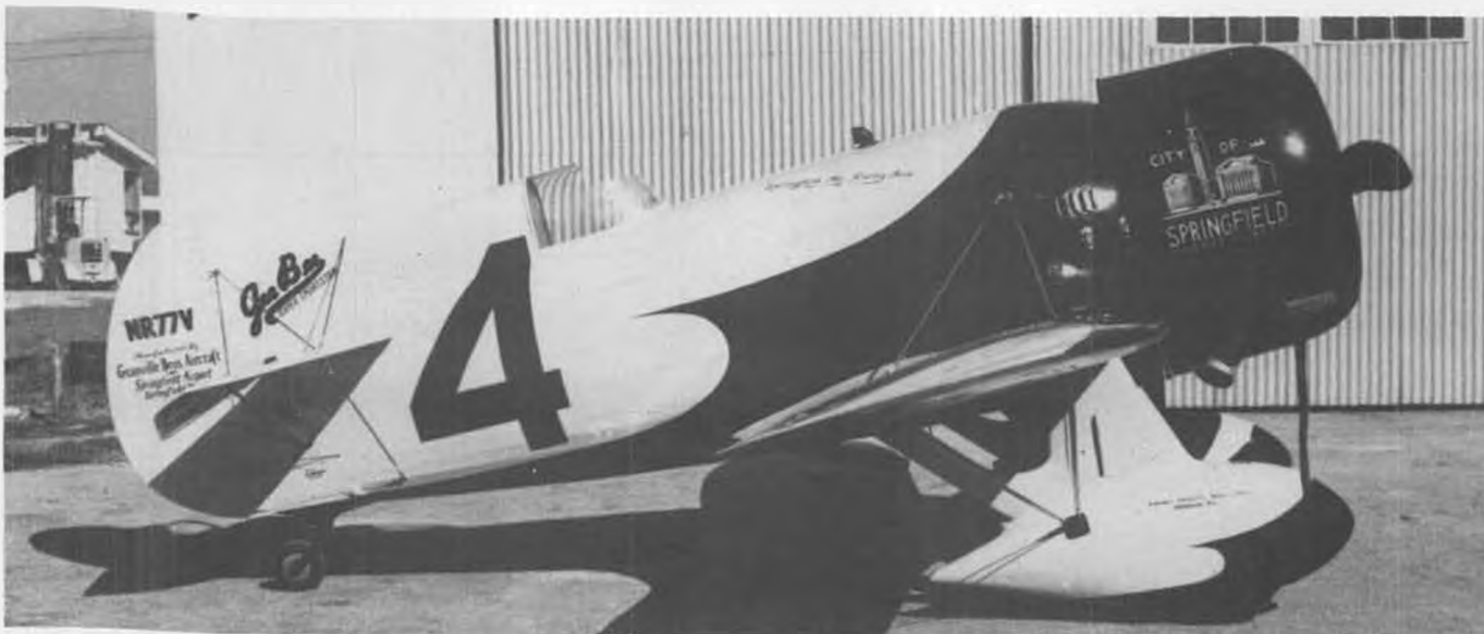
Bill Turner's incredible Gee Bee Z reproduction shortly before being completed. Note the thin wing section. Flight tests have been 100% successful; Turner claims the Gee Bee is even more stable than his "Miss Los Angeles" Brown Racer reproduction.
