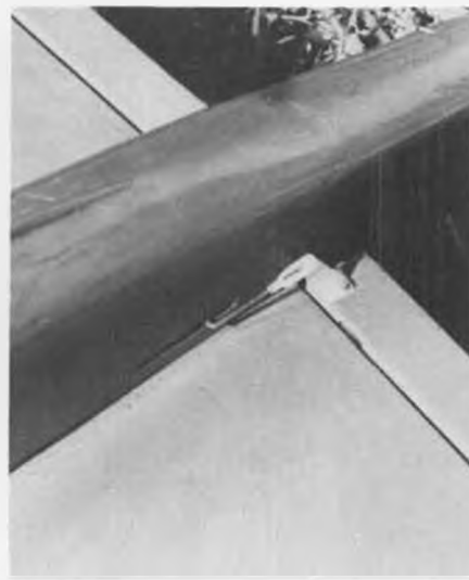
Aileron linkage details. See text for Al's comments about bends in aileron pushrods.
