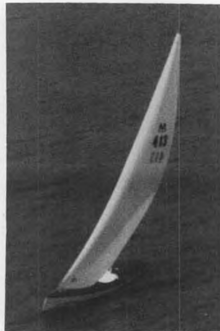
Jibstay has sagged under wind pressure both aft and to leeward, resulting in increased camber in mid-parts of sail.
