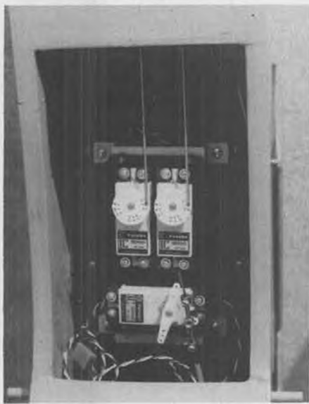
Radio installation. Note spring override on throttle servo. Five-channel Futaba system.
