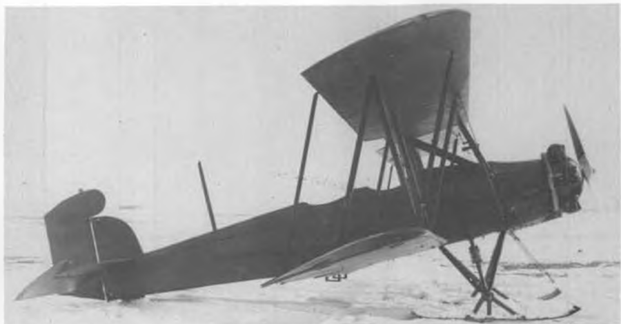
Fledgling NC-8661 was equipped with lights, radio, and skis. Big ailerons made the Fledgling easy to control, but they became stiff at airspeeds over 100 mph.
