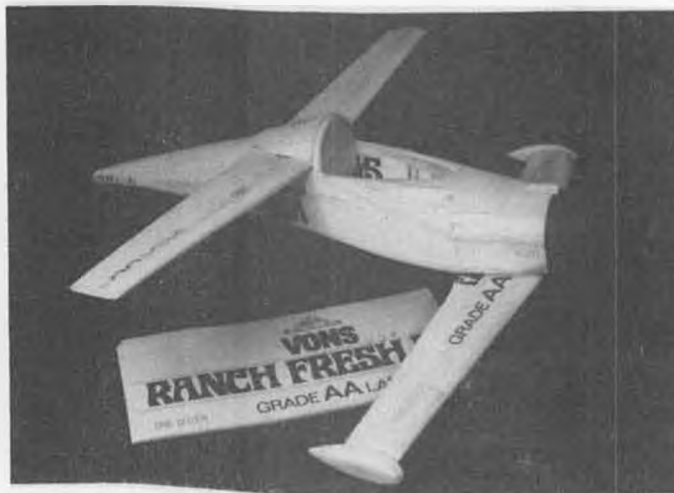
Herb Kelley, of Yucca Valley, California, demonstrates use of foam egg cartons in his "Quickie" flying scale model. All joints are made with Titebond, sanded like balsa.
