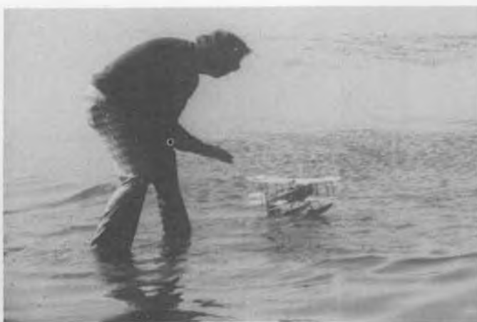
Nice action shot of Ken Johnson launching his Sopwith "Baby". Floats are open structure, covered with paper.
