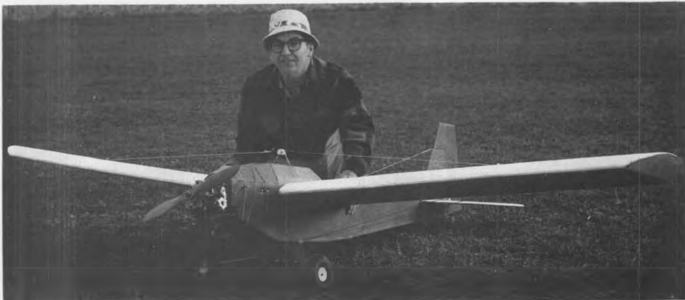
Norman Delaney's cardboard R/C model is very similar to the ones that Dave Gray and the fellows at Du-Bro were testing their prop drive units on. Norm's model spans 113 inches and is powered by a Quadra. Does not appear to have ailerons. Simple and inexpensive to build.
