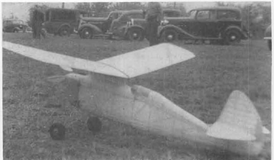
Tom Mountjoy's last F/F model, the Avenger, built in 1941. Ship was powered by a Brown Jr., mounted inverted. Real unusual lines, too bad we couldn't get the plans.
