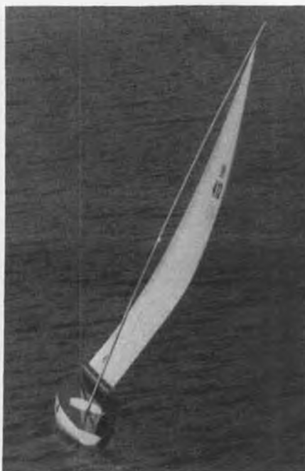
In this photo, the mast has bent off to leeward, which has accentuated the slacking of the jibstay.
