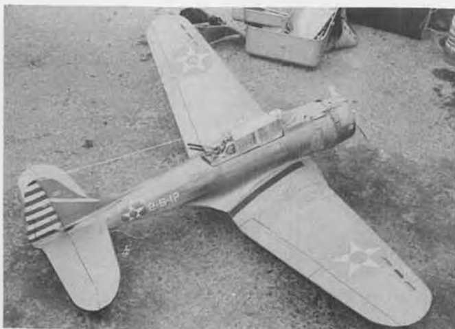
Absolutely gorgeous SBD-3 by Gary Paczkowski is based on a Guillow kit. Has rudder/elevator/throttle controls, flies with a Tee Dee .049. Gary added six inches to the span to get a little more wing area to better carry the weight. Full up elevator releases bomb.
