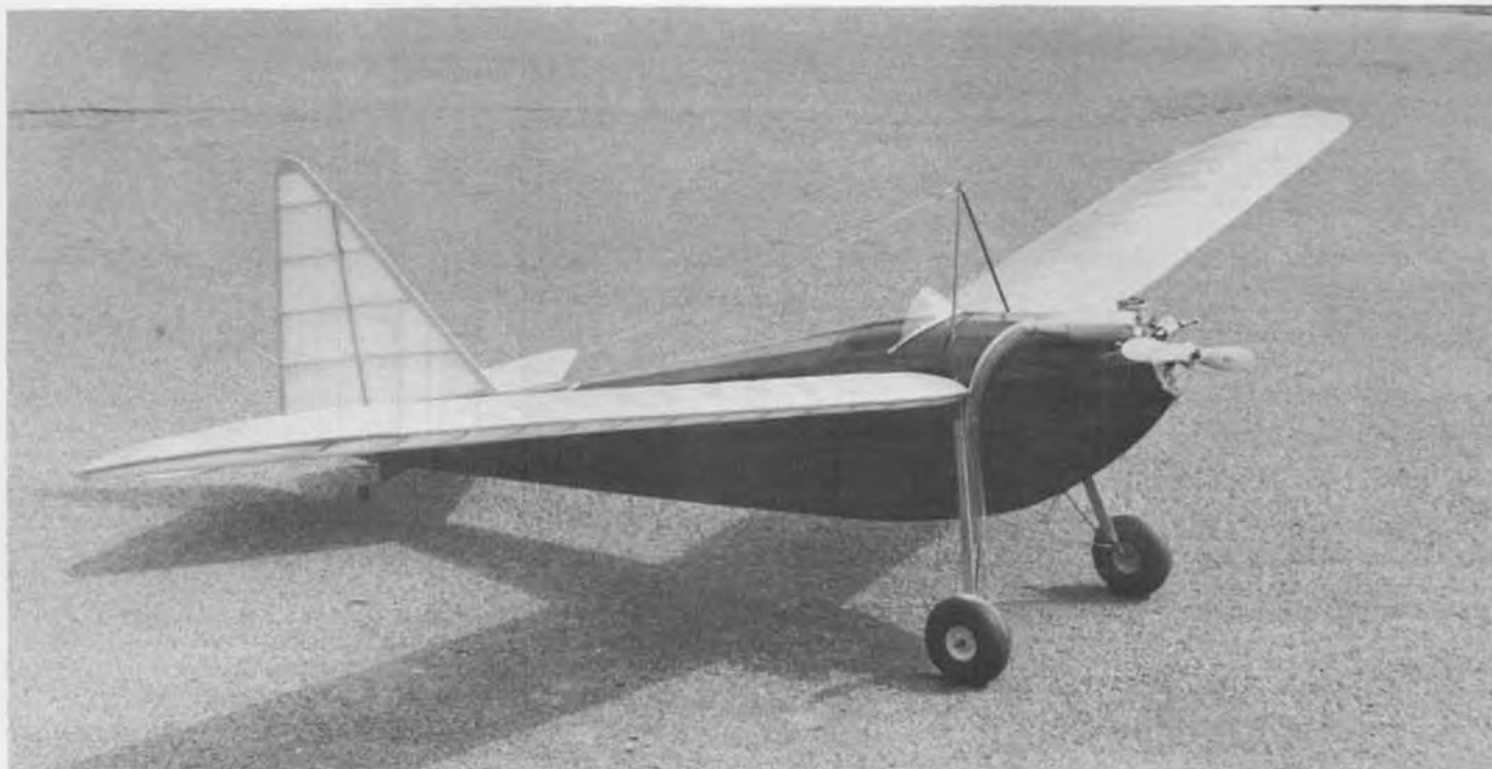
We published plans (91074-O.T., $4.50) for this great semi-scale, 8-foot span Buhl Pup old timer from a 1936 M.A.N., and surprisingly, sold only a few copies. This one built by Capt. Charles Strange, USMC, Camp Pendleton, Calif. Webra Speed 40 power, 6-1/2 lbs., Super Coverite.
