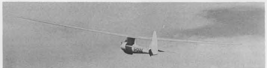
John Foster showed up with an unusual bird, an old British design called the "Hjordis." Aerodynamically clean model has no spoilers, is said to be a tough one to land.
