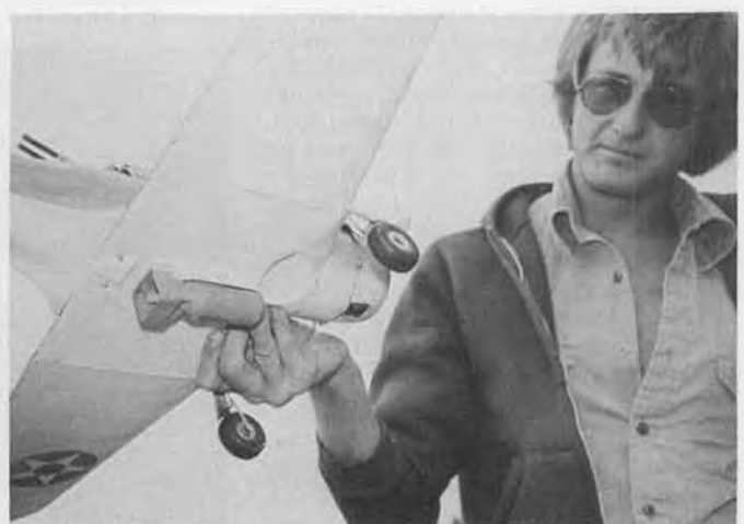
Absolutely gorgeous SBD-3 by Gary Paczkowski is based on a Guillow kit. Has rudder/elevator/throttle controls, flies with a Tee Dee .049. Gary added six inches to the span to get a little more wing area to better carry the weight. Full up elevator releases bomb.
