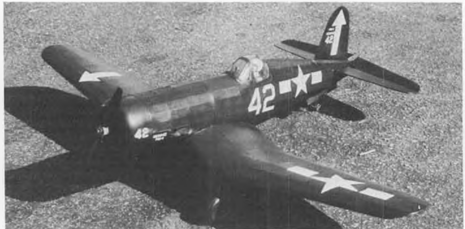
Tony Naccarato is at it again, this time with an electric control line scale Corsair! Power is an Astro 02 with the R/C battery pack. Weighs 12 oz.
