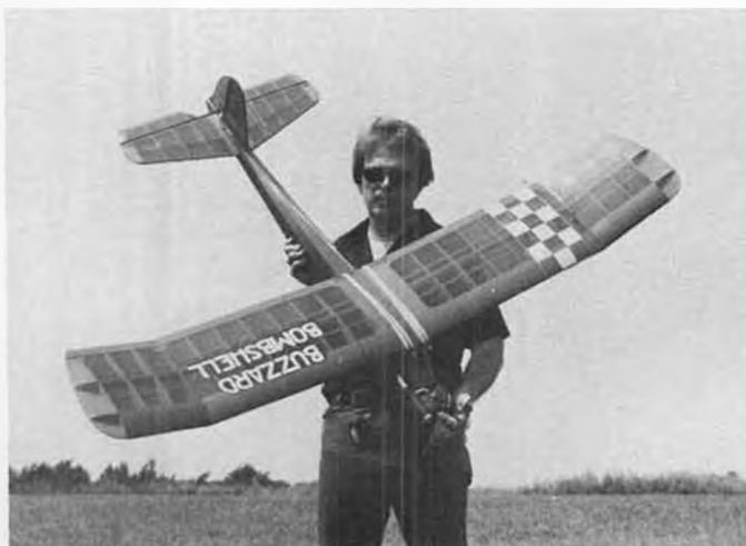
Duie Matenkosky with his 4K's kit version of the Buzzard Bombshell. Solarfilm, Enya .35, Kraft/Ace radio combined for 3 channels.
