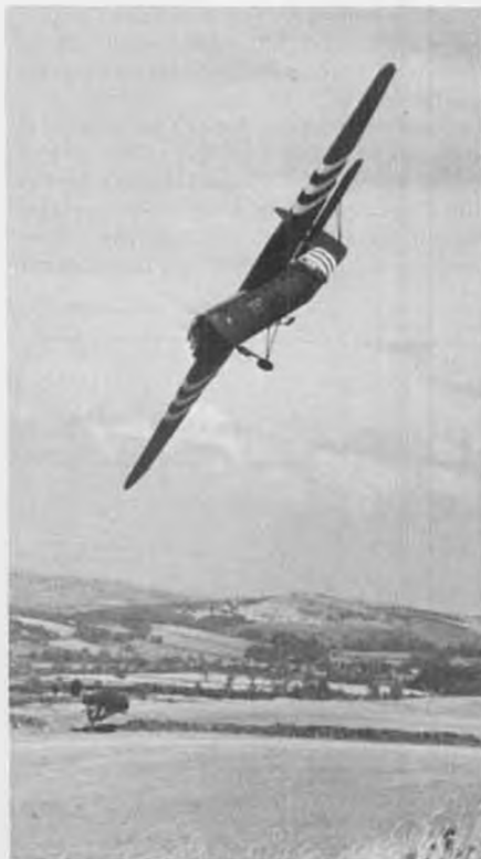
Brian Eagle's WW-II Horsa troop glider experienced aileron flutter on one such high-speed pass, lost one aileron entirely. Got it down OK, though.
