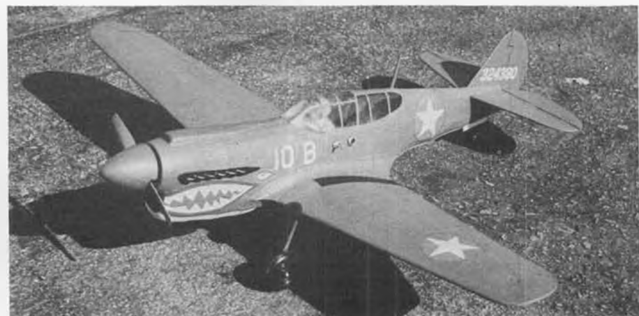
Bob Trace has the lightest of the electric C/L warbirds, comes in at just 10 oz. All of these models are built from Guillow kits, fly on 20 to 25-foot lines, indoor or out.
