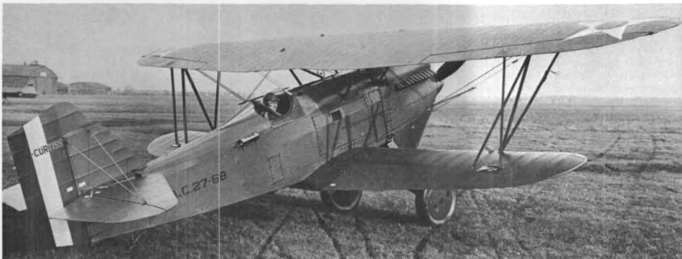
The P-1B, subject of our drawings, had larger wheels than earlier Hawks and redesigned radiator and cowl. Color was khaki overall. This one sports a new Air Corps number, but the rudder still has Air Service red, white, and blue vertical bars.
