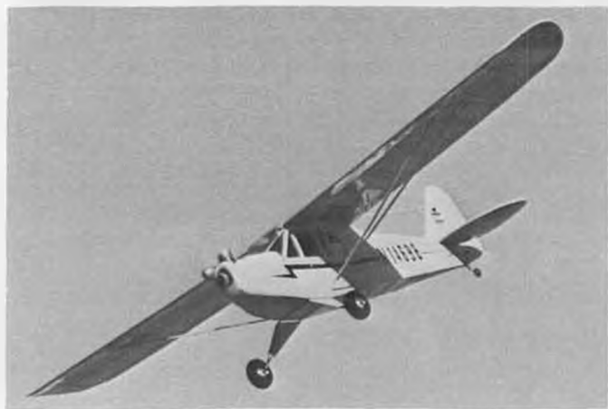
The M.E.N. Cub's highly undercambered wing and light weight make for an easy, slow-flying model. Photo by Bill Knorr.
