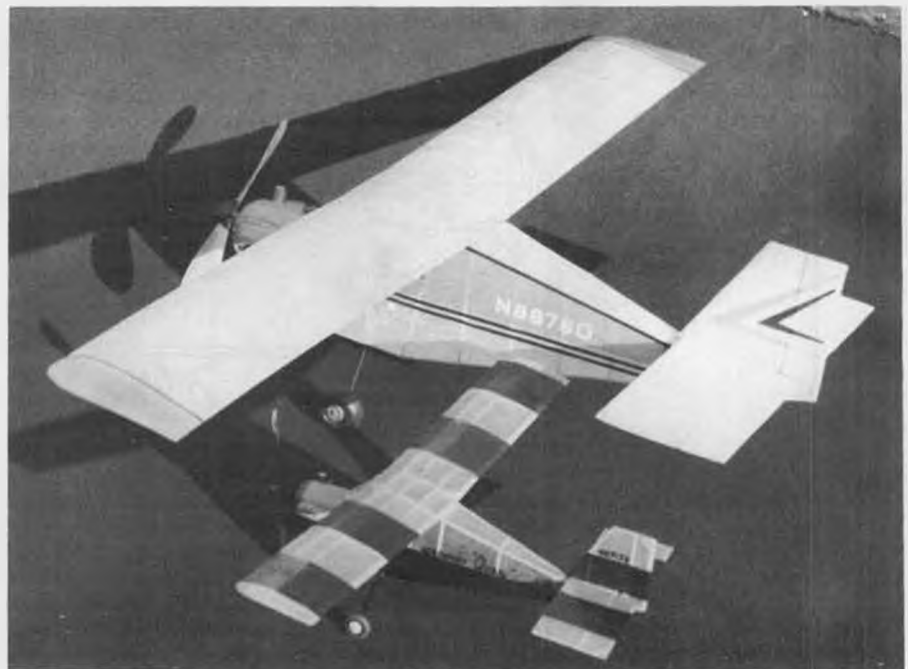
Father and son Quails. The large one is recommended for beginners because the larger wood sizes are easier to handle, and the large size also makes the big one easier to trim for flight.
