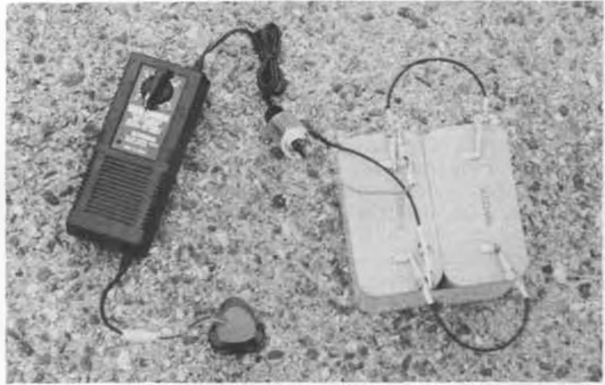
For field charging, the Kraft charger can be hooked up to a 12-volt battery, in this case two gel-cells in parallel.
