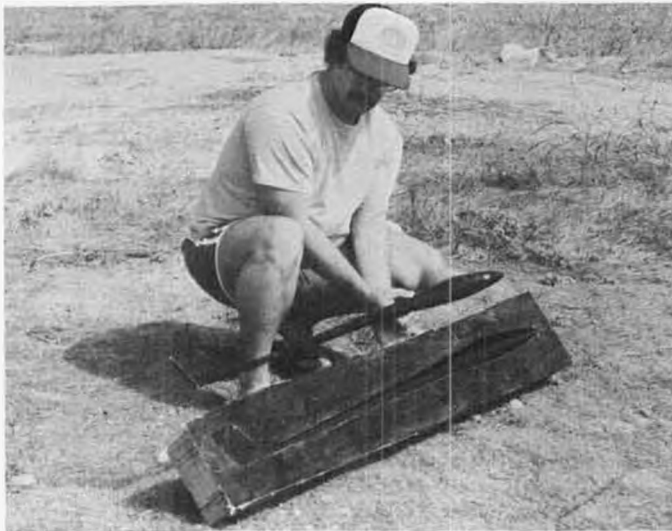
Rick Schrameck holds the fuselage plug and mold for his new F3B design. Looks like a lot of work . . . and it is.
