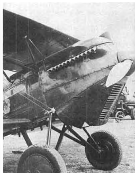
Thirty-one Hawk AT-5A trainers with Wright J-5 engines proved unsuccessful; 24 were converted to P-1F's with D-12 engines. Photo by Ed Chavez.
