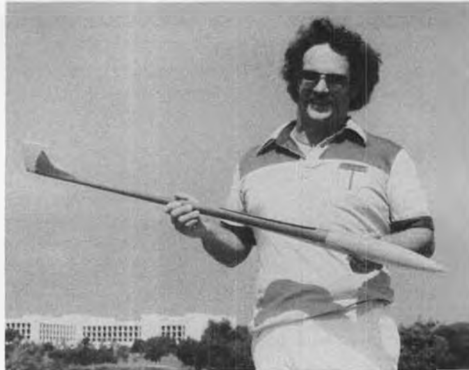
Rick poses with a finished fuselage. Dark areas are carbon fiber reinforcement. Text gives full details.
