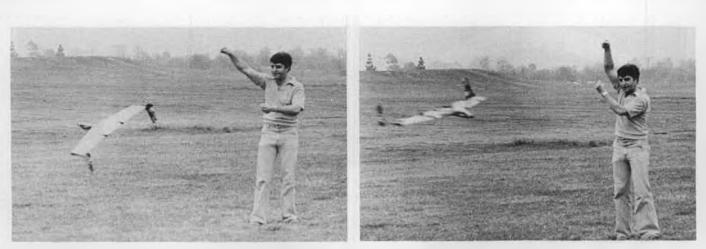
Author-designer, Larry Renger demonstrates the testing technique used for determining CG location and trim settings for maximum stability. Model is swung around right side up and inverted . . . when it flies like this, it's ready to fly R/C.
