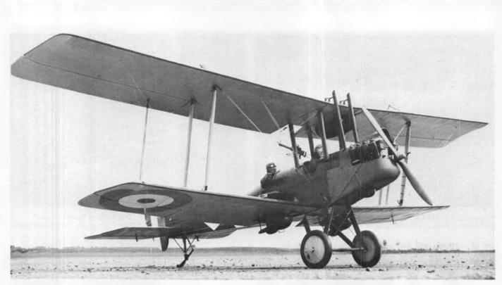
Magnificent 1/6-scale BE 2e, built by David Deadman, from Roy Scott design, as kitted by Practical Scale. OS 60 H engine. Rudder, elevator, throttle, and bomb dropping. Ailerons not working, and not found necessary.
