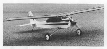
Note wide tread of the landing gear. Extra dowels probably for float gear.
