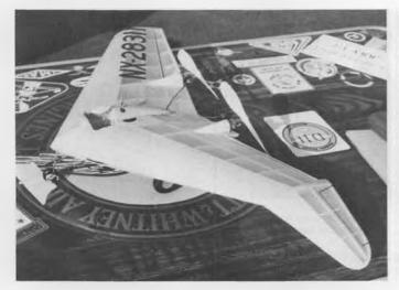
Northrop N1M Twin CO2 powered scale ship, with pendulum control on the elevons, built by Daniel Walton, Liberal, Kansas.
