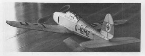
By TOM HOULE . . . Originally intended as a trim and balance test bed for a later six-foot version, this 18-inch, rubber powered scale model of a German trainer has proved a worthy flier on its own merits.
