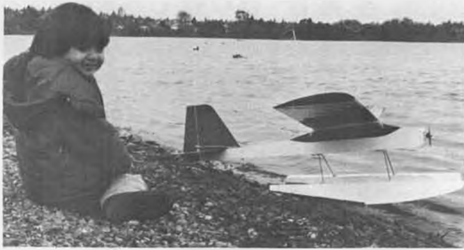
The Sea Gull and Victoria Poling at the lake. Sea Gull flies well on Astro 075 and Astro 15 at 3-1/4 to 4 lbs. flying weight.
