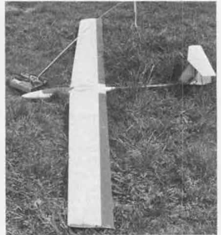
Dohle 84, designed by Dr. Helmut Quabeck, modified (T-tail) by Herbert Heil. See text.
