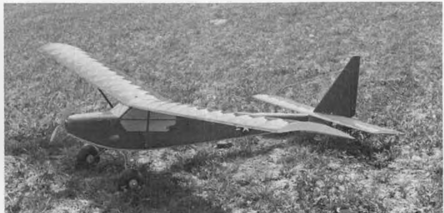
Glider towing and parachute dropping plane, by John Evans of Reno, Nevada. Uses modified M.E.N. Cub wing, modified Oly II tail surfaces, original fuselage.
