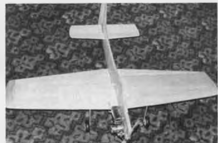
Midwest Skyraider by Gerald Schamp awaits paint job. Mods to kit include; built-up profile fuselage, sheeted wing. Enya 40 engine.
