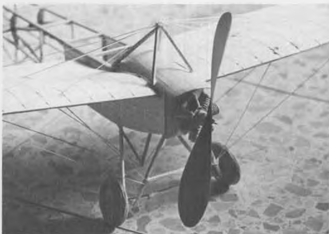
All-balsa rubber powered Somer Monoplane constructed by model book author Amos Hadas, of Israel.
