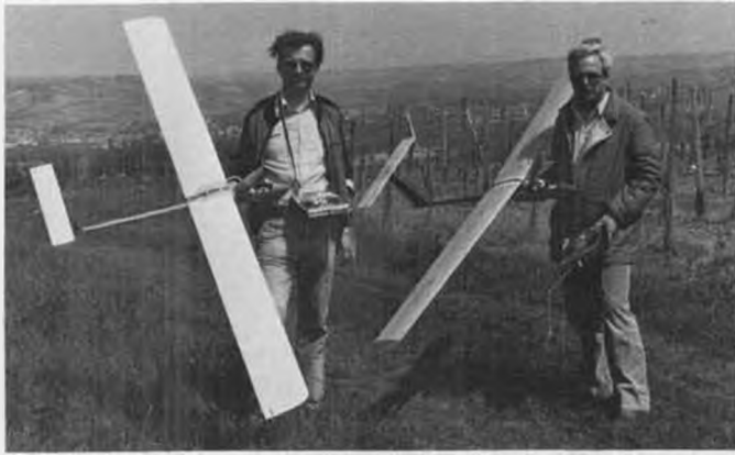
Identical molded fiberglass two-meter ships, built and designed by Herbert Heil (left) and Ralf Markwort. See text.
