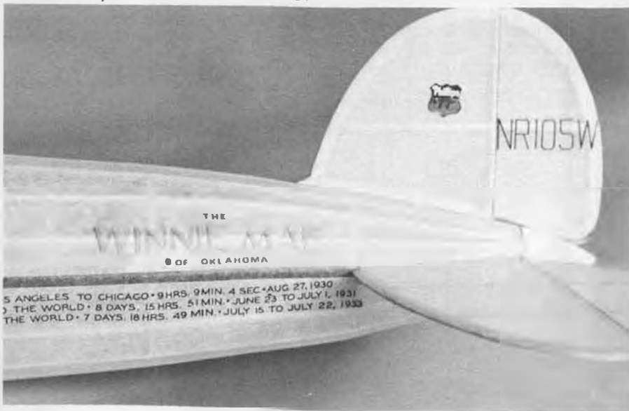
Tail detail (Say that several times in a row and you're ready for a waltz!). Both the rudder registration and the lettering below the trim stripe are Decalon decals (see text).
