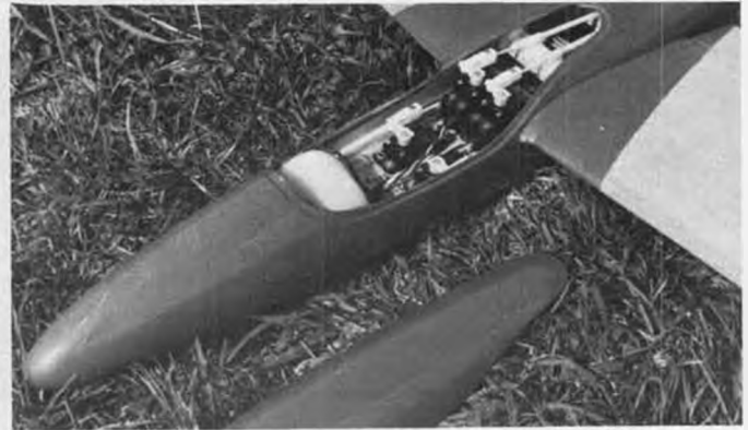
Floh interior. Front two servos control V-tail from Tx mixer. Rear servos control mixed flap and aileron functions (flaperons).
