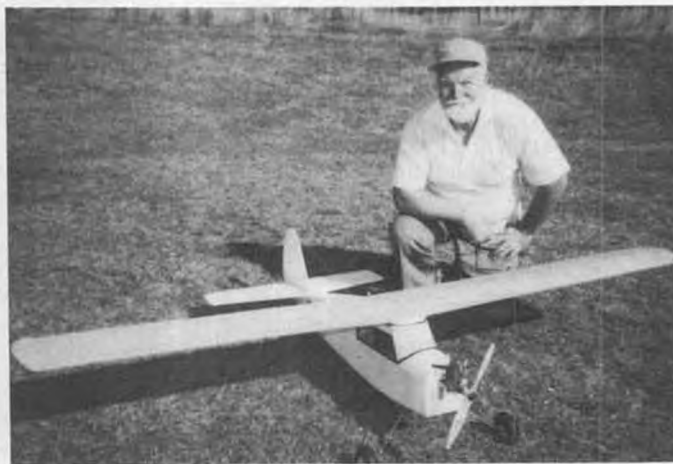
Del Bowers, of the Puget Sound Rocs, with his 92-inch span, Saito 45 powered Cavalier. A fine trainer combination.
