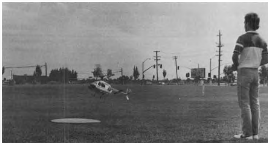
Robert Gorham sticks another one on the pad during autorotation demonstrations at Merced. This is the Jet Ranger body on Cobra mechanics, as described last month.
