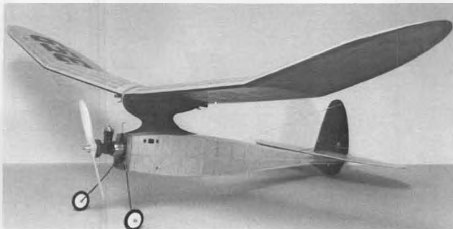
Model has a wing area of 315 sq. in., spans 50-1/4 inches and weighs 17-1/2 ounces. Use a dark color on the bottom of wing and stabilizer for best in-flight visibility. Prather nose weight.
