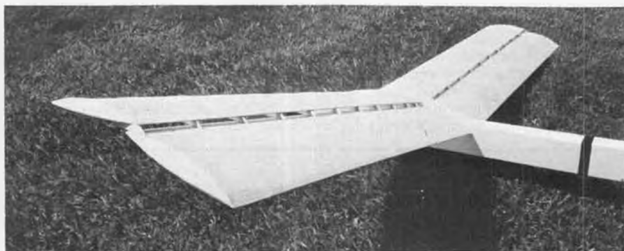
Slotted forward wings on Gossamer Slow Poke I.
