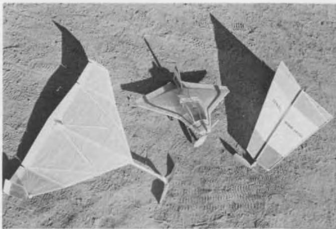
Variety of Northrop Wing contest entries (l to r): Dan Walton's rubber-actuated variable incidence tail, his Peanut Dyke Delta, and Bill Hannan's low A/R demi-delta with tissue covering on bottom only.
