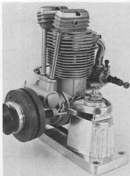
Al's OS FS-120 in Tatone's new engine test unit. Of cast aluminum, it's rugged and fuel proof. OS has CH Electronics Ignition Conversion, runs beautifully.
