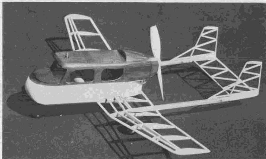
Partially finished Wheelair. Note CO 2 filler on top front of cabin, soda straw twin tailbooms, and wing rib cut from some old printwood! Keeping proper incidence angles require extra care.
