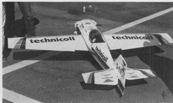
Diabolo, by Tsugutaka Yoshioka, Japan, former World Champion. OS 108 FSR Twin power, JR PCM-9 radio.
