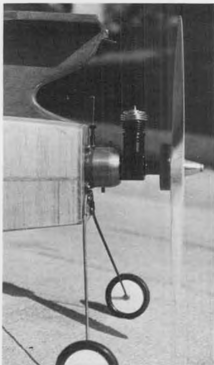
Cox Black Widow has five head gaskets and a Golden Bee tank. With 8x4 prop and 5% nitro fuel, it'll run nearly seven minutes.
