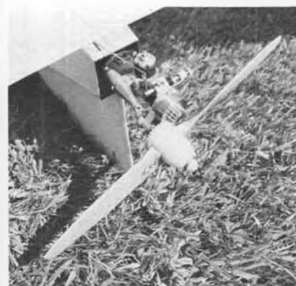
Nine-inch prop on Gossamer Slow Poke I was turned by geared G-Mark .03 engine. All photos taken in May of 1983.
