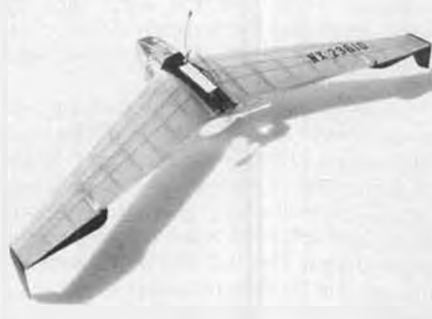
No. 7752 THE ALIEN $2.50 Pendulum controlled flying wing pusher for Brown CO2 power. Daniel Walton.
