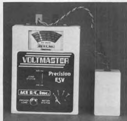
The Ace R/C Voltmaster, precision four-range Expanded Scale Voltmeter (ESV), shown with 500 Ma 'square pack' for size comparison.
