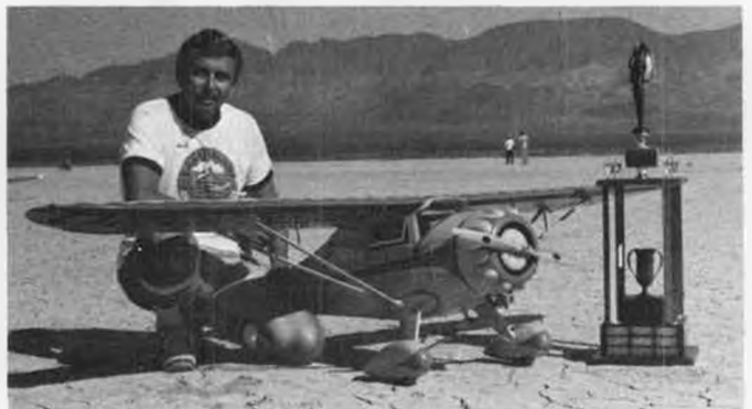
Best Scale winner, George Harlan, Irvine, Calif., with his Monocoupe. Weighs six pounds, 96-inch span, powered by Webra 91.
