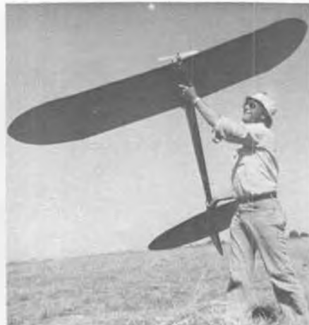
Bob Stalick shows launch technique for his D Quell. Model is silk covered, Epoxy and glass clothup front. Photo by Bill Giffen.
