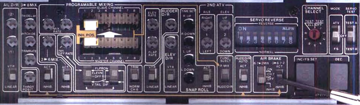
The 8SGA (airplane) programming and trim panel. New programmable mixing and aileron differential control, plus 2 servo test circuits and digital ATV control.
