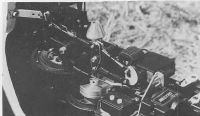
This closeup shows the homemade push-pull mod on Curtiss' elevator setup. Bellcrank made from old sideframe material and it is supported by two 3mm ball bearings. This reduces unsteady aerodynamic loads feeding back from the blade pitching moment to the poor servo output shaft.
