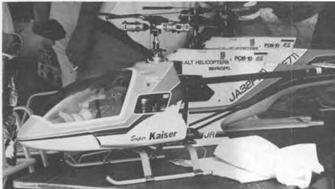
Part of the Japanese display team's TSK Super Kaiser model. It uses the same hingeless TSK H-30 main rotor head as on Ishikawa's machine. A high quality, but expensive, pod-and-boom model.
