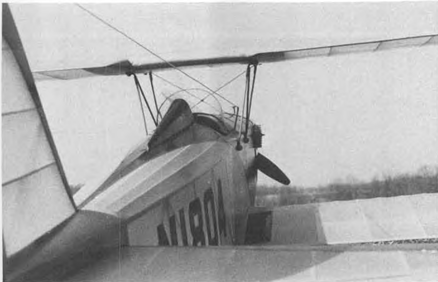
Coat hanger wire cabane struts are rugged, yet easy to bend into shape. Short aluminum tube brings antenna clear of windshield. Flew for two seasons with PCS "metal can servo" radio.
