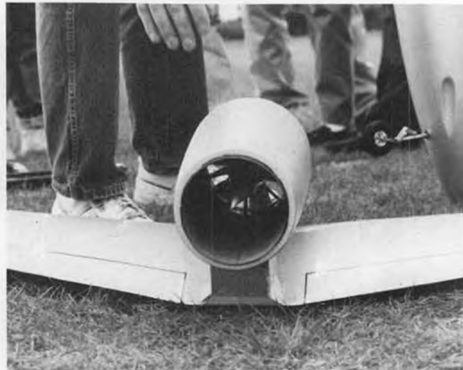
Close-up of twelve bladed fan unit. Keller motor twists 14-15,000 rpm with a thrust of 2 kp (4.4 lbs.).
