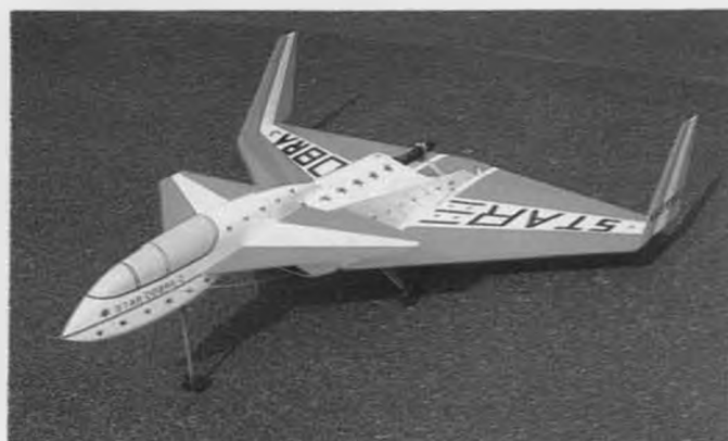
Jim Harrison's Star Cobra II. OPS 45 powered Thorjet fan. Weighs 8-1/4 pounds.
