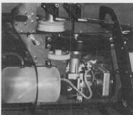
The 2-stage gear reduction design. The 1st stage is driven by the clutch bell housing. The 2nd stage is driven by a pinion gear running inside the Delron gear housing. Note the location of the remote glow plug connector and clear plastic cooling skirt.
