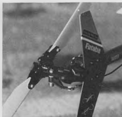
New gear box and ballraced sliding pitch control mechanism is extremely smooth. Tail blade grip has radial and thrust bearing. The metal fin with the integral skid wire is very robust.
