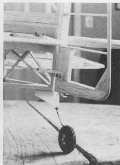
Tailwheel linked to rudder by piece of strip aileron horn swivel.
