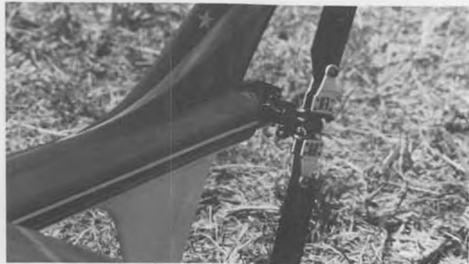
Double ball bearing tail rotor blade grip. At 5:3 to 1 ratio (tail rotor:main rotor) this fast tail rotor speed should give excellent yaw response. Response might be even better if the tail rotor is on the other side. Very slick fin fairing.
