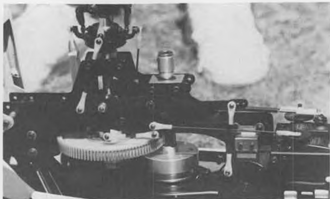
Inside Dobashi's helicopter. No driven tail rotor. Torrington bearing engine starting system. No push-pull control linkages. The large servo wheel is for collective pitch. It is very plain and simple! It proves that it's skill that wins.
