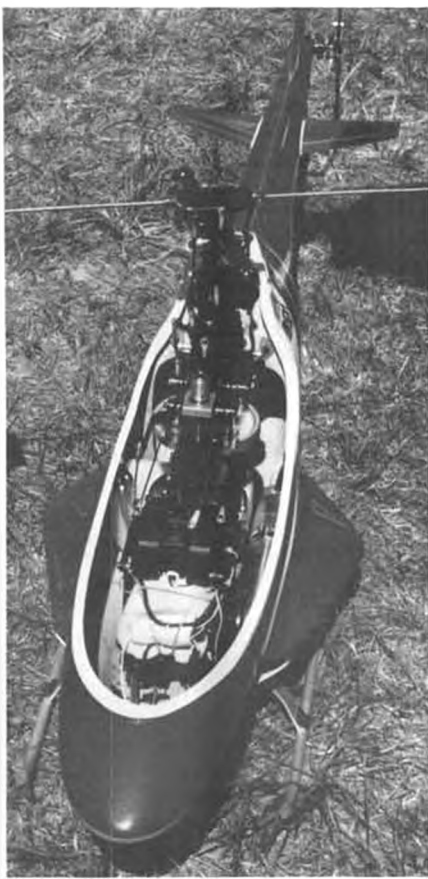
Very slick looking fuselage. Muffler on the left side of the fuselage. Note the air cooling intake scoop at the front of the stubby wing. Small wing like this may improve longitudinal stability without unloading the main rotor thrust.
