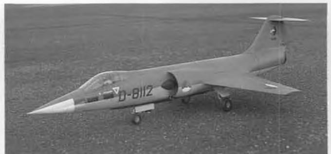
Jim Harrison's super Thorpe F-104. Thorjet fan, OPS 65. Very fast, but doesn't seem to benefit from engines over 45 size.
