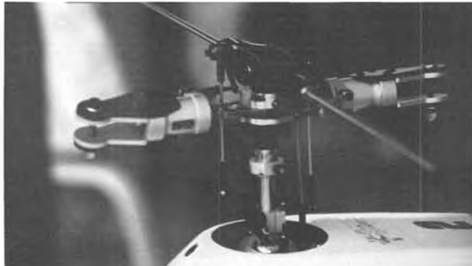
Closeup of the TSK H-30 hingeless rotor design. 44,000 yen, or US$340 just for the rotor head. The spring steel flexbeam gives slopless, no dead-band, linear cyclic control response.
