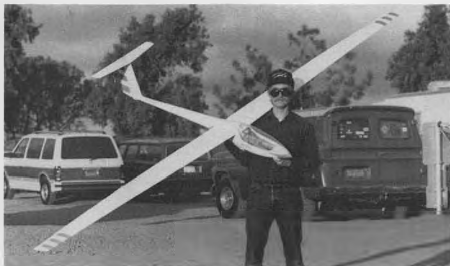
Bill Liscomb and his 1/5 scale DG-202 with thinned Eppler 374 airfoil. 1/4 scale also available.
