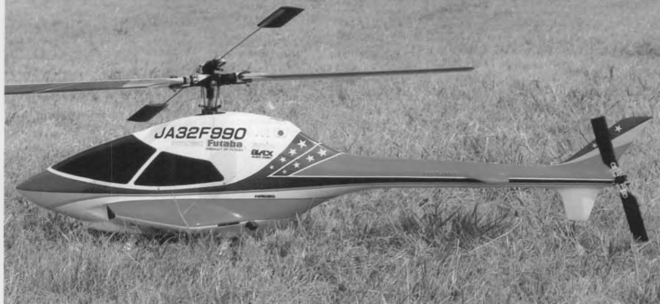
1989 F3C World Champion Dobashi's model helicopter. Hirobo mechanics, Hirobo SSR rotor head, and Korukawa aftermarket brand fuselage. Soft teetering head and heavy, thick Hiller paddles give smooth flight characteristics.
