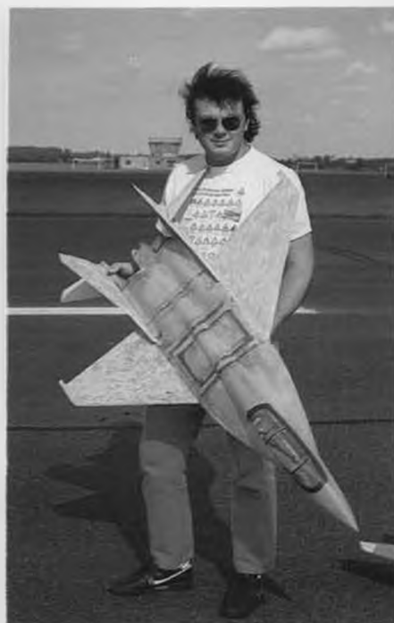
Trestrall's pilot, Paul Leighton, with third prototype two-seater MIG-29. Weighs 7-3/4 pounds ready to fly.
