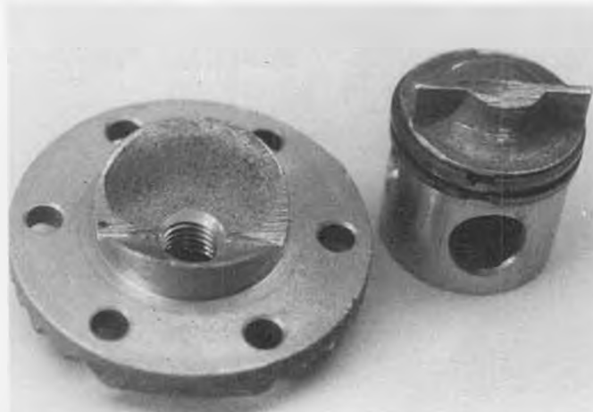
Stu sez each KOMETA MD5 should come with a fine file for finishing. The piston hit the bottom of the cylinder head as this engine was turned over. Note the dual piston rings with "Z" ends. Perestroika may put a halt to this engine's production.
