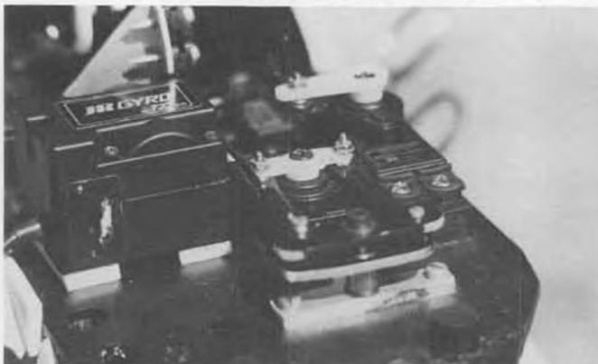
The roll servo commands go to a push-pull setup first, then back to the washplate bellcranks. Note the ball joints are all located under the servo arm to minimize torsion exerted on the servo output shaft.
