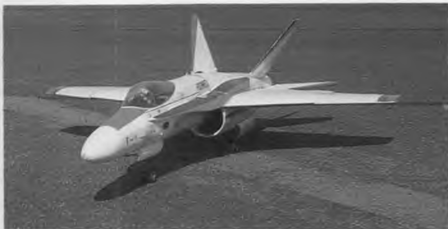
Paul Thorpe's F-18 Hornet. Now eight years old Picco 80, Thorjet 9-blade Micromold fan. Balsa, ply, and foam construction, 12 pounds.
