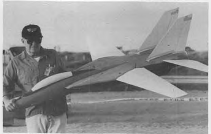
Bob Reynolds "Top Gun" fuselage F-14 with oversize flying surfaces. Model features only elevon for control.
