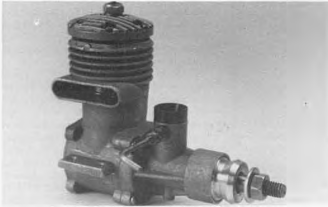
The Soviet KOMETA MD5 is a .29 glow engine. MB reader Jim Donick was lucky to get a marine version before his U.S. employer transferred him back home from Moscow recently.
