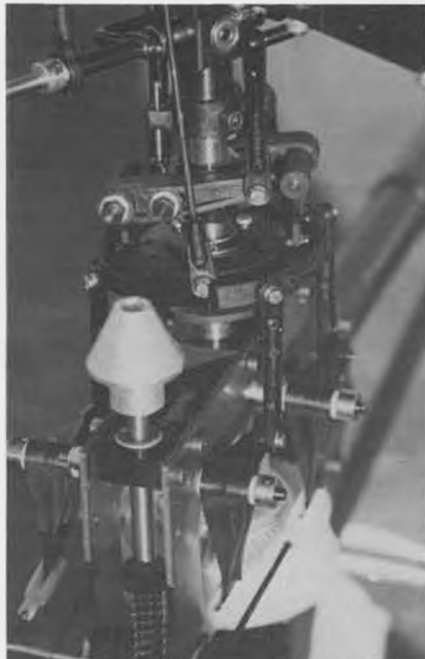
The swashplate is supported at 4 points with 4 bellcranks. Delron bushing mixer is very free. Spring loaded starting shaft and cone pops up after the electric starter is lifted. This reduces vibration.
