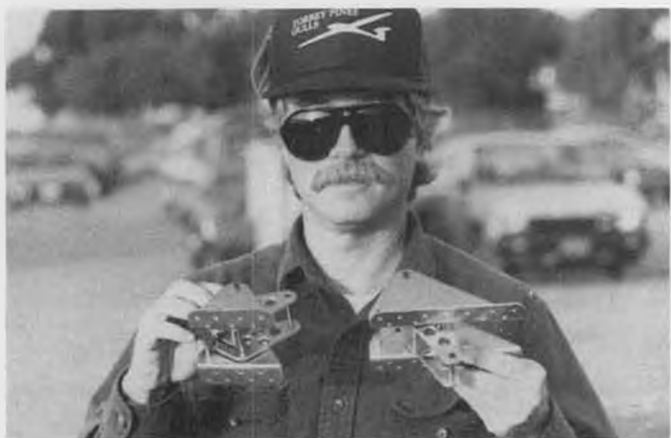
Bill Liscomb and his scale retracts in 1/5 and 1/4 scale. Many models at the meet used his retracts. NOTE: One retracted, the other extended.
