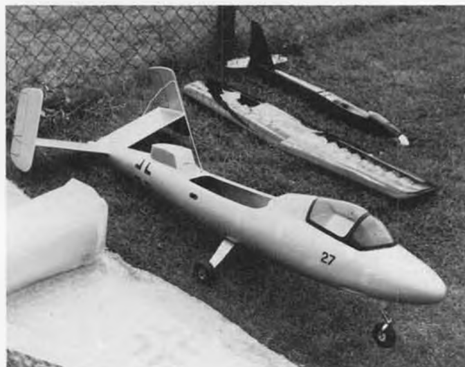
Karl built the plane from a Bauer kit, the ducted fan is also from Bauer. Fuselage shows plenty of room for larger cells.
