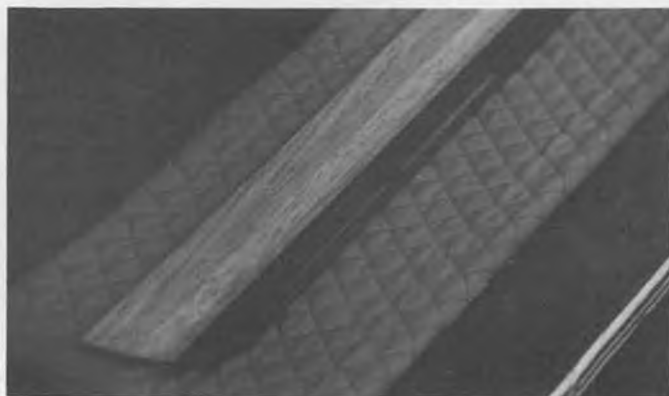
Dobashi's wooden main rotor blade with lead weights. Entire blade was covered with fiberglass cloth and polyester resin. The dark color leading edge is actually made up of about 30 laminations of hard wood.
