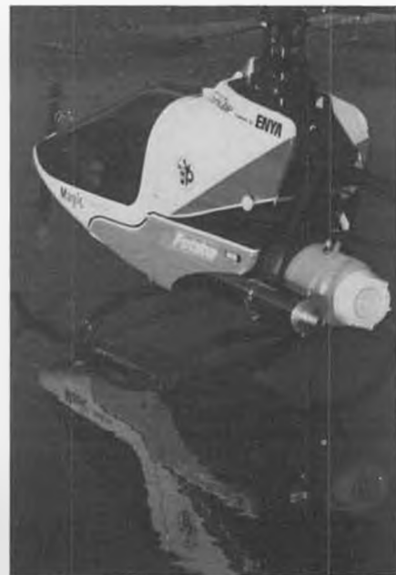
The canopy is specially designed for the Schluter muffler. The large fuel tank provides over 20 minutes of flight time. Wide skids prevent tipover.
