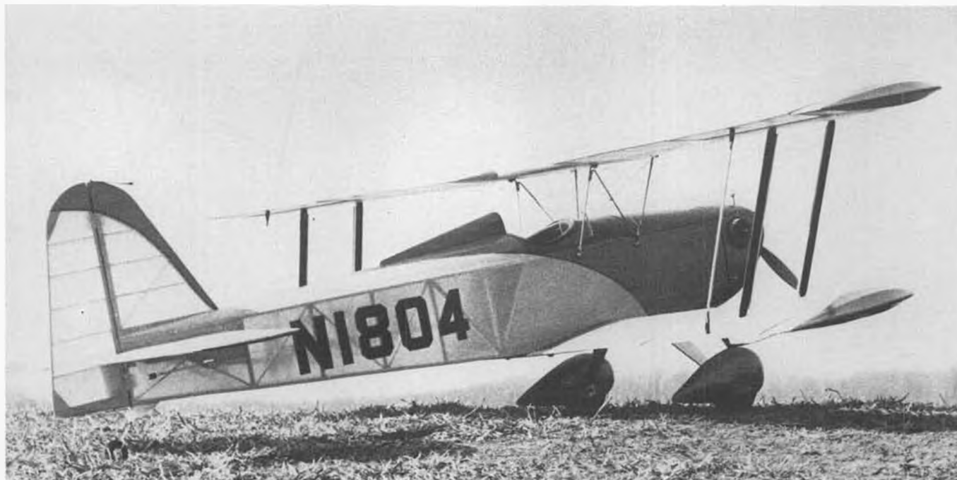
Always a sucker for that transparent finish, we covered the Goose with yellow Silron, used many thin coats of clear nitrate, added blue butyrate trim and black butyrate numerals, then finished with several coats of butyrate clear. Rudder area has been enlarged for better knife-edge flight.
