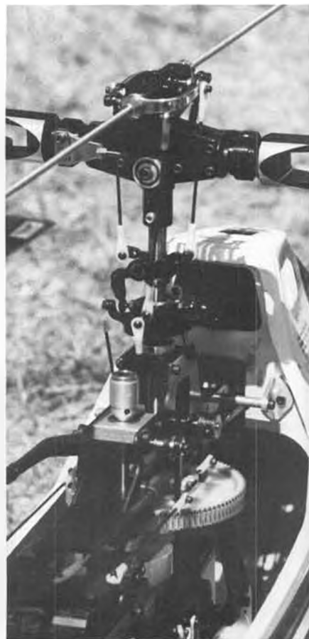
The Hirobo SSR (Super Sharp Response) single teetering rotor head. Pitch control bellcrank is on the left side. An extra I-arm is added to prevent pitch change when collective pitch is varied.
