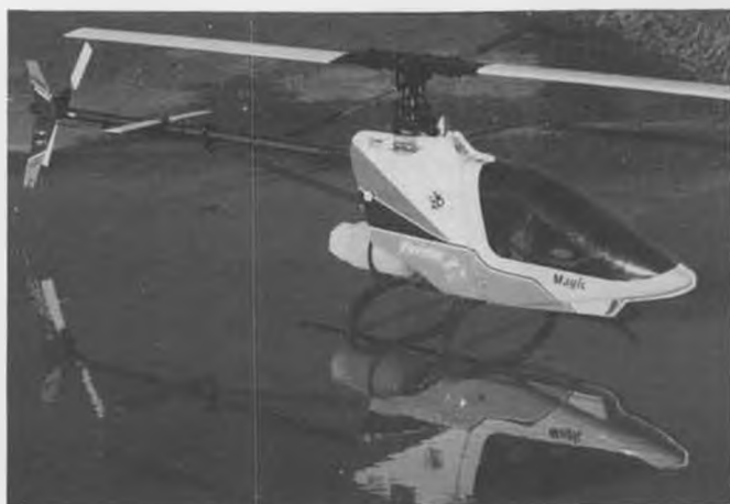
This is one of the smoothest hovering and flying model that we have tested. At 58.7" diameter main rotor, it is one of the largest 60-size pod-and-boom helicopter. It will even fly off (shallow) water!
