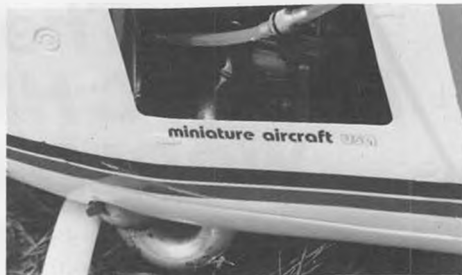
A very tight fit Magna Pipe exhaust system on the X-Cell Long Ranger.
