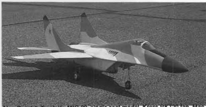
Alex Cornish Trestail's MIC 29, single seat model. Kress RK720 fan, Mac pipe, OS 25. Dolly undercarriage with steerable nose wheel.
