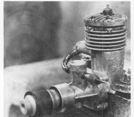
Notice how the KOMETA's prop driver would scoop dirt into the front bearing. Fuel poured out the front bearing (see the drop that's formed?) as it ran. Vibration was so violent with a 9-4 prop that a Richter Scale in Central Florida would have gotten a reading!
