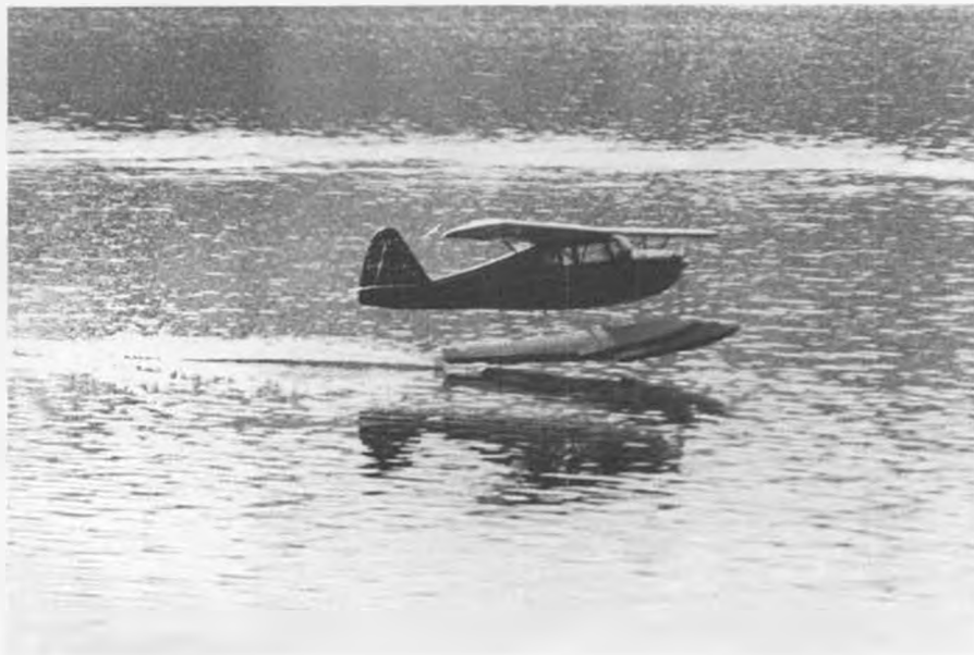
Bob Benjamin's Porterfield on floats. Pulled around by a geared Cobalt 25 swinging a reworked Zinger 13X6-10 . . . excellent flying machine. Bob built a new wing with a thicker airfoil (12%), Phillips entry and ailerons.
