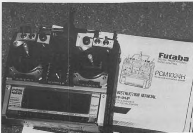
The Futaba 9VHP helicopter radio has almost all the features that you can dream of and more. The instruction is clearly written. The LCD screen prompts you for easy programming. Programming is done with the 10 keys under the screen.
