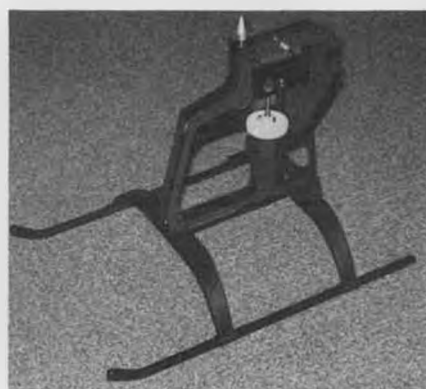
The main structure and tail boom are anodized metallic red. The frames have channels running on the inside that make the structure very rigid. If the kit is built according to the instruction, gear mesh will come out perfectly.
