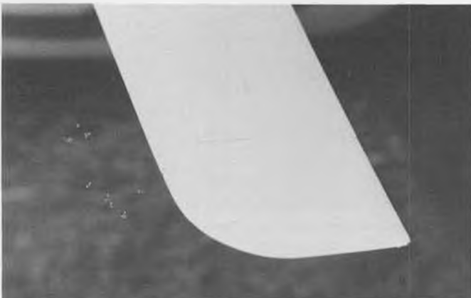
Swept tip on Tim Scloonard's Long Ranger. Swept tip reduces profile drag and consequently reduces engine torque needed.
