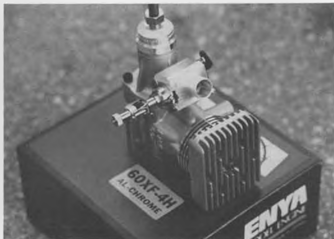
The Enya 60XF-4H Aluminum Chrome engine is used in our Magic. It's a non-ringed engine, and there is plenty of power. Very smooth idling.
