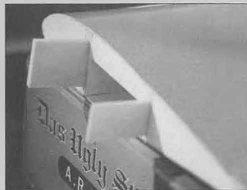
These ARF wing joiners are alarmingly short, and may give way during violent maneuvers.
