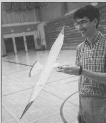
Bob Randolph and his winning F.A.I. Microfilm model, a result of much testing and refinement. It consistently logs flights of over 40 minutes.
