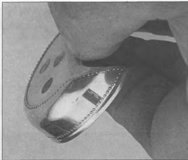
(Left) This 1912 Clement Bayard Peanut by Wijand De Joode of Holland was constructed from plans by Benno Sabel of Germany. (Tondra Alfery photo) (Right) Peanut Fokker triplane cowling by engraver Sam Welch features 142 hand-made .010 diameter rivets and tiny nameplate.
