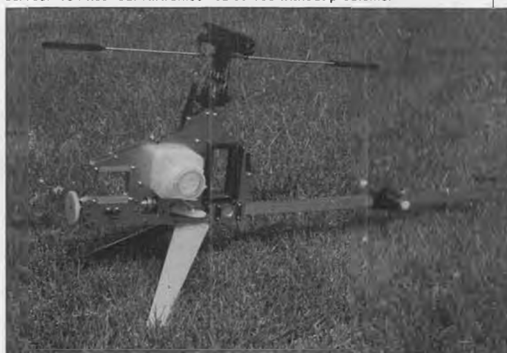
The completely assembled main structure includes the metal side frames, metal tail boom, aluminum dural struts, main rotor, rotor drive mechanism, engine mount, fuel tank and servo tray. The thing on the tail boom is for supporting the plastic fuselage shell.
