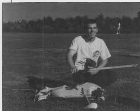
Peter Cooke, the ace helicopter and airplane pilot at James' field, decided to give the Whopper a shot. He had three successful flights, but on the fourth, the engine lost power and the Whopper sank slowly to the ground. Wang had to built another balsa tail! The moral: use a healthy 60 engine. Autogyros will not tip stall like airplanes, they just sink gradually to the ground.
