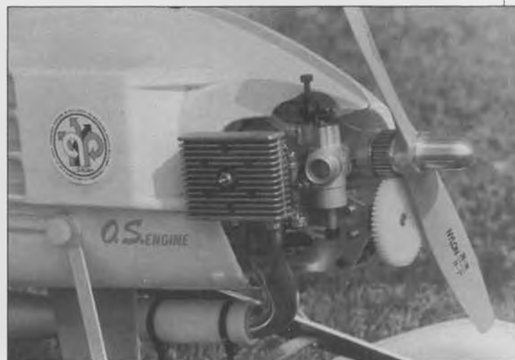
Closeup of the engine and rotor drive gear. Even though the nylon gear is constantly being driven, it can slide forward or back. When it slides back, the main rotor is driven by the engine. A fifth servo is needed to control this. James used an O.S. 61 SFH engine with Robbe header and tuned pipe. A very strong .60 and 12-6 prop is recommended.
