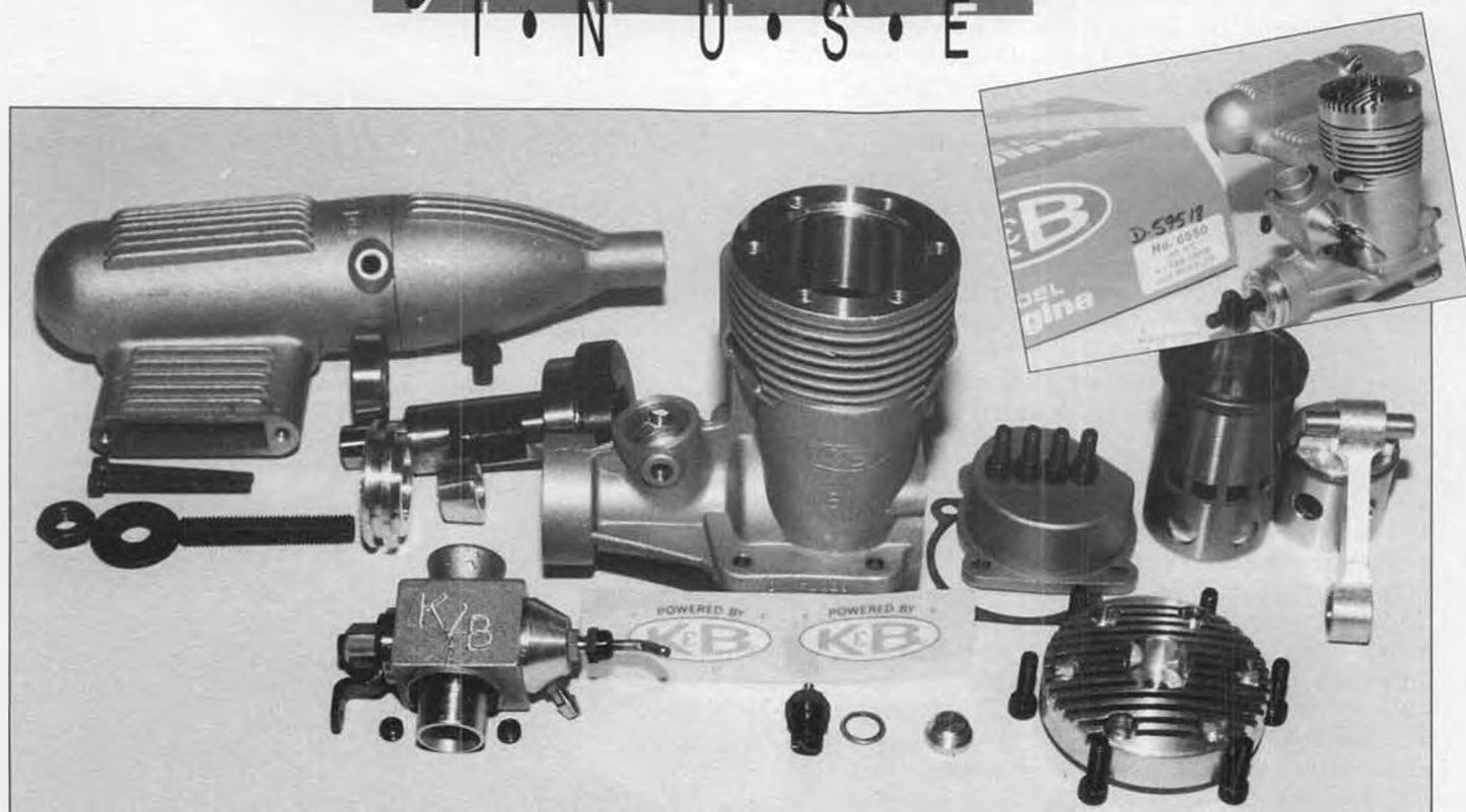
Teardown shows the glitter/glamour of modern CNC machining. Upgrades include a split collet for a truer running prop drive washer, larger bypasses for more power, new high tech rear ball-bearing, and other subtle improvements. (Insert) The K&B .61 RC engine has been in continuous production in the USA for over 20 years. It is fully guaranteed against defective materials and/or workmanship for 90 days.
