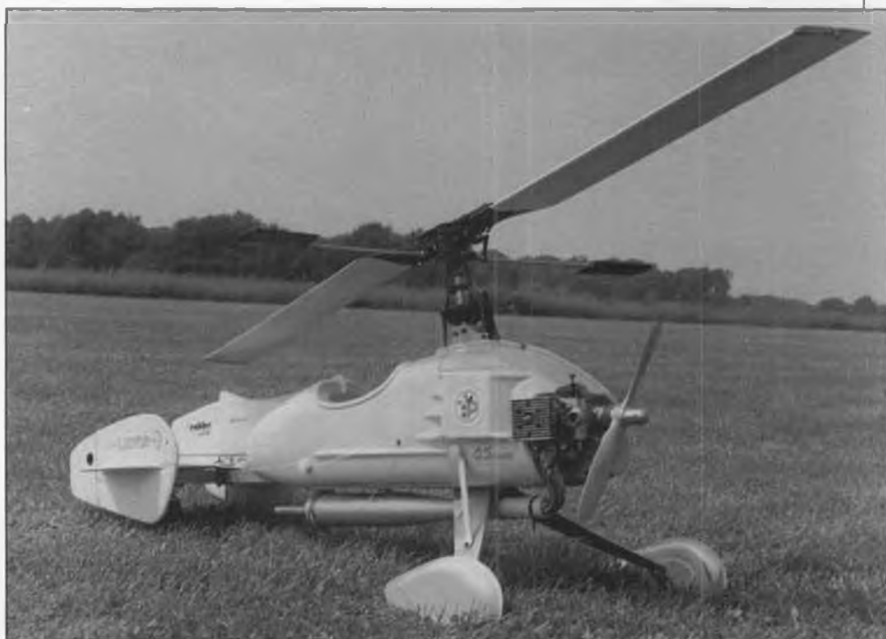
The author's Whopper before the first flight. The rotor span is five feet and it weighs 10 pounds. It is powered by an O.S. 61 with Robbe special tuned pipe and header designed for the Whopper. Radio is the Airtronics Vanguard 6 FM with five servos used. The main rotor is driven by the engine for takeoff, but windmills freely while in flight. Aircraft's pitching and rolling motions are controlled by helicopter-style swashplate cyclically varying the blade pitch angle to tilt the rotor disk. A slow but stable flying model. Requires diligence on takeoff. Note that even though the rotor blade is three inches above the vertical fin, on a bad takeoff or landing, the blade can come down to strike the fins. The author has rebuilt the balsa tail a couple of times already!
