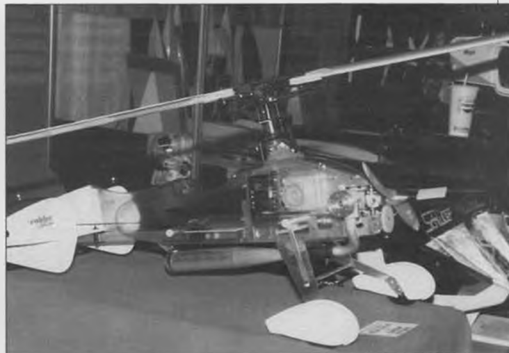
The completely assembled Whopper before the clear fuselage is painted. This one is Robbe's display model. Robbe sells a special tuned pipe and header designed for the Whopper. This header is highly recommended because conventional pattern plane style headers will not clear the fuselage. A muffler also will not clear the fuselage. But you can use Robbe, MAC or Hatori pipes with Robbe's header.
