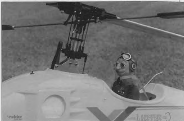
The Ace 1/4-scale "Captain Eddie" pilot in Dave's Whopper. The wire sticking out behind the pilot is a Deans base-loaded antenna, highly recommended to replace the long, dangling receiver antenna. Cut out on the fuselage side reveals fuel tank. The swashplate and main rotor is the same as on Schluter model helicopters. Cyclic controls are used to control the tilt of the main rotor. Only very sophisticated full-size autogyros have cyclic controls!
