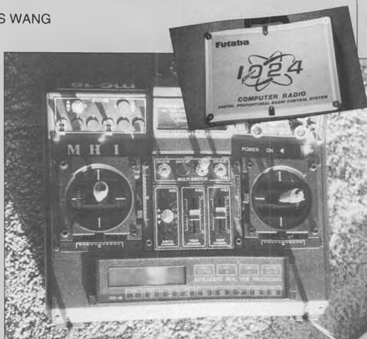
The European version of the JR programmable helicopter radio. The Euro radios are shaped like a tray. Note two brackets at the bottom of the transmitter for neckstrap. (Insert) The metal transmitter case is a very good investment to protect those modern programmable transmitters with toggle switches sticking out everywhere. James bumped off one of those switches, and including shipping, it cost $40 to replace the switch.
