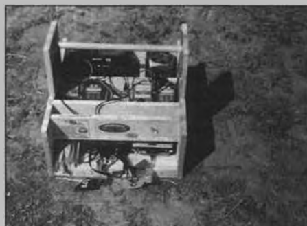
Bob Taylor's homemade electric flight box. Note the room for two transmitters and a car battery. Astro 112 charger on the left, 115 on the right, and digital voltmeter in the middle.
