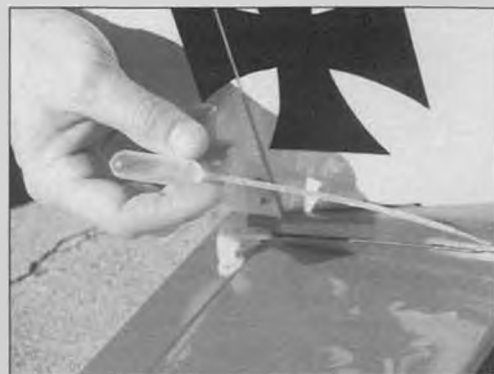
The amazing CA applicator from Art Gross Enterprises. This little squeeze bulb puts the glue exactly where you want it with absolutely no waste.
