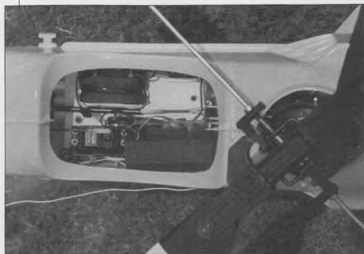
This top view shows the Airtronics Vanguard 6 FM receiver, battery and rudder servo inside the pilot cockpit location. Mount the switch here for easy access. David has a dummy Ace pilot mounted here, too.
