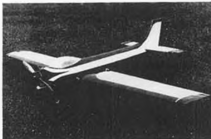
No. 10751 THE LITTLE ONE $8.00 Economy size, .40 powered pattern ship has rolled ply fuselage. By Dick Sarpolus.
