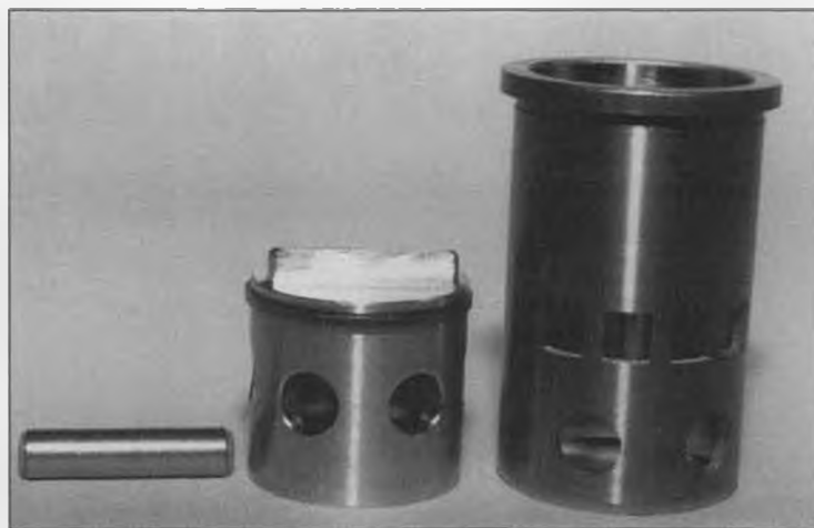
Text explains how to avoid getting a cylinder in backwards, and other helpful tips. Teflon pads on the wrist pin (left). Inner bore of the cylinder (right) is chrome plated.
