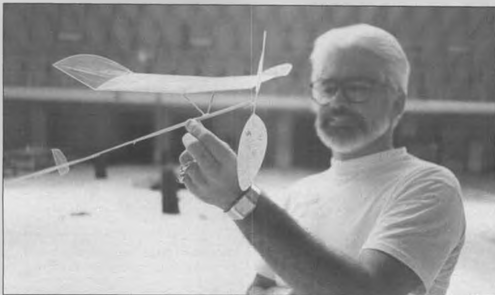
(Above) Underside of the Walt Mooney/Dick Baxter ornithopter model. (Left) Beautifully built Easy B model by Bob DeBolt. Notice the V-shaped wing posts, which prevent downthrust due to motor stick bowing under heavy rubber winds.
