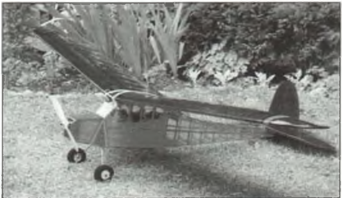
■ LEFT: The Solar Eclipse is Jerry Smartt's "solarized" modification of an Airtronics Eclipse motorglider—wing contains 30 solar cells which power the motor through a four-cell NiCd buffer battery in the fuselage. ■ RIGHT: One of the best possible RC trainers and also a real threat in seven-cell O.T. electric competition is the Cleveland Playboy Sr. Vince Masa built this V-dihedral cabin version (could also be built with a pylon fuselage and/or a polyhedral wing) from an old Leisure Electronics kit. Leisure kit designs are now being produced in Canada—see text for details.
