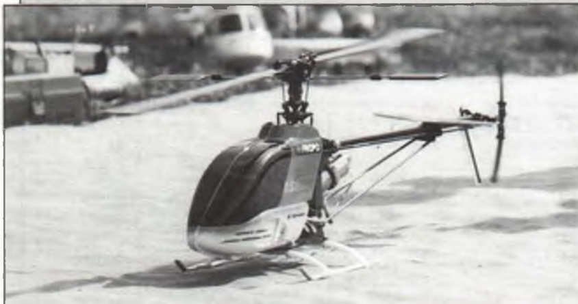
Curtis Youngblood's X-Cell 60 Custom. He's using Miniature Aircraft's extra large horizontal stabilizer and optional large, weighted paddles for improved forward flight stability. Note the 1/4-inch graphite arrowshaft used for tail rotor pitch control.
