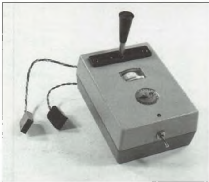
The Servo Driver JSM from Custom Electronics, a useful tool for testing for proper servo operation and installation. Available with or without connectors.
