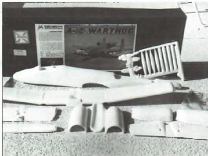
■ LEFT: The A-10 Warthog kit as it comes out of the box. ■ RIGHT: For simplicity, Art chose to go with a single rear-mounted pusher engine—in this case, a YS .45, on account of its power and built-in fuel pump. For more ambitious modelers, two Kress RK-720 ducted fan units can be mounted in the engine pods.
