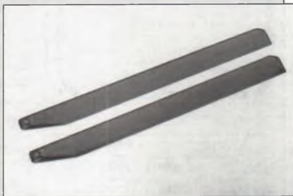
The graphite main rotor blades used by Curtis. The blades have a symmetrical airfoil and slightly swept tips, and are custom made by MHP in England. They are now exclusively distributed in the U.S. by Horizon Hobby Distributors.
