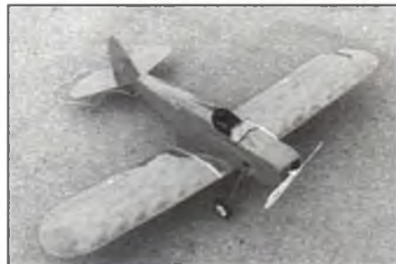
Nice building job on this Davey Systems Flybaby by Bob Grindle. Motor is a direct drive Astro 035 on six cells. Story in this month's column illustrates the importance of building light.
