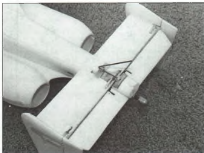
■ LEFT: Underside view of the tail shows the sturdy wire tailskid which protects against propeller damage. ■ RIGHT: View of the Warthog's belly shows the standard fixed gear installation. If installing retracts, they'd go inside the clear plastic wheel pods. Note also the functional flaps—very useful in landings. Art recommends you don't leave 'em off.
