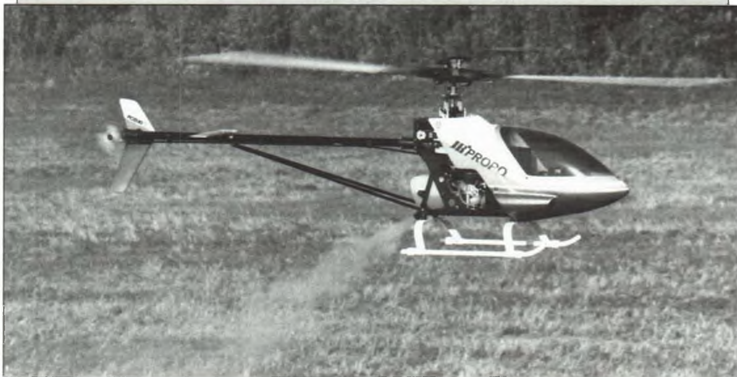
The new .60-size Kait Omega Grand Prix was flown to a 2nd place win at the 1993 F3C World Championships in Austria by 1991-92 World Champ, Kazuyuki Sensui of Japan. Model has modular aluminum side frames, an extra long tail boom and metal 10-S11 teetering head—and that's just for starters. More in text.
