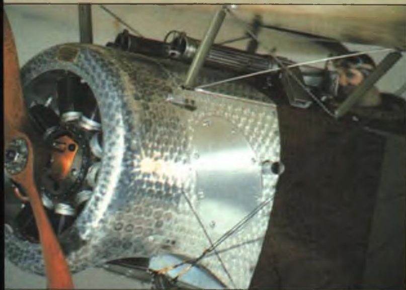
■ ABOVE: Incredible cockpit and Vickers gun detailing on the author's prototype Swallow. He even went so far as to make the pilot's head, stick and rudder bar move with the servos! Many of the detailing techniques used here will be explained in the concluding article next month. ■ LEFT: Dummy radial engine is made up of Williams Brothers Le Rhone cylinders; crankcase is cut out as needed to fit over the Astro motor and gearbox and is held in place with two small screws. Brass plate atop the cowl reads: IN THE EVENT THE PROPELLER OR ENGINE BEING REMOVED, GUNS MUST BE RETIMED.
