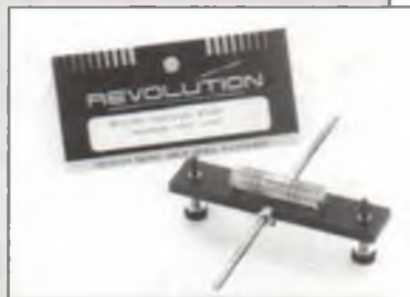
This precision blade balancer is part of the new Revolution line of helicopter accessories from Horizon. Rotor blades bolt to both ends of the anodized aluminum body, then the wire shaft is placed over the edges of a couple of drinking glasses and the blades brought into balance as indicated by the bubble balancer on top.
