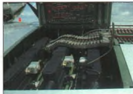
Some warbird restorers go to extraordinary lengths in the name of authenticity; this P-51's wing guns are fake, but note the minute details, including the loading instructions on the door. Photo by Tom Perzentka.
