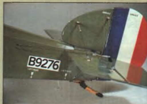
Empennage details. The steerable tail skid (also scale) goes a long way toward making the Swallow handle well on the ground.
