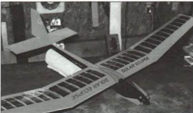
■ LEFT: The Solar Eclipse is Jerry Smartt's "solarized" modification of an Airtronics Eclipse motorglider—wing contains 30 solar cells which power the motor through a four-cell NiCd buffer battery in the fuselage. ■ RIGHT: One of the best possible RC trainers and also a real threat in seven-cell O.T. electric competition is the Cleveland Playboy Sr. Vince Masa built this V-dihedral cabin version (could also be built with a pylon fuselage and/or a polyhedral wing) from an old Leisure Electronics kit. Leisure kit designs are now being produced in Canada—see text for details.
