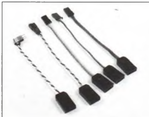
Custom Electronics' receiver-to-servo adapters are available to match most popular receivers and most popular servos without resorting to plug butchering or wire splices.
