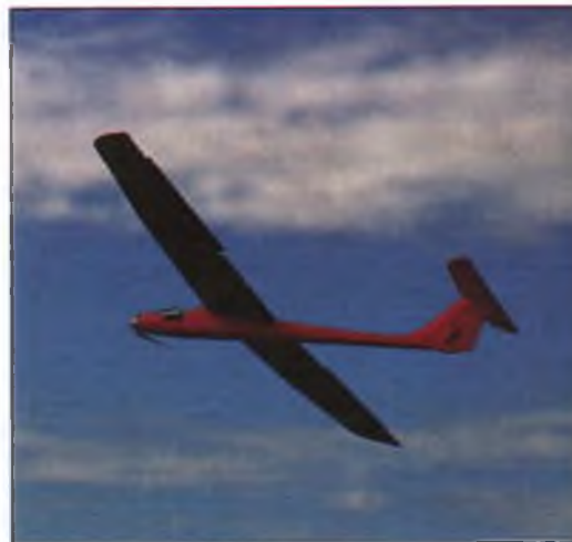
The Calibra cruises by with the ailerons in the spoileron mode. This is one clean airplane, and with a wing loading of almost 19 ounces per square foot and the very fast HQ 1.5/9 airfoil, it doesn't like to slow down. Spoilerons are an effective way of getting the ship on the ground before it winds up in the next county. John Lupperger photo.
