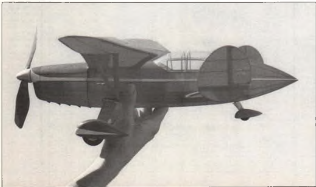
Striking Delanne 20-T-02 tandem-wing by Terry Pittman of Annandale, Virginia spans 19 inches and features Brown B-100 CO 2 power. Plans were based on those from French modeler Gerard Porcher.
