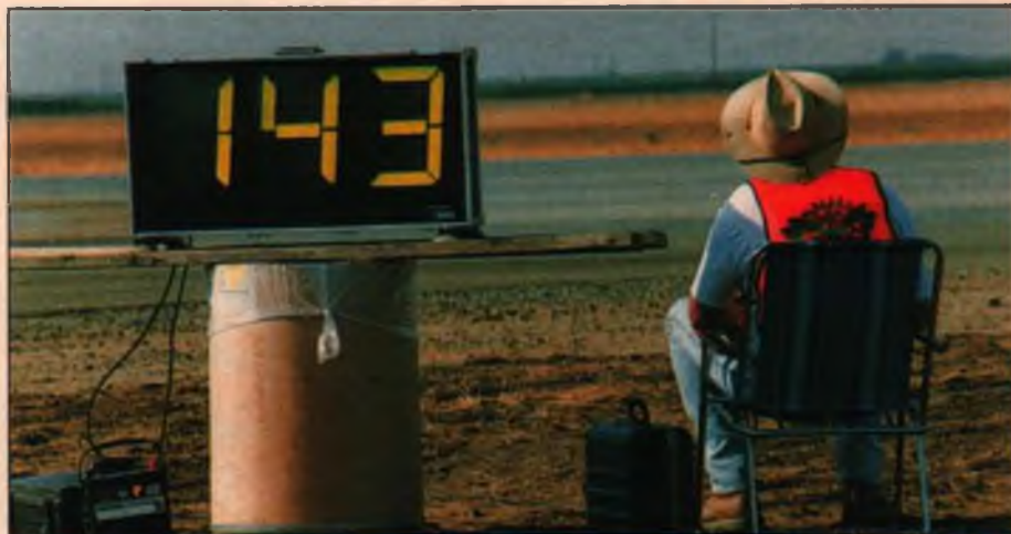
An example of the type of facilities used at Madera—a radar speed gun provides instant display of the models' speed as they fly the course.
