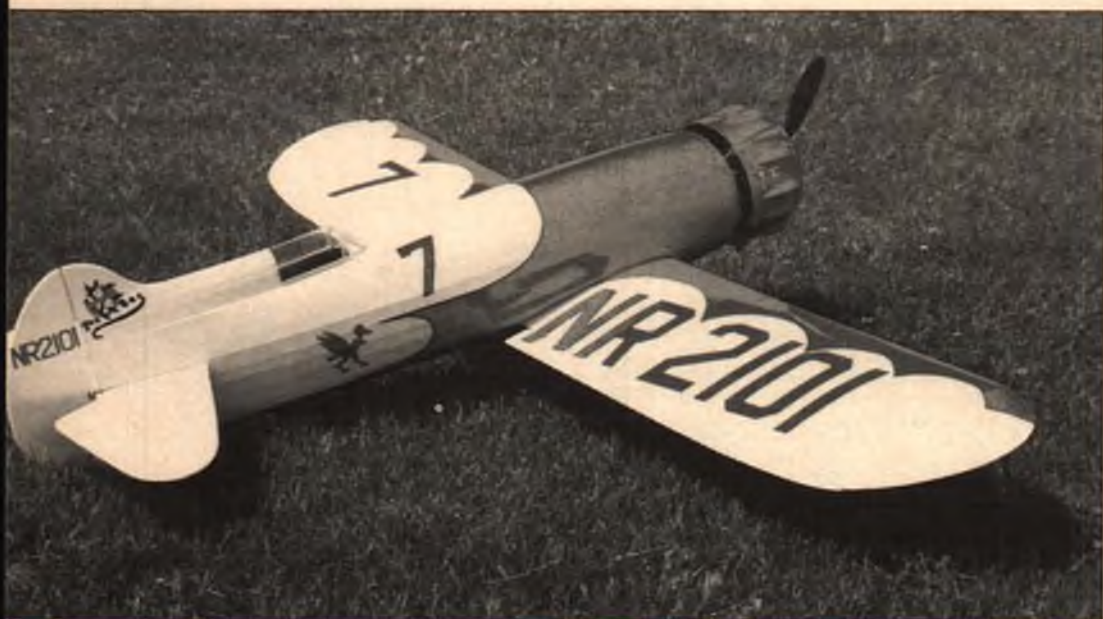
Don't be fooled! Henry Haffke's vivid "sorta scale" RC Gee Bee R1/R2 Long Tail racer is actually a highly modified Peashooter. The 6-1/2 pound model spans 60 inches and is powered by a K&B .40.
