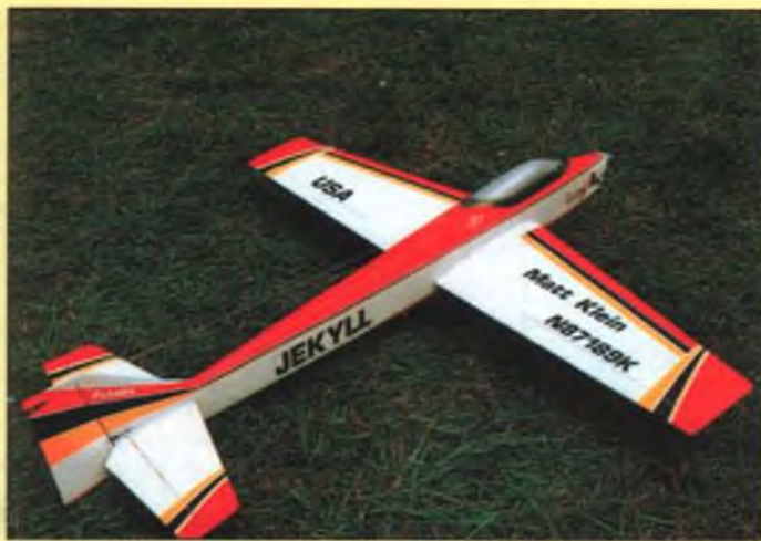
Ohio Masters pilot Matt Klein operates with this RC City Jekyll. YS .81 two-stroke powered, Futaba radio.
