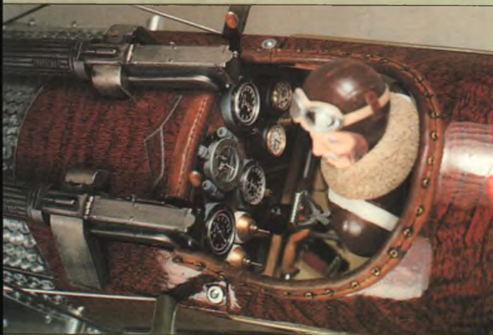
■ ABOVE: Incredible cockpit and Vickers gun detailing on the author's prototype Swallow. He even went so far as to make the pilot's head, stick and rudder bar move with the servos! Many of the detailing techniques used here will be explained in the concluding article next month. ■ LEFT: Dummy radial engine is made up of Williams Brothers Le Rhone cylinders; crankcase is cut out as needed to fit over the Astro motor and gearbox and is held in place with two small screws. Brass plate atop the cowl reads: IN THE EVENT THE PROPELLER OR ENGINE BEING REMOVED, GUNS MUST BE RETIMED.
