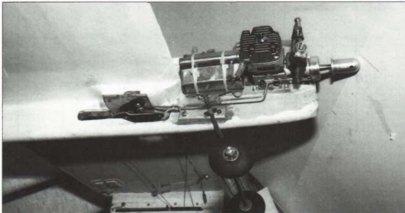
Orin Humphries' old reliable Curtiss Seagull Profile Carrier ship has all of its controls mounted externally—a good way to go for your first three-line model, as everything is accessible and easy to work on.
