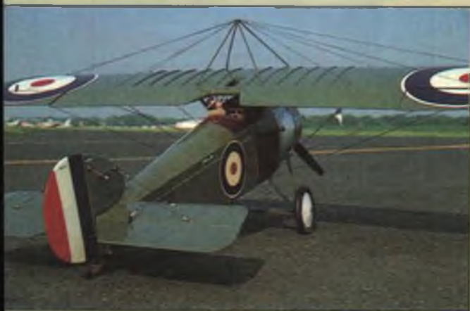
■ ABOVE: A 3/4 rear view reveals the 12 scale rib stiffeners and the tiny opening in the wing for the pilot's upward view. Also evident is the typical Sopwith gap under the fin for adjusting the horizontal stab's angle of incidence and rigging. ■ RIGHT: The author (right) and his buddy Dave Baron, who has been the test pilot for the Swallow project from the start. Model was originally flown with an Astro 15, then a 25, and is presently flying with a geared Astro 40 running on 18 cells. Loops from level flight are no problem with that much power, and the model easily cruises at half throttle. ■ FAR RIGHT: Disassembled nose section shows many interesting fitting details. The dummy carburetor intake pipe on the fuselage side slides in and out and serves as the electric power system arming switch. Here the geared Astro 40 has been set in place and is waiting to be strapped down securely with rubber bands.
