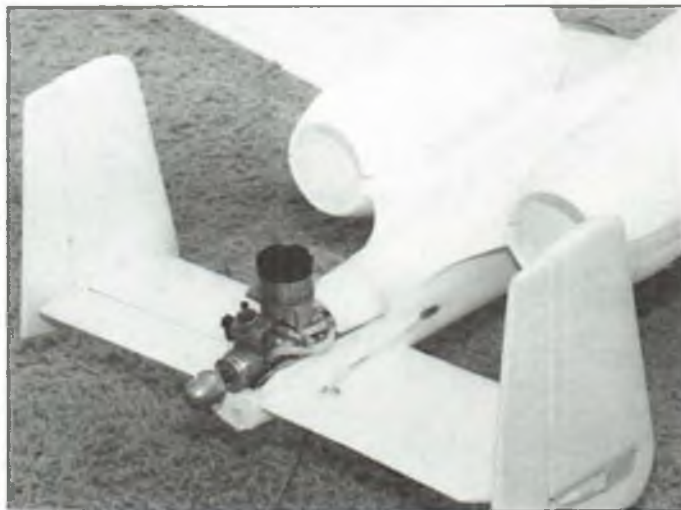
■ LEFT: The A-10 Warthog kit as it comes out of the box. ■ RIGHT: For simplicity, Art chose to go with a single rear-mounted pusher engine—in this case, a YS .45, on account of its power and built-in fuel pump. For more ambitious modelers, two Kress RK-720 ducted fan units can be mounted in the engine pods.
