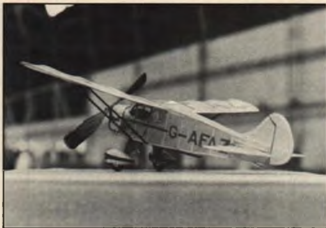
The Wico has nice proportions for stable flight, and the long scale landing gear and high thrustline allow a generous size propeller to be used.
