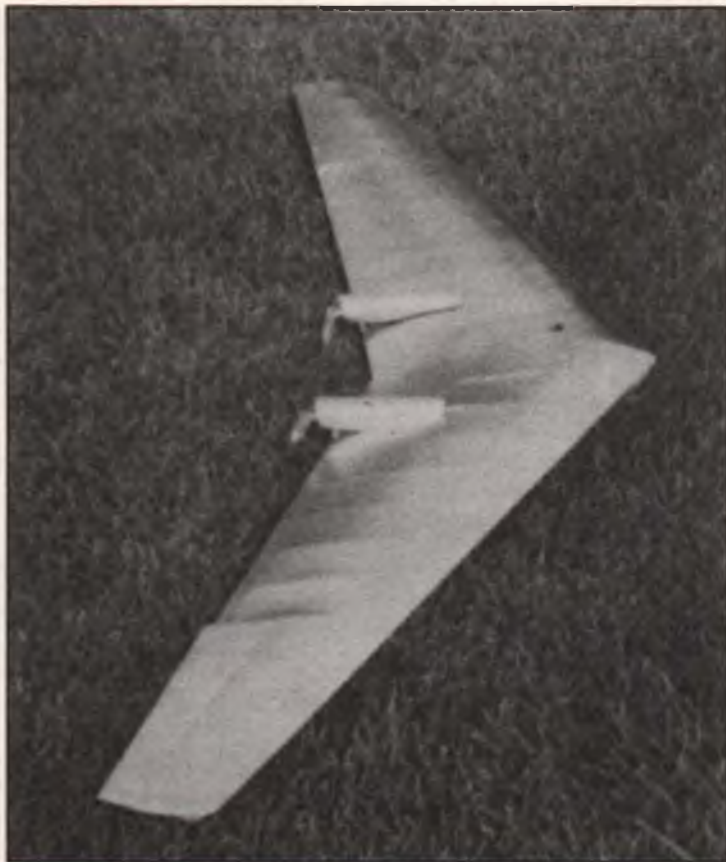
What looks like a Northrop W3M flying wing is actually Bob Taylor's twin electric adaptation of a 2-meter Klingberg Wing sailplane. Uses two Peck-Polymer Silver Streak 035 motors running in series on a 12-cell pack.
