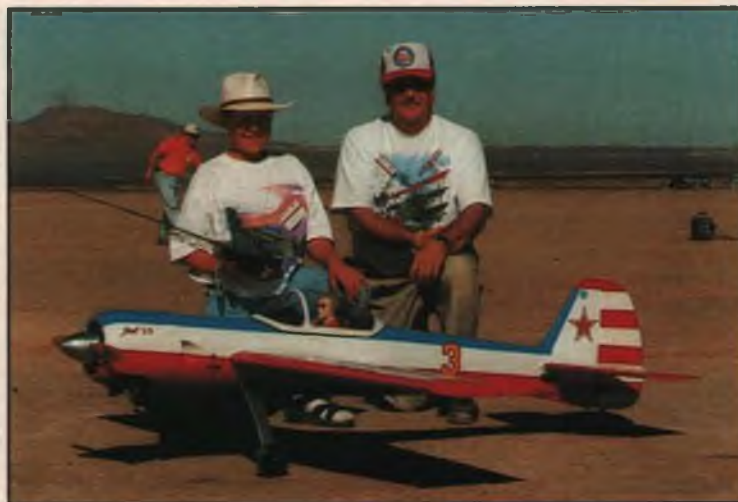
Junior Achievement winner Mark West poses with his caller and his scratch-built Yak-55; 86-inch span, 23 pounds, and a Zenoah G-62.
