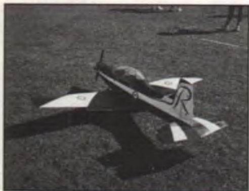
If all goes according to plan, Century Jets will soon be distributing this Pilatus PC-9 in the U.S. Designed by New Zealander Ron Cavanaugh in 1/5 scale, it spans 82 inches, and a Super Tiger 3000 is said to be ideal.
