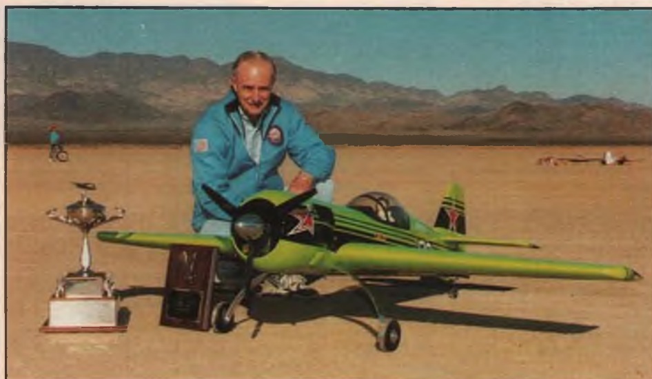
■ LEFT: The award for Best Finish rightly went to Gerald Scheuerman for his flawless Byron Sukhol Su-26M, finished with automotive lacquer. Model spans 82 inches, weighs 24 pounds, packs a Zenoah G-62 under the cowl. ■ BELOW: Even though it didn't win an award, Carl Hansen's well-detailed 133-inch Boeing P-28 is still a remarkable piece of work. If it's not half-scale, it must be darn close. Model is finished in auto enamel, weighs 70 pounds.
