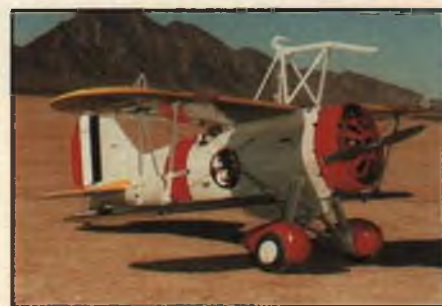
Declared Best Biplane After 1918: Ken Perkins' Curtiss P9C-2 Sparrowhawk, a flawless reproduction built from Cleveland Model Co. plans. Spans 70 inches, weighs 22 pounds, uses an Airtronics radio.
