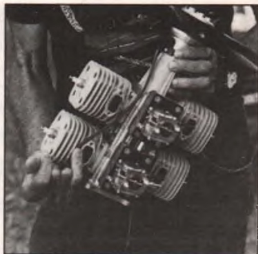
At Snohomish, Bruce photographed this example of 3W Modelmotoren's 160-84 horizontal four—a real brute! It displaces 9.8 cubic inches, and it's not their biggest engine either.
