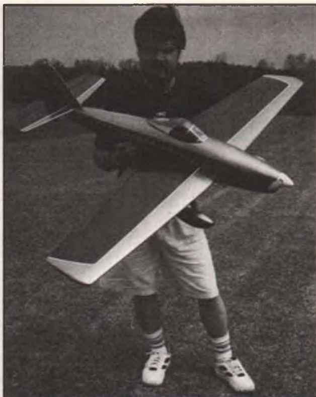
■ ABOVE: The Hummingbird Mk III is the latest in Gene Morman's series of original electric designs. Geared Astro 25, 16-18 cells. Base is obviously a fine craftsman and has turned out a very nice looking and sporty design. ■ BELOW: Jim Ruggiero turned out this simple original design shoulder-wing job, dubbed "Cherry Sandae." Pictured here as first built, Jim later added a 3:1 gearbox so as to be able to swing a much larger prop, resulting in a considerably faster climb as well as a longer overall motor run.
