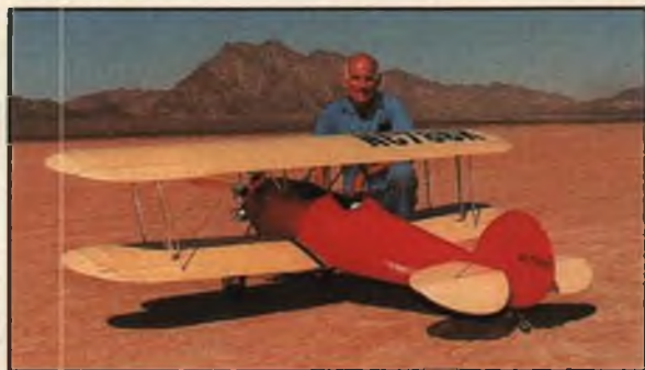
Mike Brewer, who hails from Astoria, Oregon, flew his Nieuport 28 to a Best WWI victory. Model was built from a Proctor kit, is finished in latex paint, is equipped with an Enya VT-240 twin and JR radio.
