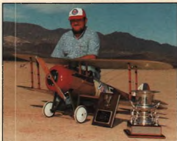
Mike Brewer, who hails from Astoria, Oregon, flew his Nieuport 28 to a Best WWI victory. Model was built from a Proctor kit, is finished in latex paint, is equipped with an Enya VT-240 twin and JR radio.
