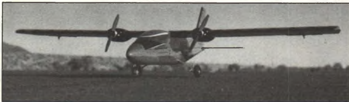
Another of Steve Gurley's projects is a Partenavia P-68 twin kit from Graupner, available in the U.S. from Hobby Lobby. Thrust is provided by two inexpensive Graupner Speed 400s turning Cox 6x3 props.
