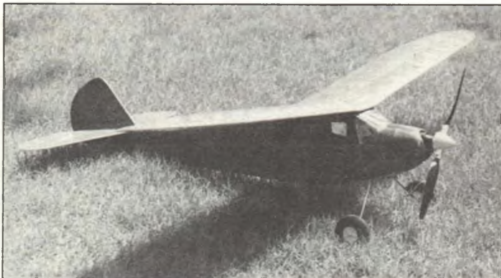
William Whitten's slick little cabin ship is actually a 1936 design by Ben Shereshaw, called the Air Trails Sportster. Midway Models kitted it for .10-.15 gas power, scaling it up slightly to 50-inch span. William's electric conversion includes a geared Astro 15 running on 10 cells—he says it flies great.
