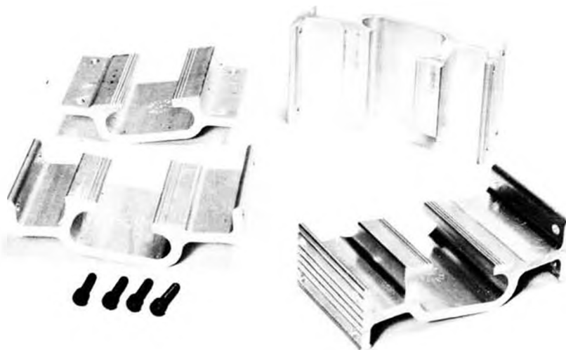
New "Slant 40" engine mount by Octura. Ten degree slant gets exhaust out of boat. Designed to take .19 through .40 size engines. Extruded aluminum, anodized black.
