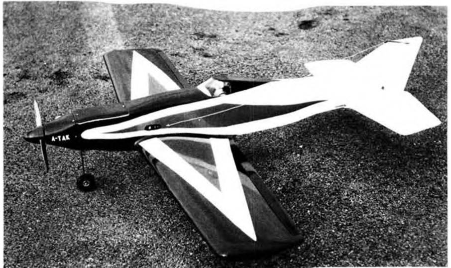
"A-TAK" by MALCO. Has 50" balsa over foam wing. For .40 engines.
