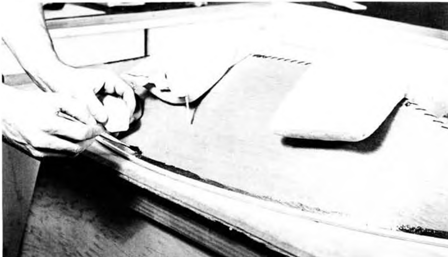
Resin is first brushed onto the keel seam where weights will rest. After placing the weights over waxed paper to prevent sticking, the rest of the keel and side seams are resined. Presto! A hull!
