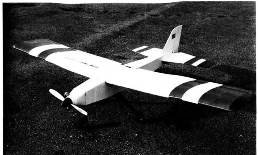
"DER FLUG" by MALCO. Built up 60" wingspan with spruce spars. For .40 engines.
