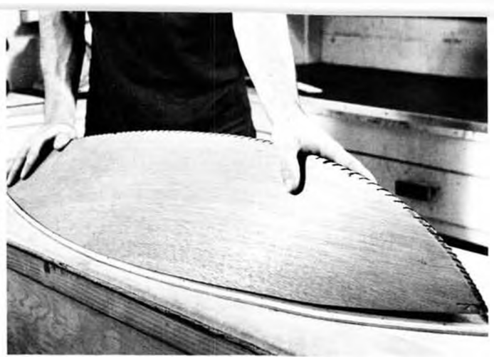
Sides have now been spread apart and pressed down and outward toward side strips. Entire hull of 1/8" Luan mahogany plywood.
