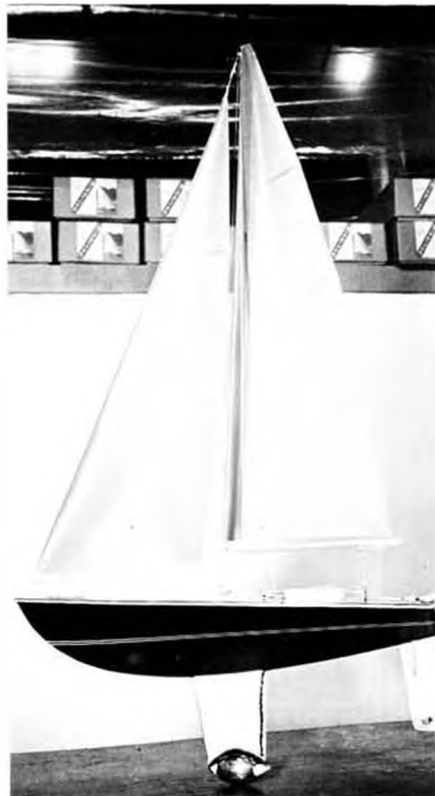
The completed Pea Pod with 4 pound fishing weight for keel ballast. Sails of cloth or plastic.
