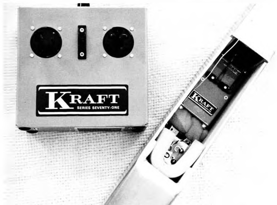
The Kraft 2-channel brick rests comfortably in the fuselage. Balance was achieved without placing the battery pack way up in the nose, though there is room for it.
