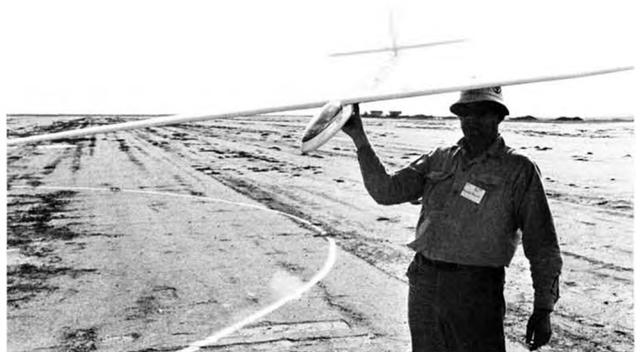
Konrad Nierich holding Tern, designed by Ralph Grose. Wings flex from anhedral to zero dihedral in flight. Ship weighs 7 pounds!
