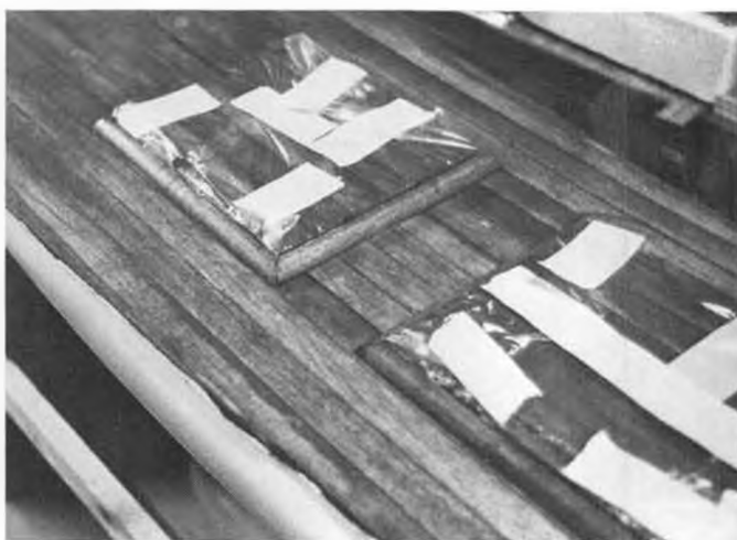
Photo No. 5: Outer coaming in place around "baggie"-covered hatch cover. Confused?
