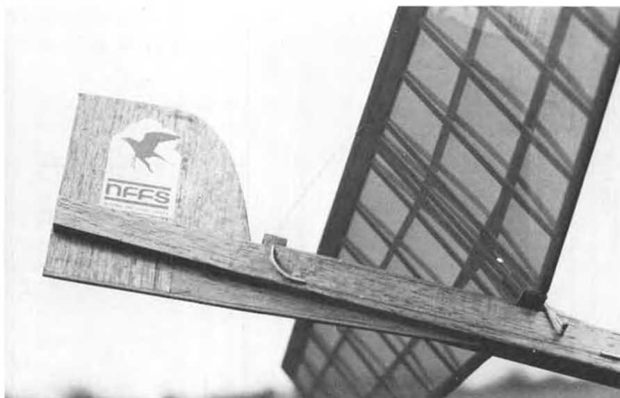
Aft fin version in DT position. In either case, the thrust line comes above the fin, giving a natural right power turn. Glide turn is to the left.
