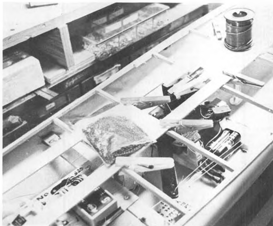
Photo No. 3A: Deck planking just getting started. Center plank laid first for aligning the others. Spring type clothespins are a necessity in model boat building!
