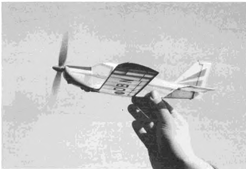
Since hand launching is usually allowed at contests, Walt decided to build this ship with the gear "retracted." Note slight washout in wing panel.
