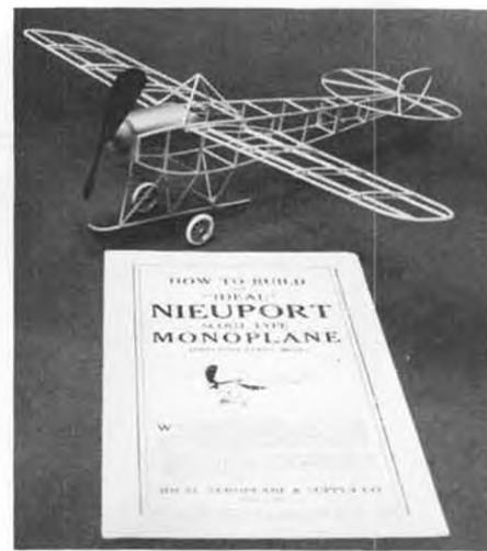
Peanut Ideal Nieuport framework follows original construction.
