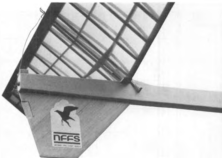
Sub-fin version in the dethermalizing position. Clean, simple construction is a sign of excellent design work. Note left rudder tab on fin.
