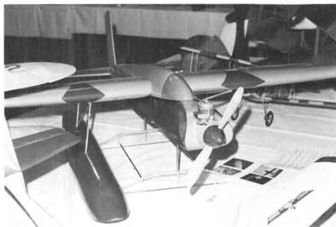
Clever "Seatract" by Francis Reynolds. Floats retract into fuselage sides. Huge hardwood "T" section joins fuselage and wing center
