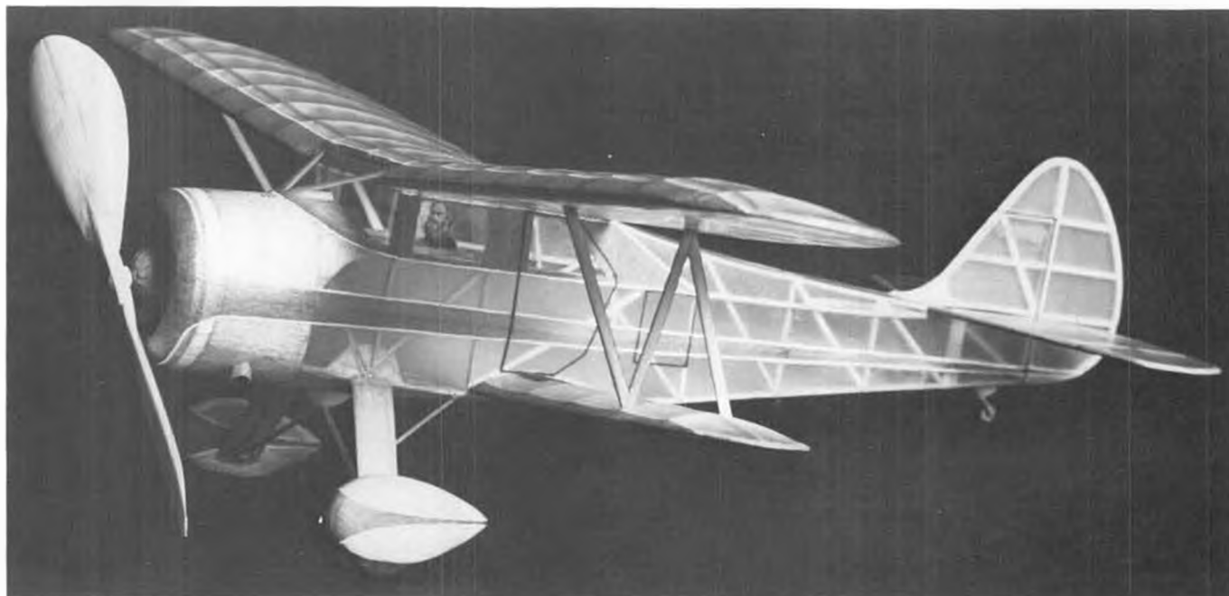
Super indoor Peanut Waco SRE by Ron "Vacuum Table" Williams, built from Micro-X kit parts to plans from Mooney (MB), Berkeley U/C kit, old Waco newsletter. Japanese silk-tissue, clear nitrate, plasticized dope, 8.2 grams. Best flight 45 seconds. High scale points at Glastonbury.
