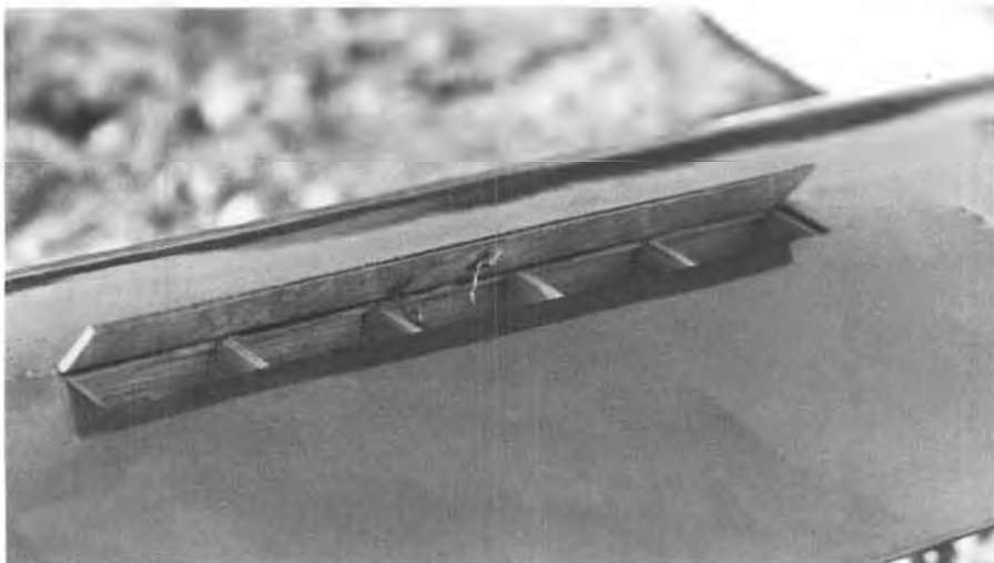
Spoiler mechanism, also by Bob Mickelsen, uses rubber band tension to hold spoiler open, rather than the usual reverse. Servo pulls it down. Spoiler material is counter-top Formica.
