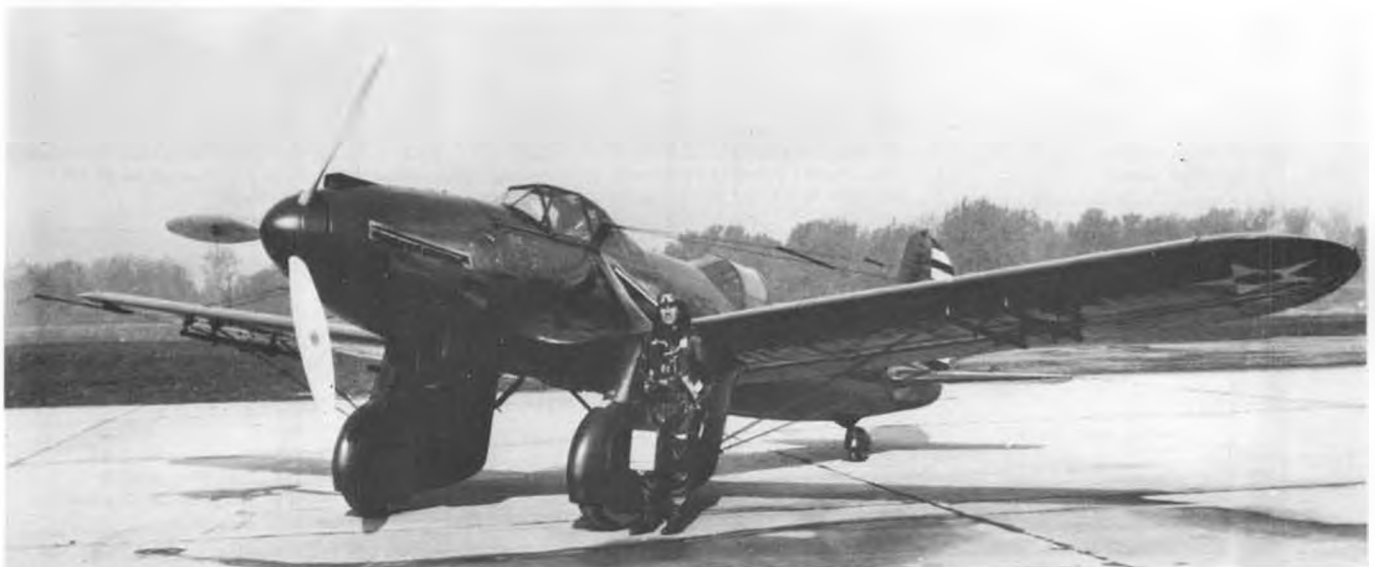
Completely equipped test pilot, with clipboard on leg, ready to test the YA-8A at Wright Field. Geared engine and other mods added 500 pounds over weight of A-8. Nose of this lone geared Conqueror was smoother than regular model.
