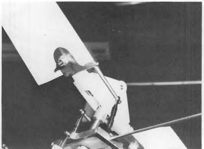
Underside shot shows Delrin main rotor hub, rotor blade attach bracket, and pitch control arm.
