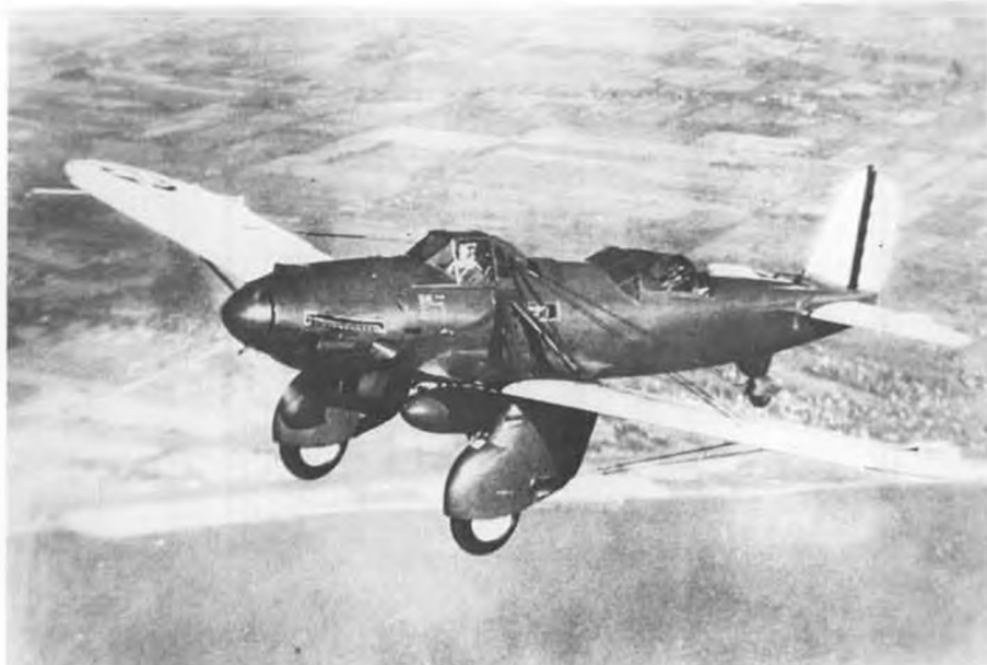
The geared version of the Conqueror, in this A-8A, had reached its peak at 675 hp. Forty-six subsequent Shrikes were powered with the 690 hp Wright Cyclone radial.
