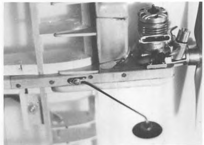
Two photos by D.D. showing his landing gear mounting method for Slow Combat. Reinforcing dowels in motor mounts also show well. Airplane is Dirty's as-yet-unnamed design. He'll call it something after he finds out how it flies . . . perhaps unprintable!
