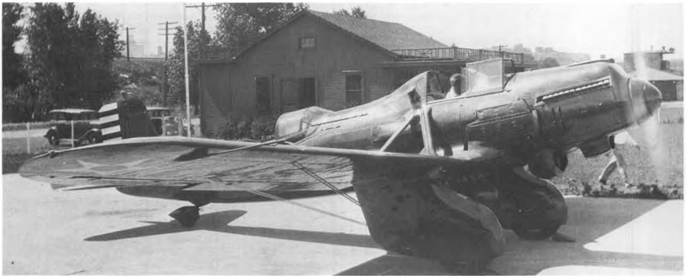
The 600 hp Conqueror was famous for running hot, and additional oil cooling was had by making the ten gallon tank flush with the fuselage contour and adding an air scoop. Note how much more advanced the airplane looks compared to the cars.
