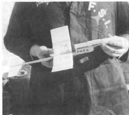
Two photos showing the power pod mounted and removed from the hand-launched-glider fuselage. Most any glider can be used . . . just move the fin to the bottom!
