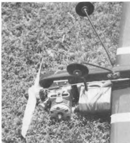
Engine and tank installation.
