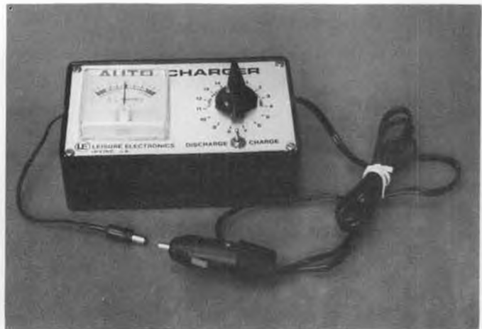
Auto Charger works off car battery, provides controlled discharge and charging of drive batteries.
