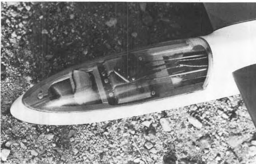
Photo of canopy latch system sketched on next page and developed by Bob Mickelsen, of Clovis, New Mexico. Neat and positive.
