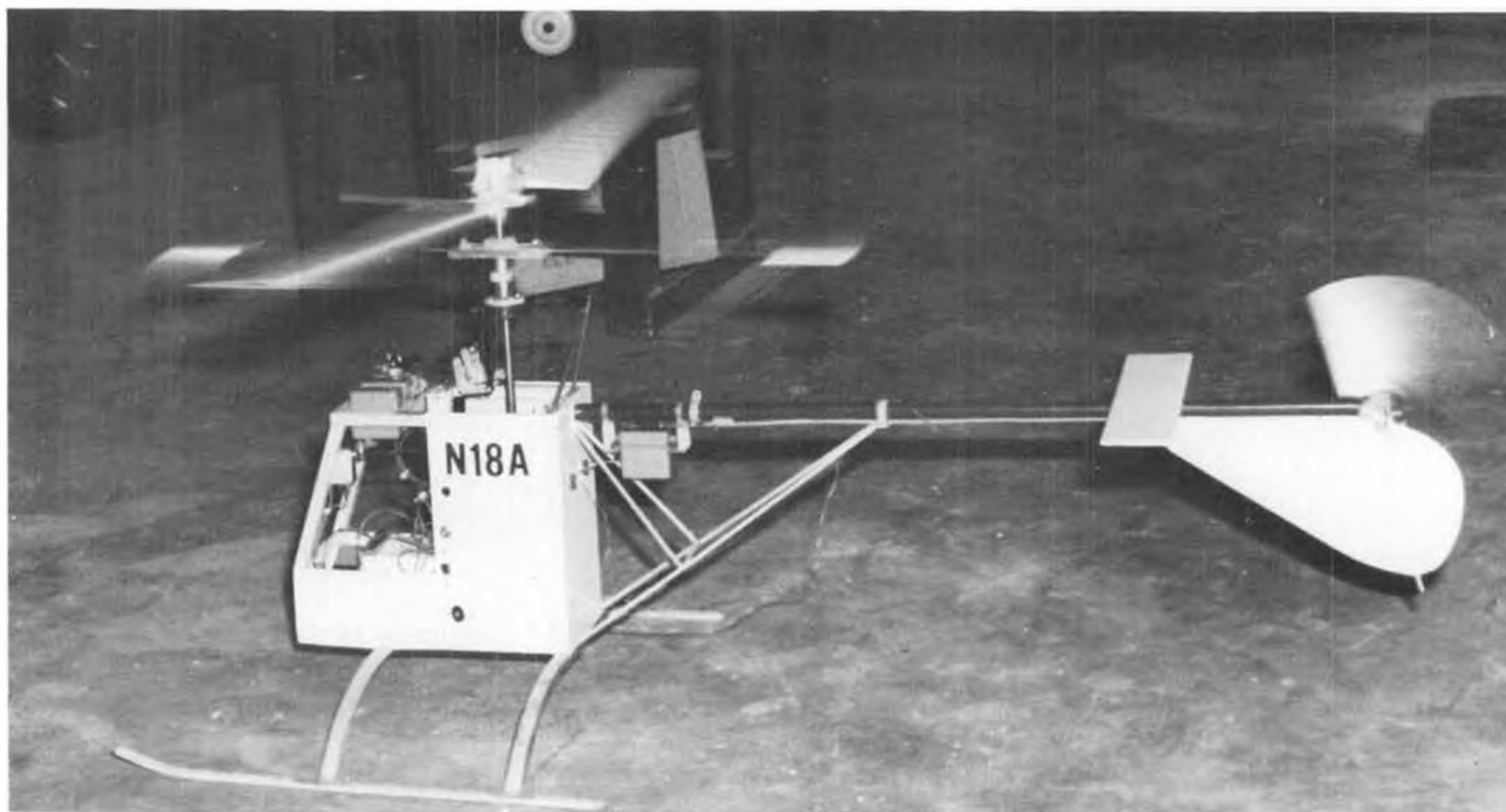
Charlie Gilbert's experimental electric powered chopper gets up a head of silent, smokeless "steam." Power-to-weight ratio is still on the weak side. Chopper will lift off and "swim" around, but does not quite fly. Success is not far away now!
