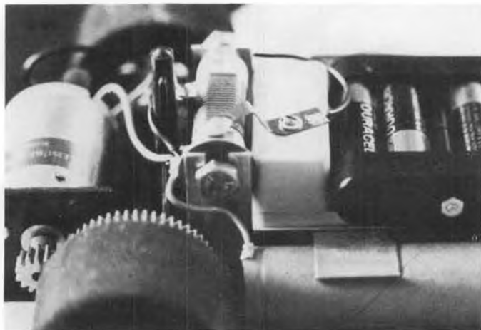
Speed control wiper arm must be adjusted for full sweep. Best that power batteries are discharged or disconnected for this operation!
