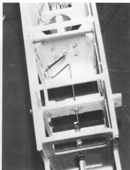
Rear view of actuator mounting shows crank linkage. Loose fit is important . . . no binding.
