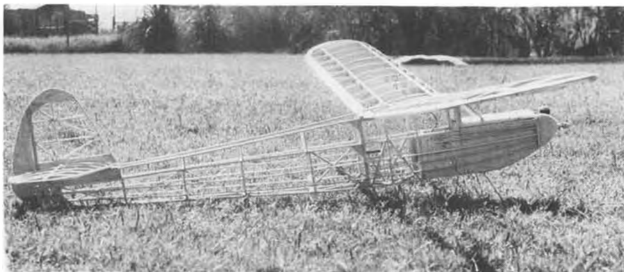
If you don't like pretty framework, this is not for you. As with the original Westerner, the frame features an intricate network of diagonal bracing.
