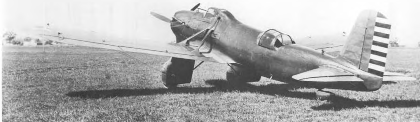
The Shrike was the Air Corps' first all-metal airplane. Fixed rear canopy on this prototype XA-8 was a tight squeeze for the gunner. Looks like you'd have to put on your parachute AFTER you bail out!
