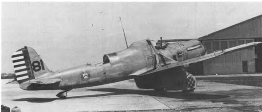
Late in service life, the pylon and rear canopy were modified. This one at Command and General Staff College, Fort Leavenworth, Kansas.
