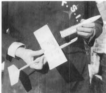
Two photos showing the power pod mounted and removed from the hand-launched-glider fuselage. Most any glider can be used . . . just move the fin to the bottom!
