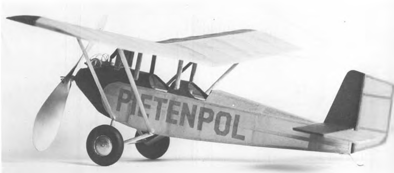
This is Ron Williams month! Built from Peck-Polymers kit, this Pietenpol is covered in yellow, black, and red (letters) tissue, silver struts. Weight 14 grams, almost twice the Waco! Photo by Thorney Leiberman.
