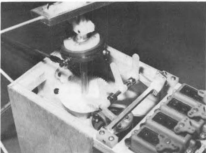
Electric motor is mounted in "V" wedge, driving main rotor bevel gear. Note tail rotor drive take-off.
