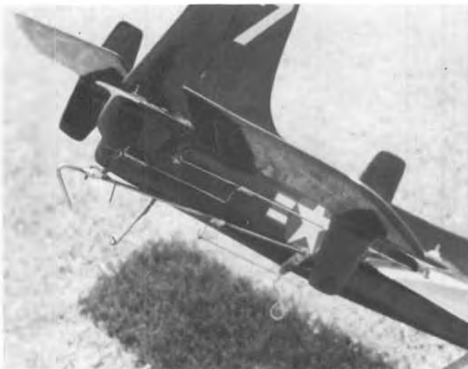
Arresting hook and release mechanism. Rudder deflection release gimmick also shown.
