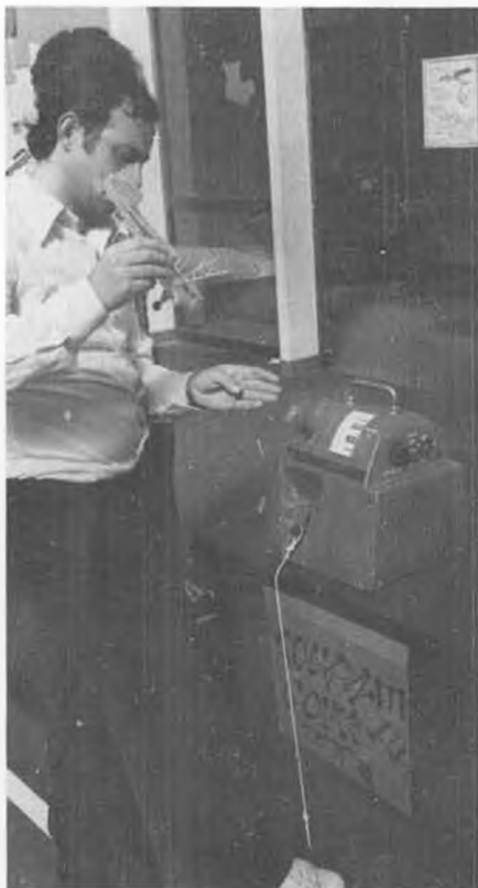
"Tourne Gomme", a French electric rubber winder, has counter and variable speed.
