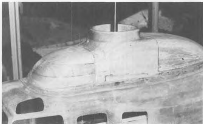
Top cabin fitted to fuselage. Main rotor shaft has been installed. Glassed over for strength.
