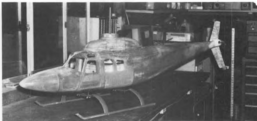
Basic fuselage prior to priming and painting, vertical fin installed. Shrike fuselage is available separately, along with wing saddle cover and molded windshield. See text for complete info.
