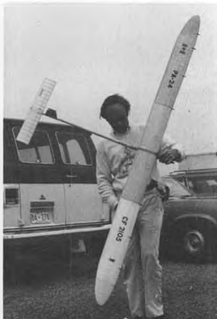
Canada's Pete Allnut rigs turbulator on his all-balsa winged A/2. Note ply outrigger ribs to hold elastic shirring turbulator line.
