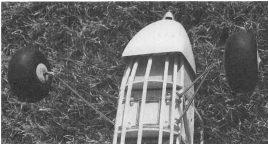
The pre-formed I.M. (Japanese) landing gear is clamped in place before adding the bulkheads and stringers. Makes covering a little tricky, but any other method would be design deviation.
