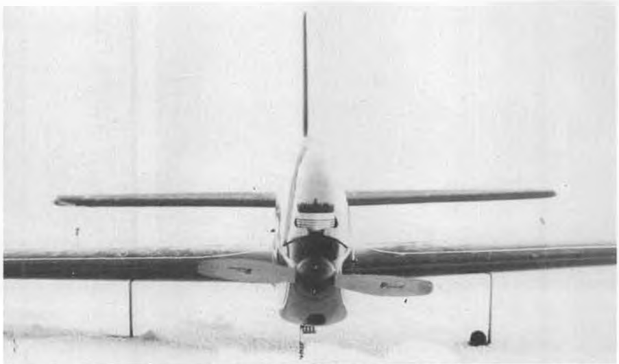
Hurry with the pictures, Bengt, it's sinking into the snow! Clean frontal area provided by the enclosed exhaust system is obvious from this angle. OPS 60 RCA engine. More info in text.
