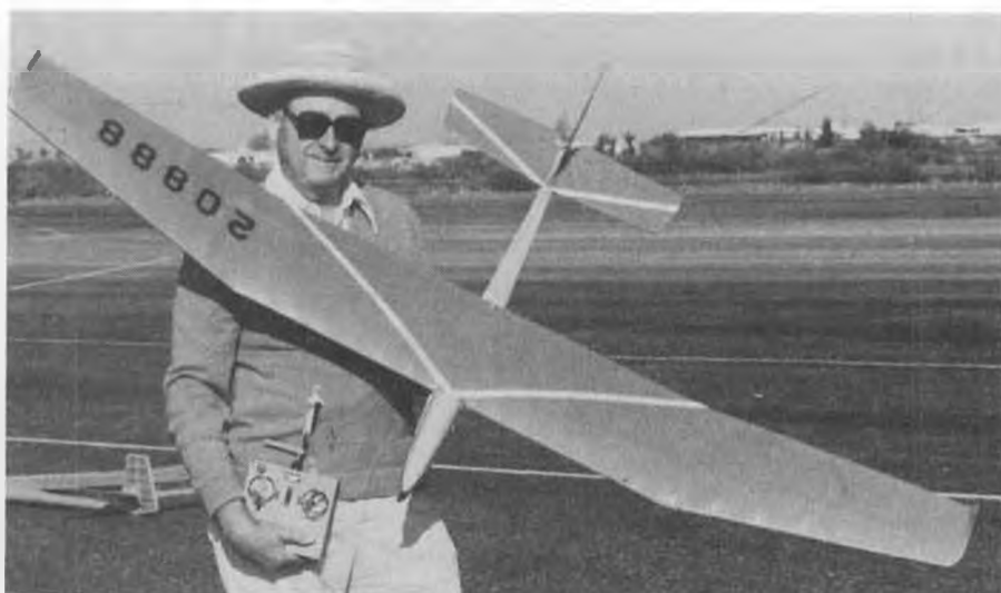
Another "Buteao", this one by TPG member, Al Doig. Ship meets the 1978 AMA 2-meter specifications, has the same airfoil as the Olympic II, plug-in wing tips, and 700 sq. in. wing area.
