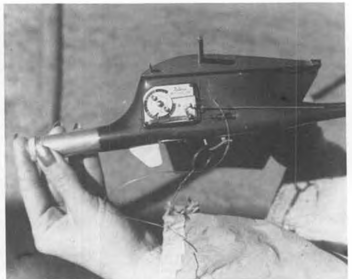
Front end machinery. Russian circle-tow hook. Extra line trips timer when hook releases. Vane protects hook. Cigar tube nose.
