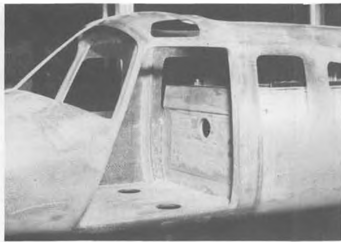
Cabin door cutout, engine box installation, door framing. Access holes for glow plug and for landing gear shocks.
