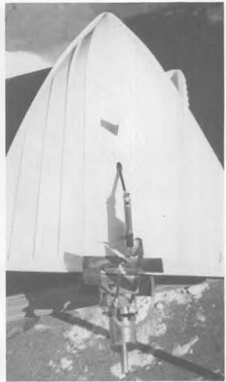
Bottom view of Northwind. Drive shaft off-set for torque. Flat-head bolts resined over for smooth running surface.
