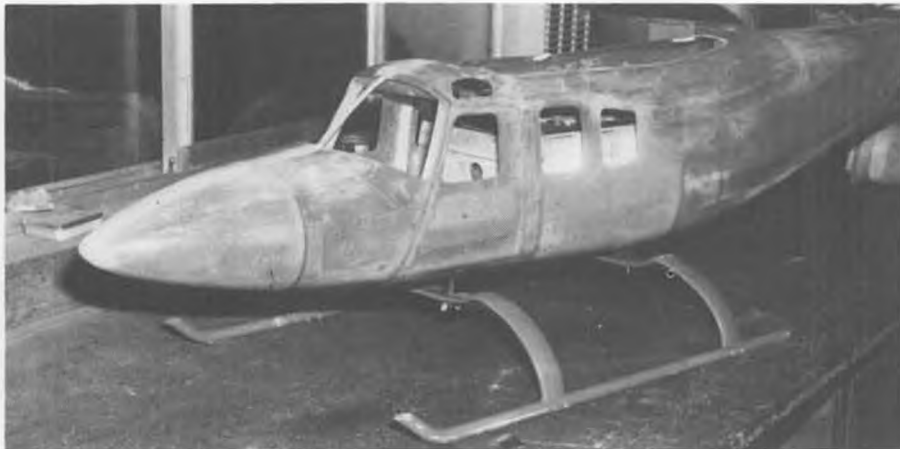
John molded his own landing gear struts to conform to the under surface of the Shrike fuselage. Location of all forward bulkheads can be seen in this photo.
