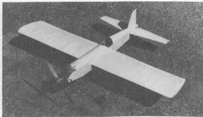
All exposed edges of cardboard are capped with balsa strips, such as the wing ribs, and the outside edges of the tail surfaces.
