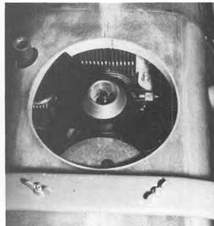
Note 1/32 ply shroud around fan hole. Ducted fan principal for cooling. Exhaust stack in other hole. Heat sink on engine.
