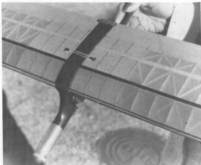
Rubber band around dress snaps assure that wing will stay in place. Aluminum clip keeps trailing edges aligned, relieves towing stresses.
