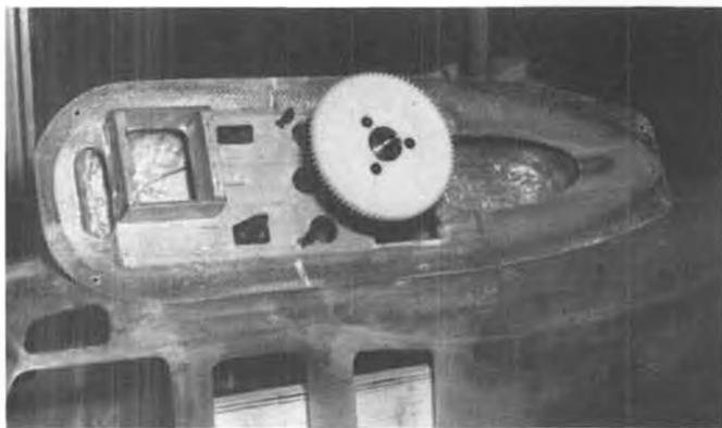
Underside view of cabin top shows main drive gear on shaft, fittings, and servo mount for mechanics.
