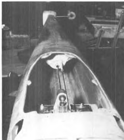
View toward aft end, shows tail rotor drive shaft and pushrod control supports.
