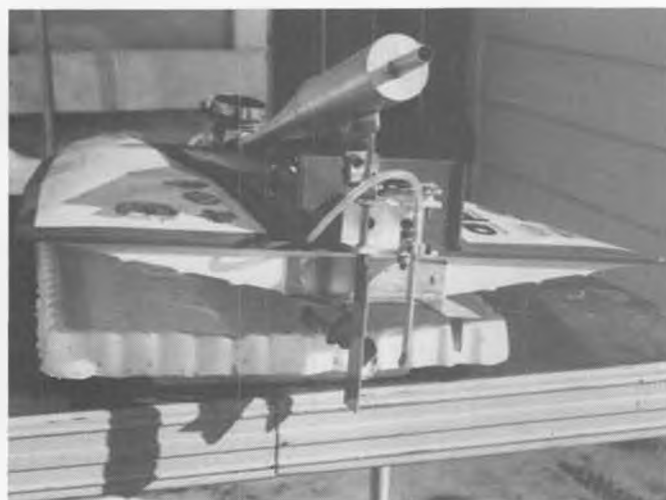
Transom shot showing the rudder and rudder plate installation. Also, note author's bracket for the tuned pipe.
