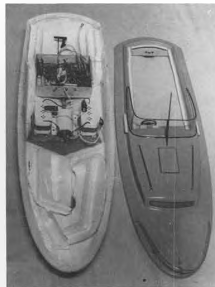
Completed boat with scrap foam flotation glued in fore and aft sections of hull. Deck attached with silicone for possible removal.
