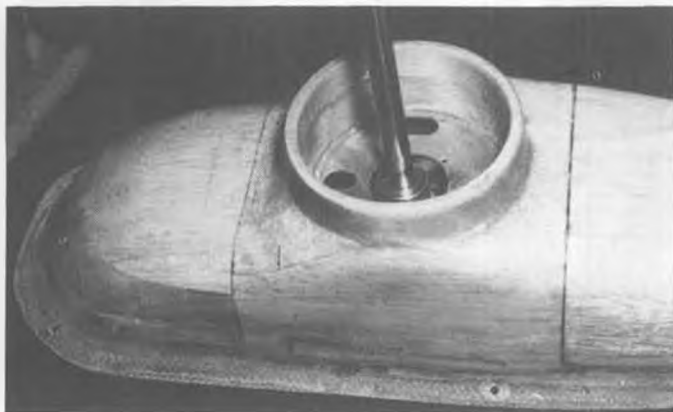
Cabin top details. Main rotor shaft and aluminum bracket installed. Balsa blocks have been hollowed out.
