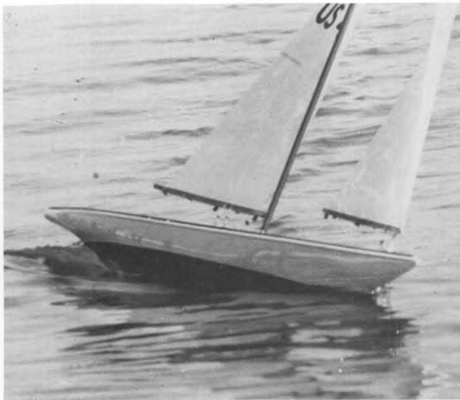
EC/12-Meter showing the excessive heeling and huge quarter-wave which develops when sails are overtrimmed. Photo by Doug Barry.
