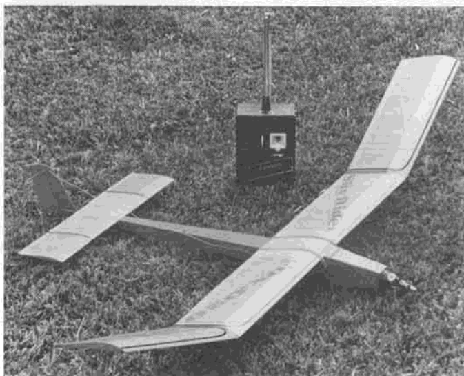
This rudder-only glider is over-powered with a Tee Dee .020!
