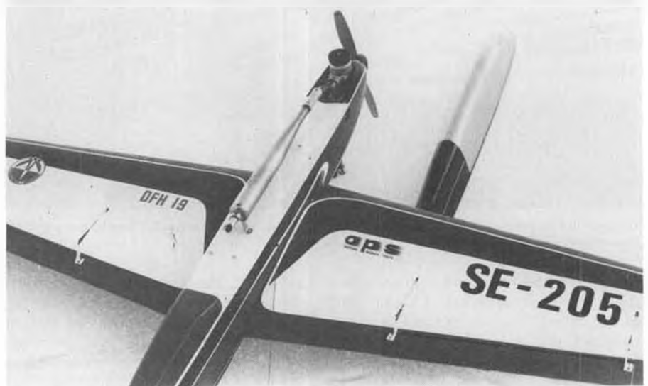
There's room to spare under the large and unusually shaped canopy of Bengt Lundstrom's new pattern ship. And now you see why it has that shape! Nice solution to a new problem.
