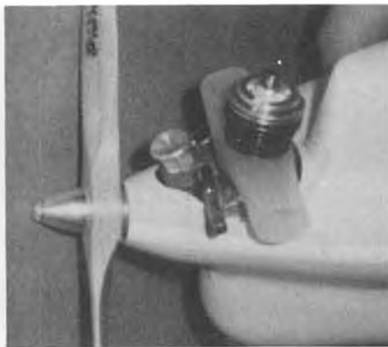
Davis Diesel "Stax" exhaust stack is silicone rubber, stretched and slipped into place.
