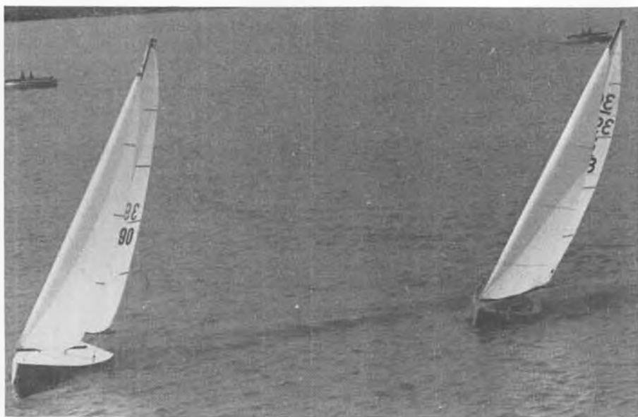
The weather boat's sails are absolutely perfect! Jib leech is parallel to main leech, and both sails are working top to bottom. Too much twist in rig of leeward boat. Tom Patterson photo.
