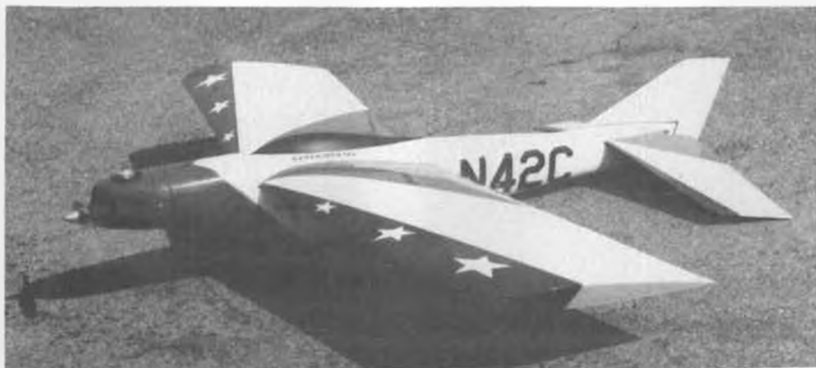
A Tigercat 1/2A racer by its designer, Ron Clem. This one uses an experimental upright engine configuration, but proved to be slower than the Tigercats with inverted engines.
