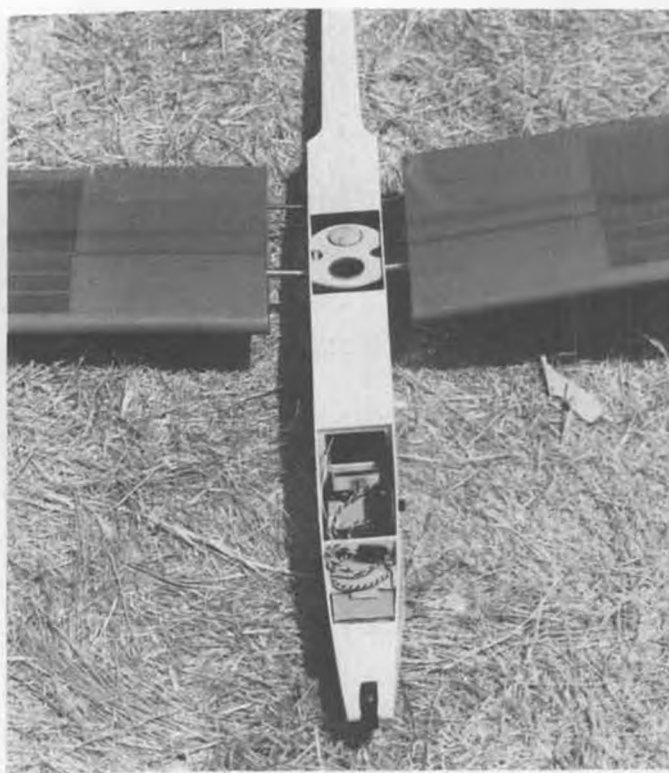
The Ace Express with hatches removed to show radio and ballast boxes. Model weighs 43 oz. empty, can carry up to 1 lb. of ballast.
