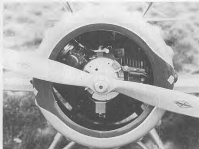
Most successful engine in the Gulfhawk so far is a 1.6 cu. in. Home-lite with a 1.9 crankcase and 2.5 carb. Turns 20x6 prop.
