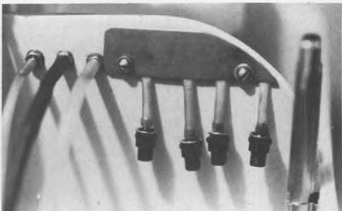
Spare glow plugs dangle from short pieces of surgical tubing. They won't fall off, yet are easily removed when needed.
