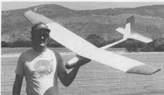
Two views of Ken Raymond's original design two-meter ship, the "Flamingo". Pylon mounted wing makes good sense, as it allows maximum use of wing area and reduces the interference effect of the fuselage. Model has 710 square inches, weighs 40 ounces.
