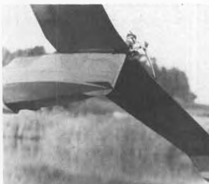
Underside view showing wing keys, water rudder, and spray deflector.
