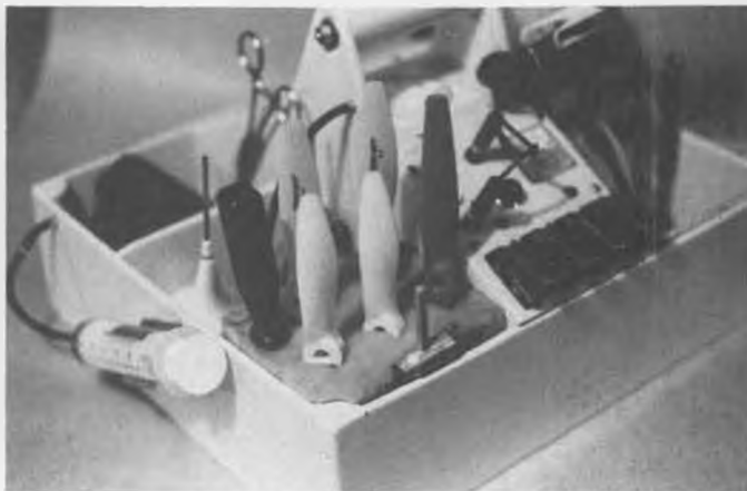
Spare props fit into slits in foam rubber . . . easy to get to if you're in a hurry. Fuel syringe is held in place by a fuse clip.
