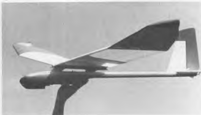
Two views of Ken Raymond's original design two-meter ship, the "Flamingo". Pylon mounted wing makes good sense, as it allows maximum use of wing area and reduces the interference effect of the fuselage. Model has 710 square inches, weighs 40 ounces.
