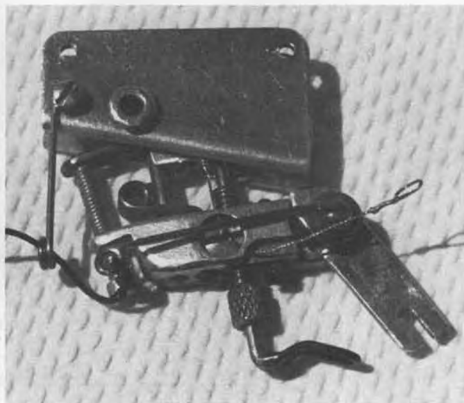
Bob Hatschek's towhook with a simple modification for automatic timer start (see text). On left is the hook in the latched position. Timer start line is attached to loop in wire on hook latch. On right is the hook in the unlatched position. Timer start line is free to move as latch moves back.
