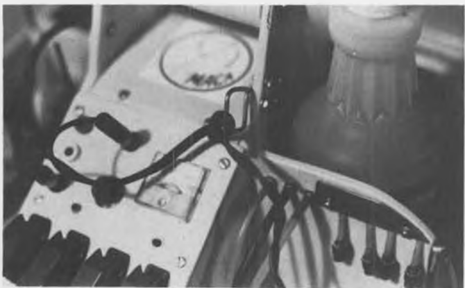
Closeup shot showing the glow plug leads tied to the wire restraint. Important if you want to stay plugged in.
