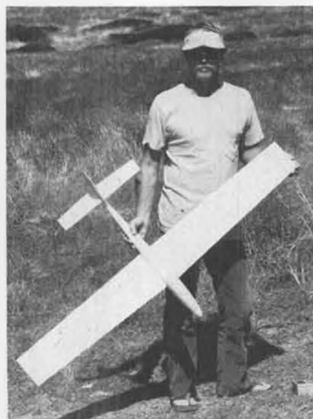
Alan Nelson's Foo Fighter has clipped wings for tighter turns. Normal span is 7-1/2 feet.
