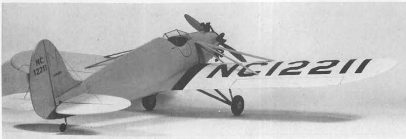
One of the neatest kits from Flyline is the Kinner Sportster. The model shown here was built by Hurst Bowers. Span is 39 inches, power is a Cox Golden Bee, control is by a 3-channel Cannon "Super Mini" radio. Scale is 1 inch to the foot. Design also flies well as a free flight.
