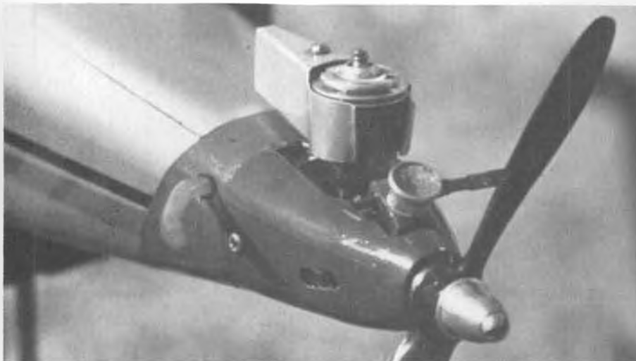
Closeup of the nose of a "Quicksilver" 1/2A pylon racer, by an unidentified builder, showing the combination cooling duct and heat sink.
