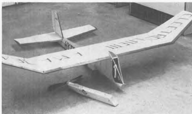
The Electrolite III with power pod detached, about 6 ounces of airplane in a seven foot span! Looks like typical pre-war F/F.
