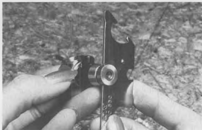
By unscrewing the carburetor housing nut, the prop drive plate is forced off the splines of the crankshaft.
