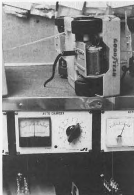
The Astro Flight resistor charger, charging a car at a local indoor race track.
