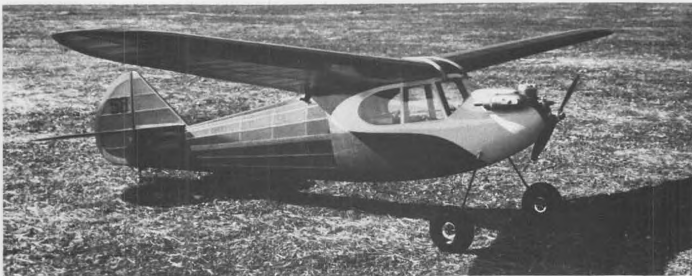
Bob Oslan, of the SAM 49'ers, did a beautiful job on this Scientific Commodore. Even though it's R/C (Futaba), the orange silk covering keeps grumbling among O.T. purists down to a minimum. Model spans six feet, takes off easily at half power with Enya .29.
