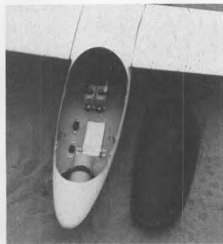
No shortage of radio room in the Foo Fighter! Fuselage has 10 to 20 layers of cloth.
