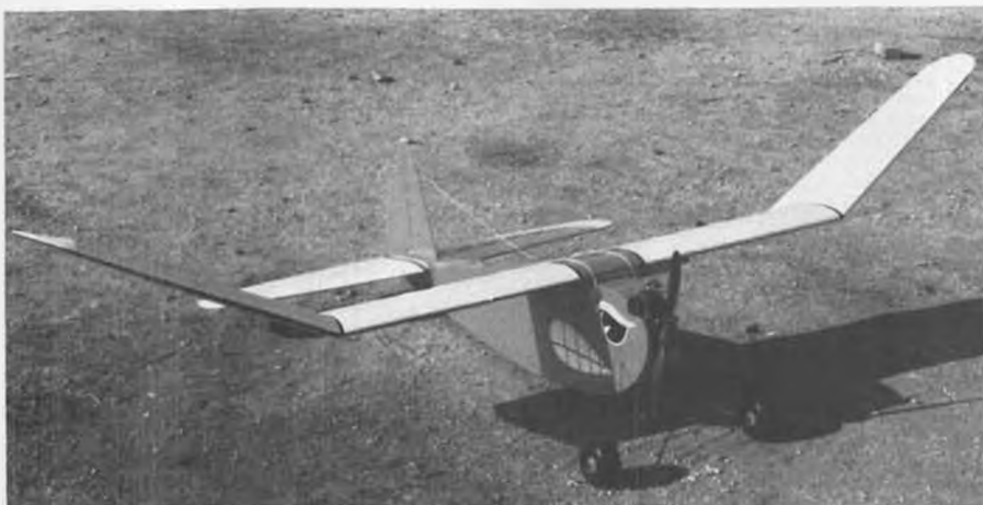
MB's very own Phil Bernhardt cleaned up at the last SAM 49's R/C Texaco with this Ehling Contest Gas Model. Powered by Super Cyke, controlled by Futaba. Model has full-flying tail.
