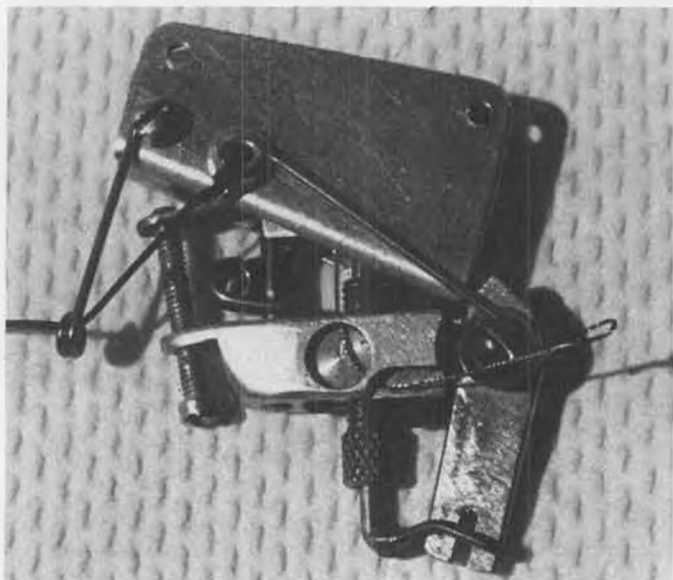
Bob Hatschek's towhook with a simple modification for automatic timer start (see text). On left is the hook in the latched position. Timer start line is attached to loop in wire on hook latch. On right is the hook in the unlatched position. Timer start line is free to move as latch moves back.
