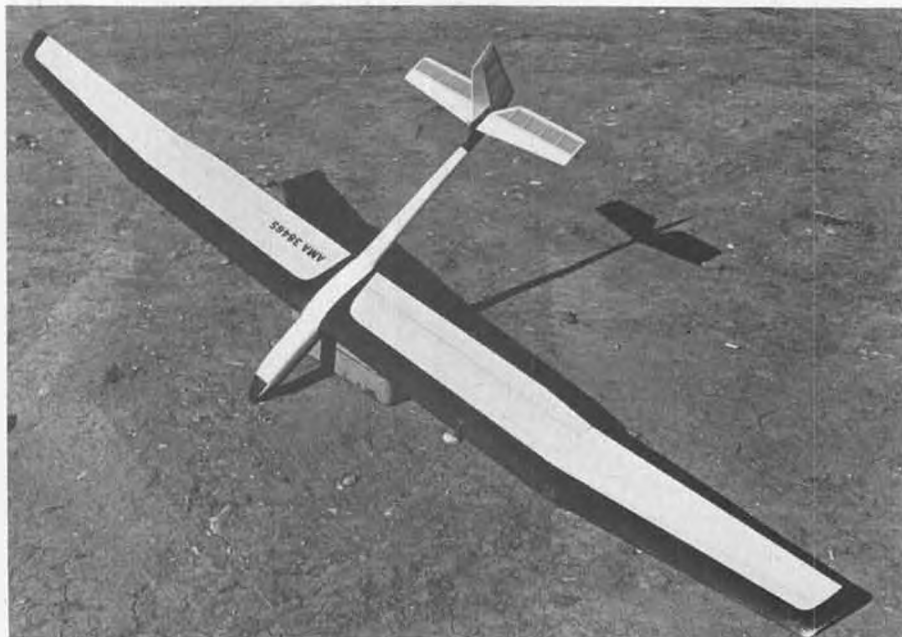
Herb Smith's latest (and best) FAI ship is the Invader Mk. IV, which placed 8th at the FAI Finals at Pensacola. Has a 114-inch span, 836 sq. in., 8.5 oz. wing loading.
