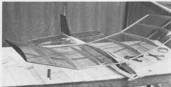
Mitch Poling's model had a fairly low aspect ratio wing . . . to say the least. Wing was too flexible, almost folded in flight.
