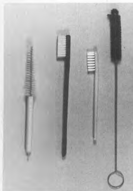
Cleaning tools required to do basic 1/2A engine rework (l to r): bridge and clasp brush, two toothbrushes, and test tube brush.
