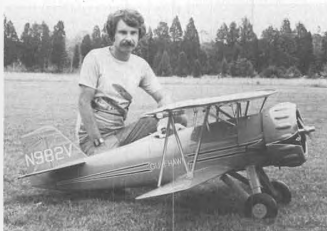
John Preston, of Falls Church, Virginia, sent in these photos of fellow NVRC club member Kirby Crawford's beautiful 2/9 scale Curtiss Gulfhawk. Conventional construction, weighs 26 lbs., and has a very effective smoke system. Plans were scaled up from Westburg 3-views in MB.
