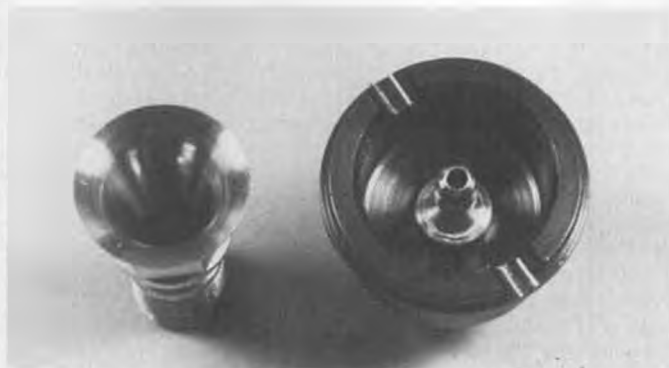
A custom enlarged venturi and pressure backplate. Pressure backplate is preferred over the pressure tap on the carb housing.
