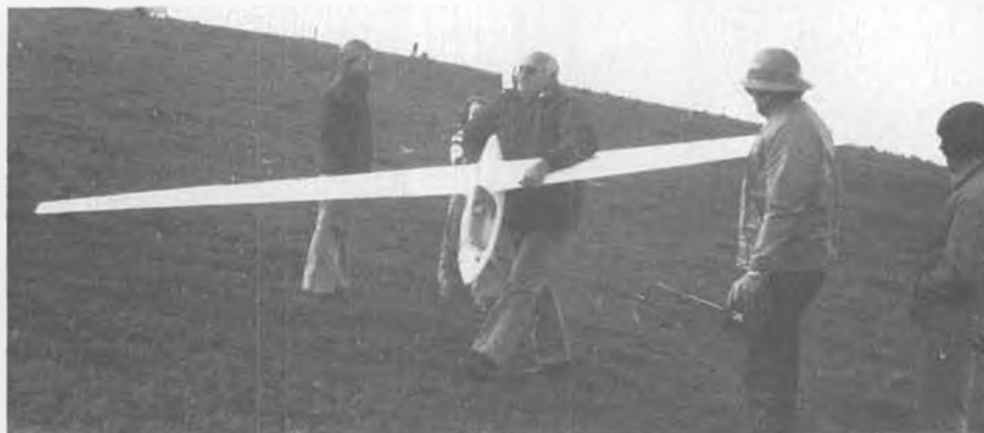
Brian Laging, of Australia, carrying his 1/3-scale Foka 5 (it's not a 1/4-scale Fokker 5, as mentioned in the text). Ship has a span of 14 ft., 10 in., and weighs 14-1/4 lbs.
