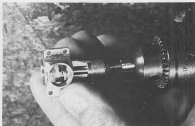
Lapping the case to the crankshaft using a variable speed electric hand drill. Procedure fully described in text.
