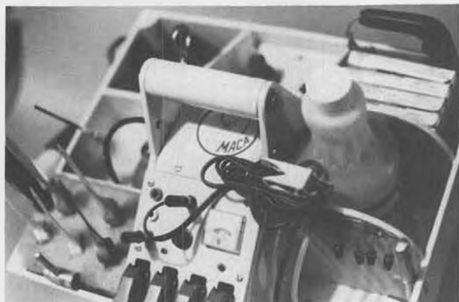
Another shot of the ready-to-go box. Power panel runs off 2-volt wet cell in compartment directly under carrying handle.
