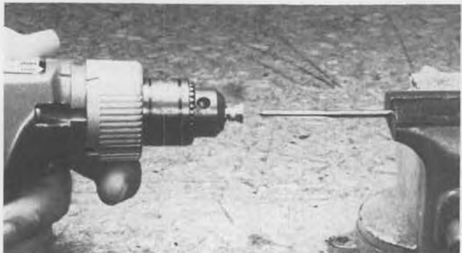
Reaming a venturi by holding it in a variable speed drill. This is an easy operation to botch up, so be careful.
