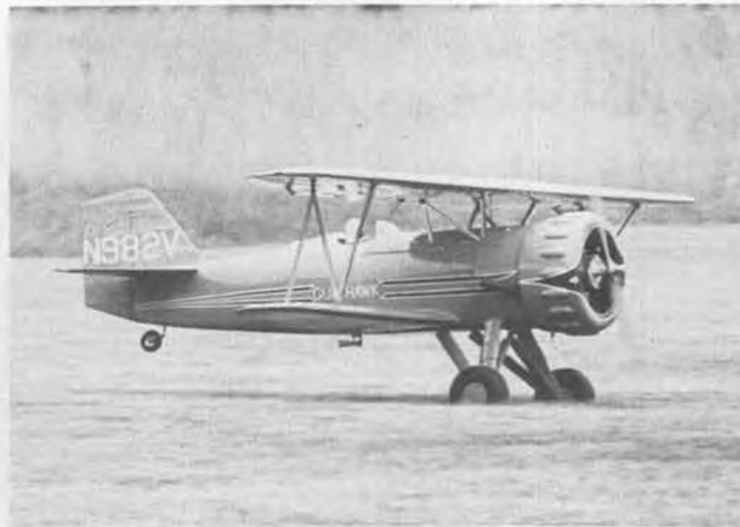
John Preston, of Falls Church, Virginia, sent in these photos of fellow NVRC club member Kirby Crawford's beautiful 2/9 scale Curtiss Gulfhawk. Conventional construction, weighs 26 lbs., and has a very effective smoke system. Plans were scaled up from Westburg 3-views in MB.
