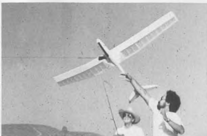
Bob Flores launching the Pixie for Sandy Edwards. Note that the outboard wing panels are longer than the inboards.
