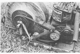
Jim Martin developed this winch using a plywood reel and a gasoline engine from a washing machine. Looks like an antique!
