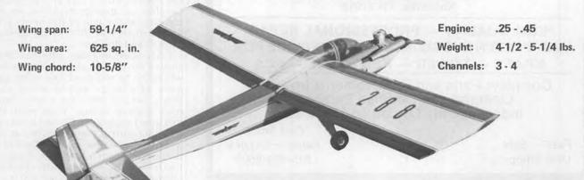
Designed by Joe Bridi for the AMA, this mid-size stable flying R/C model aircraft boasts sturdy, step-by-step construction. This kit includes photo-illustrated building notes written for the first-time builder, a clear canopy, dural main landing gear, piano wire nose gear, Bridi Hobby engine mount, and special hardware. For the beginner to R/C, it's a great first plane. For the experienced R/C pilot, it's a quick building, economic, superb fun flier.
