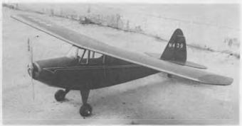
Before and after covering photos of Bob Boucher's latest scale ship, a Porterfield Collegiate. Span is 72 inches, power is an Astro 15 with prop speed reducer. Uses lightweight structure throughout to keep the weight down to a reasonable 4 to 4-1/2 lbs. Watch for the kit.
