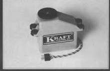
motor allows this servo to deliver in excess of 56 oz.-in. of thrust and a transit time of 4/10 of a second for  $100^{\circ}$  rotation.
