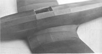
Two examples of card stock fillets. These are most commonly used on rubber scale models because of their light weight. They're also one of the easiest types of fillets to make.
