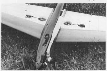
Underside shot shows Southern R/C retracts, pipe mount, and aileron pushrods. Monokote on wing and stab saves mucho weight.
