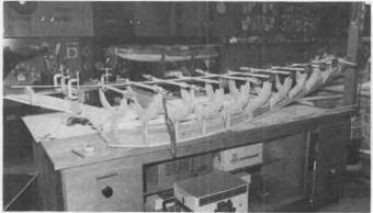
The keel and all bulkheads were cut from 1/2-inch mahogany plywood, later planked with balsa strips, then fiberglassed.
