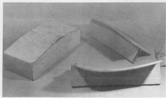
Special sanding blocks for sanding framed-up wings can be made from a solid block (left) or built-up like a wing platform on a pylon.
