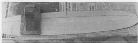
Initial shaping of the wing airfoil is done with an abrader, available at hardware stores. These things take off the balsa in a hurry, so don't get carried away!
