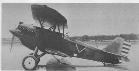
P-1B was delivered to McCook in Dec. 1926. Tunnel radiator is experimental, windshield is new. Tubes on lower wing contain fireworks for a Fourth of July celebration.
