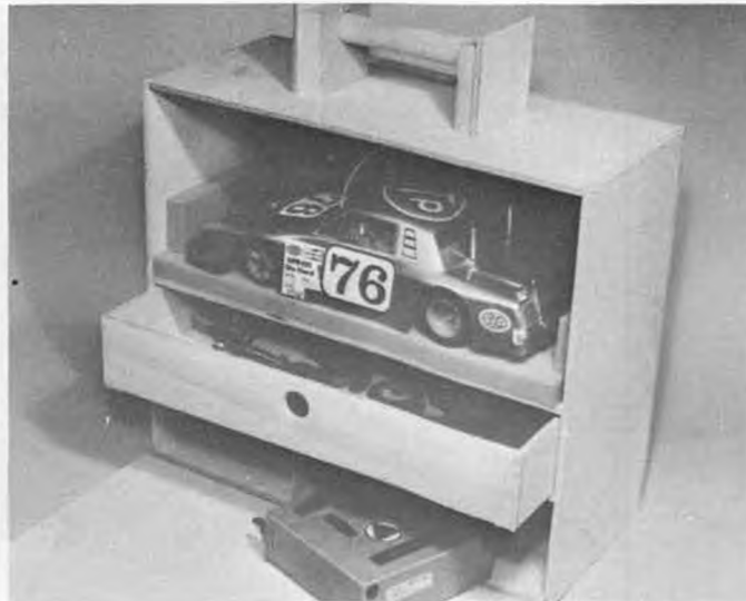
A little thought and some pieces of 1/4-inch ply can result in a handy pit box for indoor racing.
