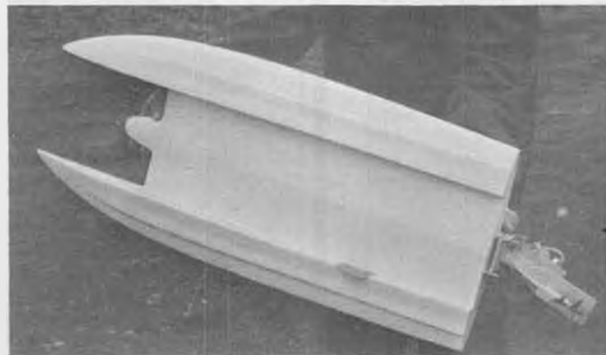
Bottom view of J.V.S. 7.5 Tunnel, showing sponson side strakes, tunnel bottom vee, and turn fin.
