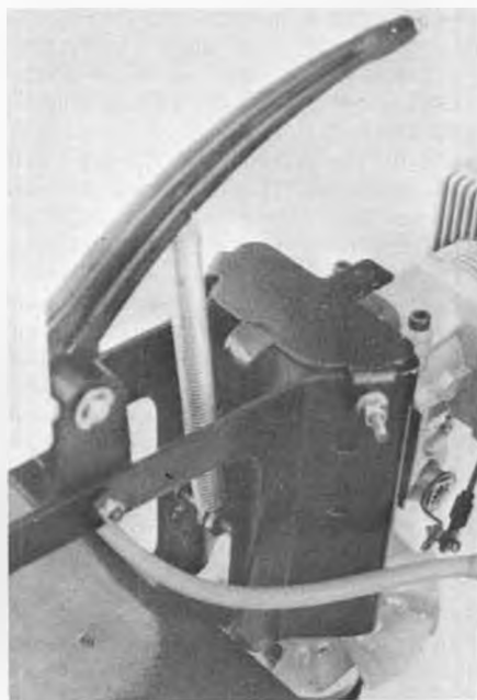
Spring to counterbalance weight of servos. Holes in main frame for access to allen heads.
