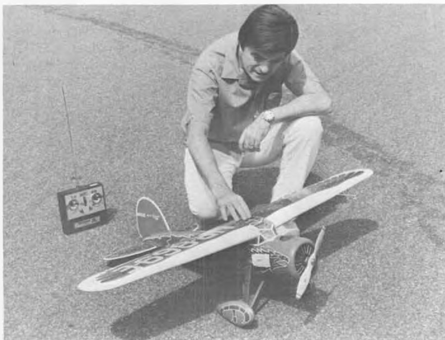
Walt opens sliding hatch on his Vega to turn on receiver switch in cockpit. Dummy radial engine is strength member of cowlings, dressed up for appearance.
