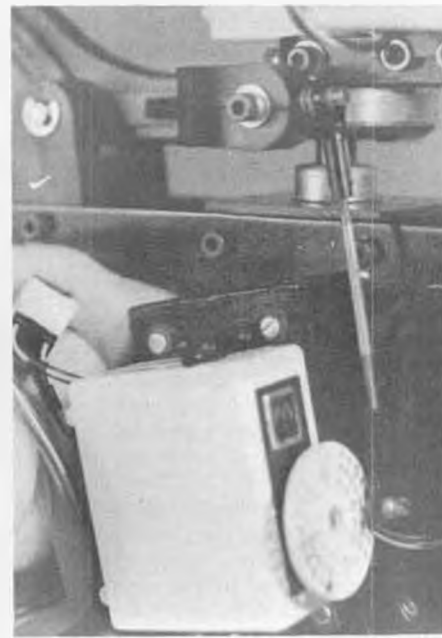
Ray added 5th servo for independent collective. Mounted on left side of main frames.
