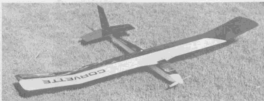
The Corvette by Parker, span 70 inches, wing area 630 sq. in., 36 ounce flying weight with Astro 05XL or Leisure 05.
