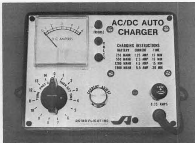
Latest Astro 4005 AC/DC charger. Charge any pack up to and including 8 cells. Charge info on panel. More in text.
