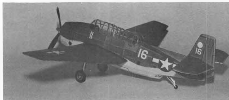
Peanut TBF Avenger modeled from Monogram 1/48 plastic, which is Peanut size, by Scott Rubke. Plug-in gear, decals, and scale prop come from kit. Flies over 30 seconds. Rubke photo.
