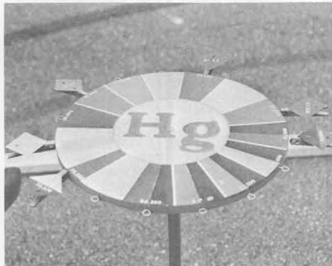
Monterey club's neat frequency pin board. Heavy base prevents tipping, top spins for easy access to pins.
