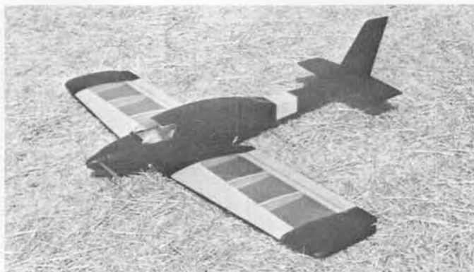
Lil Joule, hot 1/2A Pattern with 05XL or Leisure 05. Span 37 inches, area 273 sq. in., 28 ounces. Aileron and elevator.
