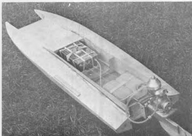
Octura Wildcat with G&M Radio Box installed, twin 8-ounce tanks, K&B 7.5 Outboard, and K&B throttle linkage kit.
