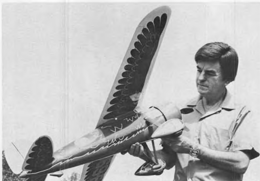
Walt justifiably admires his handiwork. Pattern on bottom side of wing and stab same as on top. Scale wheel pant blister strengthens joint to strut fairing.
