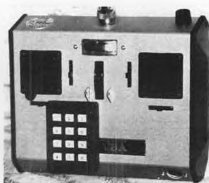
Keykoder system by Vantec provides 12 new on-off commands of one channel.
