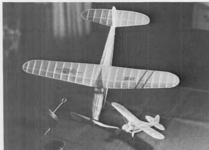
AIR XX "Sparky" weighs 3.5 grams. Grapenut Piper Vagabond flies on one loop of .017 rubber. Author's models and photo.
