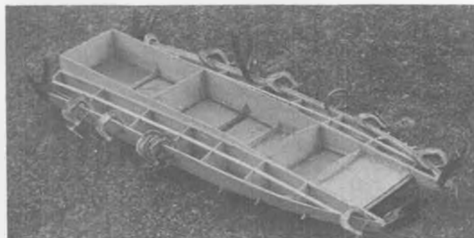
Part way through construction of the Octura Wildcat Tunnel. Sponson side clamped and pinned in place.
