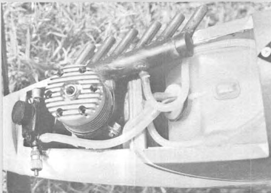
The home made exhaust system, with six stacks, to give the appearance of an inline engine. Also includes a tap for fuel tank pressure.
