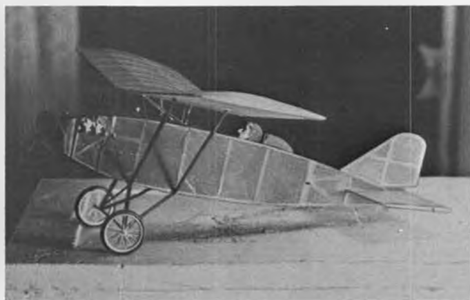
Indoor Waterman "Gosling" spans 16 inches. Uses Hungerford spoke wheels and sheet wood prop. Colored condenser paper.
