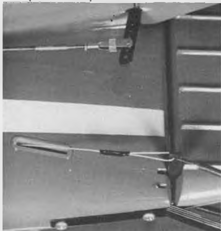
Control surface hardware is identical to normal configuration. Elevators are independent.
