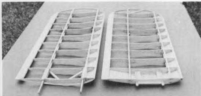
This view of the upper and lower right wings shows spar extensions required in the top wing and locator tongues required in bottom.
