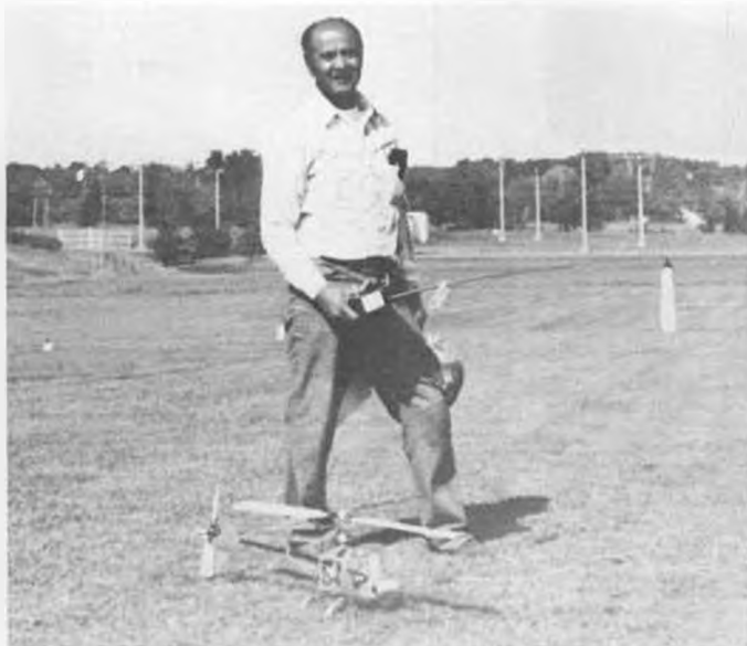
Charles Hampton poses with his Ishimasa helicopter which is twin 05 powered, and carries eight sub-C cells. KRC meet, Hatfield, PA.
