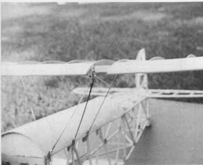
Step 4, rigging procedure: upper wing spar extensions slide into the space between the center section's spars.
