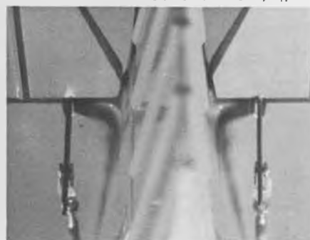
One method of actuating independent elevators. See text for alternate method.
