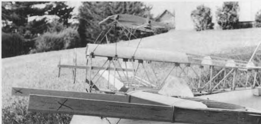
Step 3, rigging procedure: one pound bags of shot are used to stretch out the landing wires and straightedges are used to adjust wing incidence from root to tip.
