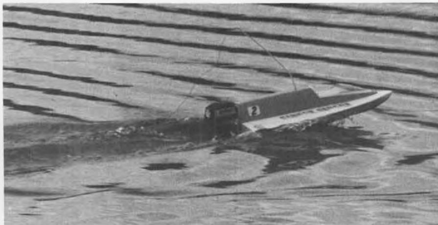
The Santa Monica monoplane hull electric powered boat is very maneuverable. It exhibits good handling and slower speeds that are perfect for beginners.
