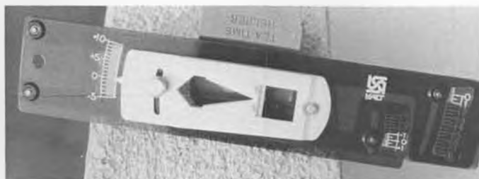
This very neat, high quality gadget is a Kalt pitch gauge which can measure from -9 to +18 degrees on clockwise rotating heads.
