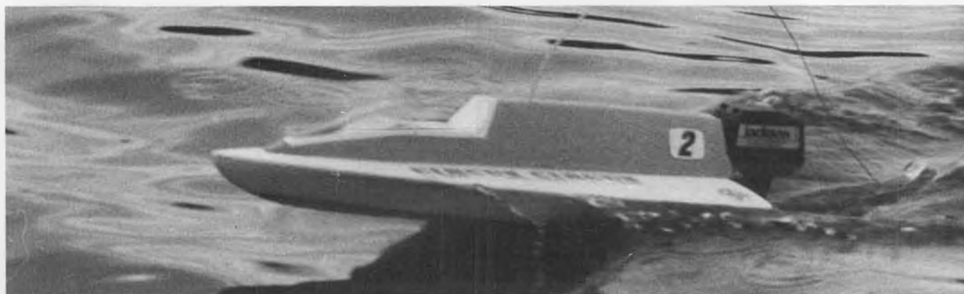
Another running shot of the Santa Monica from Octura Models. Top speed with the Jackson 38 is about ten miles per hour . . . not that fast by gas engine standards, but a lot cheaper to run!
