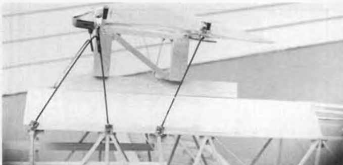
Step 1, rigging procedure: template positions center section of top wing while holes in end ribs receive spar extensions of wing panels.
