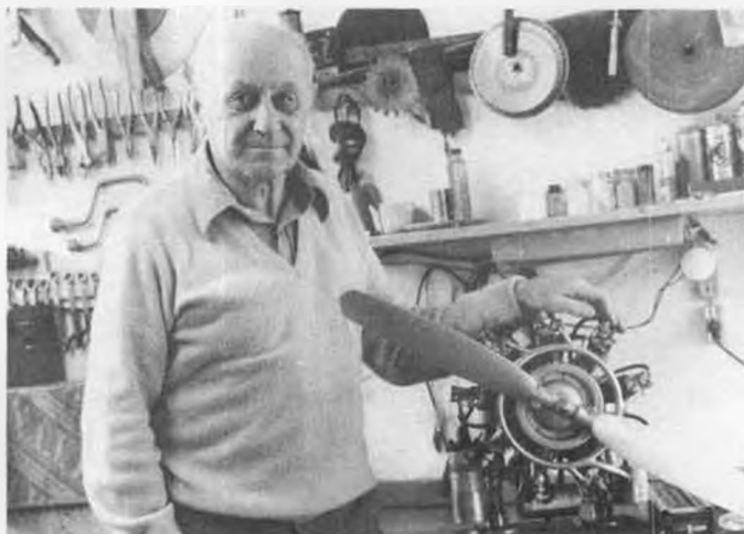
Another of Ed Glenn's projects was this working replica of a Wright Whirlwind radial engine. Over 10 hp produced.
