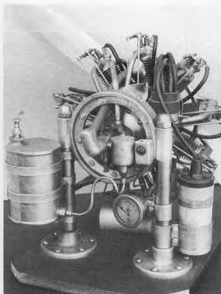
Rear view of the Wright radial reveals fuel system details. Note carb air horn at cylinder.
