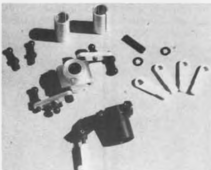
Complete Bell-Hiller mixer and articulated follower (black piece at bottom) convert the Baron 20 to a Bell-Hiller head.
