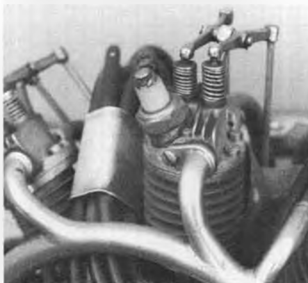
Bosch 11 mm spark plugs were used. Note collector ring and rocker arm details.
