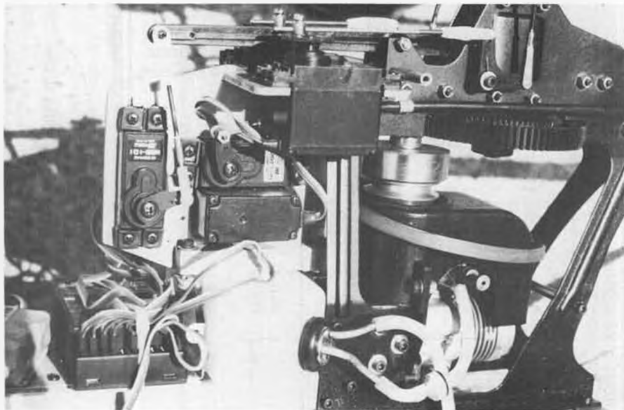
A closeup view of the Baron 20 reveals the five servos that control the chopper: collective servo is at far left, throttle servo is bottom center, tail rotor is middle, and top two are cyclic pitch.
