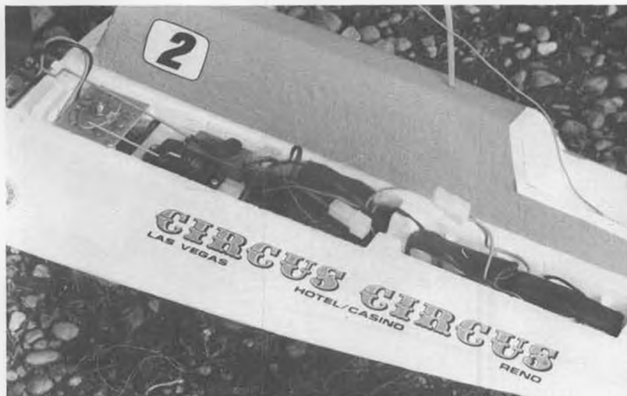
For proper balance, the six-cell battery pack should be positioned in the forward compartment. Receiver and its battery, servos, and speed control are amidships.
