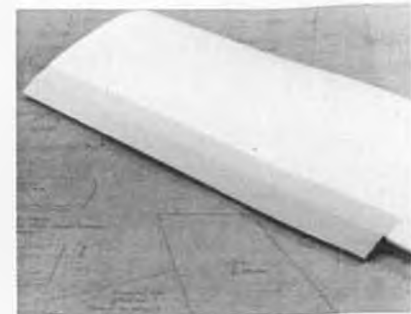
ABOVE: How to cover a foam wing Wonder . Start by covering bottom side of aileron. Flip aileron down, then cover top side. You may epoxy or tape torque rod to end.
