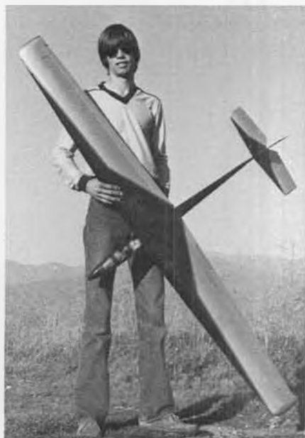
John Harrington designed and built this slope glider called Thrasher using a rather thin 9% airfoil with 2% camber. Features camber-changing flaperons. Flies super.
