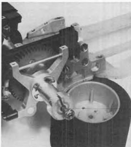
Recently released all-aluminum carriers end previous problem of bent plastic carriers. Nice machine work is evident.
