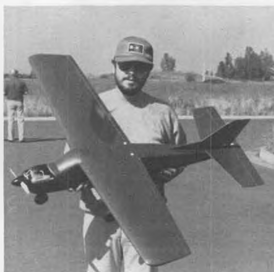
At the suggestion of Sig dealer Henry Barklay of Eugene (WA) Toy and Hobby, Mike Ferris modified his Kadet MKII fuselage to take a Kavalier wing. As you can see, it made an attractive combination which flew beautifully without requiring any trim changes.
