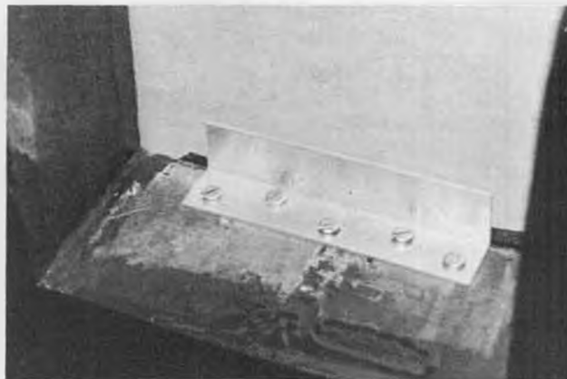
Close-up shot of the wing's leading edge at the center. The piece of aluminum angle screwed on to the spar joiner secures that part of the wing in place when the 1/4-inch bolts are installed in the rear. The fuselage is sandwiched between the forward part of the ribs (open section in picture) thus keying in the wing.
