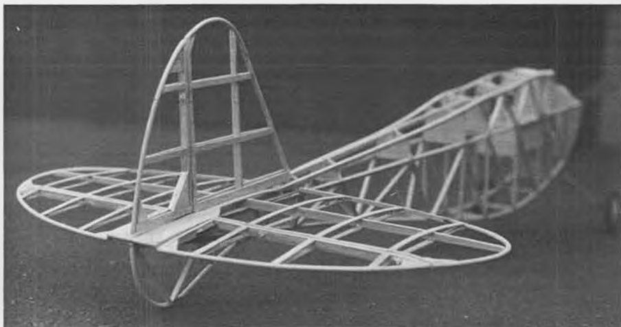
The graceful curves of the Feather Merchant's tail surfaces really make her an attractive model. Reed is an easy material to work with. Stab and fin/rudder are very lightweight and strong.
