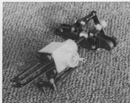
Tail rotor gear box. Bellcrank visible on bottom, metal tongues on left side for horizontal stabilizer mounting.
