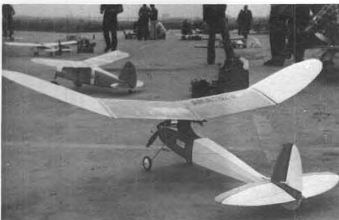
15. This snappy looking Swoose was built by Maurey Fine. Orange and white color scheme, and O&R .29 front rotary valve motor.
