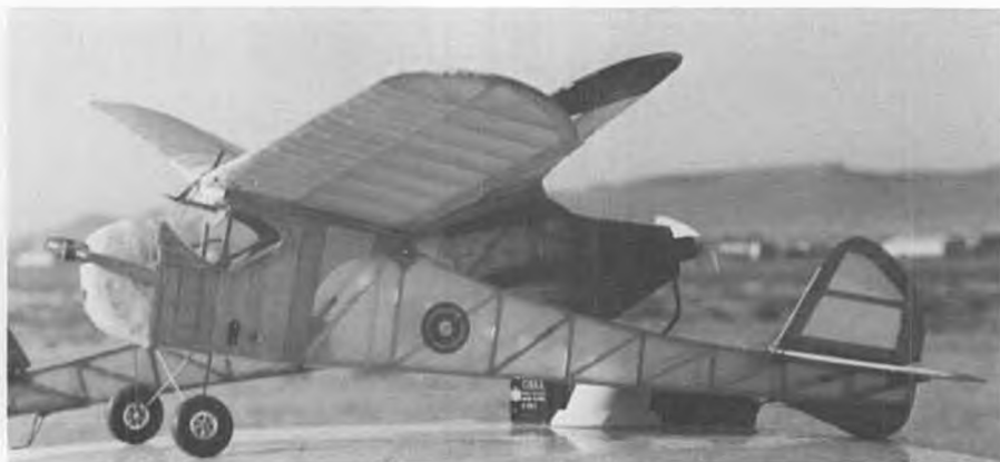
11. Gordon Coddling has been converting his modified Hepcats to electric power. He has installed a couple of Estes Skymax motors.
