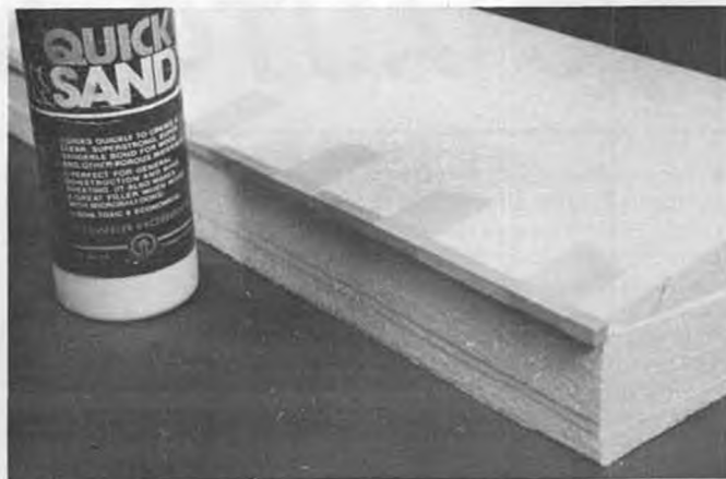
Glue trailing edge balsa piece to the trailing edge of the foam core with white glue. Tape keeps the piece from moving while glue sets.
