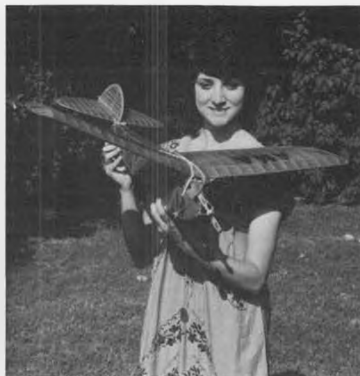
Chris Baker poses with her dad's F/F Powerhouse . Bill Baker made the model from MB plans. The 020 electric installation is super simple. Model flies well.
