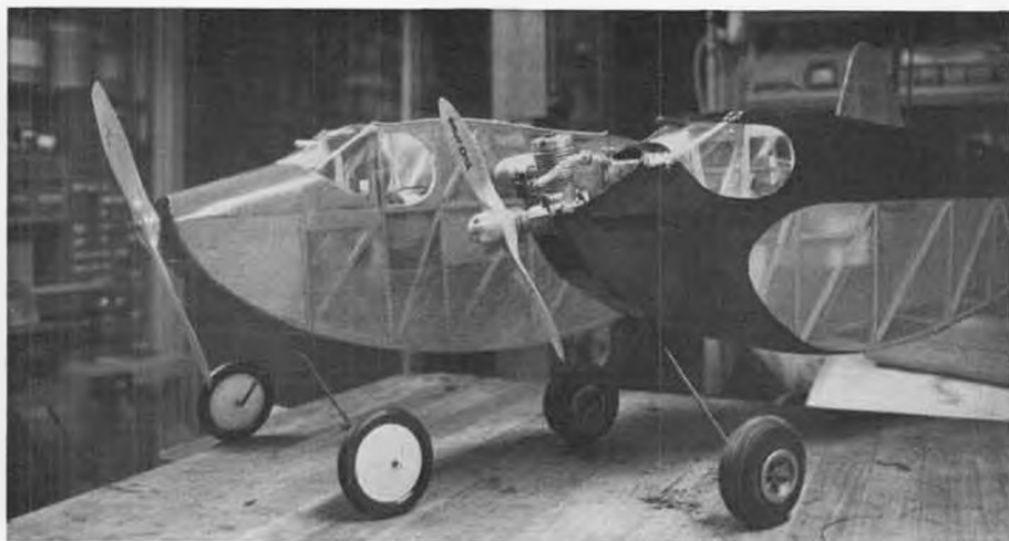
Electric snout and gas snout . . . just to show you how it looks either way. Glow engine is an H.B. .25 non-Schneurle. Ask Lehmberg Ent. about engine/kits combos.
