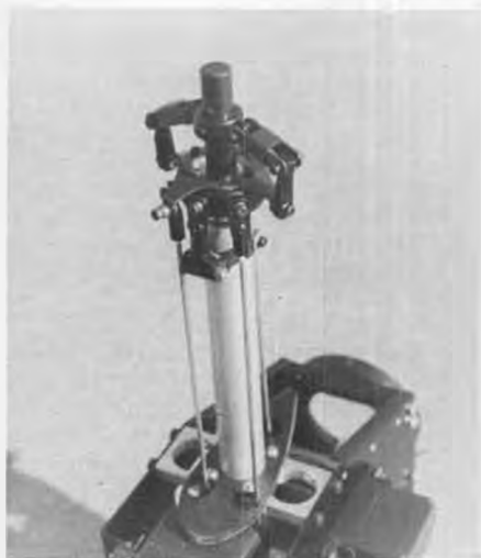
Main shaft pipe and swashplate detail . . . to be covered with aluminum fairing.
