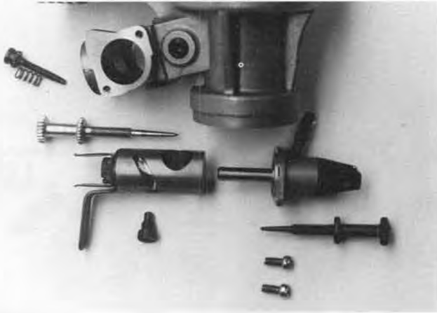
Carburetor's barrel features over 1/8-inch lateral leaning-mixture movement. Carb body is silicone sealed to the crankcase casting.
