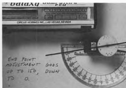
ATV (endpoint adjustment) program allows increase or decrease.
