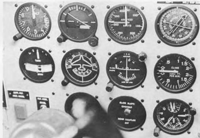
The instrument bezel is hand-fabricated from scrap plastic, the instrument face is cut from cardboard, and the clear instrument covers are from old plastic storm windows. Instrument needles are brass paper fasteners.
