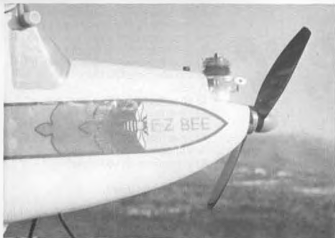
Plastic molded nose of the E-Z Bee with Cox .049 ready to go.
