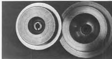
Smaller cylinder head button is for the Fox .40 Standard and you can see how the miracle plug fits down into the combustion bubble's dome. The larger button is to a Rossi .65 and has a K&B 11 plug in place.
