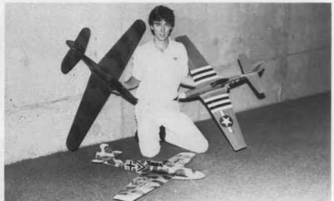
Slope Scale's Brian Laird shows three of the four Slope Scale gliders in his line. Partial kits feature polyester-glass fuselages and foam-core wings.
