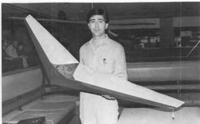
Future Flight's Rollin Klingberg and the Klingberg wing. The only true flying wing kit known. This was a stability test bed for a full-size, rigid wing, foot-launched glider.
