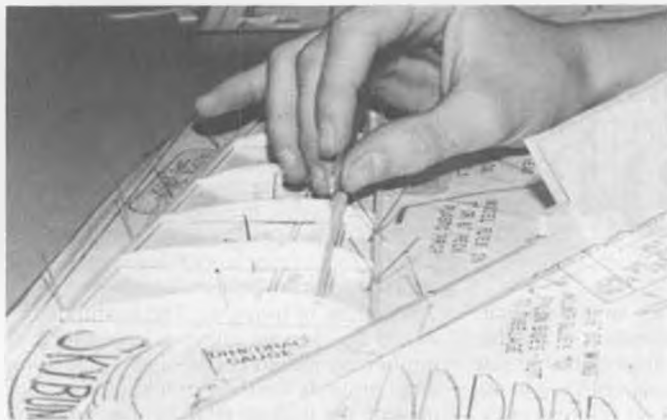
Fit wing spars after notching ribs in position with notching tool.
