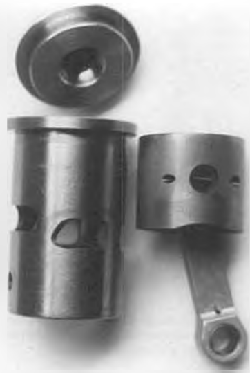
Front view of piston/cylinder shows inclined Schnuerle ports through cylinder wall and also the unique method of retaining the wrist pin inside the piston with a tiny steel roll pin.
