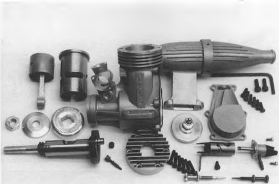
The Fox features the long-wearing economical match of a Meehanite cast iron piston running in a steel cylinder. High back door has one transfer port cast into it.
