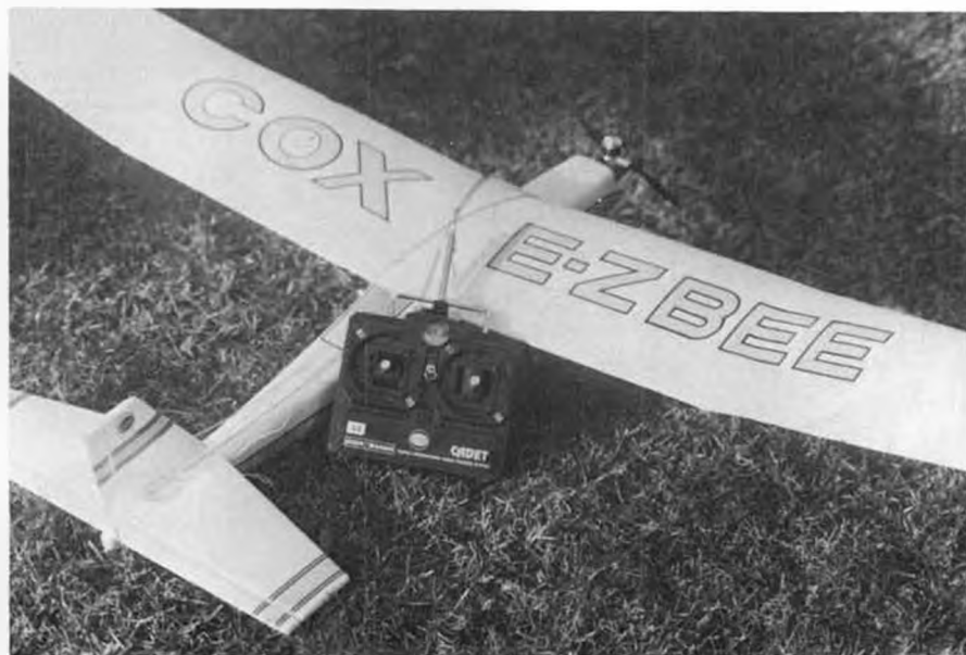
The E-Z Bee with Cox/Sanwa Cadet radio. Digital proportional system offers simultaneous control of two functions when second servo is installed.
