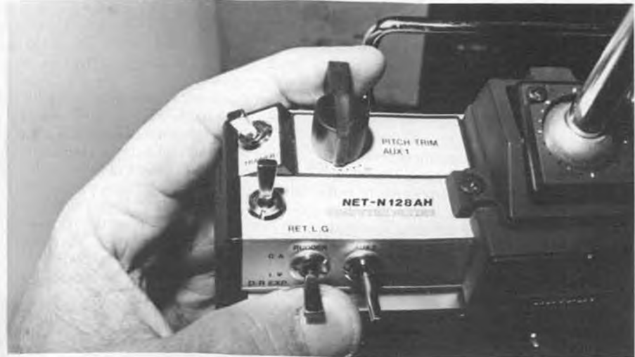
Collective pitch trim lever is easy to find.
