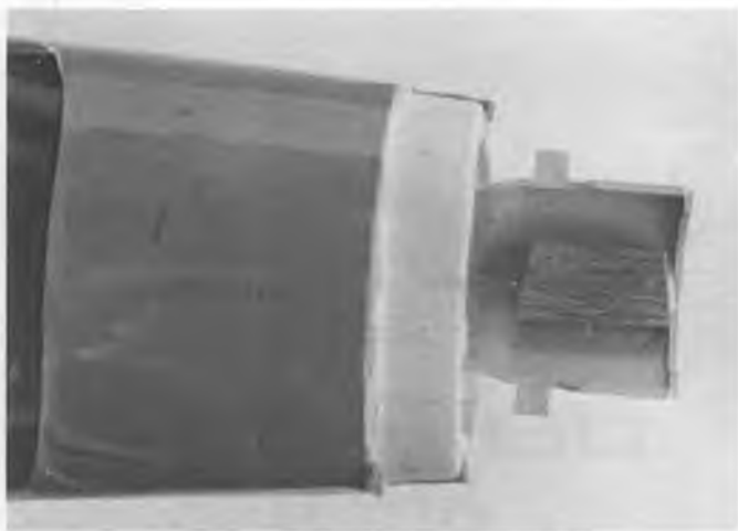
Balsa block used to shim AP 29 or 05 motors in MRC's Cessna 172.
