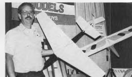
Larry Pettyjohn holds the latest prototype combat slope glider. Indestructible fuselage and disposable foam/cardboard wings means you don't fear mid-air or crashes anymore.
