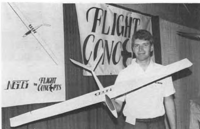
Simon Marsh of Flight Concepts holds the Nisus slope or thermal glider. Designed for speed and efficiency; comes 90% RTF.
