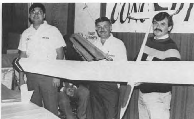
The only U.S. made, F3B-ready R/C sailplane is the Flight Concepts Eagle. Secret Selig airfoil, vacuum-molded fiberglass and balsa sandwich hollow wings are state of the art.
