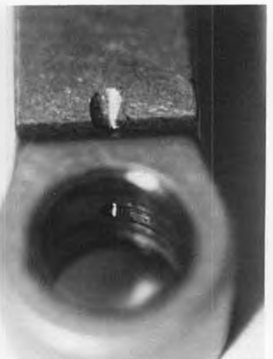
Close-up photo shows how lube hole is drilled in a better location at rod's top and bottom bearing. Purpose of careful oil-rich break-in is to seat these bearings as well as to finish forming the piston/cylinder fit.
