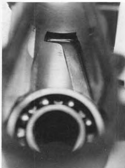
A look through the high back door shows the front transfer Schnuerle port and how fuel flow is directed away from the exhaust.
