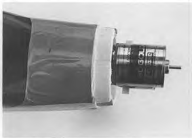
LeMans 480 motor (05) installed, ready for the rubber bands.
