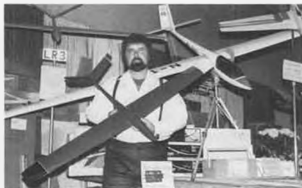
Gary Anderson of American Sailplane Designs holds the RAF, a wingeron-elevator control 1.5m slope design.
