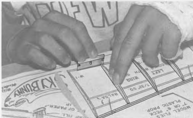
After laying down the L.E. with 'Xed' pins, trim each rib to fit the T.E. exactly. Then glue on the T.E.
