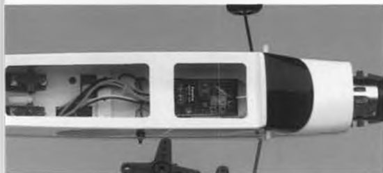
Hooked up with a pair of S133 micro servos, this system is perfect for electrics like our Hirobo/Futaba Professor.
