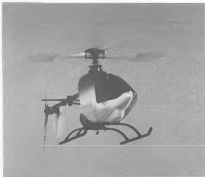
Here's looking at you, kid! Very wide stance on landing gear. Strong vertical fin with integral wire tail skid, one of the best.
