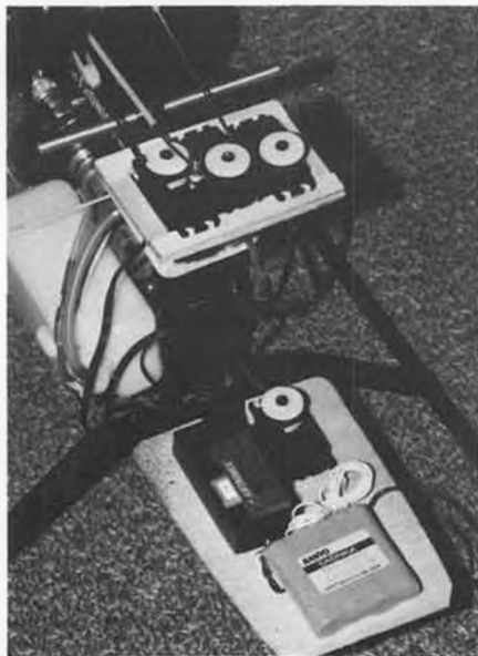
Simple radio installation. Standard Airtronics airplane radio used, using four servos; pitch, roll, tail rotor, and throttle. Optional gyro is highly recommended.
