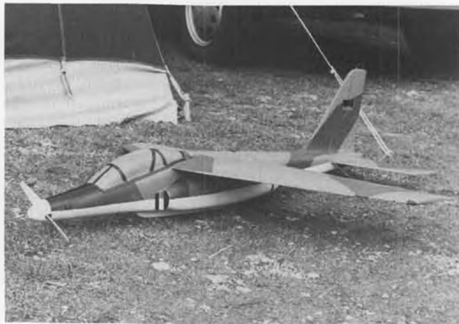
Sport scale Alpha jet from Topp-Modelle, spans 40 inches, five pounds, for 15 to 25 gas, so Astro 15 or 25 with 12 to 14 cells can do it.
