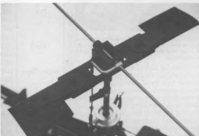
The one-piece molded hingeless rotor head. Has soft individual blade flapping and Hiller control. Works great.
