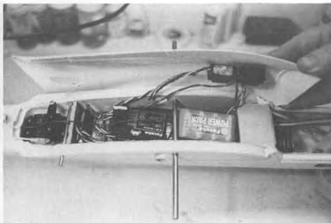
It's a tight fit all the way! Note cut-outs in hatch to clear servo arms. Moving battery forward makes ship nose-heavy.
