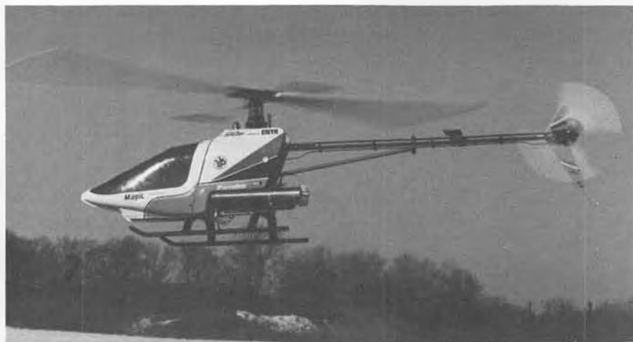
Author's Schluter Magic in very stable hover. Head speed is 1700 rpm. At 10 pounds, 6 ounces, it is still very nimble. Note canopy/fuselage cut away to clear muffer. Sixty hours to build and paint.
