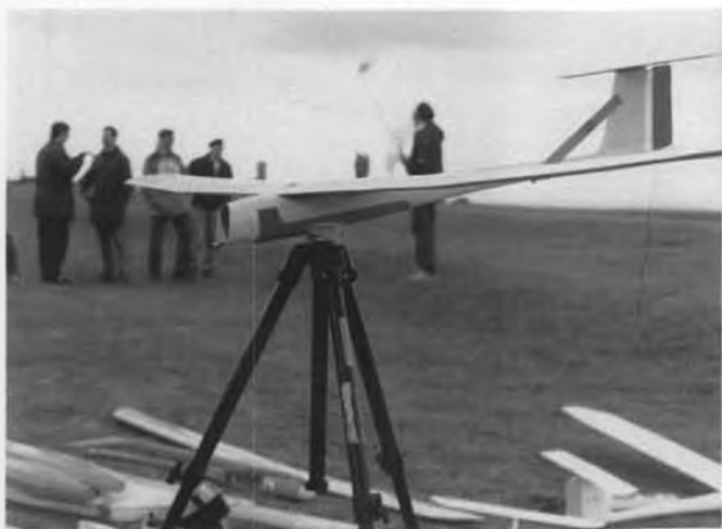
Camera tripod with molded-to-match fuselage cradle is the way to go. Open mouth front explained in photo at right.
