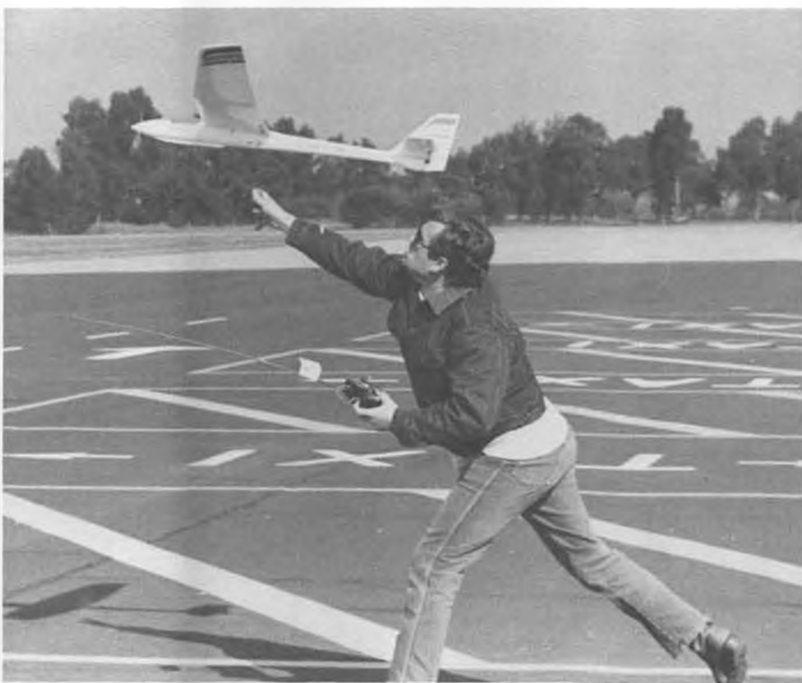
First launch. Climb is fast and flat, but very good . . . about 300-400 ft. per minute depending on battery and prop.
