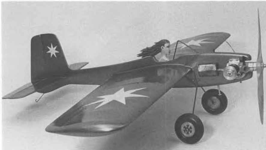
Joe Wagner's "Chicadee." Cox .15 Medallion powered, it's silk covered and equipped with big wheels for F.O.G. (flying off grass). "Buried" fuel tank is homemade unflow, pilot is "Narrow-minded Nell." Weighs 18 oz., wing area 220 sq. in. Model is 12 years old and flies great.
