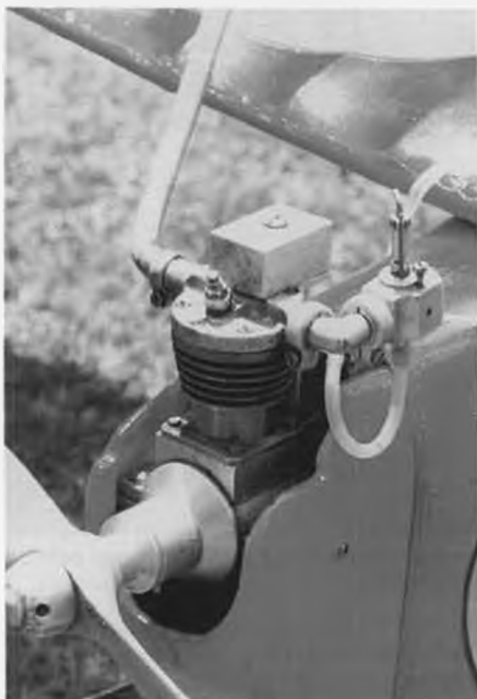
15. Bruce Abell machined up this good-running "Matador" .60 four-cycle engine for his Lackey Zenith.
