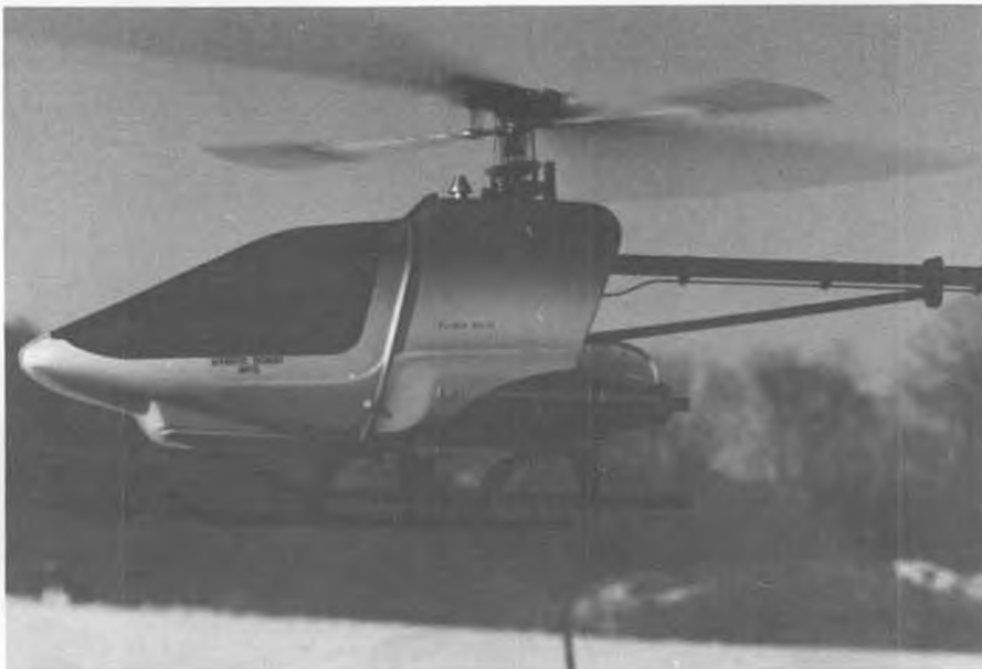
The author's Magic with canopy/luselage painted by Ray St. Onge, of Hybrid Hobby Mfg. Note the deformed area caused by the heat of the muffler.
