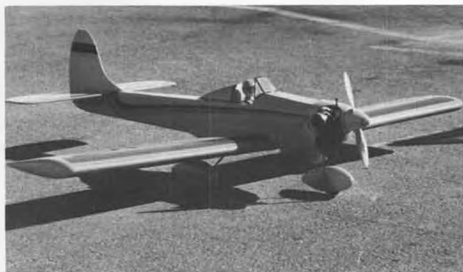
This Starhawk was jazzed up with rounded fin and rudder, wheel pants, and side-mounted engine.
