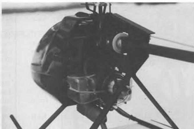
Rebel designed for regular 40-45 airplane or hell engines, standard mufflers. Cone start feature for airplane electric starters.
