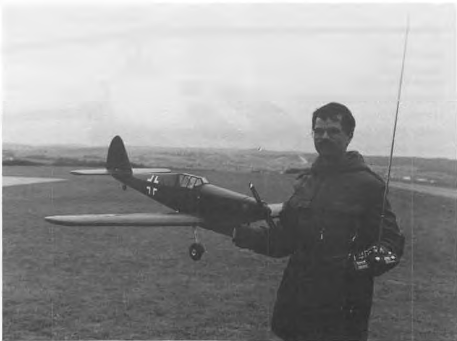
Fridtjof Schussler and his Keller 50/11 powered ME 109 from an Engel (Germany) kit. A .60-size model, it flies exceptionally well on 20 sub-C cells, weighs 7.7 lbs. See text.
