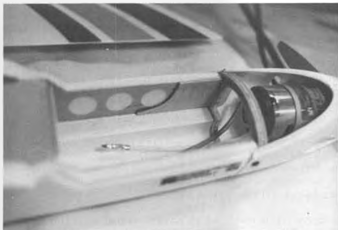
Motor attaches to light ply mount with four small screws. Motor housing is separate blow-molding.
