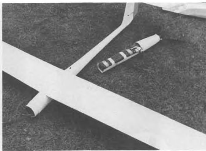
Removable nose with battery cradle is popular for F3E types. Makes for easy pack change. Throttle included in pod, in front of pack!
