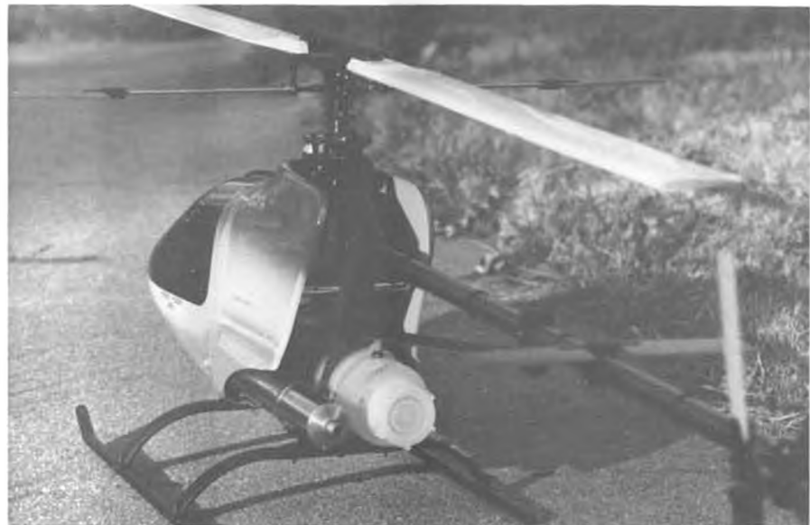
Like Champion and Scout, Magic has 20-minute fuel tank. Air hogs love it! Magic designed for Schlueter's own 924 silencer system. Adjustable incidence horizontal tail. Under-slung flyboy. 58.7-inch main rotor diameter.
