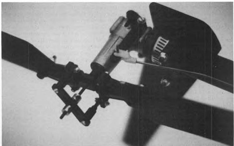
Tail rotor gear box is factory assembled. It is a wire drive system. The vertical fin is pre-cut from Bob Violett's Magnalite material.
