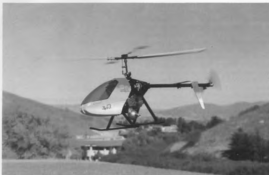
Soft flapping hingeless head makes Rebel very stable. Compact size (42-inch rotor diameter) makes it convenient to transport, yet big canopy makes it easy to see at a distance.
