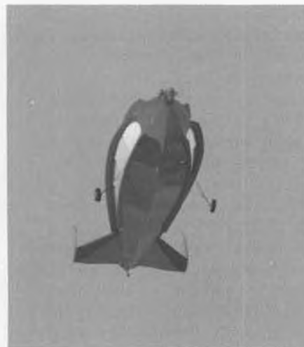
The R/C Space Ship is 60 inches long, "span" is 20 inches, dry weight is 2-3/4 pounds, power is an O.S. .25 and radio is three-channel. Construction article coming soon.
