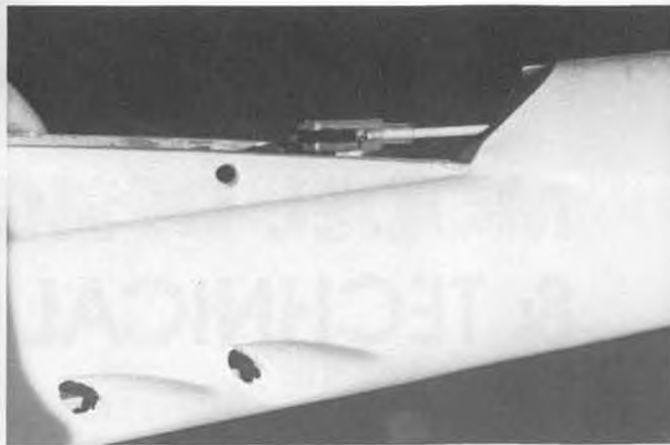
Micro servos are a must! Use inner control arm holes or excess height will interfere with hatch fairing.
