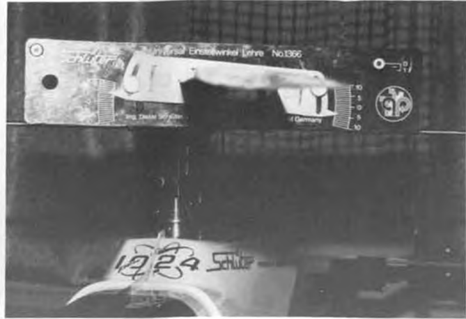
Schlueter pitch gauge is used to set the main rotor blade pitch. Very useful tool the author has used for the past six years.
