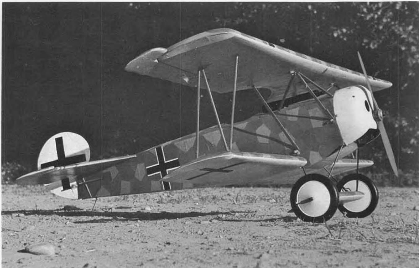
The Fokker D-VI was a little-known fighter in WW-I, but the family resemblance is easy to spot. Fuselage, engine, cowl, and tail surfaces come from the DR-1 or D-VIII, the cantilever wings are D-VII. Model spans 51 inches, weighs four pounds less radio. Superfigre 40 turns 11-4 prop. Photo by Phil Foster.
