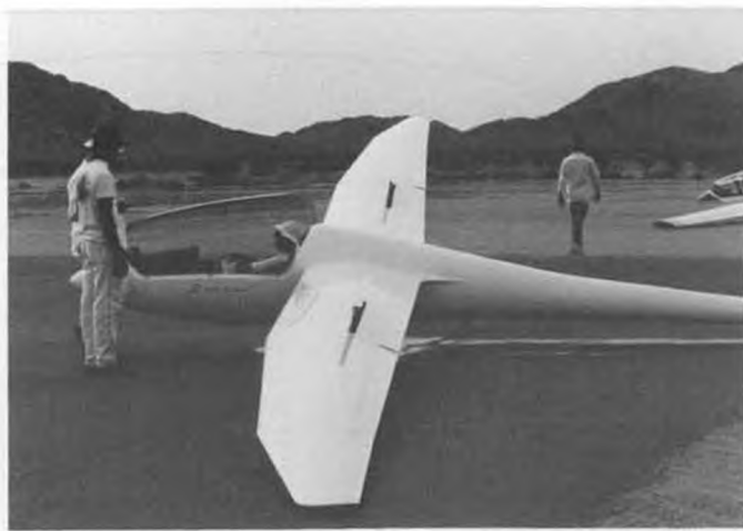
Tate Wilford offers Discus 3-view, along with photo of the real bird, showing forward sweep of trailing edge of main wing panels. Trailing edge goes to perpendicular at last tip panel, however.
