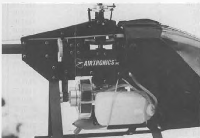
An 8-ounce Du-Bro fuel tank, metal swashplate, wide stance landing gear, easy, slide-on canopy. Everything simple.
