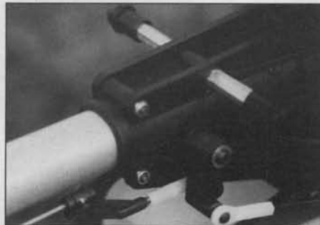
Canopy is held in place with the two posts sticking out at the back of the frame. The tail boom can be pulled off by loosening two bolts and the two posts. Tail rotor control rod can be disconnected at the tail boom and frame junction.
