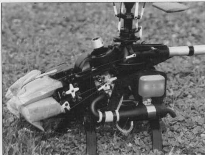
Left side of the Enforcer. Top servo is fore/aft cyclic. Middle servo is collective pitch. Bottom servo is throttle. If you have an Enforcer, then you will notice the servo sequence that the author uses is different from the instruction. When you build one you will see why. Century Import's Mini Tuned Pipe was used.
