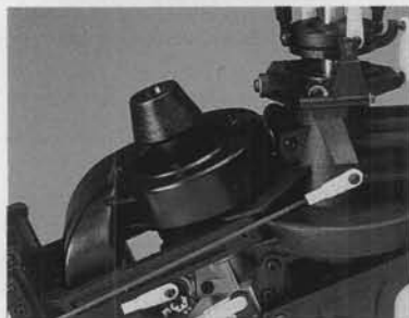
Top cone start and forward canted engine for easy engine starts.
