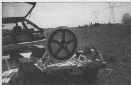
Brian Smith of Ohio mounts his winch and retriever to a small trailer. Easy transport, no lifting (bad back, you know), perfect alignment on setup, and easy maintenance (no bending over to work on it). That's pretty neat, agree?
