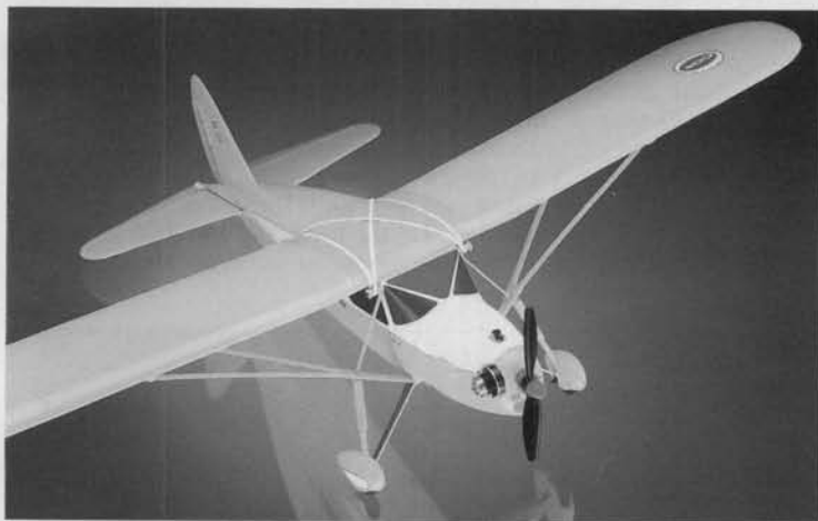
FAIRCHILD 24 38" Wingspan 28" Length Cox .049 Engine Powered
