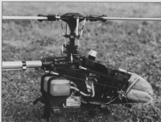
Right side of the model. Enforcer features straight pushrods from all the servos to the control bellcranks. The GMP gyro fits directly underneath the main rotor shaft. The kit comes with a gyro tray and clear plastic cover to shield the gyro from exhaust. Kalt kits are the only ones that come with a fuel filter. Use thicker fuel line than the one supplied with the kit.
