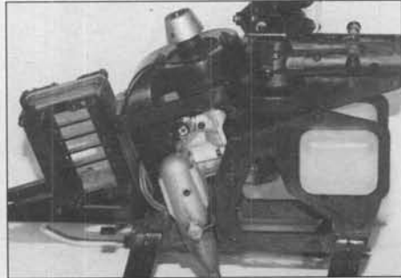
The main frame, with servo tray, and engine installed. Conventional aircraft style muffler can be used. The entire structure is made from injection molded plastic parts. They are almost indestructible.
