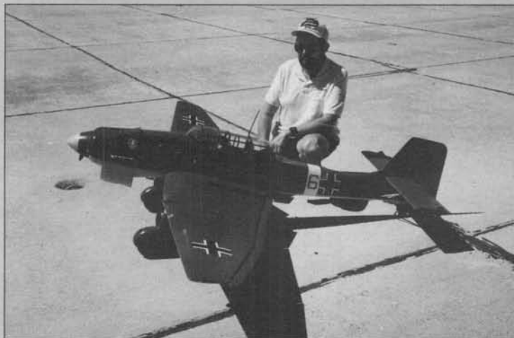
Bob Francis poses with his Stuka JU-87B. This Consolidated kit is powered by a Sachs 3.7, weighs 28 pounds, and has a 104-inch wingspan.
