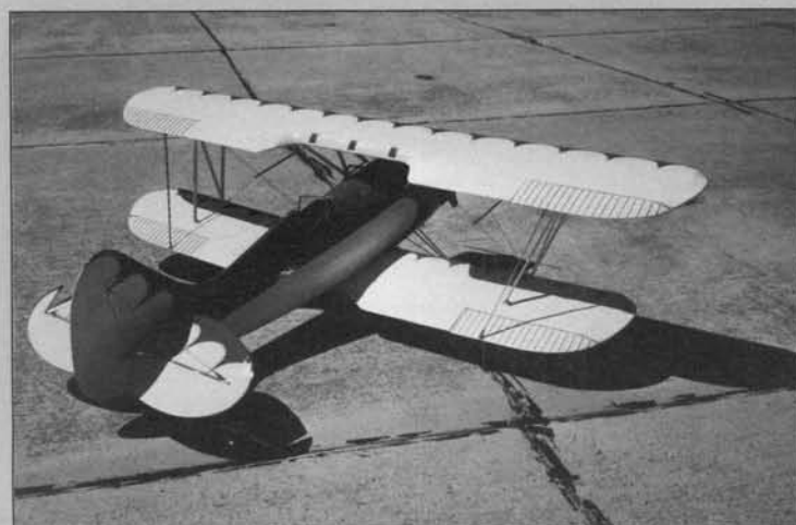
A Waco UPF-7 built by David Newell weighs 31 pounds, has a 7.5 ft. span and is Zenoah G-62 powered.
