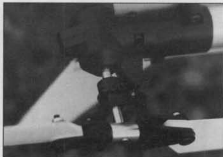
Tail rotor gear box is almost identical to Concept's. The sliding bearing pitch control system is very smooth; just like the bigger 60-size machine. Tail rotor response is excellent.
