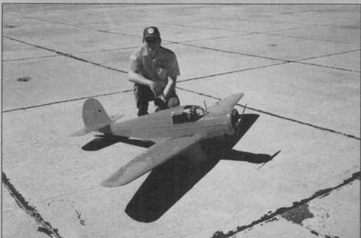
John Krohn powers his 20-pound, 108-inch Aeronca LC with a Saito five-cylinder four-stroke radial engine.
