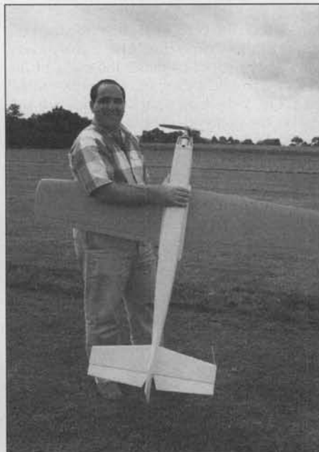
Gregor Poules' smooth flying Kaos is more of a precision aerobatic machine than a hot-dogger, performs well at 6-1/2 pounds on a geared Astro 40.
