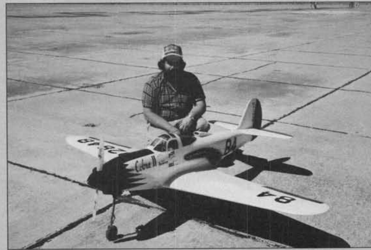
This Consolidated kit of the Bell Aircobra P-63 was built and flown by Joe Zimmerman. Power is a G-62, and the span is 96 inches.
