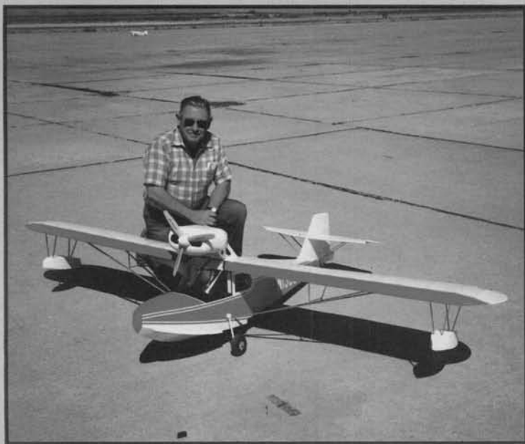
Harold Bayley built this Anderson "Kingfisher" from Tapsfield plans. O.S. 120 powered, it has a 9-foot span.
