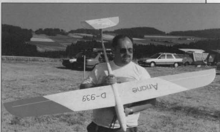
Very high-tech "Ariane 7" by Franz Weissgerber attracted a lot of attention. Not a single grain of wood inside. It is a reduced span and length version of the world speed record holder, and of the earlier Ariane flown at the last world championship.
