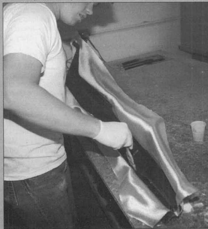
John Neff lays up a fuselage. All hand work.
