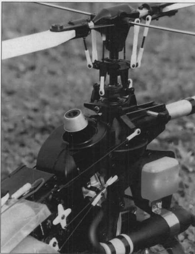
(Above) Top servo is for roll cyclic. Lower servo for rudder. A helicopter radio is highly recommended for any collective pitch helicopter. The kit comes with a very nice radio switch mounting plate that mounts on the servo tray. JR 501 servos fits nicely. JR 506 or 507 servos will not, because they are deeper and will bump into the servo behind them. (Right) Engine starter cone is canted up and forward. A unique Bell-Hiller mixing arm design gives 90% Bell-Hiller mixing ratio. The author is impressed by how the designer came up with the nifty geometry for the mixer.
