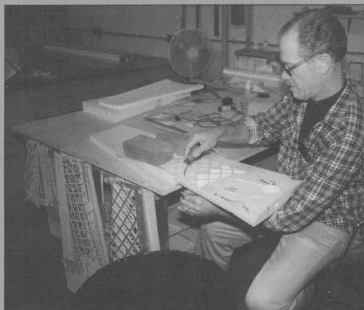
(Top) Jim Graham holds Ivan Kristensen's finished "Summit" wing cores. Quality shows. (Middle) Dave Birmingham, of RC City, honeycombs a Summit III wing for Ivan Kristensen. Note extra templates hanging from bench. (Bottom) Close up of the honeycombing rig. Metal plates on the fingers grasp the wire and carry the current.
