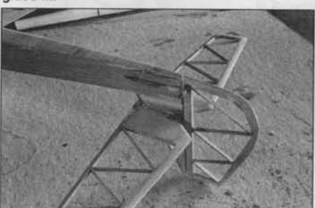
Rudder and stabilator control hook up.
