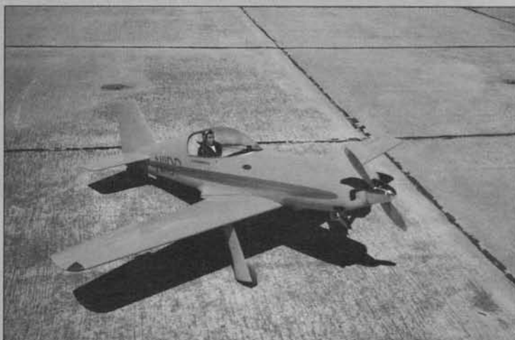
Duke Crow's Polen Special weighs 28 pounds and is powered by a Zenoah G-62 using RC's ignition system. Span is 82 inches.
