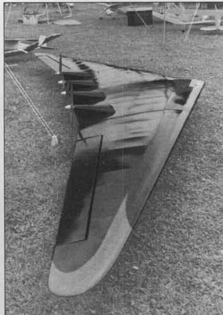
King Crimson spans ten feet and gets its power from four Leisure LT-50 motors. Needless to say, it steals the show wherever it's flown.
