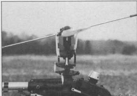
This shows the 90% Bell-Hiller mixing ratio on Enforcer which helps attribute to the hover stability. Notice when the flybar tilts, the blade pitch angle follows the flybar tilt. For example, if the flybar tilts 10 degrees, the blade tilts 9 degrees.
