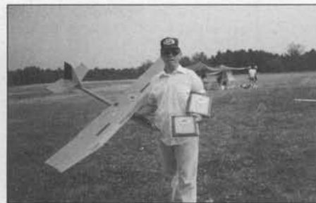
Brian Smith again, collecting the hardware with his original design 2-Meter Class ship with which he regularly cleans Unlimited Class clocks. Gentle Lady wing planform with Eppler 205 section. He says he loves it. No wonder, it works!
