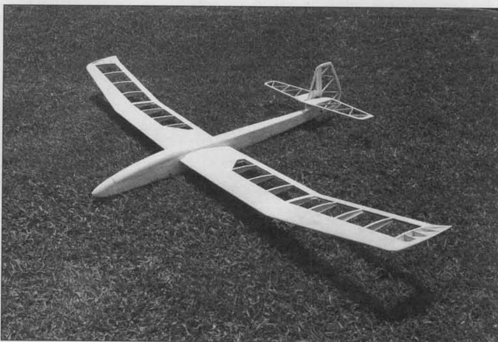
Structure detail. Note the built-up wing tips.
