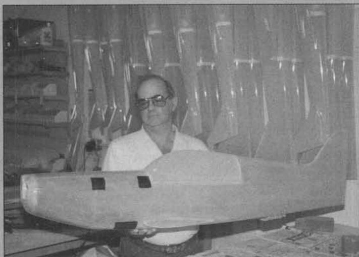
Finished TOC Skybolt fuselage weighs a mere 30 ounces!
