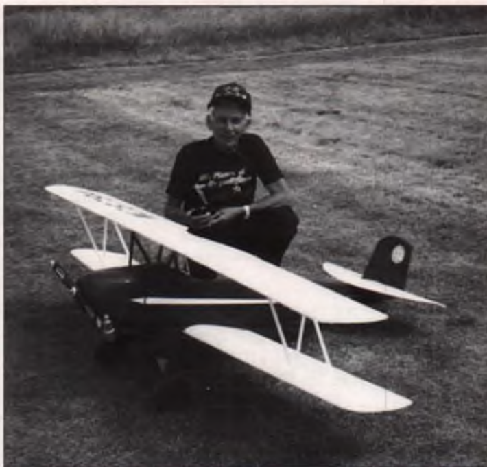
Budd Tamm said he liked the new Coverite 21st Century covering he used on his Concept Fleet biplane. The 18-pound plane uses an A&M 2.0 cubic inch Sachs engine.
