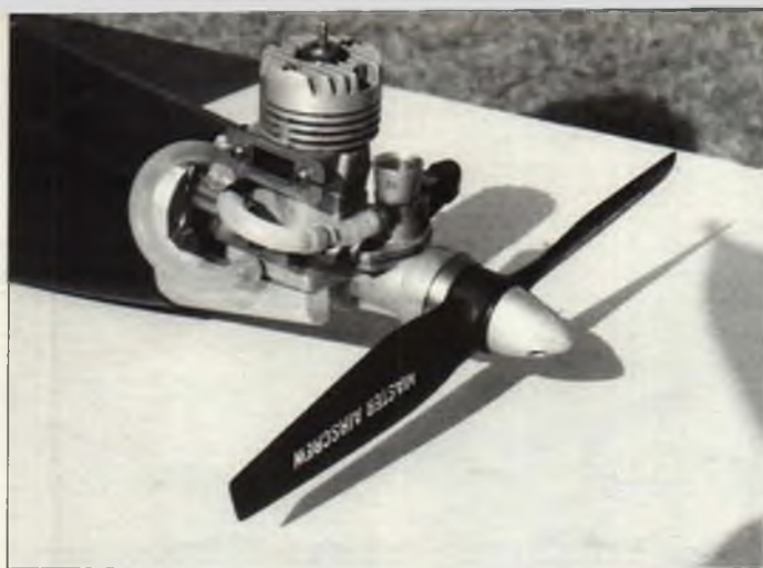
■ LEFT: The business end of Gale Holms' model sports a Fox .1588 with a 5/16-inch bore venturi and crankcase pressure setup—note that the engine mounting lug has been drilled and tapped for the pressure fitting. ■ RIGHT: Another Olympic 650 converted to C&G flying, this one by Patrick Beard of Baton Rouge.
