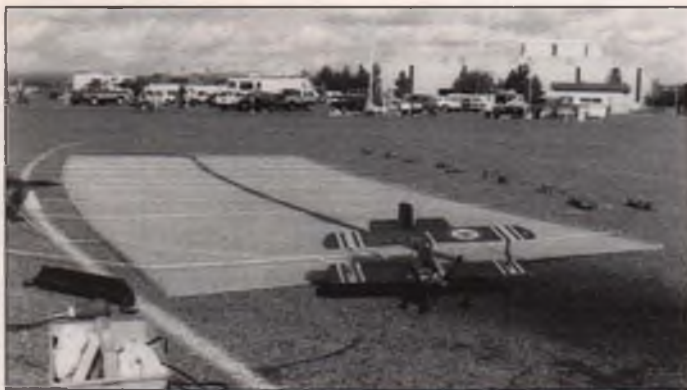
Carrier decks can be a fairly simple arrangement. This one, used by the Seattle Skyraiders, is wood laid out on the pavement, with eyelets to hold the arresting cords, and sandbags to hold the cords tight. The pilot splashed this landing. John Thompson photo.
