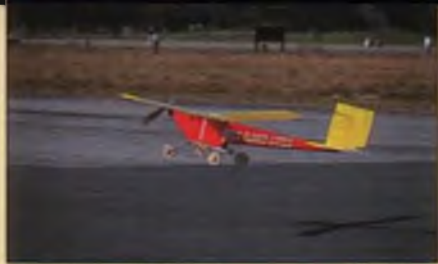
Joe Ballasch's High Plains Lifter takes off on its 2nd place cargo flight with 9 pounds 7 ounces of lead. Joe used two speed reduction drives in tandem to turn a monster 24x20 prop.
