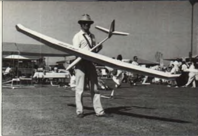
Jim Parsons and his DCU Wind Storm, finished just a week before the Visalia meet. Jim says it's an excellent flier, very smooth, and it finds lift for you easily. Features an SD7037 airfoil in the main panels with 1/2% less mean camber in the outer tip panels. The three-meter span model has 1075 square inches of area for a slightly less than 12-ounce loading.
