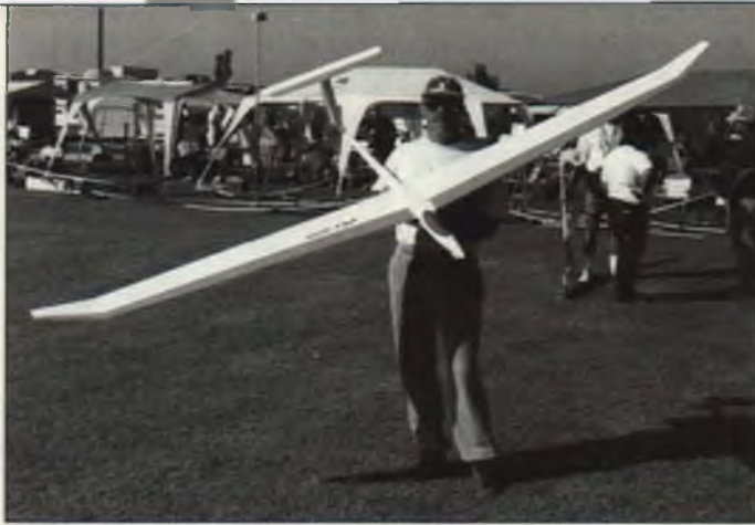
Dean Aldinger and his original design ship based on a David Mesa fuselage. Wing features the RG12 airfoil (more camber than an RG15) which Dean says has a more critical stall than the Selig 3021, which prevents it from being "horsed around." Model spans 120 inches and weighs 76 ounces, for an 11-ounce wing loading.
