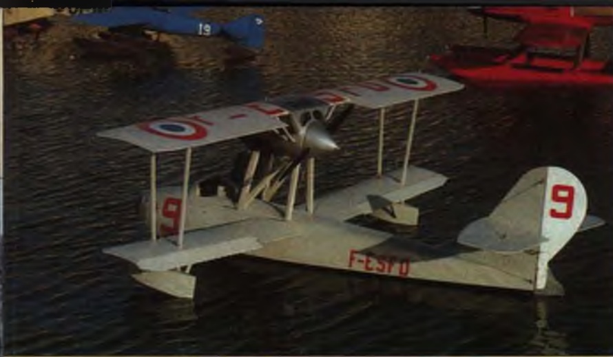
■ LEFT: Perhaps the most interesting airplane was this French CAMS 38 built by Dick Lucas and Lan Mace. The full-size aircraft never raced successfully, dropping out of the 1923 race with a structural failure. The model, which had the highest static score of the competition (82.3 points), uses traditional balsa construction, including over 100 wing ribs built up from 1/8 square balsa! Covering is Silts fabric and paint, power is an A&M Sachs 4.2 turning a 24x10 pusher prop. Dick says the model is very tricky to take off from rough water, and he and Lan sat out several heats when high waves would have put the model in peril. ■ ABOVE: A Sopwith makes a clean getaway. All of the 1914 Tabloids were about the same size and were impossible to tell apart once they got away from the beach.
