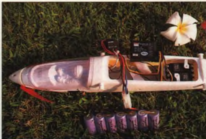
Fuselage with the receiver, speed control and battery pack ready to go in. Battery pack rests on a plywood tray, above the receiver and speed control, and is held in place with a Velcro strap.
