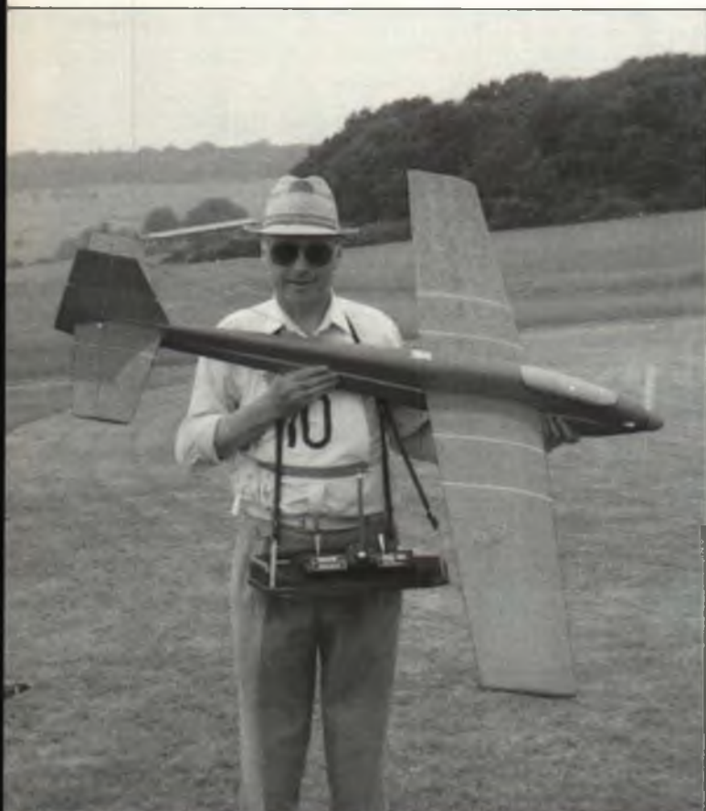
Arthur Kunkler with his original design Oreon electric pattern ship, which took 1st place at Weilmunster. Uses 24 cells, Keller 80/9 motor.
