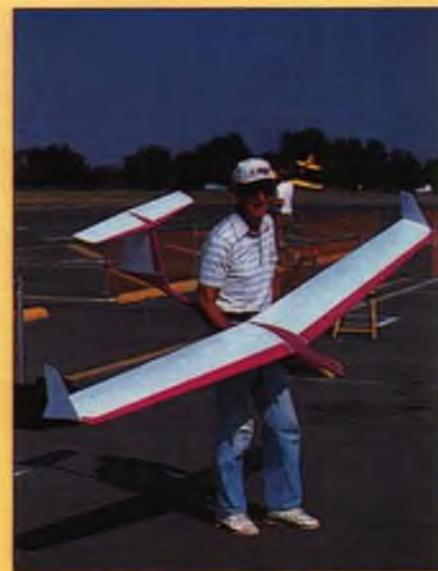
Chuck Hollinger with his winning Maxi-Fli Astro Cargo model. Chuck's model lifted 10-1/4 pounds of lead—in addition to its 4-pound empty weight—and could easily have carried more!
