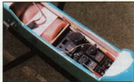
■ LEFT: Close-up of the wing center section, showing the aileron servo and linkage installation. Wing dowels on this model are at the trailing edge; the leading edge has two nylon bolts, held captive by the upper leading edge sheeting so they can't be lost or left behind. ■ ABOVE: The Futaba radio installation in the author's review model. Plenty of room for standard servos—these are Futaba S128s.
