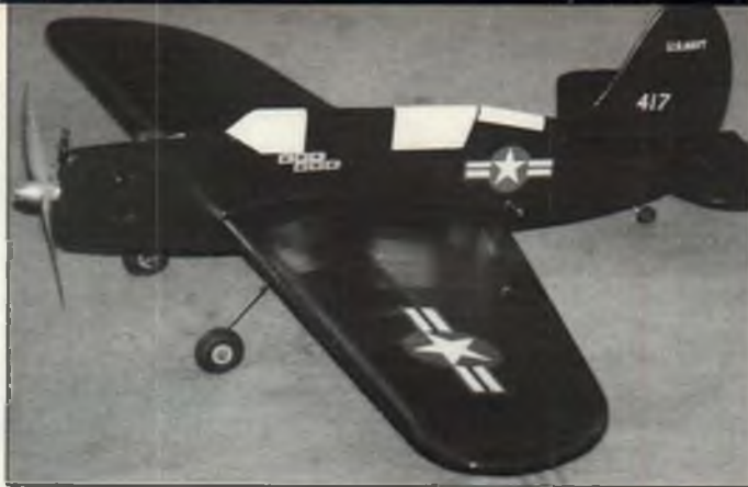
■ LEFT: John Hall's Sterling A2D-1 Skyshark for .15 Carrier, with a Cox Conquest .15, is the Northwest record holder at 194 points. It's a rugged, good-flying plane. ■ RIGHT: Hall's Curtiss SB2C Helldiver is a typical Profile Carrier model, built from a Goldberg P-40 kit and modified. K&B 5.8 power with an O.S. 4BK carb. K&B muffler (mufflers are allowed in Northwest contests), APC 9x7 prop. goes 90 mph on 60% nitro fuel. John has many contest wins with this relatively simple plane—no complicated line sliders or other tricks. Photos by John Hall.
