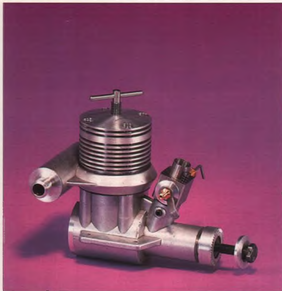
The P.A.W. .49 TBR comes with one of that company's unique one-piece cast aluminum mufflers, which clamps between the crankcase and the aluminum cylinder fin/head piece. The muffler is keyed by the four cylinder bolts and can be positioned as shown or on either side of the engine. Prop is held on by a standard 1/4-28 bolt that screws into the crankshaft.
