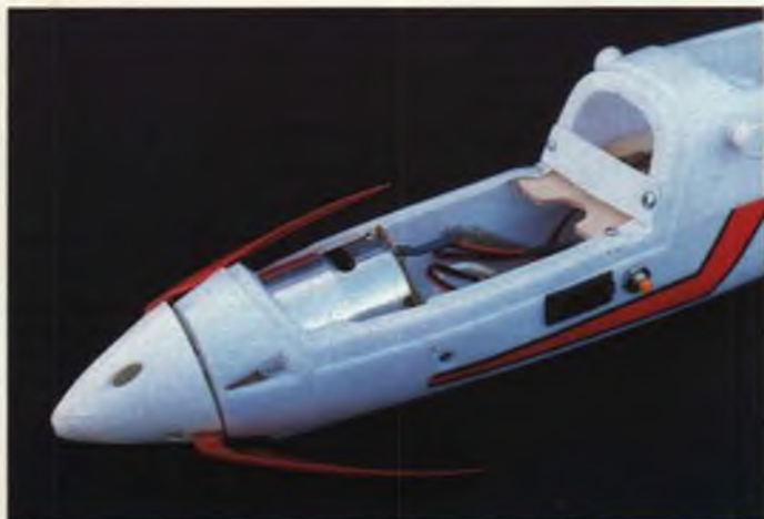
Close-up of the cockpit area with the canopy removed. Notice the author's battery retaining strap spanning the back of the cockpit. Cooling air holes in the spinner and fuselage are essential, as the motor does get warm.
