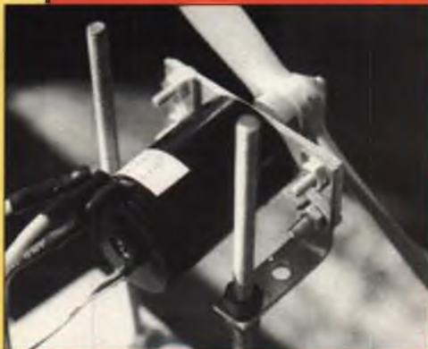
The Aveox motor that was being demonstrated at the Astro Champs—note the absence of brush holders. This seven-cell motor is physically about the same size as the "05" motors currently on the market.
