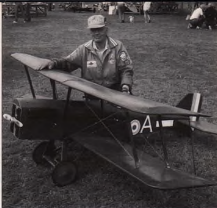
Tom Hammond scratch-built this 116-inch span S.E.5A using a modified set of Balsa USA Sopwith Pup wings. It's powered by a Quadra 50 and weighs 30 pounds.
