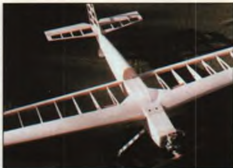
■ LEFT: The basic fuselage structure goes together quickly. The stringers support the balsa turtledeck sheeting, which has yet to be applied. ■ CENTER: Experienced builders can get the Fun-One framed up and ready to cover in only a few evenings. This photo shows the engine mounted upright, but Tom later laid it over on its side to get the exhaust down low—keeps the airplane cleaner. ■ RIGHT: The Super Tigre .34 looks small on the Fun-One but does a good job of hauling it around, even at the review model's flying weight of 4-1/2 pounds. Note the unique muffer, which can be pointed in any direction and can also be spaced close to or away from the engine as needed.
