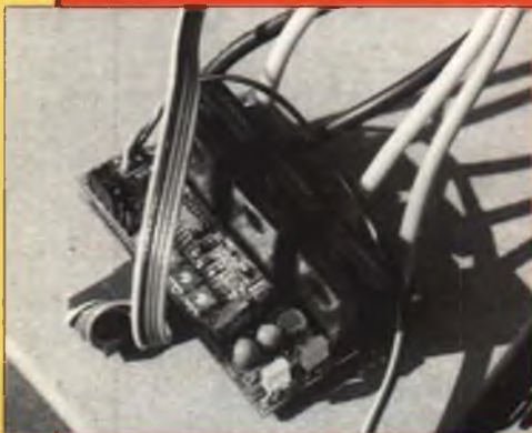
The Aveox electronic controller, an essential companion item to the brushless motor. It electronically does the current switching through the motor windings that the brushes and commutator do in a "regular" DC motor.
