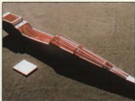
■ LEFT: The basic fuselage structure goes together quickly. The stringers support the balsa turtledeck sheeting, which has yet to be applied. ■ CENTER: Experienced builders can get the Fun-One framed up and ready to cover in only a few evenings. This photo shows the engine mounted upright, but Tom later laid it over on its side to get the exhaust down low—keeps the airplane cleaner. ■ RIGHT: The Super Tigre .34 looks small on the Fun-One but does a good job of hauling it around, even at the review model's flying weight of 4-1/2 pounds. Note the unique muffer, which can be pointed in any direction and can also be spaced close to or away from the engine as needed.
