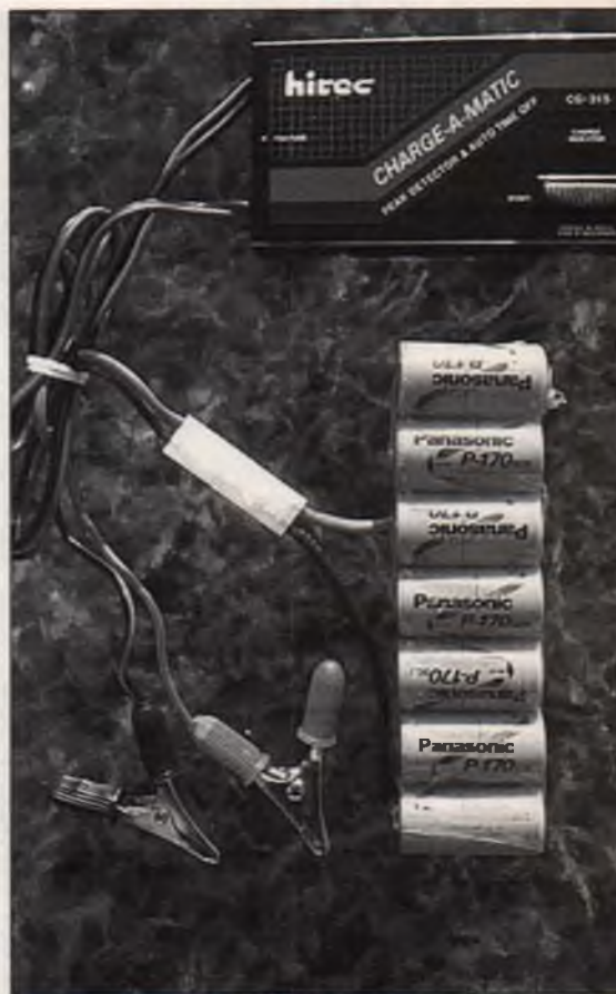
■ ABOVE: The stabilizer assembly as seen from the underside. Notice the cutout for the elevator joiner and the black band clevis keepers (one off, one in place). ■ RIGHT: Hitec CG 315 peak detection 12-volt DC battery charger with seven-cell Panasonic P-170 SCR battery pack.
