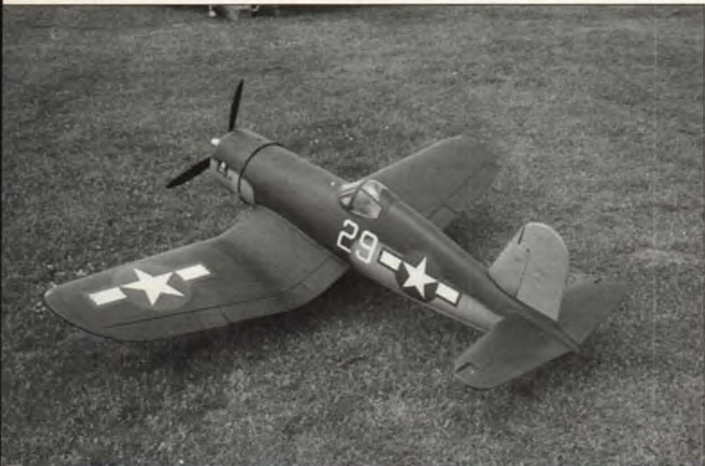
Byron's Corsair is a very fine flying plane. This one belongs to Canadian flier Ron Leavitt. It weighs 23 pounds. Power is a Sachs 4.2 with Purr Power muffler.
