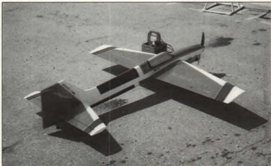
Dennis Breene's Flashback 3 original design. Y.S. 1.20, Futaba. The all-wood craft came in at 9 pounds. Photo by Dennis Breene.
