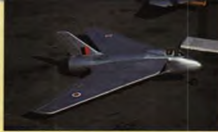
Bill Young's 2nd place finishing DH Swallow was powered by an Astro 15 turning a 7x6 duct-enclosed prop. Model's performance was lively and its sound was like a supercharged vacuum cleaner!
