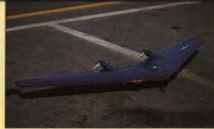
One of the most unusual entries in RC Scale was Bob Orfman's Northrop N9M-A. The scratch-built model uses an NACA 65, 3-019 airfoil and is powered by two Astro 6T 05s. Model has retract, is fast and surprisingly stable.
