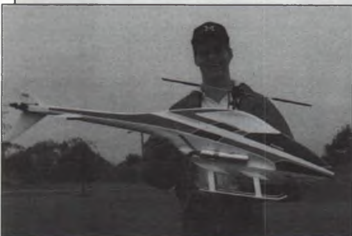
■ LEFT: Tim Lampe's Concept 60 is hidden inside a Kyosho Interceptor fiberglass fuselage. It has an O.S. .61 SX-H engine with Hatori 669 muffler. Stan Olzaski flew an equally beautiful Interceptor to 3rd place in FAI. ■ RIGHT: Cliff Hiatt transports his XL-Pro/Optima in this custom-made container borrowed from Ted Schoonard of Miniature Aircraft. Construction is cardboard with 1/2-inch Styrofoam, fiberglass cloth and epoxy. No disassembly of the model is required.
