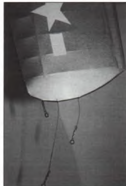
The elevator leadouts must clear the leadout guide at both extremes of the throttle range. Here the elevator leadout bottoms out at this end of the throttle range.
