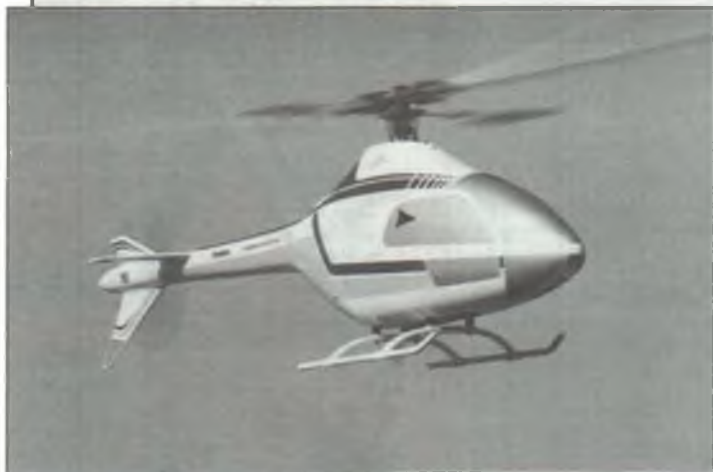
LEFT: This immaculate .60-size Miniature Aircraft XL-Pro in an Optima fuselage belongs to 1st place FAI winner Cliff Hiatt. It uses the new XL-Pro wood blades which have a 14 percent thick modified NACA0012 airfoil. Interestingly, the top four FAI winners all used Futaba 92HP radios with Futaba 153 gyros and S9201 servos. RIGHT: Second place FAI winner Tom Dooley with his backup model, a Hirobo Tsurugi. See text for an interesting discussion on how Tom sets up his models.
