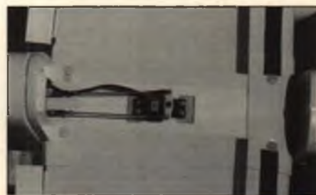
With just the canopy removed, the aileron servo and its linkages become easily accessible. Note that the wing is secured with four nylon bolts.
