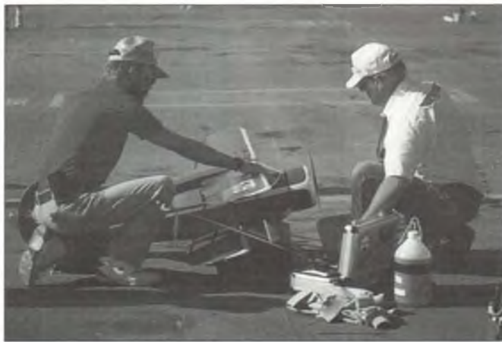
The big 76.4-inch span, scratch-built VKS 7F Waco Cabin took Charles Nelson to a 10th place finish. The 16-pound biplane is built to 2-1/4"=1' scale and features flaps, operating position lights, anti-collision beacon, and retractable landing lights. It's a copy of the last Waco ever built. Finish is Sig Coverall and dope. Charles came all the way from Berlin, Massachusetts to compete in the Scale Masters.
