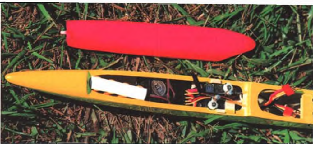
Radio gear is a tight fit within the narrow confines of the Dove's epoxyglass fuselage—which, incidentally, is the same one used on NSP's sleek Sparrow slope glider. Here, two RCD Apollo 24 micro servos (rudder and elevator) are mounted side by side at the rear of the cockpit; in the middle is an RCD 535 FM micro receiver, and up front is a 270-mAH battery pack.
