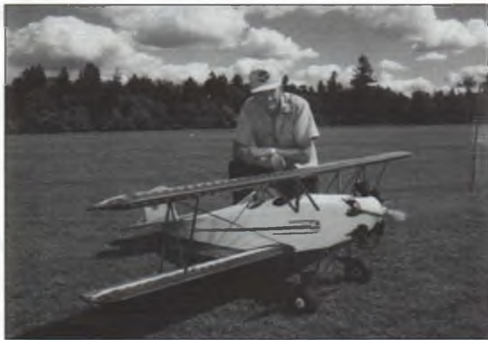
A favorite of biplane lovers, this 1/4-scale Fleet was built from the Concept Models kit by Bob Kreuzinger. The Zenoah G-38 powered model weighs 22 pounds. Photo by Brian Lea.
