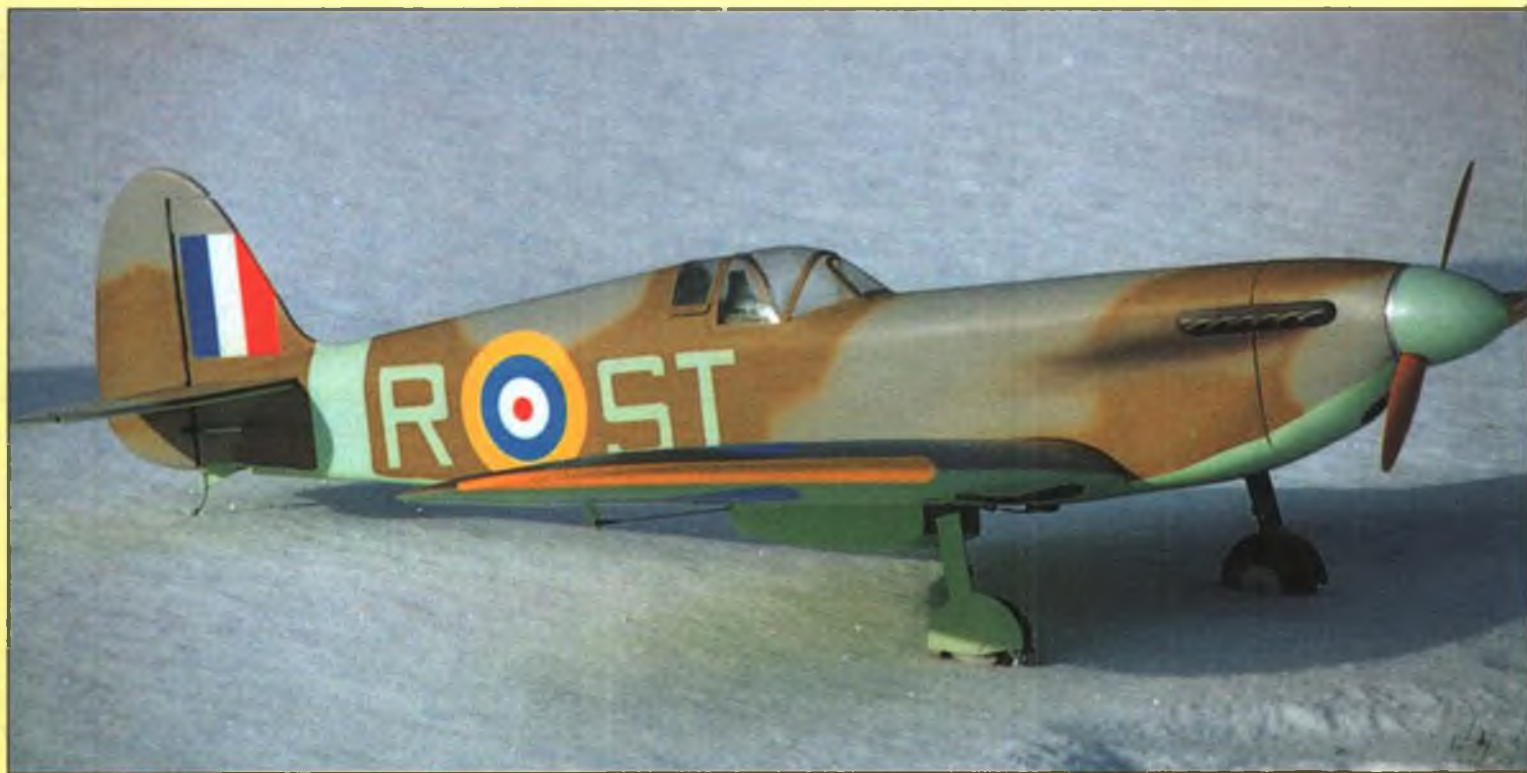
Well-known proponent of electric power, Bob Benjamin turned out this 81-inch span Dynalite Spitfire, powered by an Astro Flight cobalt 60 on 28 cells. Bob has prepared an article on converting large gas models to electric power, using the Spitfire as an example—watch for it in an upcoming issue of Model Builder .
