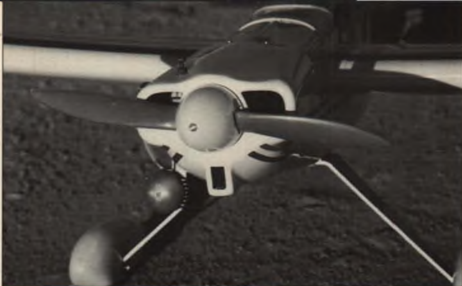
■ LEFT: Handsome ABS plastic cowl comfortably houses the potent O.S. .61 SF ABC and contributes to the airplane's sleek lines. ■ RIGHT: Removing the canopy and wing allows easy access to the radio—in this case, an Airtronics system.
