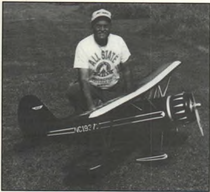
Harb Brice has a ball flying his Waco VMF-5. It spans 90 inches, weighs 30 pounds and is powered by an A&M Sachs 3.2.
