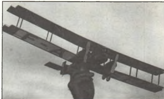
Winning the 1994 Flying Aces Club Achievement Award was Terry Pittman's remarkable Farman F.60 Goliath, which later vanished O.O.S. in a thermal. Spanned 24 inches, power came from two Keweenaw electric motors running on three 70-mAH NiCd cells.
