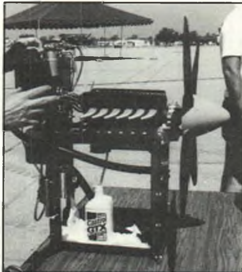
Here's a real challenge for you machinist types: a working replica of the Rolls Royce V-12 Merlin, offered as a castings kit by Richard Mahoe—see text. Total displacement is 25.75 cubic inches, weight is 18.5 pounds, rated at 15 horsepower at 4,000 rpm.
