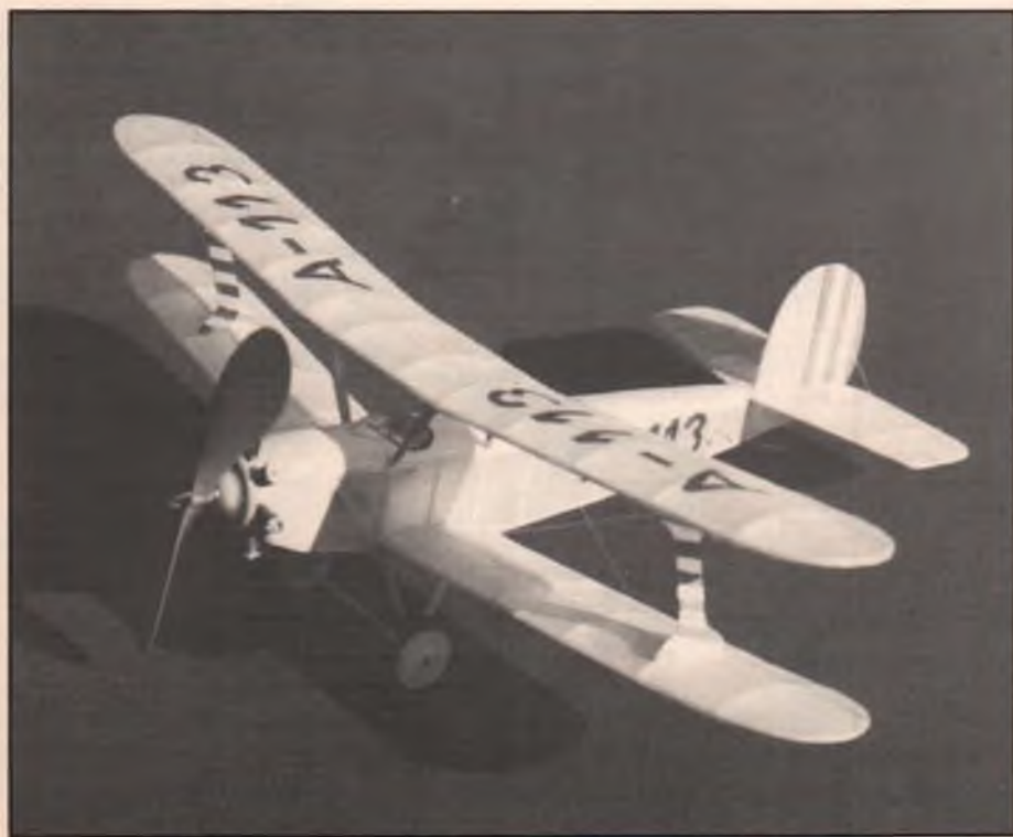
The plans show sheet balsa wing and tail tips, however, the prototype model has laminated basswood tips on the wings and vertical tail. The fuselage luffdeck could also be covered with bond paper instead of the 1/64 sheet balsa shown. Keep the weight to a minimum for best flight performance.
