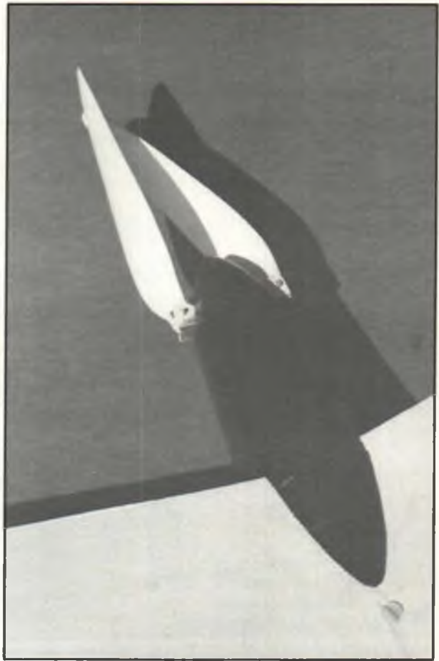
With no stops on the pusher's blades, they were free to fold over-center; fold a blade too far and it won't open on motor start-up, making for one startled pilot and a possibly damaged airplane.
