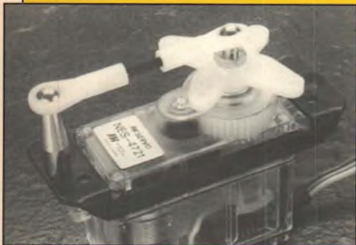
For those who demand absolute precision in their control systems, JR produces this metal servo tray and ball system to eliminate any flexing of the servo output shaft.
