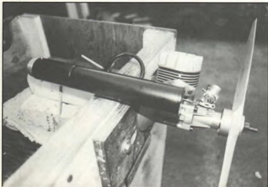
Bruce's backyard test setup included a Davis Model Products S.M.T. muffler to keep the neighbors happy.
