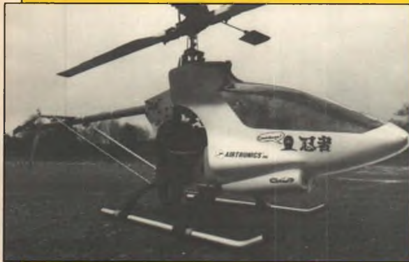
James finds the .30-.40 Ninja Pro canopy fits his .60-size GMP Legend very well. Has a Hirobo DDF rotor head, O.S. .81 RFM engine and Magna U-pipe—a great flying combination. Canopy is painted from the inside using RC car spray paint.
