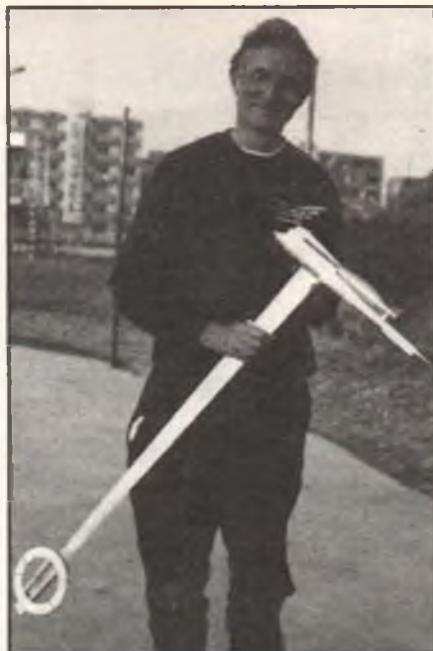
Typical of modern F2A speed models is this long-wing asymmetrical ship flown by Gordon Isles of Great Britain. Gordon's best flight was 289.2 kph—not enough to win, but good enough to put the British team in 1st place. Chen Xia photo.
