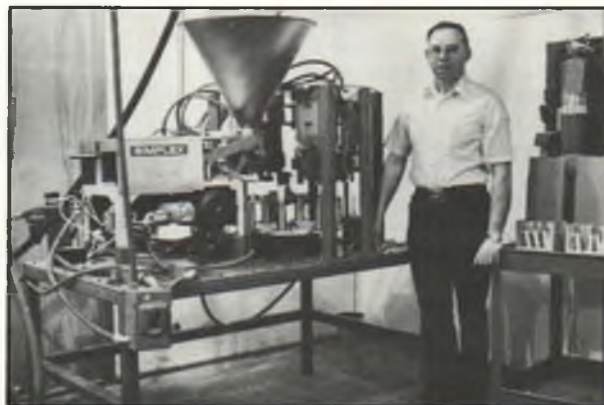
An example of Glen Sig's mechanical prowess is this one-of-a-kind machine he designed and built; it automatically files, holds and crimps Sig-Ment glue tubes at the rate of 15 per minute.
