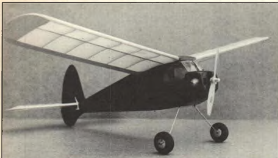
Nice photo of a Vic Smeed designed Chernub, as modeled by Mike Parker of Great Britain. It's powered by a scaled-down Mills diesel of .048 cubic inch displacement. These engines are produced in Russia and are known as "Milliskis" in Britain.
