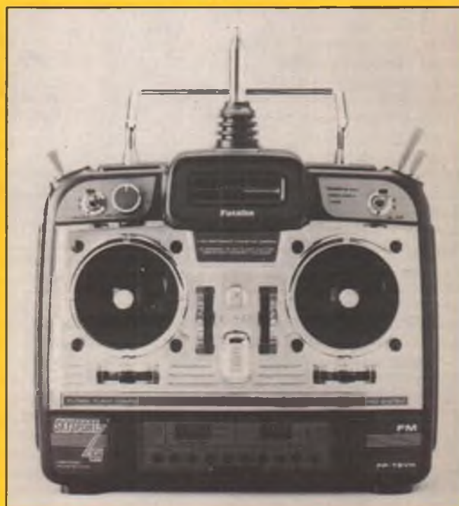
The SkySport 8VH is Futaba's low-priced entry-level FM heli radio, comes with four S148 standard servos, a 1000-mAh airborne battery, and a reliable R127DF FM receiver. The transmitter has a rounded, ergonomically shaped case and only the essential heli features that beginners and sport fliers need. Futaba photo.
