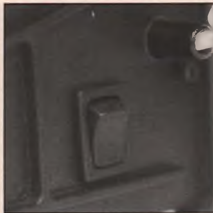
Should you prefer an on-off switch to installing and removing the power plug, one can be added simply, as seen here located just under the power plug. Details in text.
