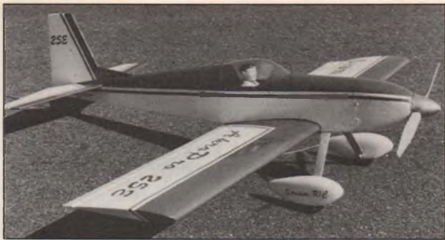
This sleek 42-inch span sport/aerobatic electric is the Akro Pro 25E, the latest kit from Stream Inc., P.O. Box 1113, Newport News, VA 23601; (804) 691-0720. It's designed for the Model Electronics Turbo Plus geared motor and a 18-cell battery pack. Quoted flying weight for the 410 square inch low-winger is only 84 ounces.
