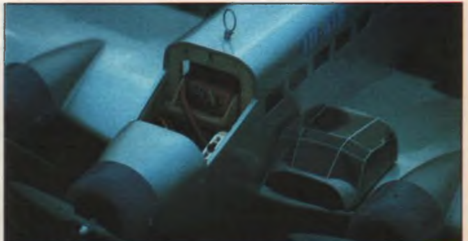
An excellent design feature of the Junkers is the quick and easy access to the motor battery via the removable canopy. A single seven-cell 1700-mAH SCRC battery pack runs all three motors and is good for flights of seven minutes or more, depending on how aggressive you are on the throttle.
