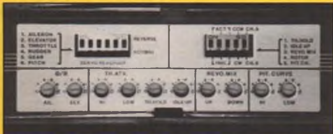
The SkySport transmitter's trim pots and servo reversing/mixing switches are protected underneath the transparent front cover.
