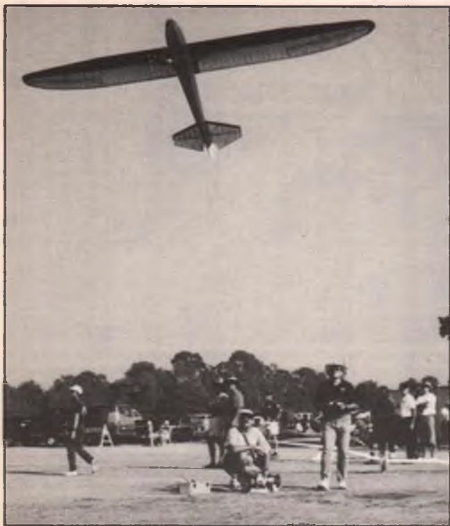
Second place honors for Best Vintage Sailplane went to Rex Powell and his Gruman Baby 2. Here's a shot of it going up the winch line under the guiding thumb of Dave Hall. Towhook position at the 1/4-chord point at the skid produced rapid rotation on takeoff. The Baby's lows were straight and steeper than most.
