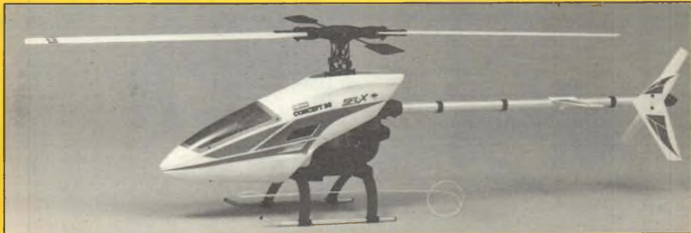
The Concept 30 SR-X is the latest evolution of the popular Concept 30 series. It has the same physical dimensions as its predecessor, the Concept 30 SR-T, but the SR-T has fewer ball bearings, no autorotation bearing, and a smaller 1.6mm tail drive wire. The SR-X's canopy is a different shape, too. Photo courtesy of Great Planes Model Distributors.
