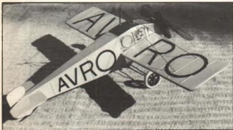
Flightmasters member Frank Faraco fabricated this fabulous “cartoon scale” 1012 Avro F from the. When mounted on a counterbalanced arm, the spring-driven propeller “flies” the model in a circle.
