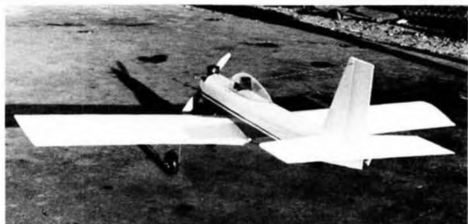
Lines of the FB (Fun Bird)-100 are clean and simple. Rolled ply fuselage is strong yet light. Canopy was added attraction.
