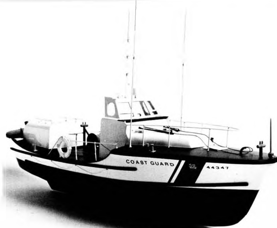
U.S. Coast Guard 44 foot lifeboat, scaled to 33" length and kitted by Dumas. For R/C and electric power. Built of die-cut mahogany frames and planked with 1/8 x 1/2 inch balsa.
