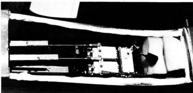
Installation employs the mounting tray furnished with the radio. Dow-Corning silicone rubber liner keeps out the exhaust gook.
