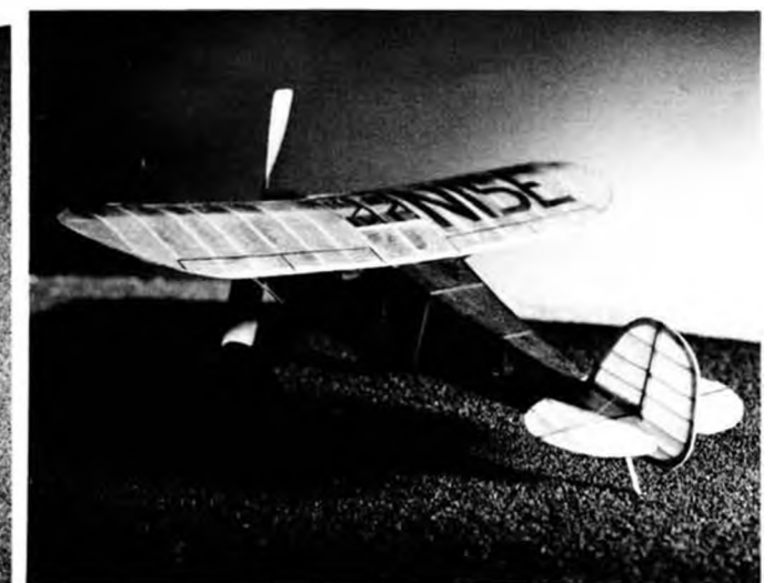
Long tail moment gives the little ship plenty of stability. Prop clearance is a little doubtful, but plastic is tough!
