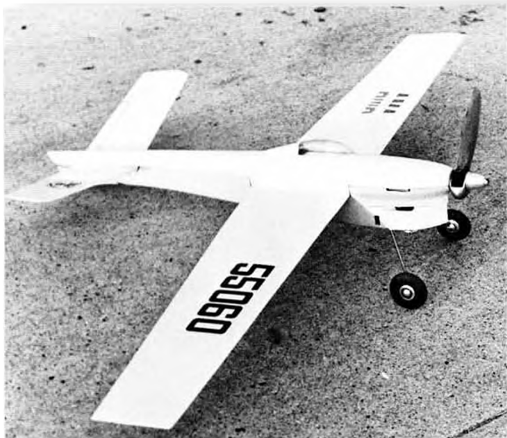
Half-A Proto speed plane by Jim Wade. Power is a left-hand Tee Dee .049 with single blade prop. Kirn-Kraft glass fuse, Cox pan, 90+ MPH.
