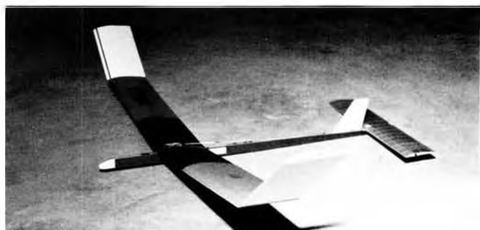
Note flat-bottomed airfoil and tip washout. Design is more stable in the usually unfavorable conditions found at a contest.
