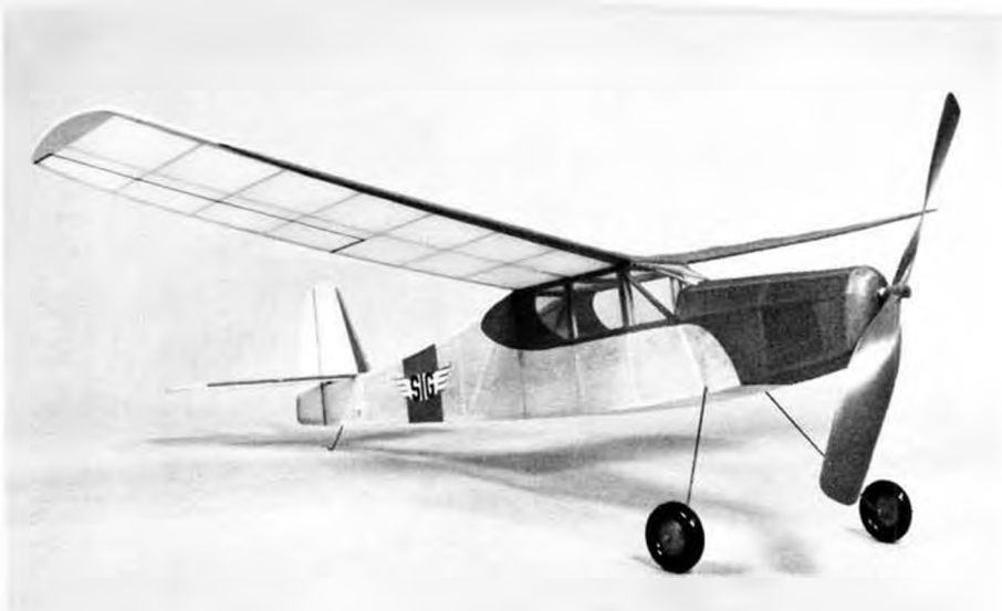
Third in the Classic Series being produced by Sig Mfg. Co. is this 21-1/2 inch span Tiger rubber powered model designed by Paul McClrath.
