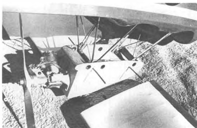
View of underside of centersection, with wing panels ready for hook-up. Note left-hand prop which was hand carved. Not really difficult.
