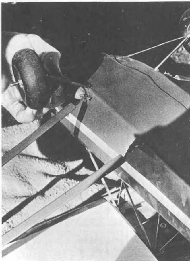
Functional wing struts are hooked on using Rand keepers. "Z" bend in 1/16 wire provides adjustments for length. Note receiver antenna.
