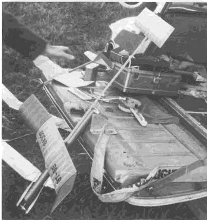
Small unlimited rubber model designed by John Clear around the Estes BT 55 rocket tube. Uses 8 strands of 1/4 Filati. Really goes.
