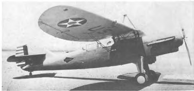
A later Wright Field O-43A with landing lights for night flying. A loop antenna and wing flaps have also been added.
