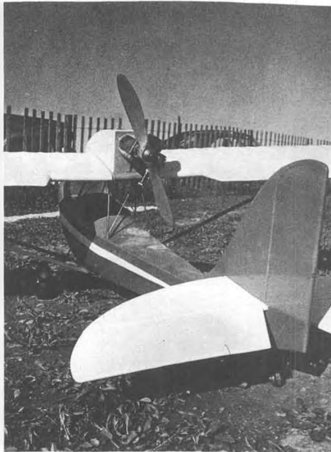
Here's a good view of left-hand prop. You can get left-hand cranks for some engines, but carving a prop isn't bad, and it'll last forever.
