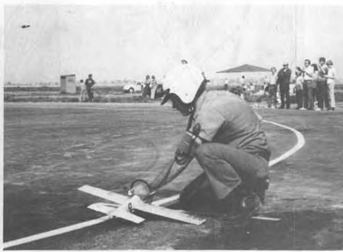
Dan Barker restarts his FAI Team Racer. Note pressurized refueling system strapped to his arm. Valley Circle Burners meet, March 17.
