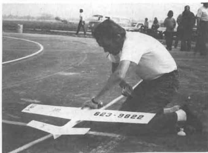
Denny Schauer restarts Slow Rat fitted with ST 35 converted to diesel. Note Allen key in mouth and finger guard, standard equipment.
