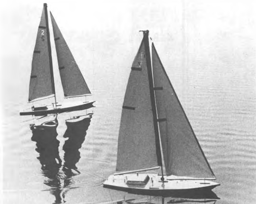
A couple of modified Pea Pods (Model Builder Plan No. 4733) built by Dick Stone and Charles Graf, Severna Park, Maryland. Beam was reduced, cuddy cabin added. Sails are nylon taffeta!
