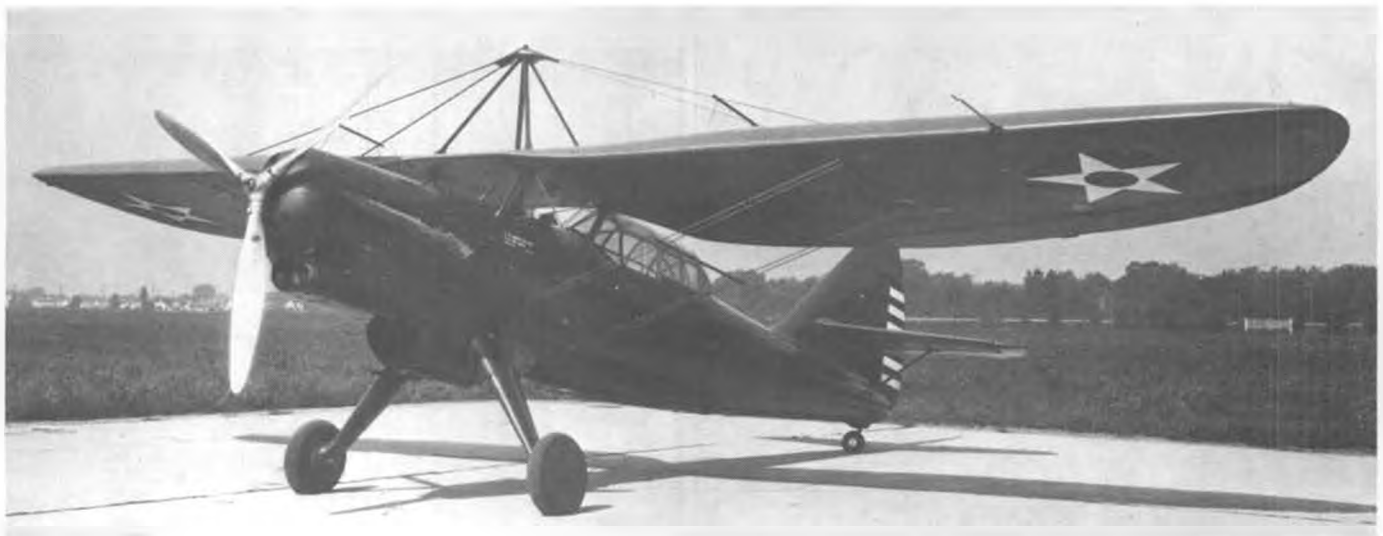
The O-43A at Wright Field with new increased vertical tail area and inset rudder.
