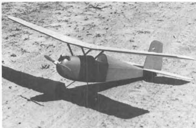
Tern Aero's neat little Starduster for .020, can be flown free flight or R/C, using one of the small Ace pulse units. See text for details.
