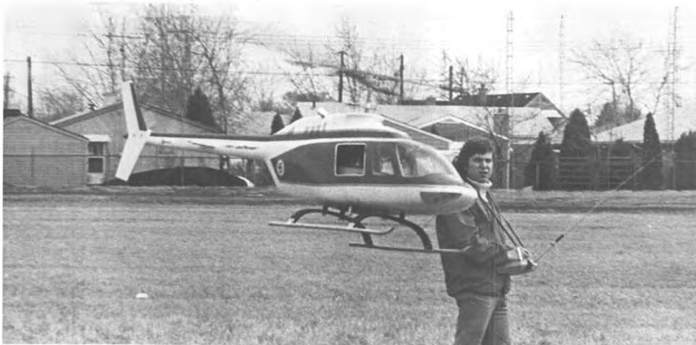
Mike Bosch, son of well known German R/C flier, is the R/C helicopter champion of Germany. Here he demonstrates the Kavan Bell Jet Ranger at the Toledo R/C Conference. This model was equipped with the latest head and the stabilizing gyro.
