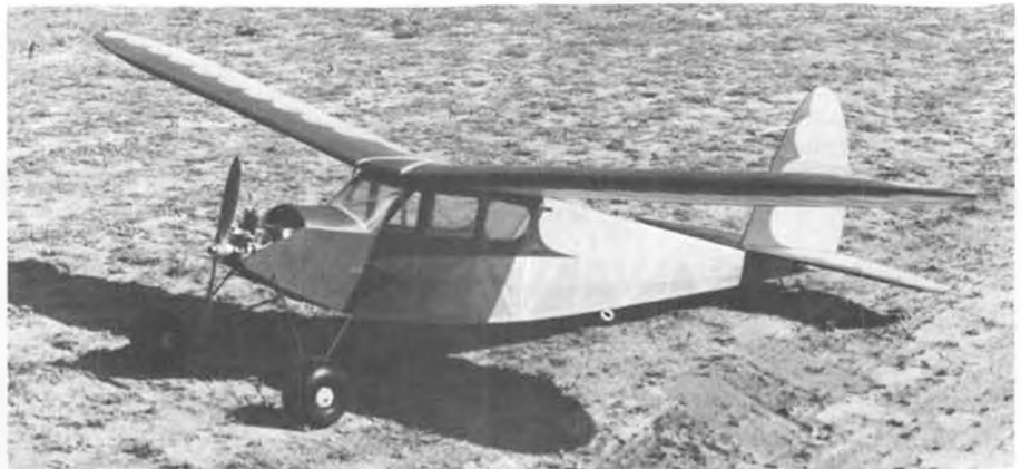
F/F Scale columnist Fernando Ramos' Flying Quaker weighs 3 pounds with Kraft 3 channel gear and Enya 45 engine. No need to say how well it flies.
