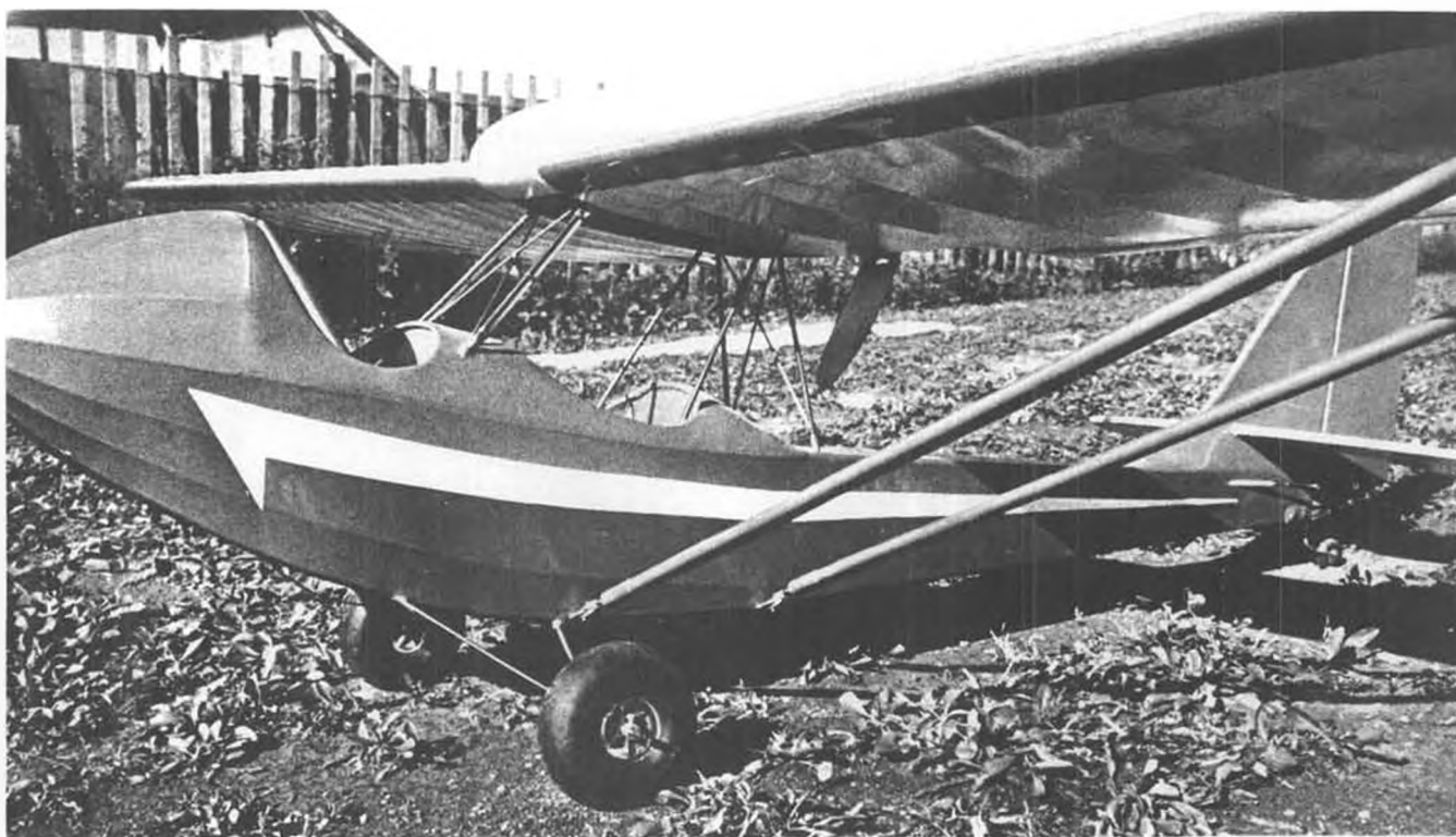
Close up shot reveals a extra strut added on by Ralph to beef up the landing gear for rough field operation. Ain't she a cute little cupcake?
