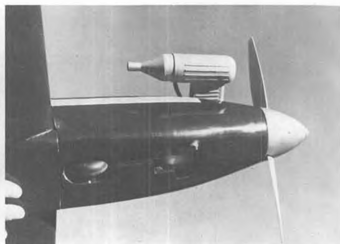
Goldberg retract nose gear in sucked up position. Note pressure tap line from Veco muffler. Fuselage and spinner blend nicely.
