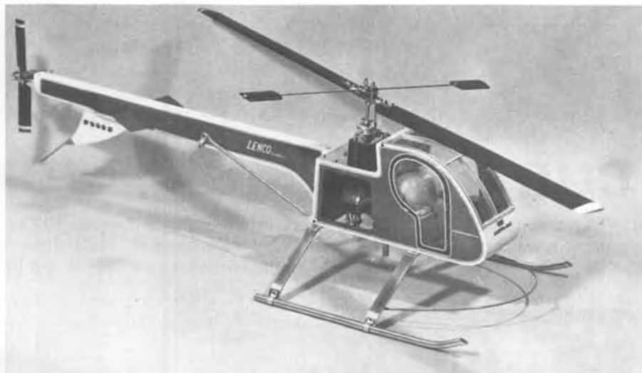
Len Sabato's latest design helicopter features easy, built up fuselage and bolt-together mechanics. Will sell for less than $300.
