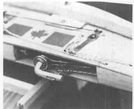
Close-up shot of Bill van Dieren's Russian tow-hook system in his Chickadee A/2.
