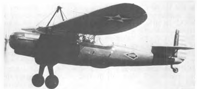
Prototype of the O-43A was one of the Y10-43's. Note the short nose, reworked cockpit, and belly blister.
