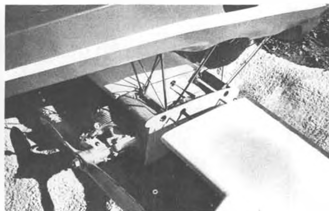
Right wing is shown attached, and aileron clevis is hooked to crank. Wing is held on by rubber bands to cup hooks. Power is an Enya 35.
