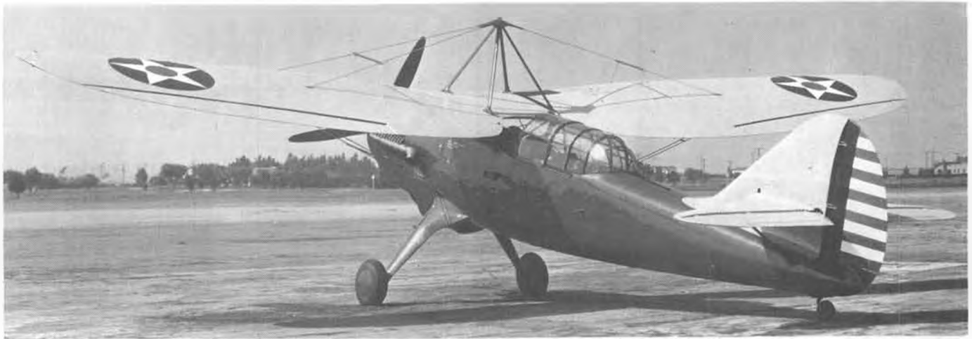
The ancient Morane parasol wire bracing was still a feature of the O-43A. Small vertical tail was soon changed to larger size.
