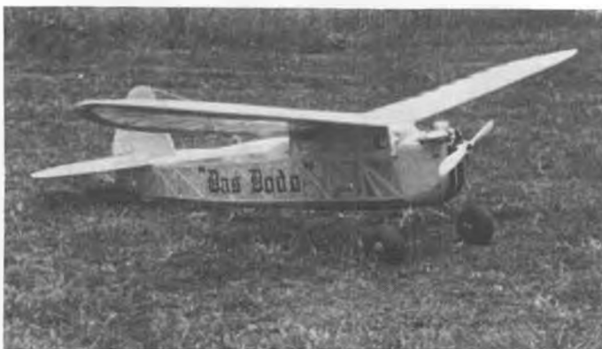
Don Heckman's Buccaneer C Special is powered by K & B 40, R/C by Heathkit. Don, from New Jersey, built it from an original kit.
