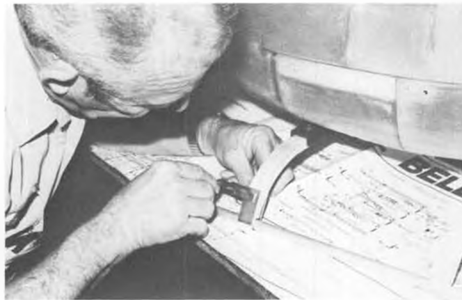
Clamping gear skid straps prior to to drilling for mounting bolts.
