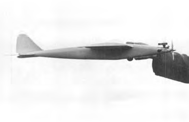
Bob Mikko's Half-A streamliner. Heat sink on head saves plugs. Pig-tail antenna is typical. Note two wheels in fuselage. Allowed by rules.
