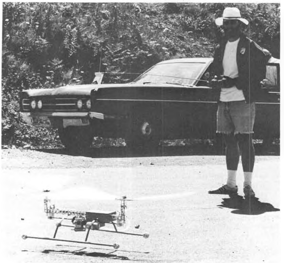
Jerry Holcomb flies his experimental tandem twin rotor helicopter. It is not perfected yet, but test flights show steady improvement. Photo by Bob Yorkston.
