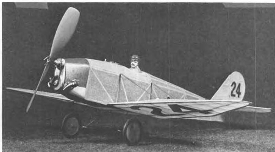
Parnell Pixie to one inch scale, by Bill Byshyn, Brooklyn, N.Y. Span is 17-1/2", length 18". It weighs 1.3 ounces.
