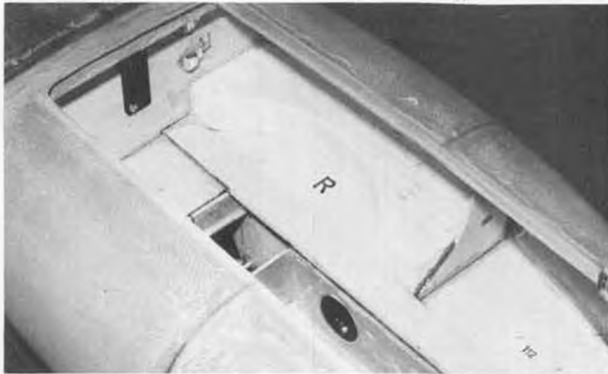
Bottom view shows tank mount (cut-out for gear) and clip for rubber band strap.
