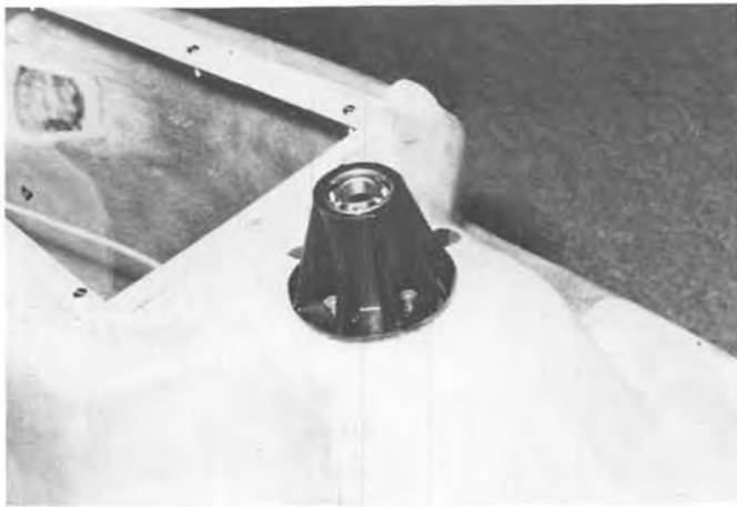
Trainer modification upper bearing imbedded in epoxy.
