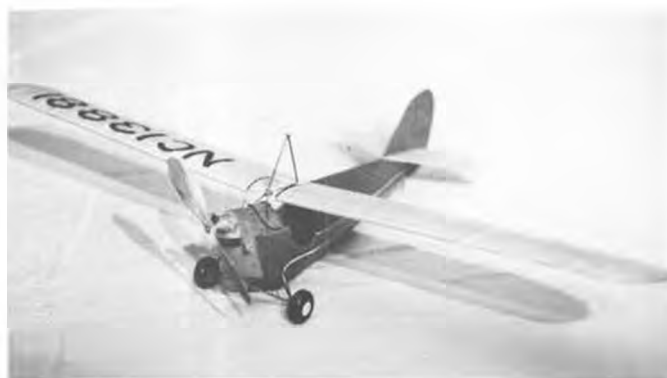
Brown CO 2 powered Aeronca C3 by Daniel Walton. Ship is built to 3/4" scale and features realistic structure.
