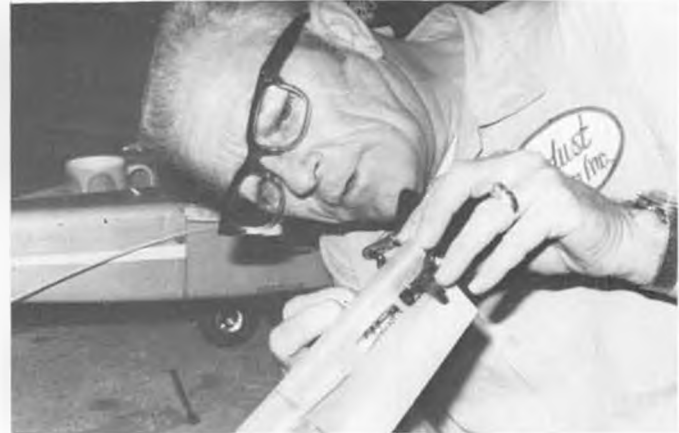
Final installation of tail rotor gear box. Yup, sure is a Tauri!
