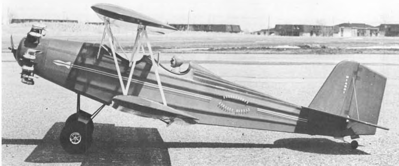
Williams Brothers scale cylinders and pilot add a lot to the realistic appearance of the ship, both on the ground and in the air. Sig Lite-Ply fuselage sides are light in weight, but very strong. Note shadows from side stringers. A kit is about to be released on this model, put out by the author.
