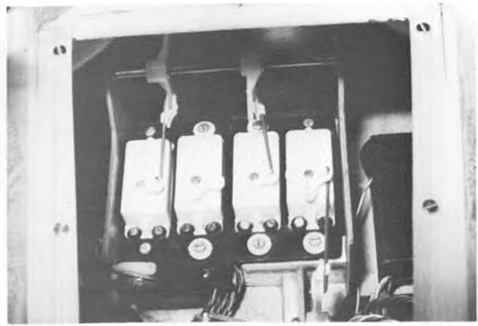
All servos installed. Radio receiver on right side, battery on left.
