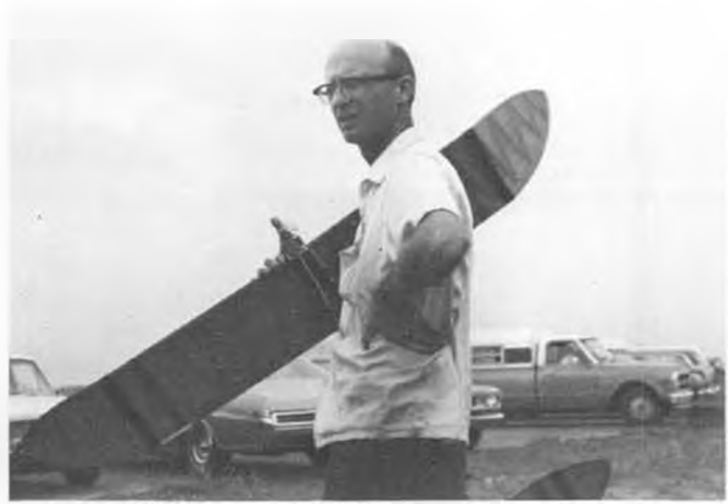
Bob Sifleet and his Centaur FAI Power model. Note wash-in tab on inner right wing panel.
