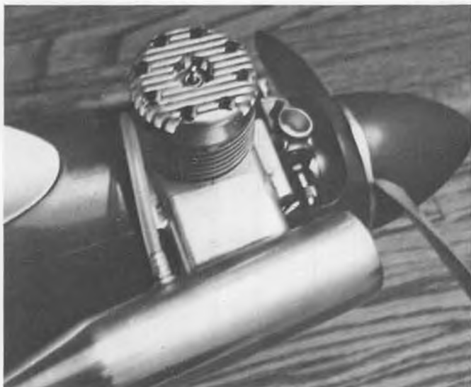
Supertigre G60 ABC engine with venturi muffler and pressure take-off. Venturi mufflers have stupidly been ruled out by FAI.
