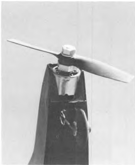
Motor installation. It is cemented into hole in firewall. Air inlet and outlet holes important.
