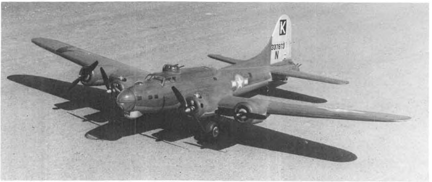
Looks can be deceiving. If it wasn't for those Cox .020 Tee Dee engines, you might not realize that this B-17G has only a 39 inch wingspan. Built from a Sterling kit by Masayuki Suzuki, of Tokyo, Japan, it has a Futaba radio on rudder, elevator, and engine cut-off, using two channels.
