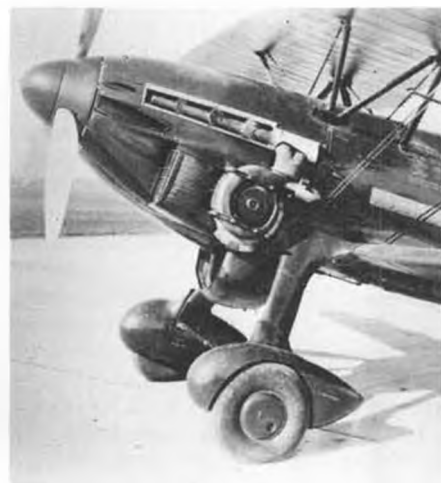
Close-up of GE F-26 supercharger, which gave XP-23 top speed of 223 mph at 15,000 feet.
