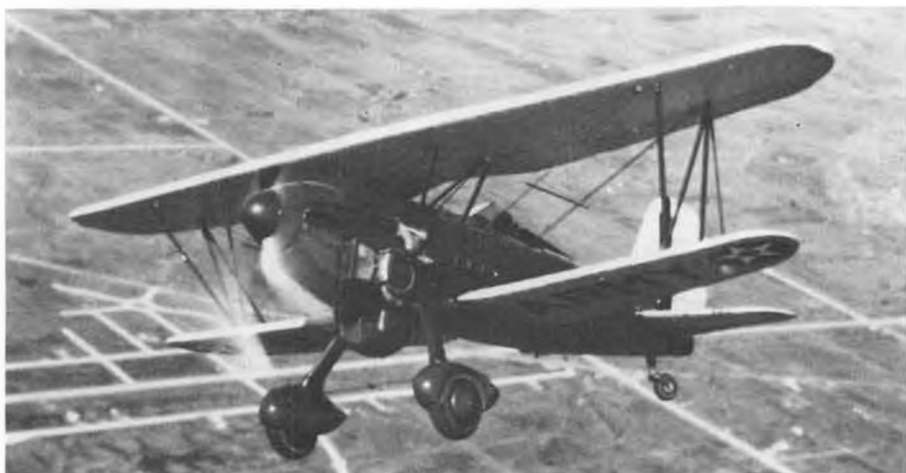
The XP-23 in flight. Rare shot shows all wheels extended, with cuffs on main gear streamlines faired with gear legs. (USAF Museum)
