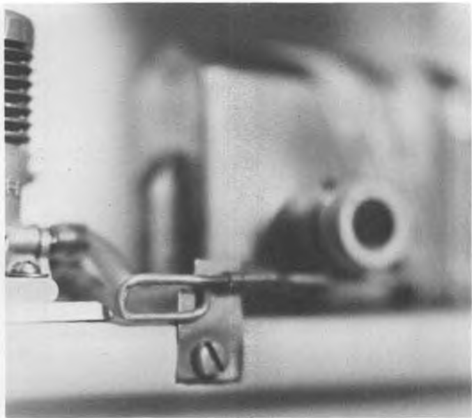
Forward end of the actuating rod, made from a Du-Bro 30 inch clevis rod.
