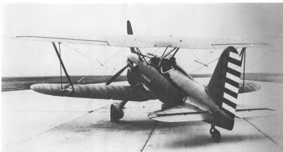
Fuselage and tail surfaces were all-metal and completely new design. The tail was later used on the XP-31 Swift.
