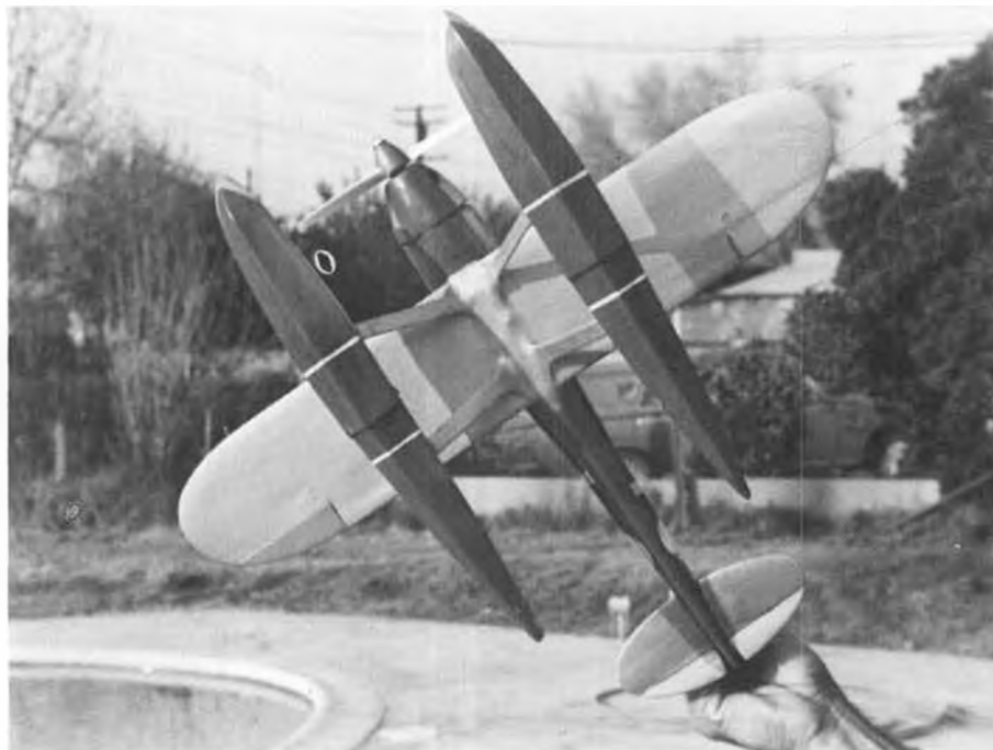
Hand discloses the compact size of this .049 powered model. Author uses an McCoy Red Head diesel to power the model shown.
