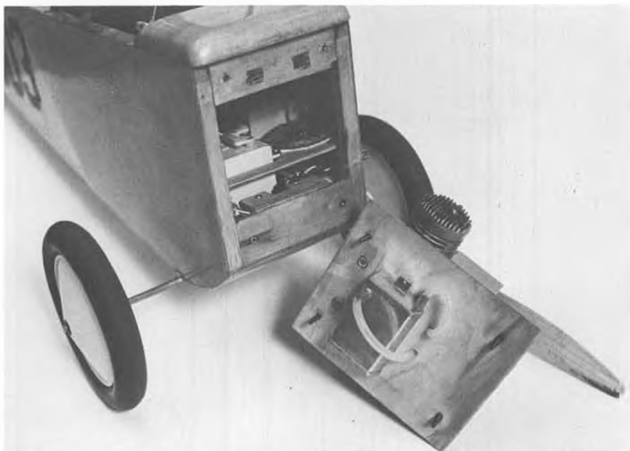
Super-sanitary tank and equipment installation. Note ballast servo-taped to mounting board. Externally operated switch in front. One ounce tank gives 6 minutes. No throttle used.
