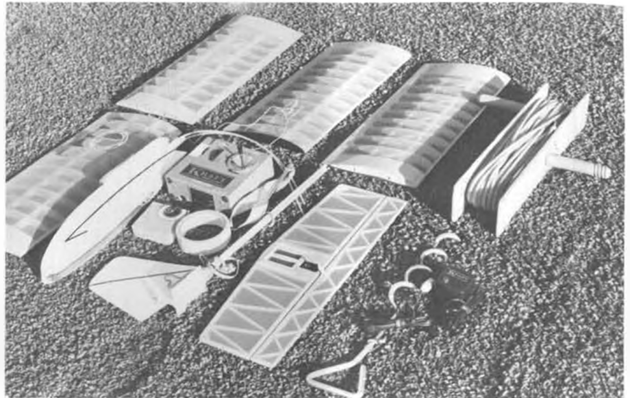
For the complete R/C soarer! Glider, transmitter, hi-start, anchor, charger, timer, and a roll of masking tape for joining panels. All of it goes in the travel box.
