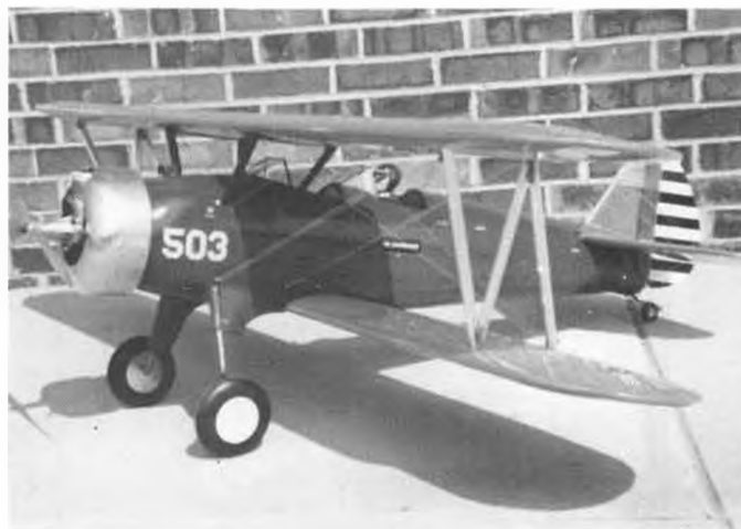
Sterling Models PT-17 by Bill Rushbrook, Lisle, Illinois. ST .71RV with throttle, 14x6 prop, 8 1/2 lbs, flies on 70 foot lines.
