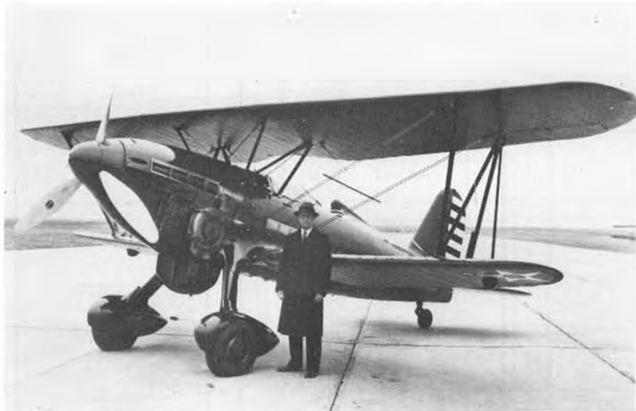
The XP-23 was the last of the 46 famous P-6E's, though only the wings remained. The rest was all new. Note clockwise rotation of prop. (USAF Museum)
