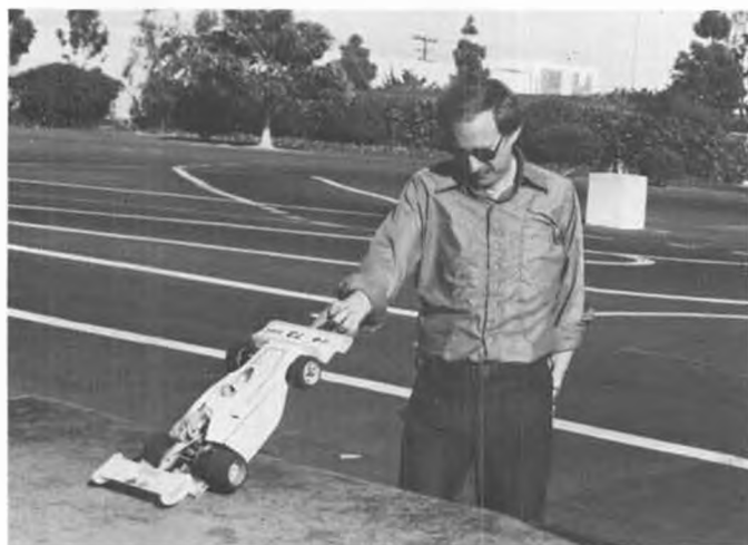
Chuck Hallum displays the visual, or "eyeball" method of checking for uniform tire contact. Line up your eye with plane of tire contact.
