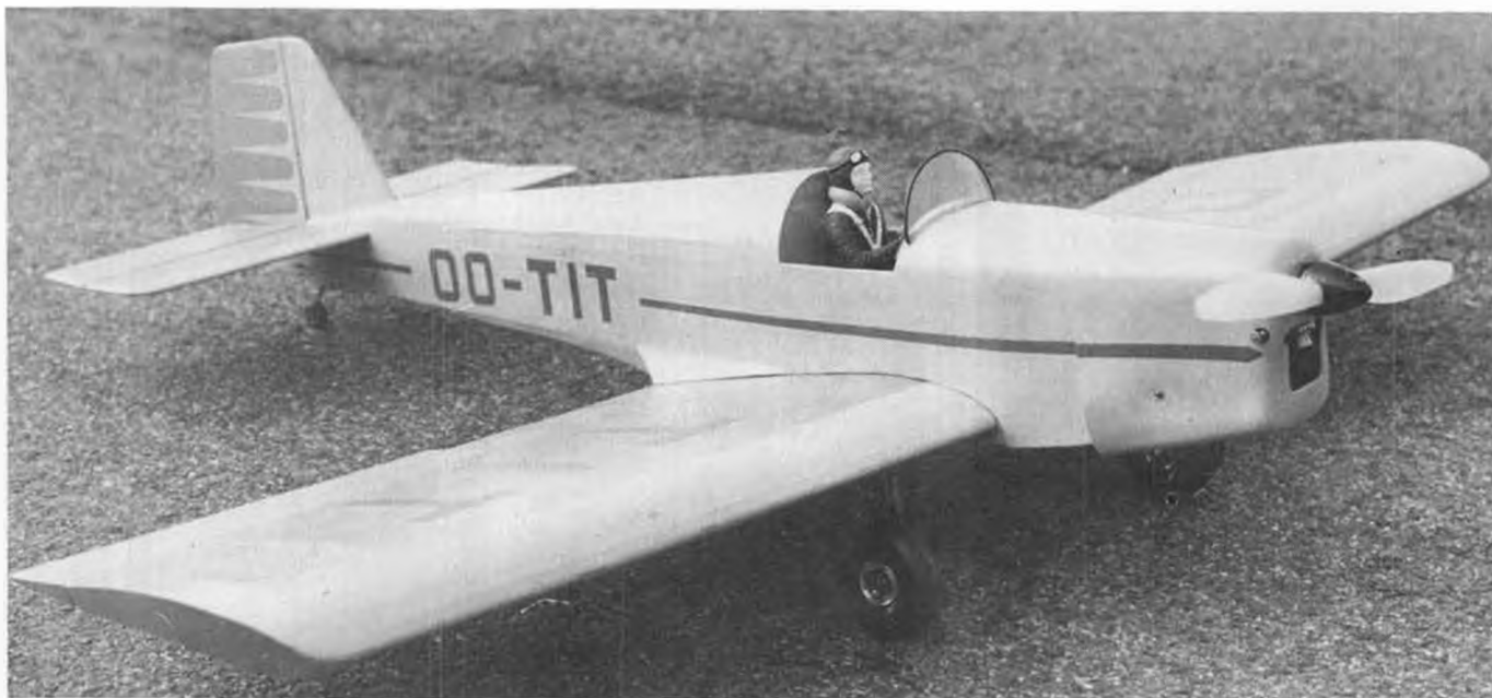
Topsy Junior, built by Mike Proctor, York, England. Ship spans 54 inches, power is an OS .40, radio is 4-channel Skyleader, weight is 4-1/2 lbs. Built from 'Complete-A-Pac' Plan. Photo by Jim Moseley.
