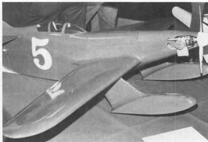
Our C/L mogul, "Dirty Dan" Rutherford, took this photo of Jerry Holcomb's unusual float plane. Note flying/water rudder.
