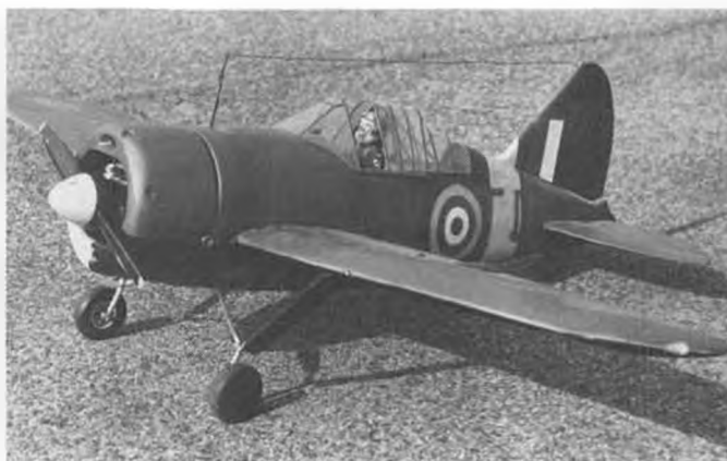
Peter Redman's Brewster "Buffalo" is scratch built, scaled from Profile book. Homebuilt retracts, 52 inch span. Moseley photo.
