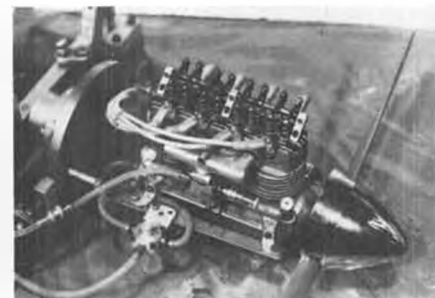
Ignition version of the four cylinder D&B engine, 1.5 cu. in., 4-stroke, runs well.
