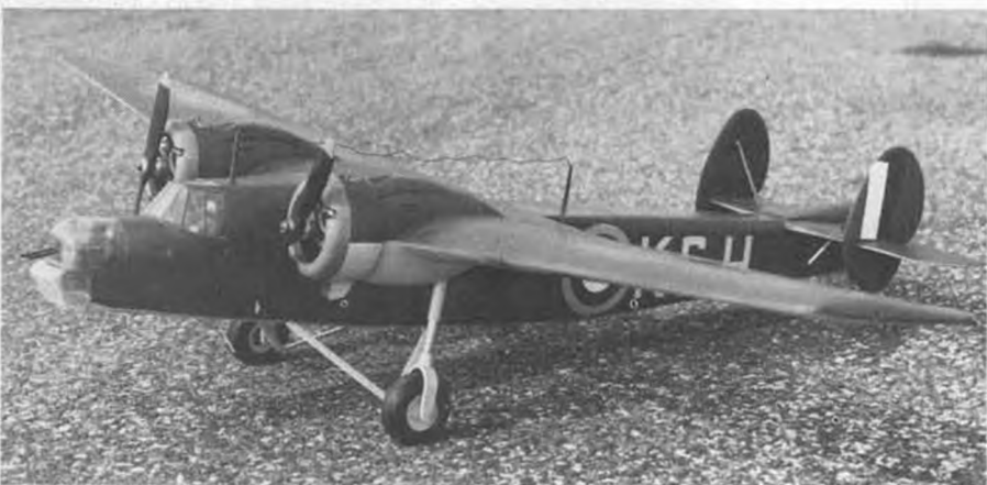
Another Peter Redman scratch-built, a 73 inch span Bristol "Bombay". The 9 lb. ship is a "floater" on two Enya .29 BB engines. Foam cored wing, flat dope over K&B resin. Moseley pic.
