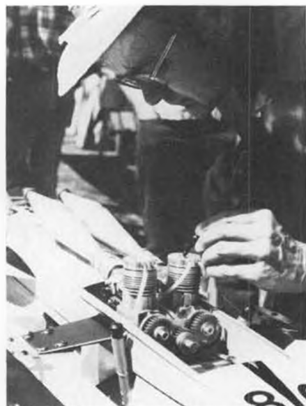
Close-up of the twin, alternate firing OPS 60's in Whitlach's record breaker.
