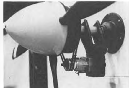
Four-to-one belt reduction drive by Midwest Industries uses friction rather than tooth drive.
