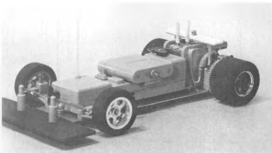
Completely stock MRP chassis, except as mentioned in text. Note center-mounted tank, aluminum pan chassis, unbreakable "A" arm spindles on front, and Racin' Rubber all the way 'round.
