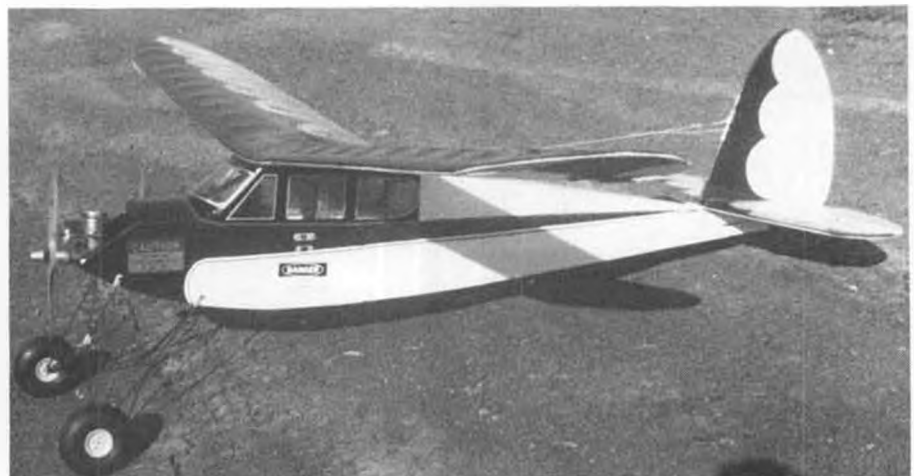
Leo's current Quaker, built from an M&P kit, Merco .49, Kraft radio, and Monokote covering. Trap door in fuselage opens and closes, permitting parachute drops, leaflets, etc.
