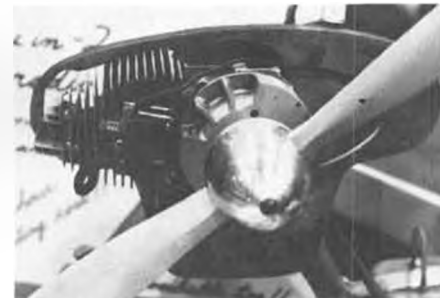
Canadian Quadra engine uses 20-1 gas and oil, magneto ignition, no radio interference.
