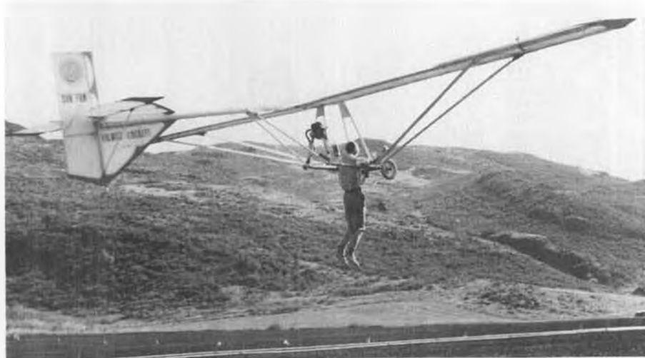
Climbing steadily, the pilot has still not "retracted" the main gear. Engine develops 10 H.P. at 7200 rpm, and burns only 1-1/2 gallons-per-hour of fuel!
