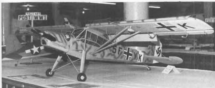
Super Mammoth Fieseler Storch by George Bussman, Seneca, N.Y. Span is 133 inches, weight is 28-1/2 pounds, and it's Quadra powered. Fuselage is built up of welded steel tubing.
