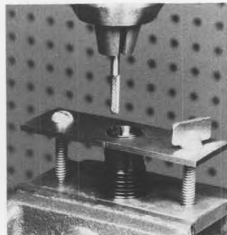
The cylinder held in a milling machine fixture, ready for remachining of the bypasses.
