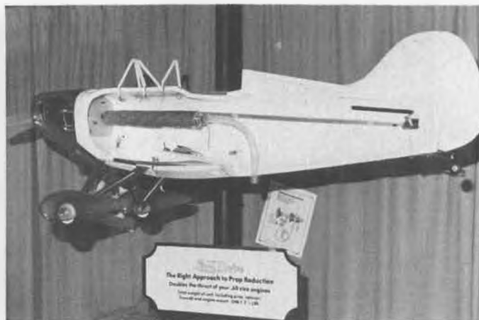
Cut-away display of the Byron Originals all-foam, 1/3-scale Pitts S-1A, showing interior pipe mounting and exhaust system.
