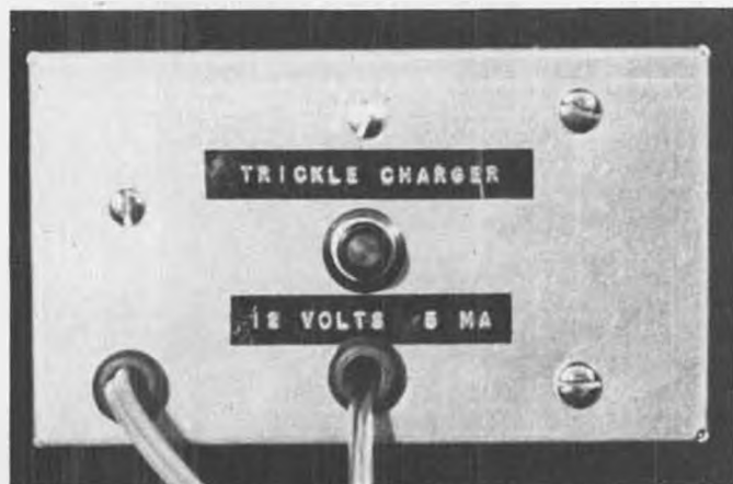
Front and back views of the trickle charger. This example was built without an on-off switch, which could be installed next to the light in the center. Note grommets used to protect A-C cord and battery leads, and piece of cardboard under the transformer to prevent shorts.
