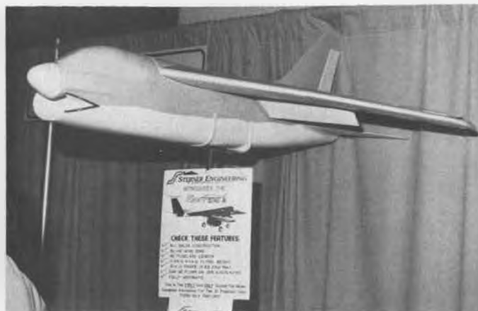
Stern Engineering, Bath, Pennsylvania, will have this A-7 Corsair kit available in June. Uses Turb-Ax 1 fan, includes main retracts.
