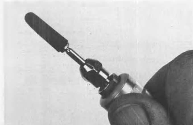
A Cratex Rubberized Abrasive in a Dremel Moto-Flex tool. It's used to "ease" the port edges to reduce power losses.
