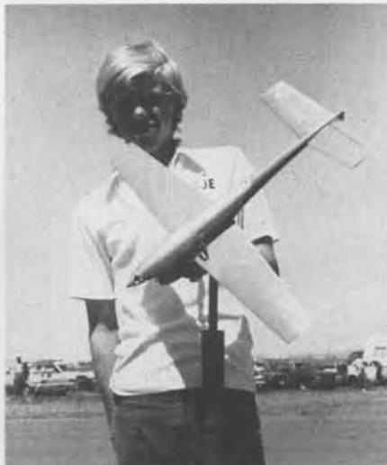
Joe Kall and his record-holding Formula 40. Inverted K&B .40 and half-pan construction.
