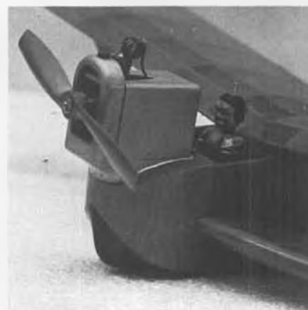
Closeup of the nose on the Dornier. Note how the tank filler is hidden in the pilot's head.
