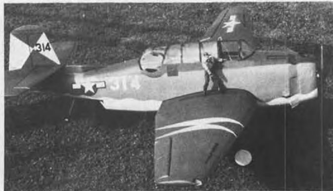
Before and after covering shots of Jim Urozik's 7-foot TBF Avenger, powered by Fox .78 and controlled by a 4-channel Heathkit. Model has a flat-bottom airfoil for high lift and slow speeds, weighs 15 lbs. Looks like GI Joe is gonna need a ladder to climb into that cockpit, Jim.
