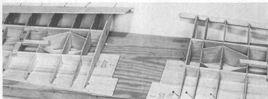
Starting to glue the wing sheeting in place. Wings are built upside down.
