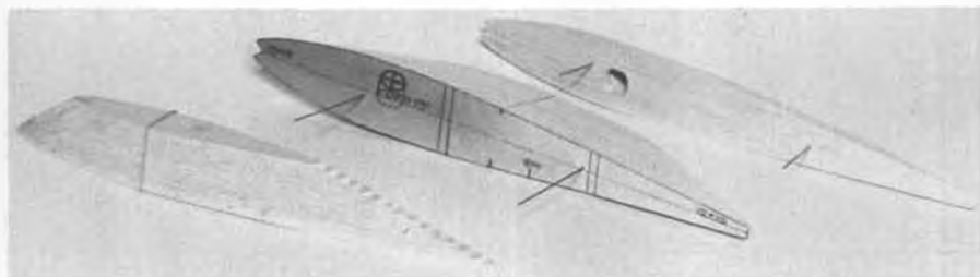
Finished wing ribs. As shown by the batch in the middle, rib blanks are stacked and pinned between plywood root and tip rib templates, then carved and sanded to shape.
