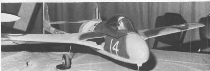
Experimental British Vampire jet, designed and built by Nick Zioli to test Midwest ducted-fan unit. Features easy access to engine and fan compartment.
