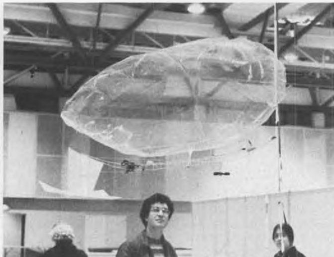
Tony Avak flew this R/C blimp at the Pasadena IMS Show for 1 hour, 40 minutes before running out of releasable ballast (BB's), thus ending the flight. The motor was mounted on a pivot and turned with the rudder, enabling it to turn in its own length.
