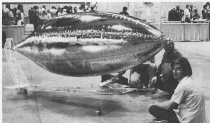
Bill Watson's was easily the most advanced airship at the Pasadena IMS Show. Like Tony Avak, Bill ran out of ballast (water), not power, so he had to bring it down. Distance covered was some 7.6 miles. Motor is mounted in rudder, providing excellent directional control.
