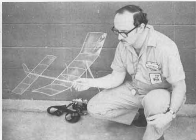
Buddy Tenny at the Nats with his 1 gram FAI microfilm job. Note the built-up tailboom. Dave Linstrum photo.
