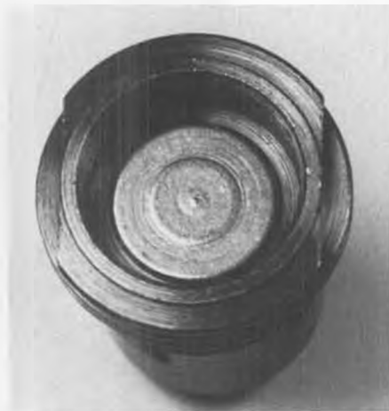
This cylinder/piston set shows the piston at the optimum barely-hold position . . . see text.
