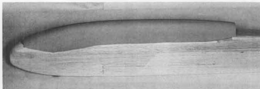
First step in making the canopy/pipe cover is to carve a balsa or expanded polyurethane block to the desired shape, as shown above. This will be used to make a female mould.
