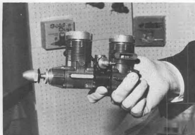
What a brute! This is the in-line HP 120 Gold Cup Powertwin. Alternate firing, single automix carb, 34-1/2 oz. Midwest Model Supply.
