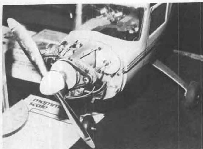
Eastcraft's electric on-board starter is an easy fit in this .60 powered Cessna. System adapts to all large engines, including Quadra.
