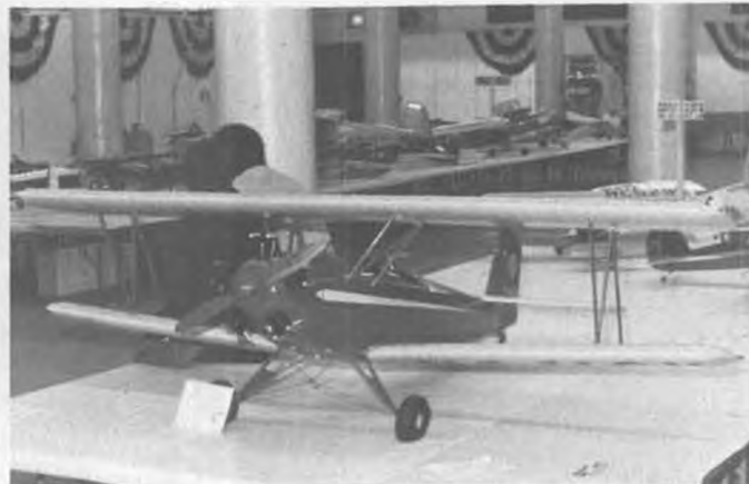
Bob Pickney, Whitesboro, N.Y., built this 1/3-scale 1930 Fleet. Ship weighs 22-3/4 lbs., span is 98", and power is a Profi with prop drive.
