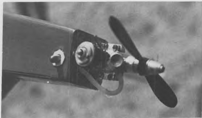
Interesting toggle switch system for turning the bladder pressure on and off, seen on a 1/2A pylon racer.
