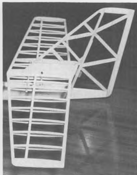
The Osprey's light, rigid tail structure. Like most original designs, it shows traces of its ancestry . . . in this case, the Windfree.
