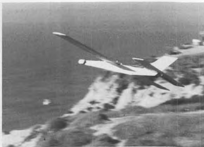
Steve's creation in flight. Uses aileron and elevator controls, balsa slab profile fuselage. Most took 2 or 3 hours to build.
