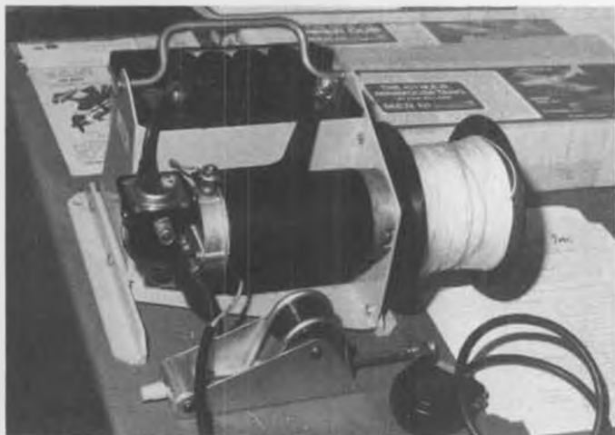
Lightweight glider winch for up to 80 oz. birds uses Sears tractor battery, available separately. From Fab-Tek. See text for info.
