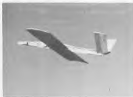
Scotty's zip-zip ship in flight. Note undercamber in wing.
