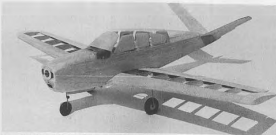
House of Balsa makes some of the neatest 1/2A R/C kits around. Shown here is the Beechcraft Bonanza, for .049 to .10 size engines and 2 to 4 channel radios. A good subject for Stand-Off Scale.
