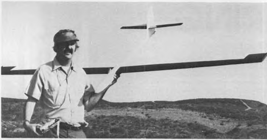
Ken Raymond is also into the design of F3B competition sailplanes, shown here with his original design 100-incher. Uses coupled ailerons and rudder, Futaba radio.
