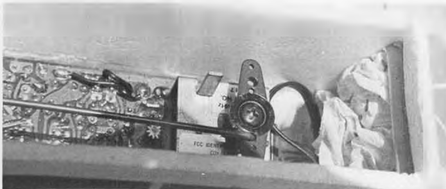
To get the least amount of rudder travel, insert the pushrod wire in the innermost hole in the servo arm and the outermost hole in the rudder horn.
