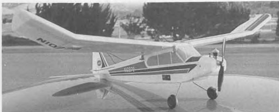
Most obvious change, of course, is the addition of polyhedral to the wing tips. This is the biggest single factor in increasing the model's stability.
