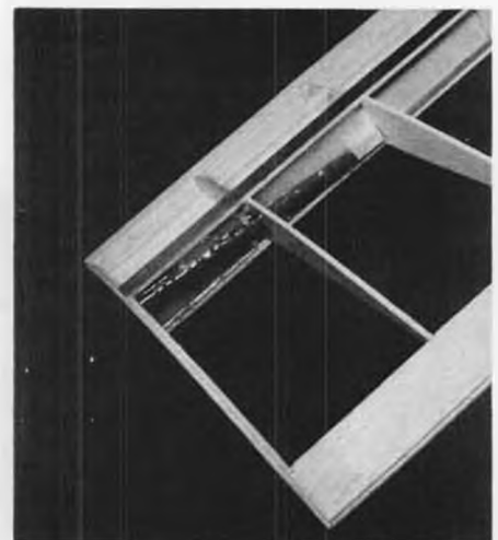
Fiberglass tube is fastened into the wing root with epoxy, and lots of it. Note 1/4-sq. plug at end of tube.
