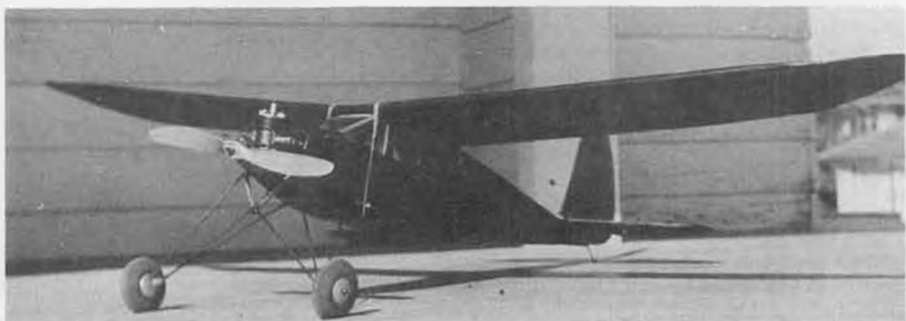
Photo No. 8 W.W. Wilson sent this photo of his Flying Quaker, complete with GHQ engine, built in 1937. Heavy aluminum prop acted as a flywheel, necessary for the engine to run at all.
