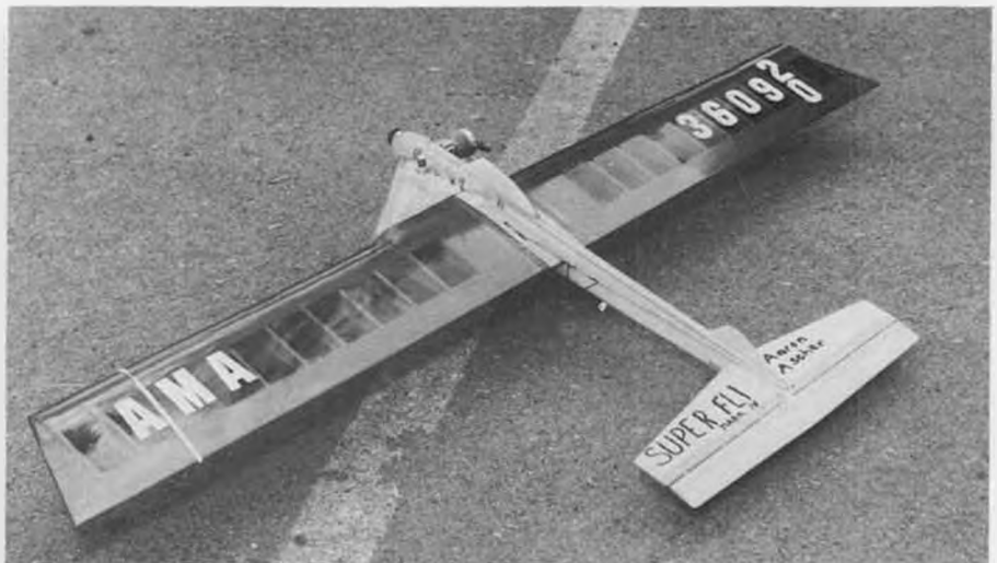
Dave Braun calls his racer the "Super Fli"; looks like it would make Combat types at home in the racing circles. Uses O.S. .36 with Nashville type tank/filler assembly.
