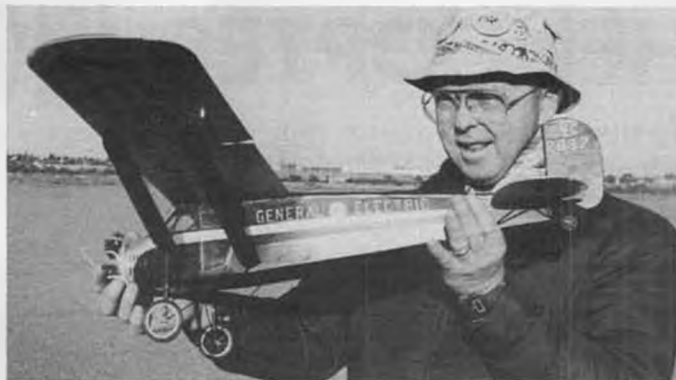
Bill Stroman and his Stinson Jr. for F/F Scale. Astro 020, 234 sq. in., weighs about 10 oz.
