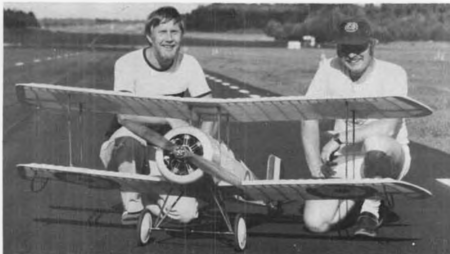
Sten Dal (left) and Greger Martenson with their 1/4-scale Bristol Scout. That's not a dummy engine in that aluminum cowl, but a seven-cylinder Damo radial!
