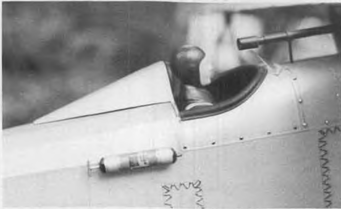
The author put considerable time into the detailing of his Hawk, as these photos show. Monokote covering was used throughout, then the model was given two coats of clear epoxy paint as a sealer. Text tells how to make Monokote look incredibly like a fabric covering.
