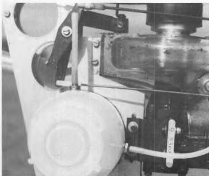
Tank has to have an extra vent and also a clunk pick-up for inverted flight. If the engine quits when you're upside down. . .
