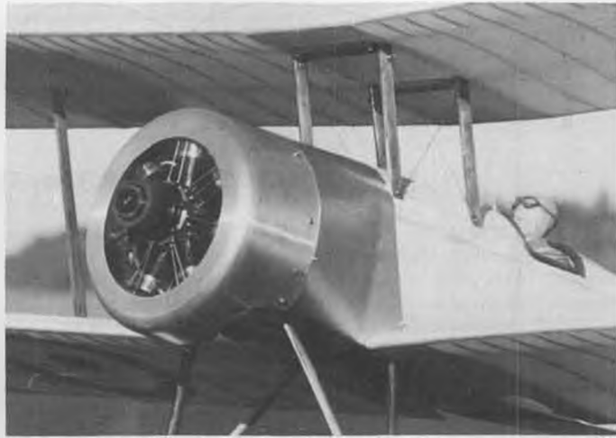
Yes, it do run, and very smoothly, too. Swings a 24x8 prop at just under 7000 rpm. Plenty of power for the Scout.
