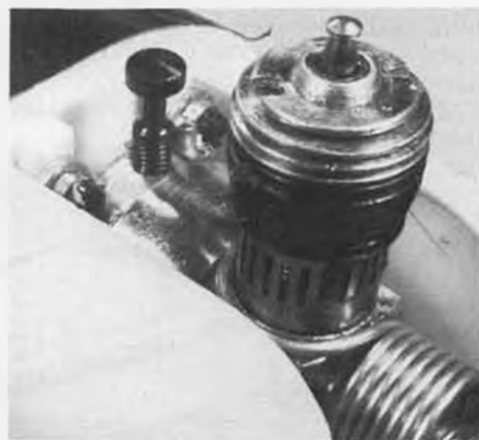
A little downthrust helps too, and is added by inserting a couple of thin washers between the engine and mount.
