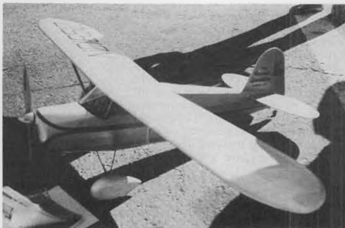
Bob Sliff's Rearwin Speedster was built from an old Cleveland plan, spans 64 inches. Astro 15 with belt drive.
