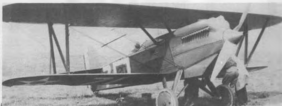
XPW-8A borrowed the tunnel radiator design, had thicker, shorter wings with a single bay of struts. Aircraft was still less maneuverable than the PW-9.
