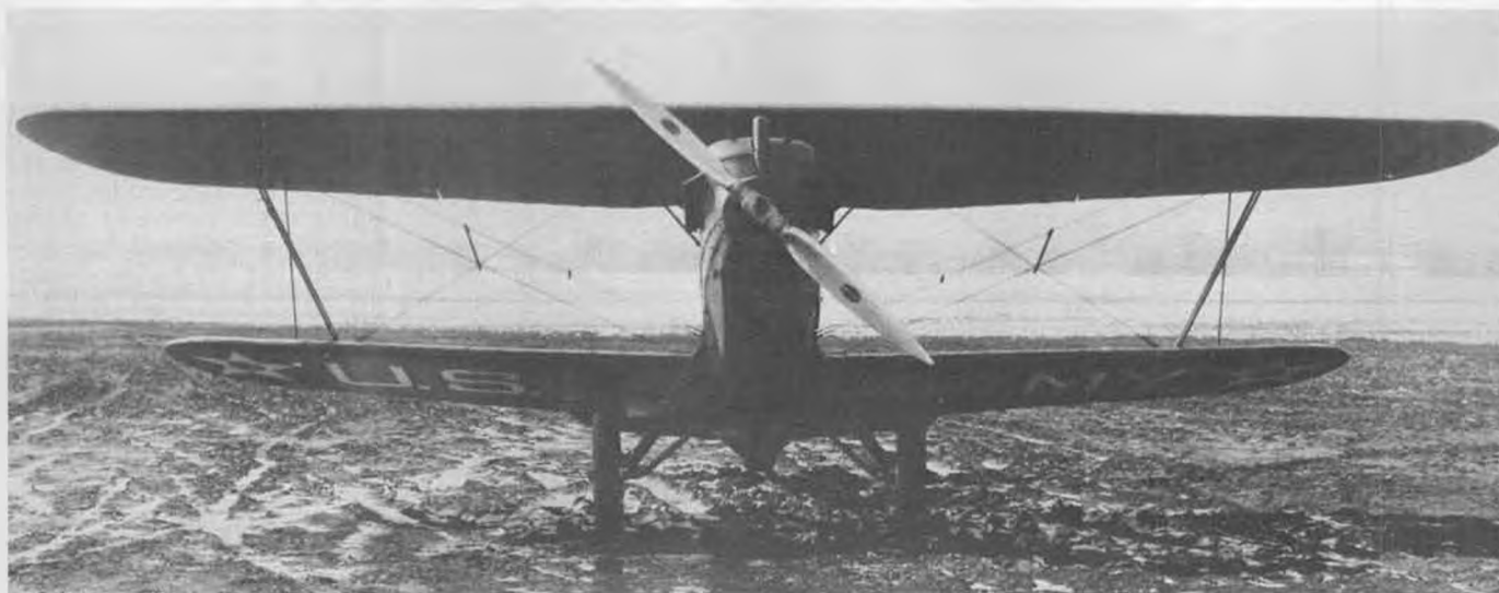
Head-on shot of the original P-1B tested by McCook officials in 1927. Tapered wings show up well, as does the experimental Hamilton Standard adjustable blade prop. Color is khaki overall with aluminum wheel discs.
