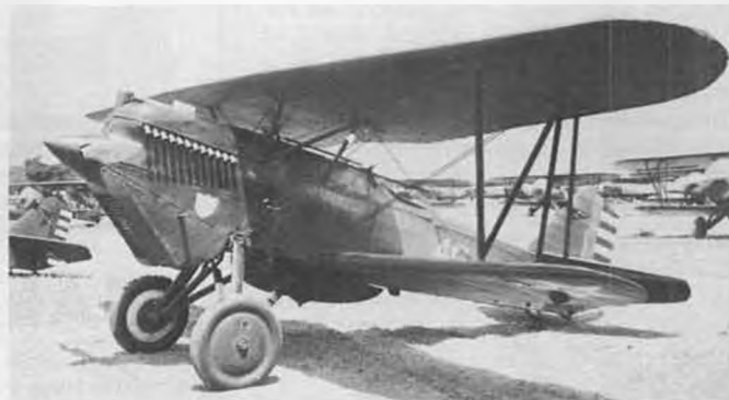
This is a Curtiss P-1C, easily recognizable because it was the only Hawk without a headrest.
