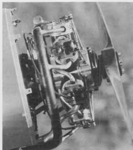
Plugs are fired by a magneto, apparently contained inside the radial engine mount.
