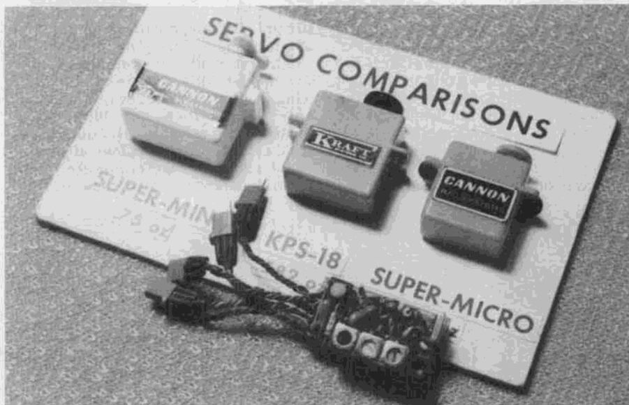
The shrinking size of servos is graphically illustrated by this display showing the old Cannon Super-Mini, Kraft KPS-18, and Cannon Super-Micro. New Cannon Rx in foreground.
