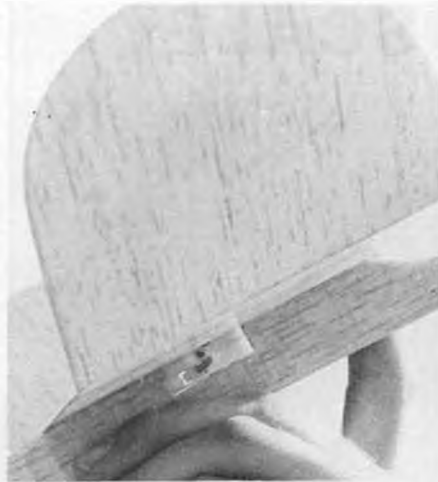
Dale Segle took a lightweight clockwork mechanism from a bathtub toy and made it into a DT timer for HLG's. Photo on right shows how it mounts into the fuselage, left photo shows DT line, release mechanism. Shaft made by soldering brass discs to brass tube, a la Seelig.
