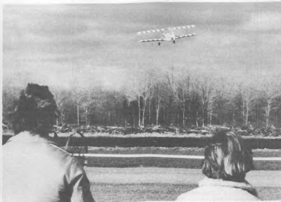
"Jersey" Jim Martin, former U.S. FAI R/C Aerobatic team member (1973) makes first test hop of the Executive Engines (now Technopower) 7-cylinder radial in a 12-1/2 lb. biplane.
