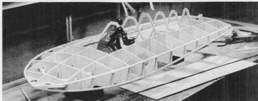
A White Heat hydro under construction. Certainly appears to have sufficient structural strength! An O&R Compact industrial engine (1.3 cu. in.) was used.
