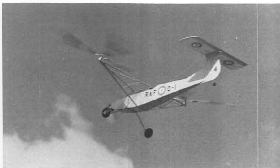
Yes, it do fly! Skip's new tail-dragger autogyro cruises overhead. Throttle sorta controls altitude; elevator changes attitude, slowing or speeding up forward motion.
