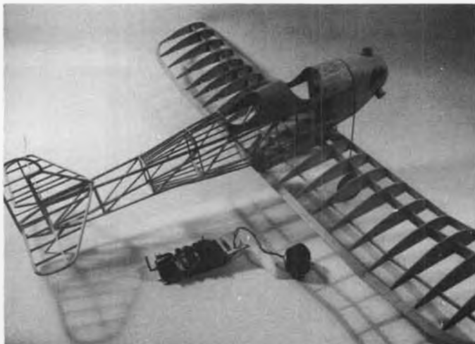
Framework shot of Hurst Bowers' NB-3 shown above. Receiver and actuator are on single board for easy removal.
