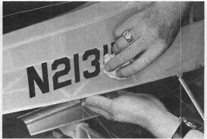
Once in position, remove moisture from under decal or sticky mylar using absorbent material; stroke from center outward, forcing out air bubbles.
