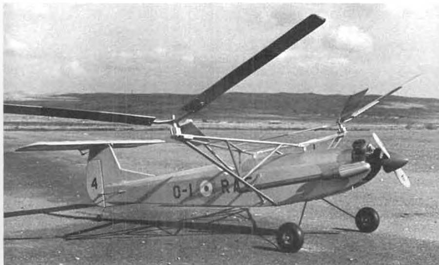
Going to a tail-dragger landing gear provides a higher angle of attack for the rotors, gets them twirling earlier in the takeoff run.
