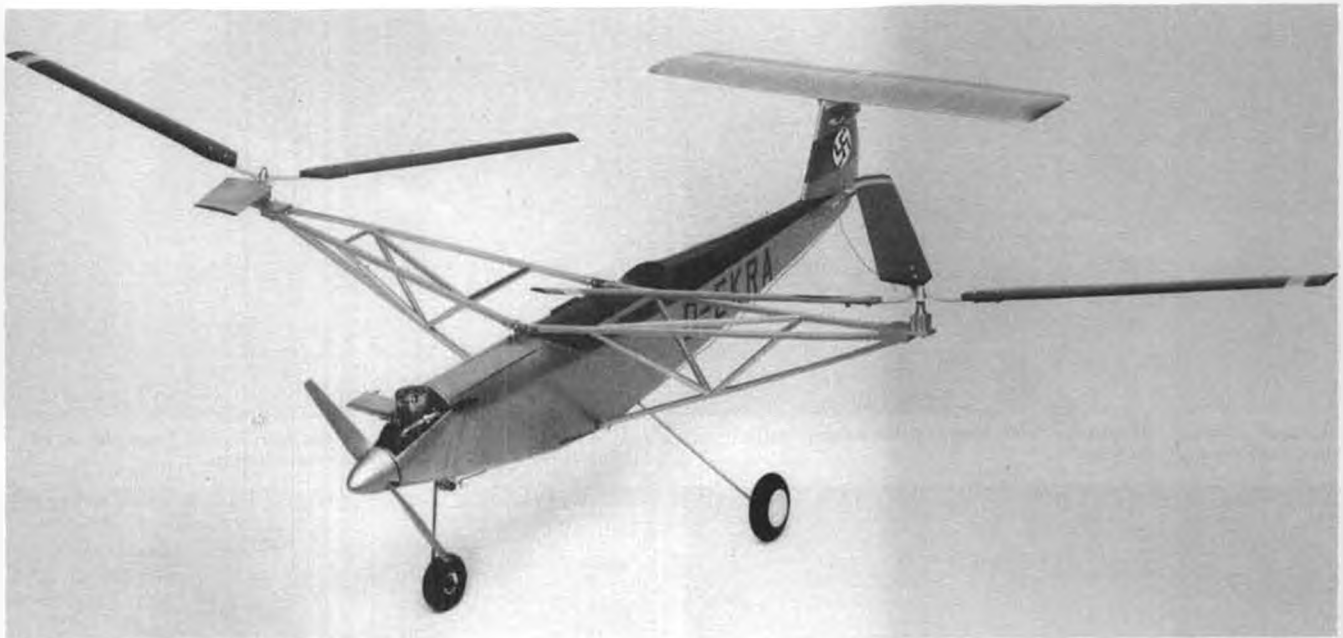
Nicely built version of Skip Ruff's Focke-Achgelis FA-61 twin-rotor autogyro (MB plan No. 4751) by Sten Persson, of Sweden. Original aircraft actually a helicopter. Cut-down prop was only for cooling front-mounted engine which drove rotors by shaft and gear transmissions.
