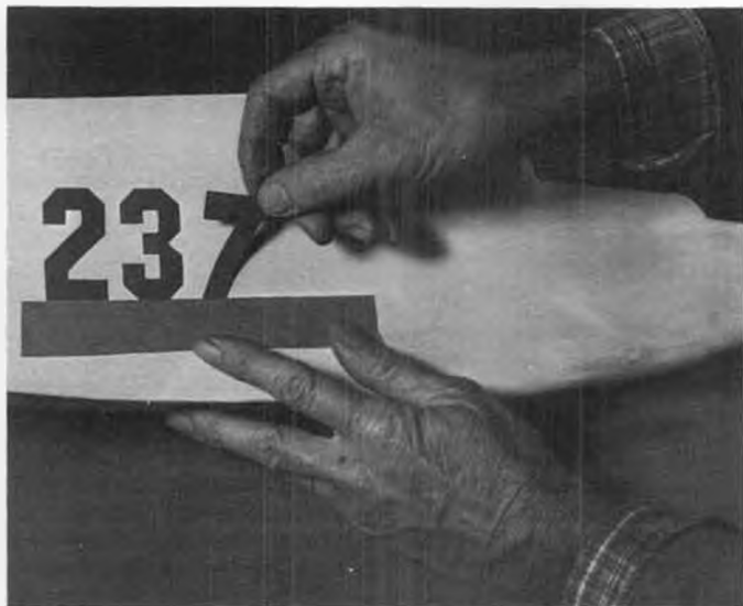
Masking tape is a good guide for positioning stick-on markings. Won't work for decals because of overlapping clear material on decal. Same problem with removing guide lines.
