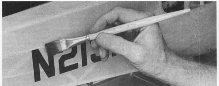
Protect decals and stick-ons from fuel with a clear coating. Polyurathene varnish is a good coating for most materials. Whatever is used, it must not dissolve marking, but also must stick to the marking material. Check before using.
