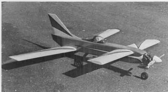
Interesting canard design by Skip Ruff (He sure enjoys staying out of the rut!) is based on Ace foam wings, is extremely stable and easy to fly. Construction article coming.
