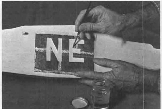
Seal stencil edges with clear sealer which is compatible with finish paint. Clear finish may bleed under stencil, but won't show. Color will then not be able to bleed, causing fuzzies.
