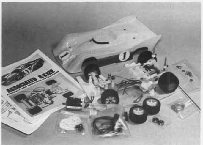
Associated Team Nats car; chassis shown in close-up and in "Group" shot with the total kit contents. Again, see text for more information (STFMI).
