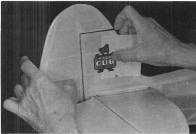
Apply decals and stick-back mylar in similar manner. Decals slip off paper backing after soaking. Sticky mylar is slid into position on detergent/water mix.
