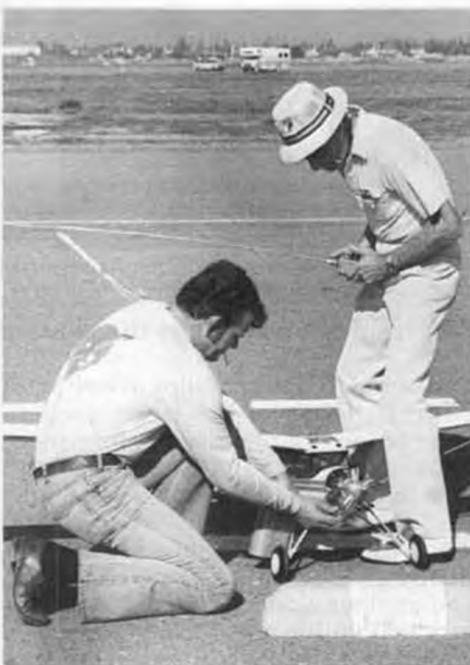
Roger Simpson fires up bottom plugs while Don braces model. Plugs can foul from long idles, need on-board battery to cut in at about half throttle, maybe just for bottom two.
