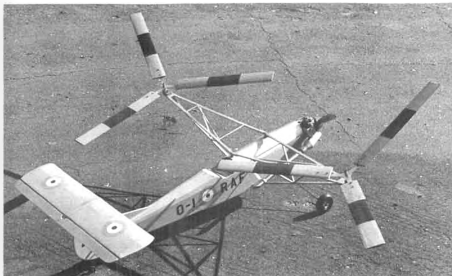
This is Skip's latest version of his original design, powered by a K & B 40 and with constant 2-inch chord rotors.
