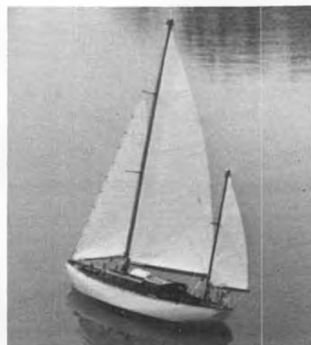
Bill Head scratch built this 30-inch L.O.A. yawl "Dream On" to 3/4-inch scale. Has 6-volt electric auxiliary, sails by Chuck Black, Futaba R/C.
