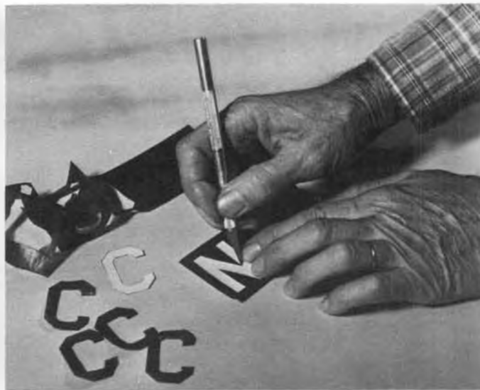
Tissue letters can be multiple cut by folding tissue accordion style, then cutting through several thicknesses. Saves time if you're building three planes at once!
