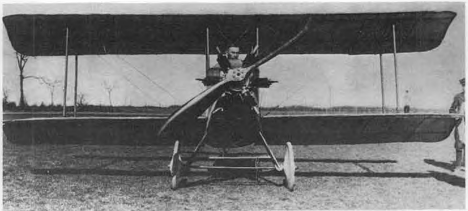
Photo like this really facilitates making of 3-view. Niemo Black in cockpit. Note clockwise (from front) prop rotation, 6-cylinder Anzani radial engine.
