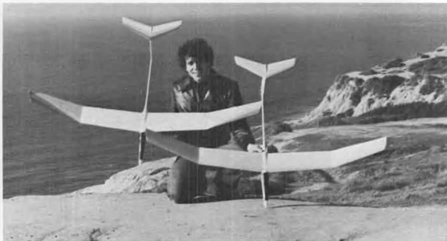
Bob Williams with two of his Shrikes at Torrey Pines. Wings are polyhedral and swept, with extremely thin airfoil.
