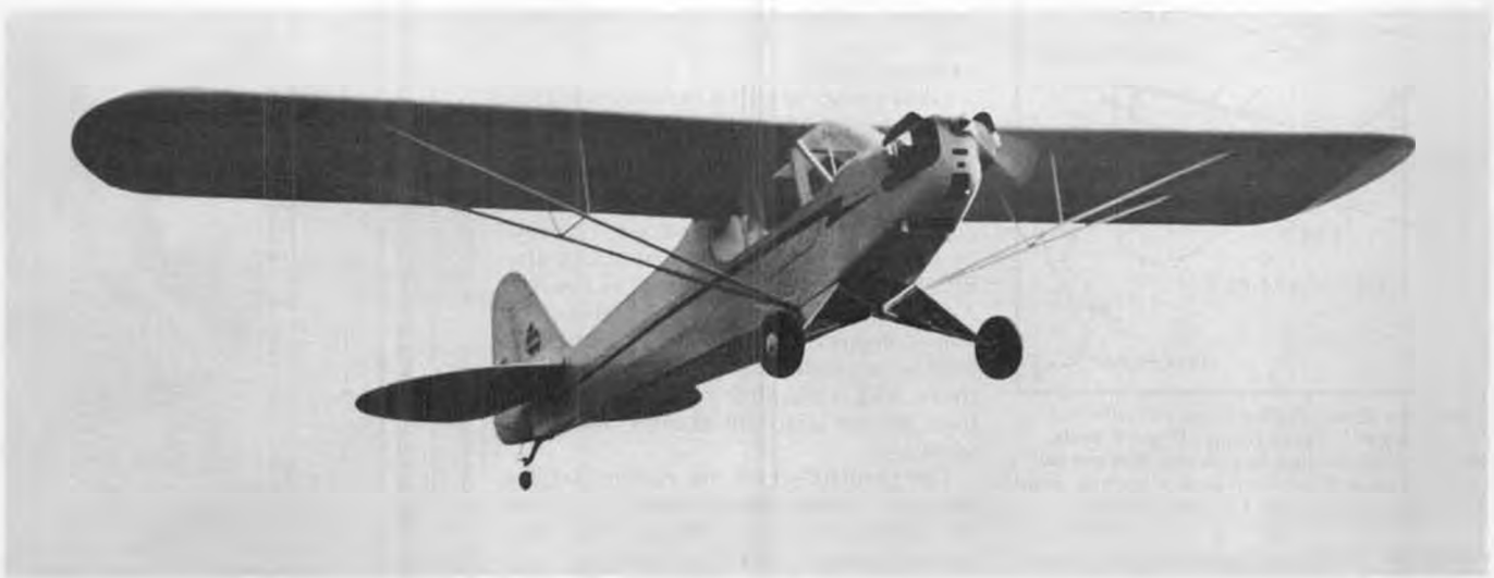
Prototype of new Sig 1/4-scale J-3 Cub, built by Ken Breiting, Malcom, Iowa. Powered by Webra 60 speed at this time. Weighed 15 pounds at takeoff. Alman's Sig clipped-wing version will be tested with methanol and diesel engines for comparison, for coming product review.
