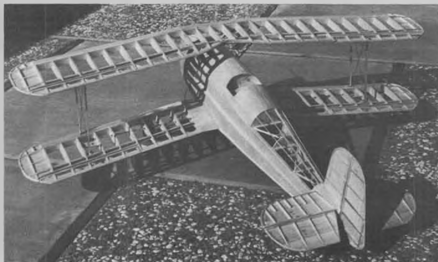
Balsa and spruce are used throughout the construction. Only modification is removal of dihedral from both wings to improve rolling and knife-edge symmetry.
