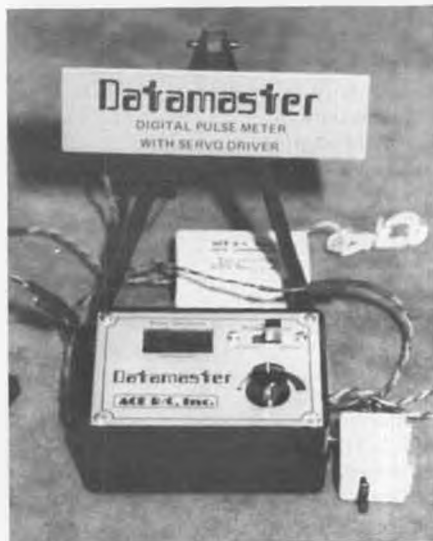
Ace R/C's Datamaster is combination Digital Pulse Meter and Servo Driver . . . in addition to other capabilities.
