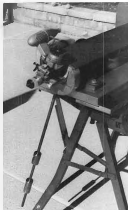
The Fox Eagle III .60 R/C engine swings the pendulum weight on the author's dynamometer. Torque gauge takes reading later.
