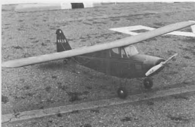
Bob Boucher's Porterfield with Astro 15 on 3:1 reduction drive. About five lbs. total. Astro Flight kit. Placed third in R/C Scale.
