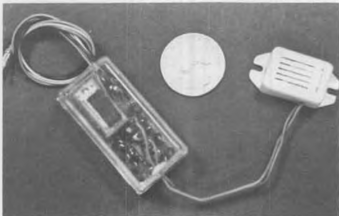
RAM's Battery Backer switches on auxiliary airborne power if primary pack fails. One of many electronic items.
