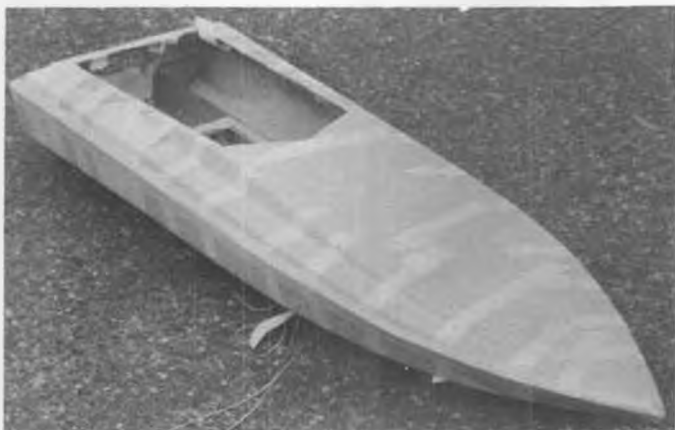
Deck and hull taped together with masking tape, in preparation for joining with glass cloth strip and resin.
