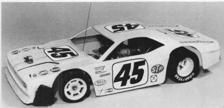
Hot tip for indoor oval racing; Leisure Super Sport chassis, six-cell power, and old JoMac hard-plastic Challenger body. Rail-rider front bumper and tough body make it durable.
