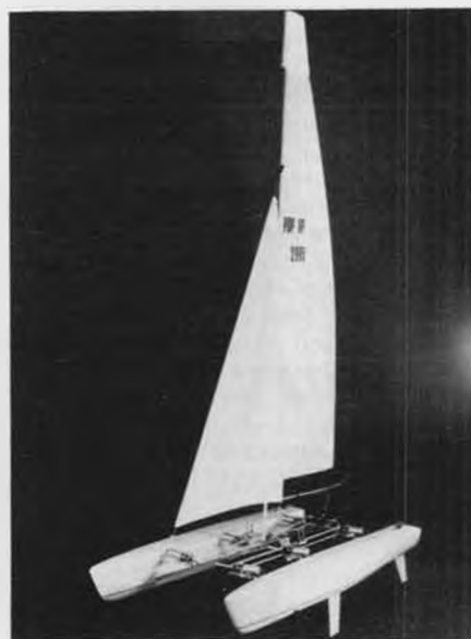
Radio operated self-righting is feature of this catamaran by Pop Up Mfg. Co.
