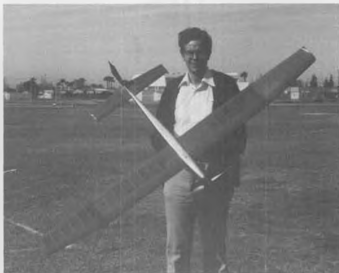
Ken Banks with two-meter original. Leisure 05 racing, eight .60 Ah Sanyos, Carrera 5:1 reduction. Climbs at 45°!
