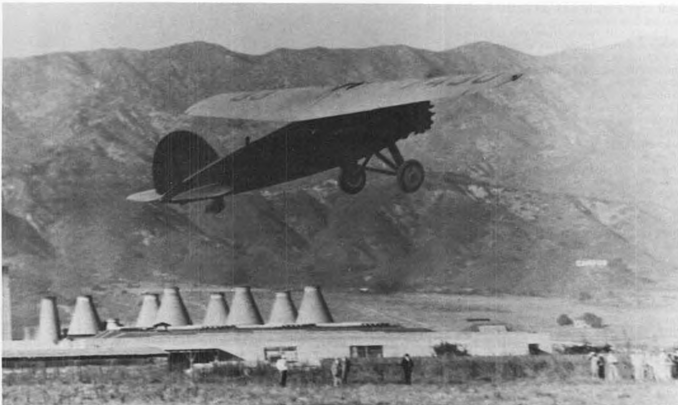
One of the first Lockheed Vegas taking off from dirt strip in Burbank. Empire China Company and Verdugo Hills in background. Note uncowed engine and absence of wheel covers, also clod of dirt on tail wheel.
