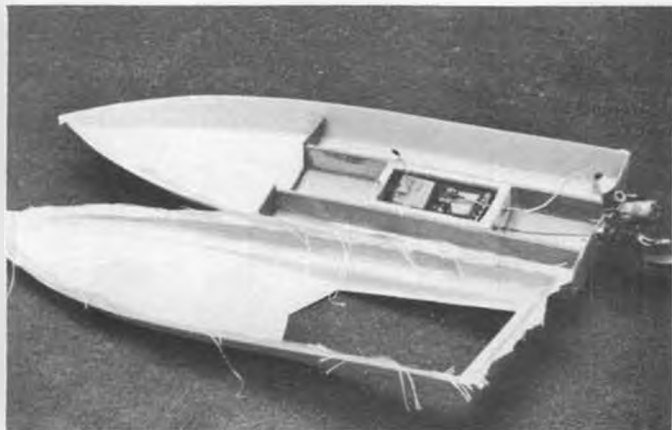
Ready to join deck and hull. Glass cloth strip has been resined to deck first. Radio compartment and linkages finished.
