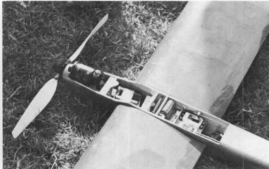
Inside details of Ken Banks' ship. Eight cells right behind motor, motor above gear drive. All is covered by neat one-piece cowling/canopy.
