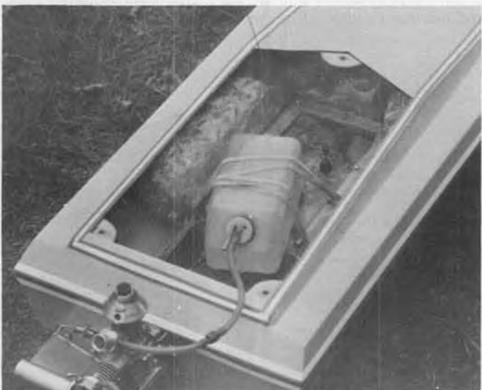
Ready to run, with fuel tank mounted atop radio box. Plastic bubble material stuffed in hull for floatation.
