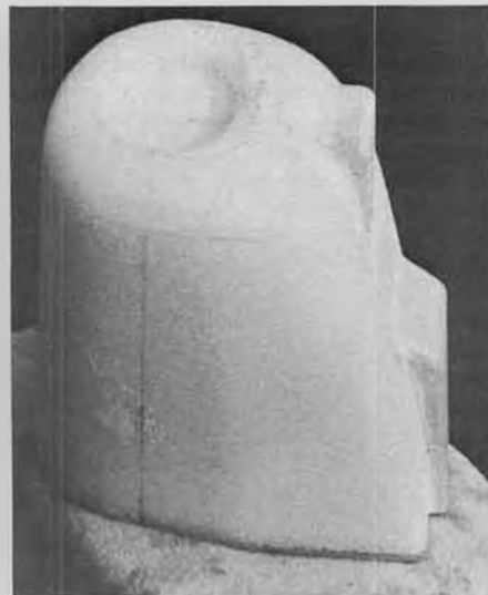
Fiberglass cowl is formed over this carved foam male mold.
