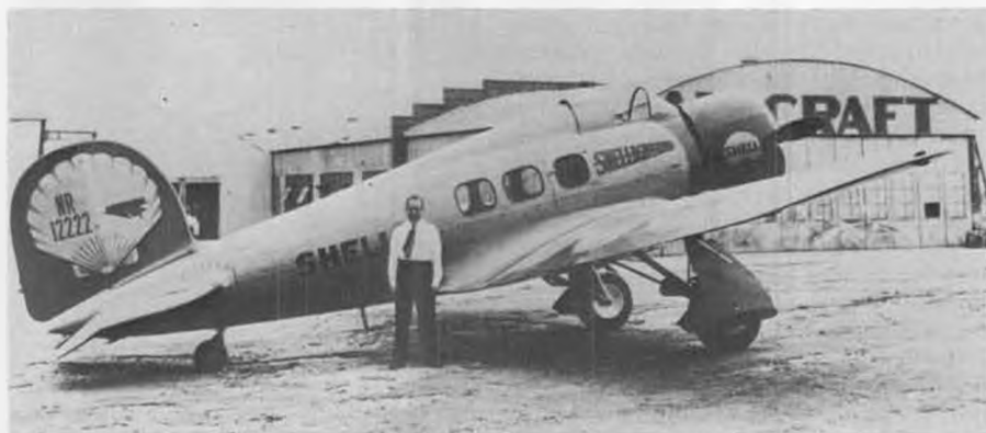
Orion was last of the "Wooden Wonder" series, and most successful since the Vega. Maj. Jimmie Doolittle stands with his "Shelllightning." Orion was only "WW" fitted with flaps.
