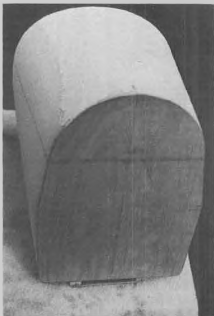
Another view of carved foam cowl mold. Wood bulkhead guides shaping.
