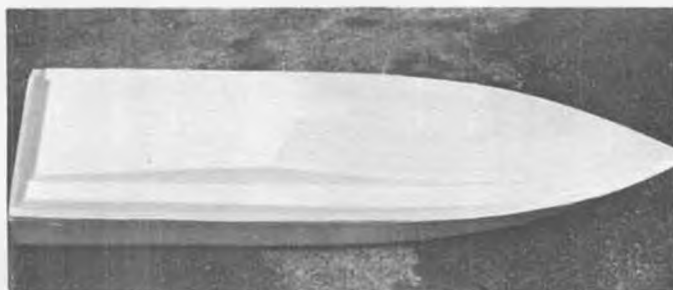
Wardcraft Offshore 33 unjoined, with rear deck still not cut away.
