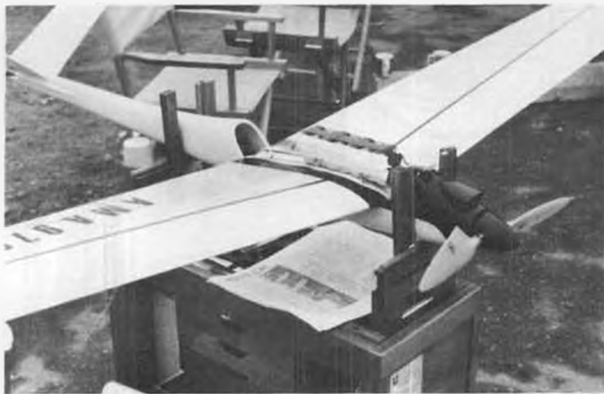
Dave Schadel's Hot River (Geist kit) with Geist samarium cobalt motor, gear reduction, prop. Uses 14 cells. Incredible climb.
