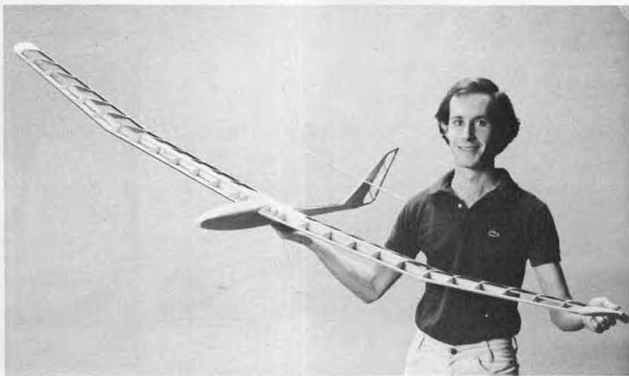
Sailplane beefed-up with cured carbon fiber composites from Twin-K.
