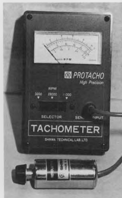
Cannon R/C Systems Protacho tachometer works off of prop or flywheel.
