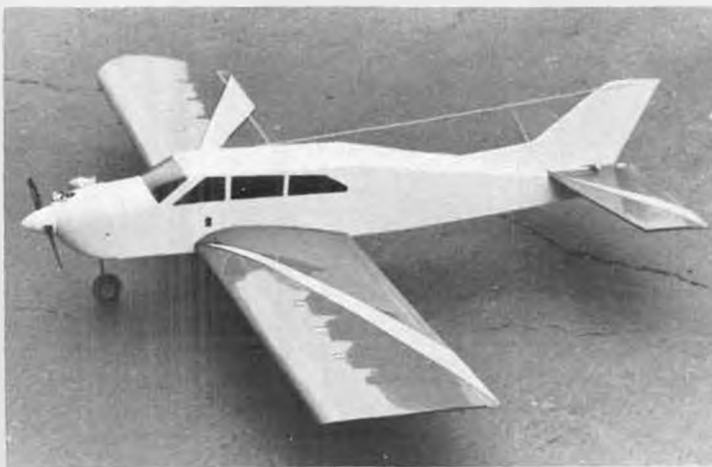
Anthony Cantarella of the Simi Valley (CA) Fliers did this Kadet MKII conversion to a low wing. He changed the dihedral to 1" under each tip, recessed the wing into the fuselage 1/4" from the bottom and mounted the engine at a 45° angle. "The plane flies beautifully."
