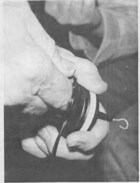
Magnetic sensor/switch inside winder tells H.P. to: "add one . . . add one . . ." etc.
