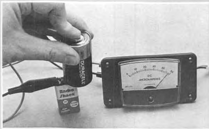
Using a 9-volt and a 1.5-volt battery in series, set the meter to full deflection. Each division is now .030 volts (1.5v/50).
