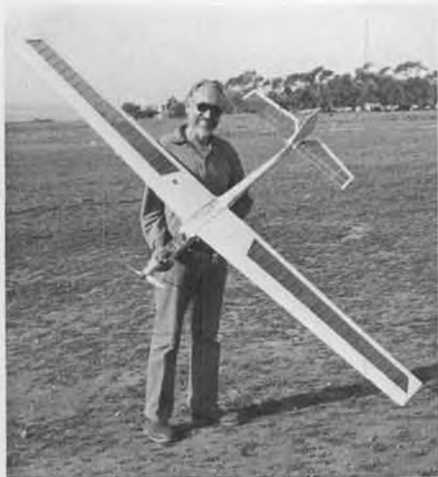
Hans poses with the Carrera Primus, a German-made electric with folding prop, gear reduction, and U-joint drive shaft.
