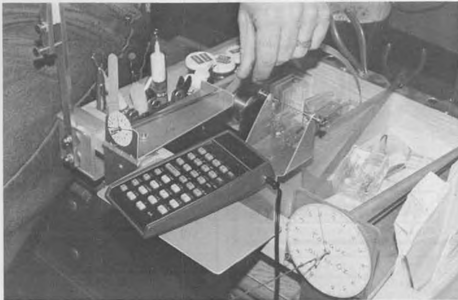
Harry Griffen's technical center for indoor flying . . . the ultimate scientific approach to winding rubber . . . H.P. calculator counts winds, torque meter measures torque.
