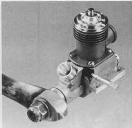
Dave Williams' bar stock .049 will turn over 40,000 rpm with tuned pipe.
