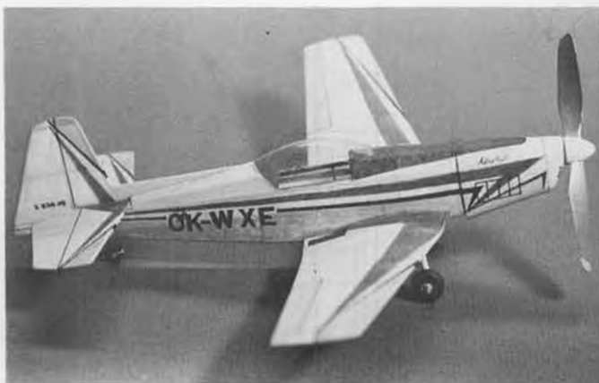
The Zlin 526 AS Akrobat Peanut model pictured here is yellow with red and black trim. The author's method of obtaining the yellow base color is to give the model a light coat of white paint followed by a coat of yellow felt pen ink.
