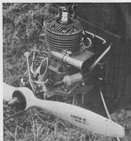
12. This is Henry Struck's classic method of designing a removeable motor mount as recreated by Don Dodds.
