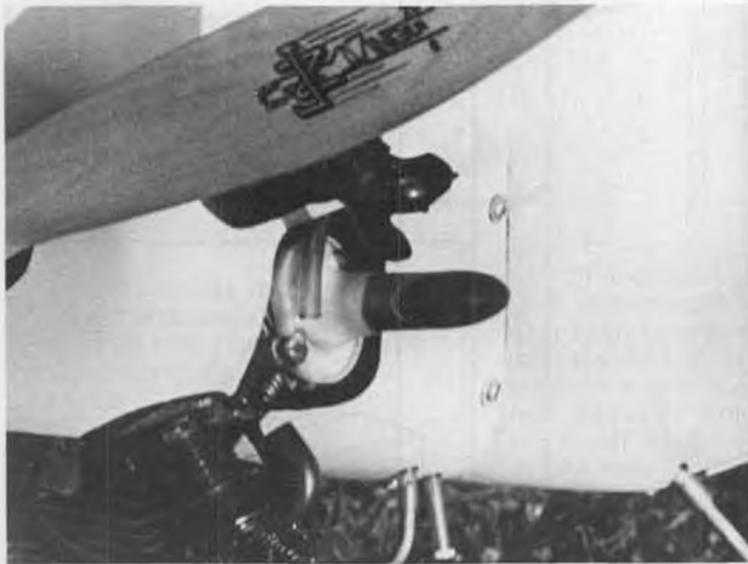
If done right, this "poor man's supercharger" or velocity stack does make a performance difference. (Edwards' Fleet.)
