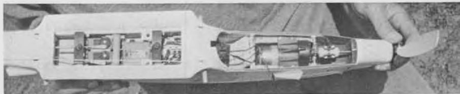
Inside the Carrera Primus lies a clever universal joint between the motor and the folding prop. Carrera motors and other accessories are carried by Wilshire Models.
