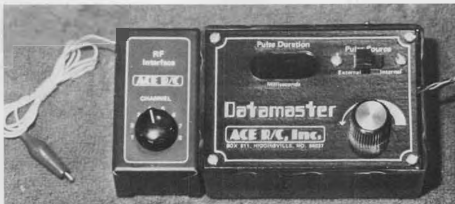
One of the many new electronic devices at the IMS show was this Ace R/C RF Interface unit which attaches to the Ace Datamaster and increases its versatility.
