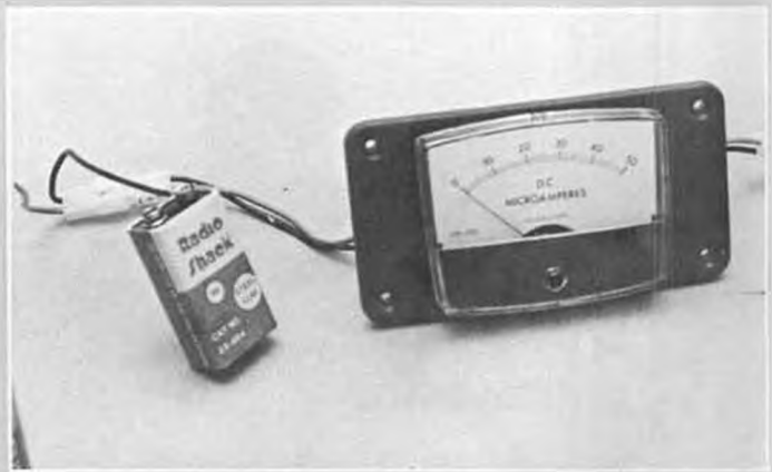
Remove the 1.5-volt battery and check the zero point on the meter. With the 9.1-volt zener diode, needle shouldn't move.
