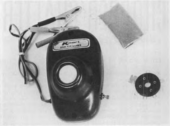
This low-cost K-Mart Spark Plug Cleaner comes complete with bag of abrasive and gap gauge. Other brands are similar.
