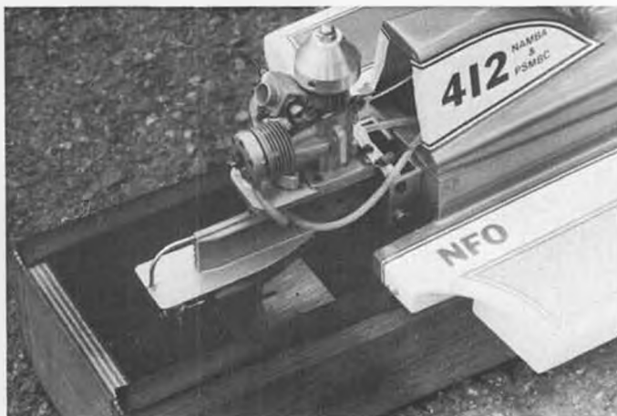
The use of an adjustable motor mount is highly recommended. K&B 7.5 with Octura 447 or 450 prop is good combo.
