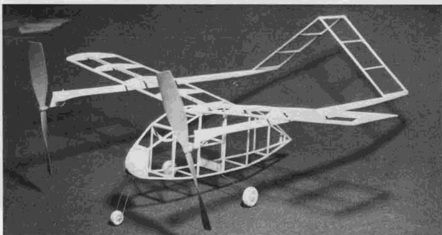
The basic framework is now complete and ready for covering. Sleek Streak props and thrust bearings are used.
