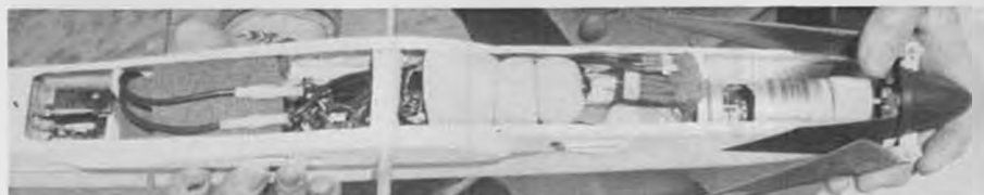
Bill Winans' Olympian carries the Geist 40/16 motor with gear reduction and folding prop. With 16 sub-C cells for a power source, the combo really performs.
