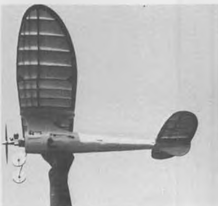
Ranger. Note wing and stab keys.
