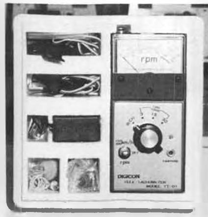
Condor Hobbies' new Tele-Tachometer, a Tx/Rx system for obtaining airborne info.
