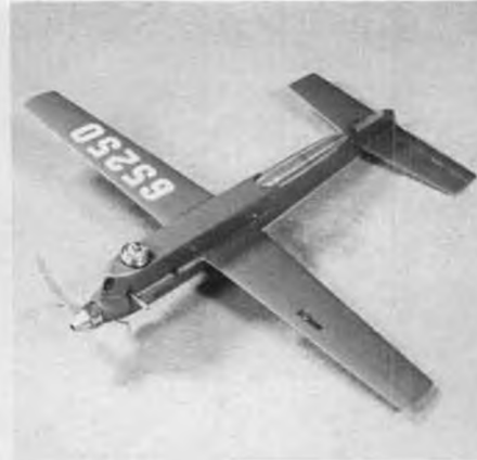
One of Dave Williams' monoline 1/2A speed models. F/G fuse on Cox 1/2A pan.
