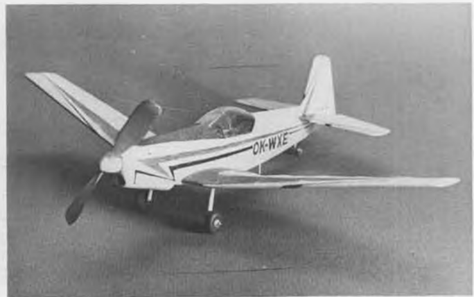
The Zlin 526 AS Akrobat Peanut model pictured here is yellow with red and black trim. The author's method of obtaining the yellow base color is to give the model a light coat of white paint followed by a coat of yellow felt pen ink.
