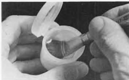
Dip brush in dope thinned 50-50 and wipe off one side of brush on lip of container.
