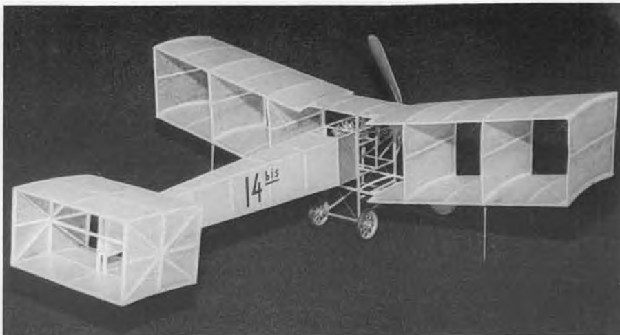
Peanut Santos Dumont 14 bis by Larry Kruse is based on a larger version designed by the master of the canard, Don Srull. Model is covered with Micro-X Early Bird tissue, with one thin coat of Micro Coat to seal surfaces. Model weighs 7 grams; rigging is 1-pound monofilament fishing line. It flies left and does over a minute consistently.
