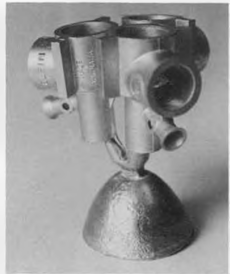
Stu was given this modeler's paperweight by Gordon. Crankcases are cast three at a time, in bunches.
