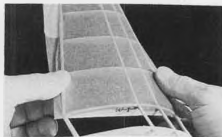
Using 60% white glue, 40% water mixture, cover top of wing in two pieces. Attach with thinned white glue, then pull out the wrinkles with your thumbs.
