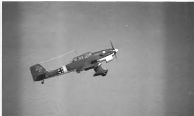
Bob Francis, Aptos, California, was 23rd with his scratchbuilt Stuka witha Sachs 3.7 gas engine. Model had flaps, dive brakes, dropped bombs, too. Wingspan was 105 inches, weight, 28 pounds.
