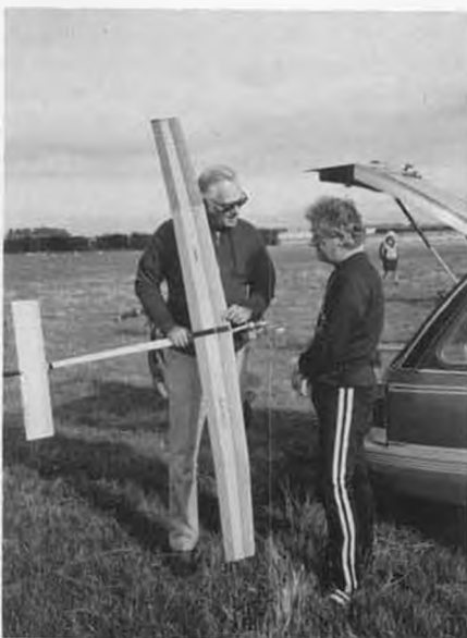
Doug Galbreath (USA) and Rex Bain (NZ) discuss Doug's F1C power model at the Pacific Free Flight Champs. The black carbon fiber fuselage was distorting in the sun, so Doug painted it white.
