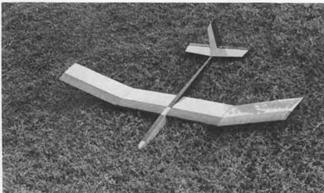
Harry Weitz's Slik 2-meter glider. Harry says the design flies very well using the 12-86 Airfoil of the Month, the S-3021.
