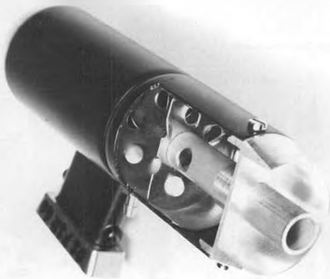
Here's what the inside of a Davis Soundmaster muffler looks like, and the reason it's so effective.
