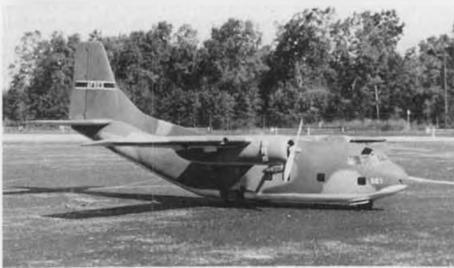
Looking like a real C-123, Ron Sear's model is control line scale. It's powered by two Wankel engines, this beauty features throttle, flaps, and retracts operated by radio control, the signals traveling through the flight lines.
