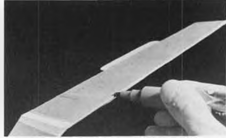
Uncolored balsa can be made to match colored tissue covering with help of a felt marking pen.
