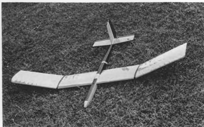
The Bumble Bee is a 2-meter, modified Selig 3021 glider. Slab fuselage, faster than the regular 3021. Extremely strong wings.
