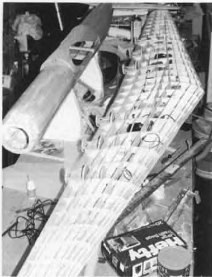
Wing and fuselage under construction shows traditional balsa formers, ribs, and stringers. Fuselage center section will be glued to the wing after motors, servos, wiring and sheeting are installed; wing assembly mates to fuselage with nylon bolts for easy access.
