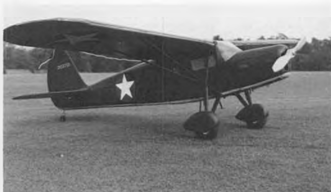
Dick Fleming also sent a shot of his '41 Fairchild UC-86, a scratch-built electric with a Hobby Lobby RX-15 motor with belt reduction, using 7 800 to 1200 mAh Sanyo cells. Covering is Micafilm.
