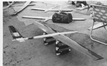
John Veale's O.D. racer is hard to beat. Fuselage is just big enough for the radio. Glass over foam wing construction.
