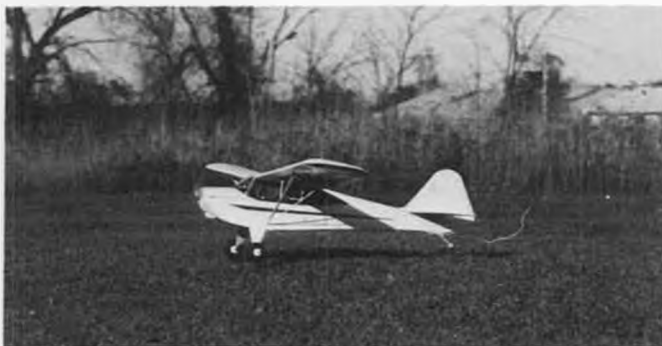
Dick Fleming's fine Taylorcraft just taking off from the grass. Dick scratchbuilt the model, with a wing area of 550 sq. inches. Weight is 55 ounces, and it is powered by an Astro cobalt 05 geared on 7 1200 mAh Sanyo cells, with Jomar throttle.
