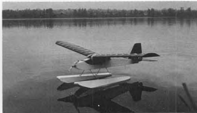
Author's Seagull, docile and easy to fly model which accepts many different kinds of motors. It will ROW on as few as five cells, although Mitch usually flies it on six cells. Details in text this month.
