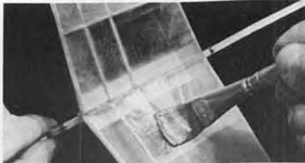
Brush dope from L.E. to T.E. and overlap the strokes. Use light reflected off surface to see places you missed. One coat of 50/50(1/2 dope, 1/2 thinner) should do fine.
