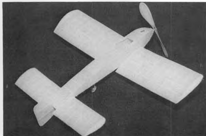
Peanut Blériot IV by Brent Saulsbury of Amarillo, Texas is from a Benno Sabel plan. Ship is covered with pre-shrunk Peck-Polymer's tissue. No dope. Weight is 5 grams, with Hungerford spoke wheels.
