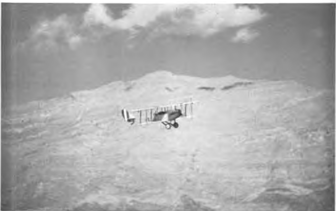
This Proctor kit Jenny flew on an Enya 80 four-stroke. Model is by Dick Hansen, Portland, Oregon. Spanned 87-1/2 inches.
