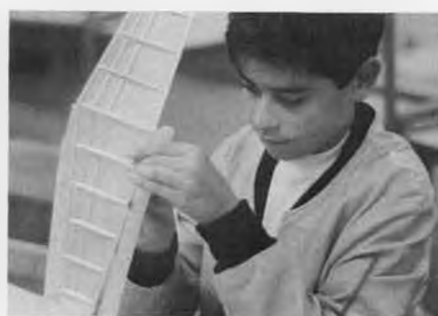
Joel Wagner uses razor blade to trim tissue. He is cutting away from his fingers.
