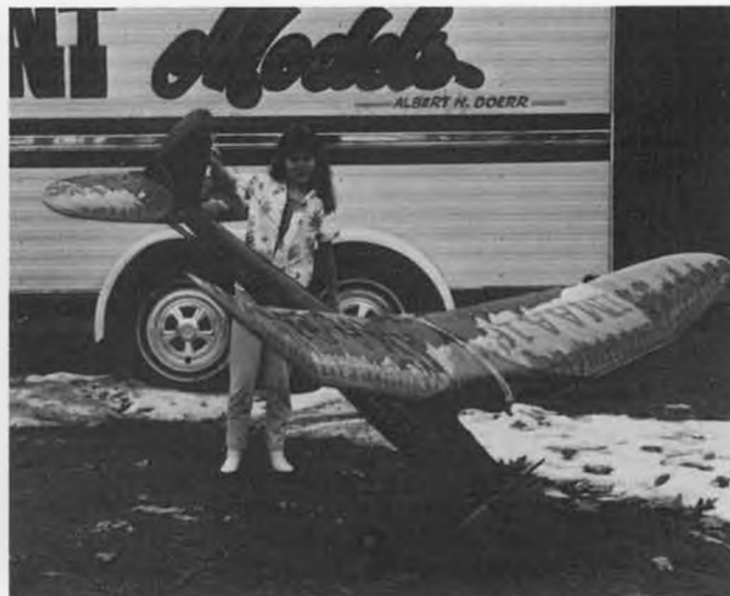
Al Doerr did an especially nice job on this double-size (13 foot) Goldberg Sailplane, powered by an O.S. FF-240 four-stroke.
