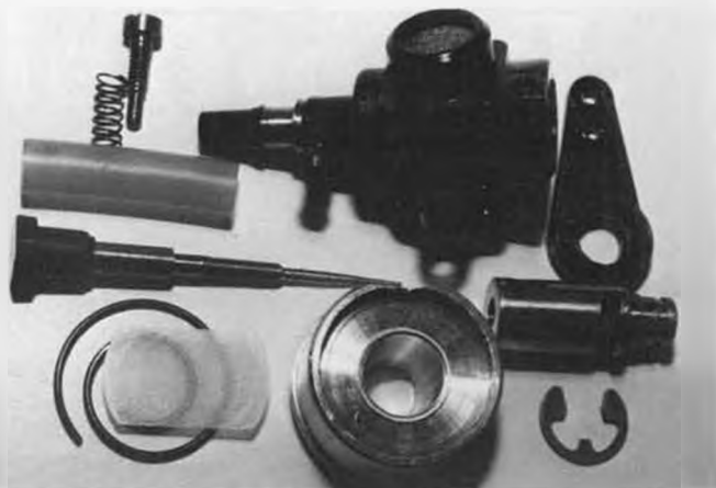
Disassembled carb. Note the teflon reed (laying on the coiled retaining ring) which serves as the inlet valve for the fuel/air mixture.
