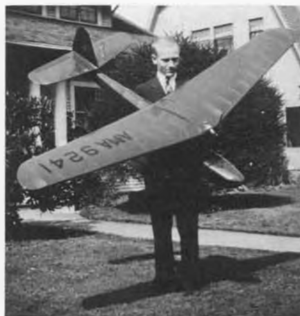
Photo from 1940 shows our columnist with an 8-foot, Super Cyclone powered F/F flying boat. Took off easily but proved to be spirally unstable.
