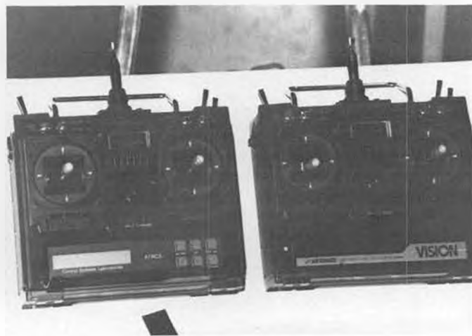
Airtronics' new Vision Series radios. They have a 16-bit microprocessor and the fastest scan rate of any of the PCM radios.
