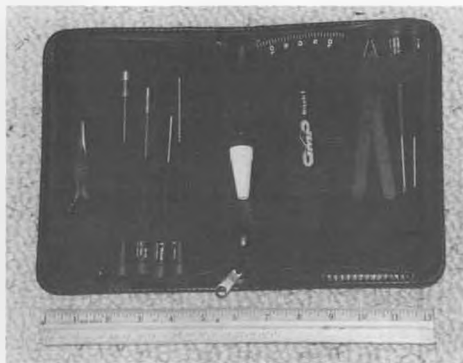
GMP's helicopter tool set includes chrome vanadium handtools, a pitch gauge, ball link plier, and Loctite. Less than $50.
