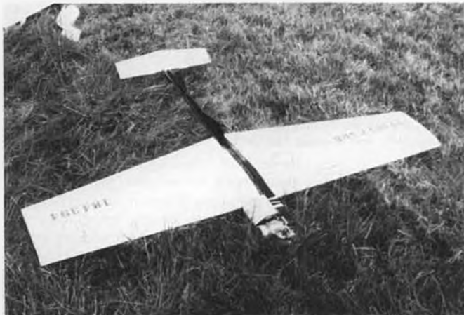
A good example of a typical Slow Combat ship. Fliers just getting into this event should pick a simple design with very few pieces.
