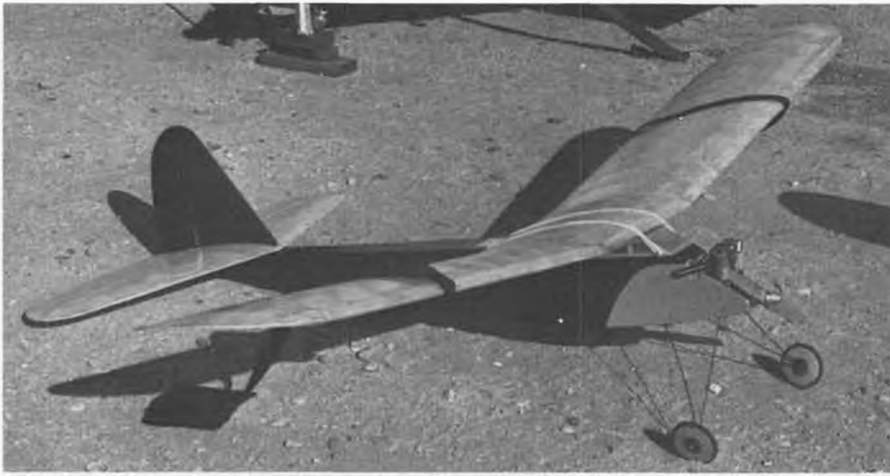
8. Just one of many competitive Chet Lanzo designs is this RC-1 built by Bob Grice of SAM 51. Uses a Saito 65 four-stroke for good climb.
