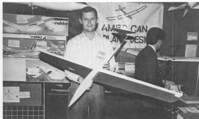
High-performance "Rotor" slope machine by Ken Stuhr uses pivoting wings to achieve the effects of ailerons and elevator.
