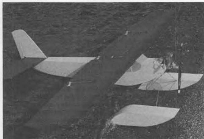
Author's triple-float seaplane, "SAM II," uses the rear of the fuselage as the tail float. Model is actually an amphibian, has thin plastic wheels mounted on the two main floats.
