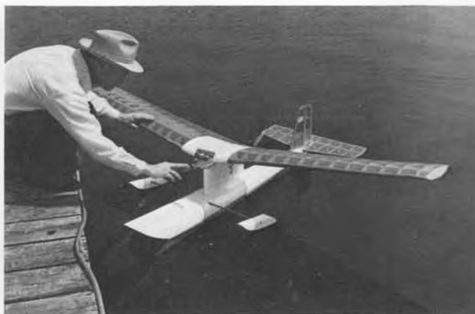
Author's world endurance record attempt seaplane had stabilizing floats (sponsons?) attached to the fuselage instead of the wing. Flew well, but radio problems did it in.
