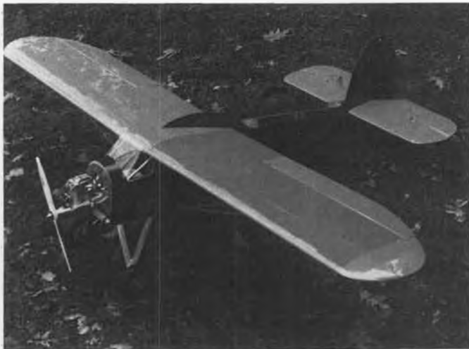
11. Don Lefferts produced this good-looking Belgian "Corsaire," modified with a different airfoil and ailerons. Uses Laser 61 four-stroke.
