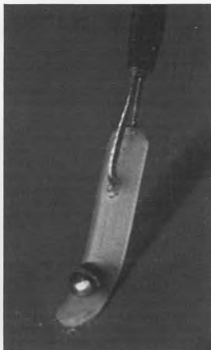
The Sage Hen's tail surfaces are wire braced. One-inch strips cut from nylon cable ties were used to attach the wires to the structure.
