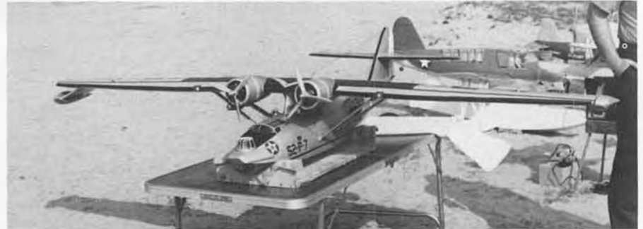
Another beauty from Sid Morgan plans is this PBY-5 by an unidentified builder. Power is two K&B .61's. Model is shown only partially assembled, which is why the wings seem to droop.
