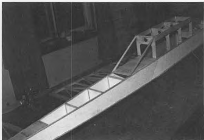
Basic fuselage structure, ready for installation of the pushrod tubes and the top and bottom fuselage sheeting.
