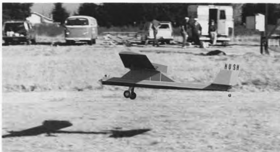
One of the prototype Sage Hens about to make a touch-and-go. You can see why she flies so well; lots of dihedral, a long tail moment, and mucho tail area.
