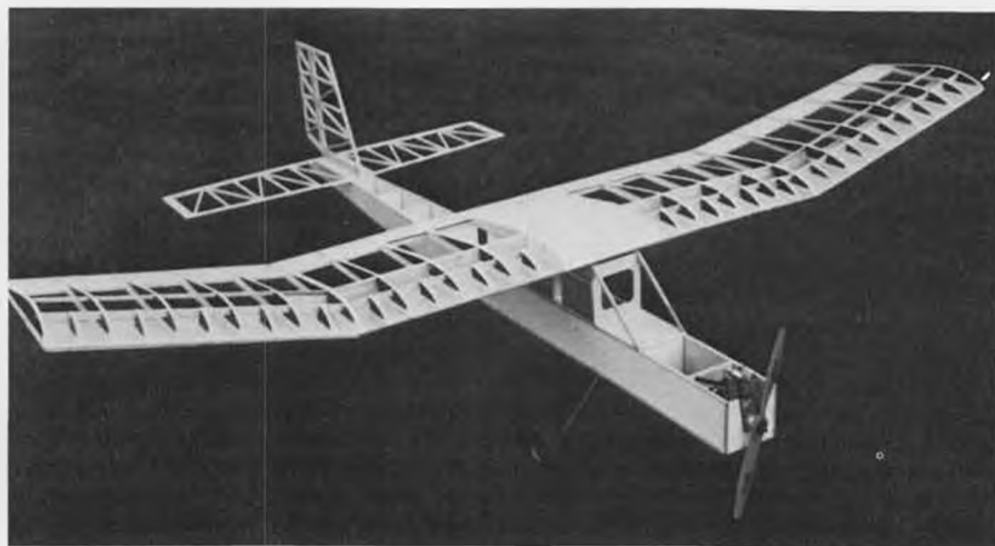
Wing construction has been modified since this photo was taken (see plan) by deleting the forward spar and extending the half-ribs back to the main spar.
