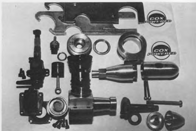
QB pretty much follows traditional Cox practice. A notable exception is the normal glow plug in place of the familiar Cox glowhead.
