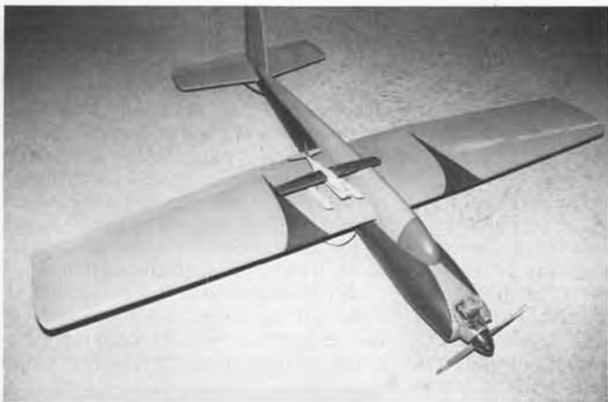
Ultra-clean "Seatract" features retracting floats (dark-colored areas on side of nose). Small scale model was used to develop the retract mechanism geometry.
