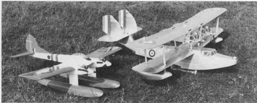
Author's two original twin-engine seaplanes, the Sea Hornette (left) and Supermarine Frigate. Sea Hornette, with only a 48-inch span, is a real wild machine with two Cox Conquest .15's.
