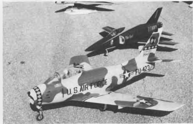
Bob Violett's F-86 Sabre. Equipped with gyro on rudder to help tracking. Has sequential operating landing gear doors. Also jettisons its auxiliary fuel tanks, for additional realism.
