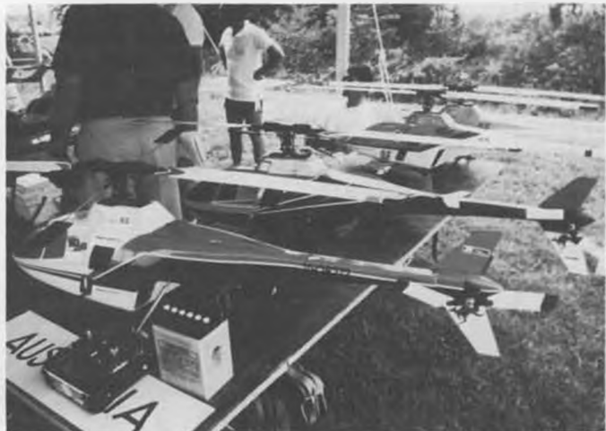
All of Australian team flew X-Cell 60's with Quicksilver fuselage. Wessel and Barbuto used Kevlar/fiberglass varying airfoil blades.
