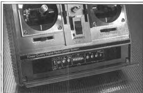
Servo reversing switches, dual rates, and more are conveniently located behind a smoked plastic window.
