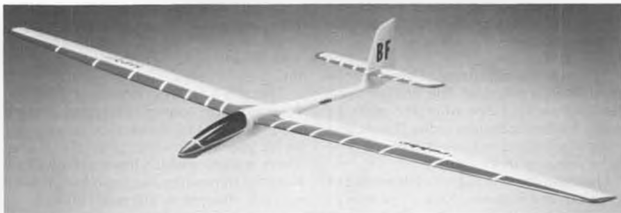
New Saphir from Robbe Model Sport. An ARF glider in two spans: 96 or 112 inches. Can also be converted to electric. Great model for those with little building time.
