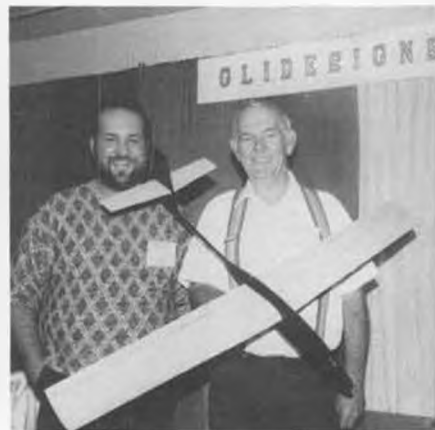
Glidesigns "Lance" ("Lance-A-Lot" not shown). Milled hollow wings from solid balsa. See text.
