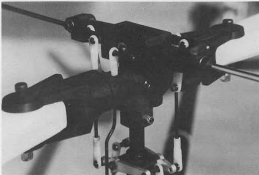
The K-5 rotor head. Above the 3mm nut you can see the teetering pin and brass bushing. See text. Sliding mixer shown has some play that needs improvement.
