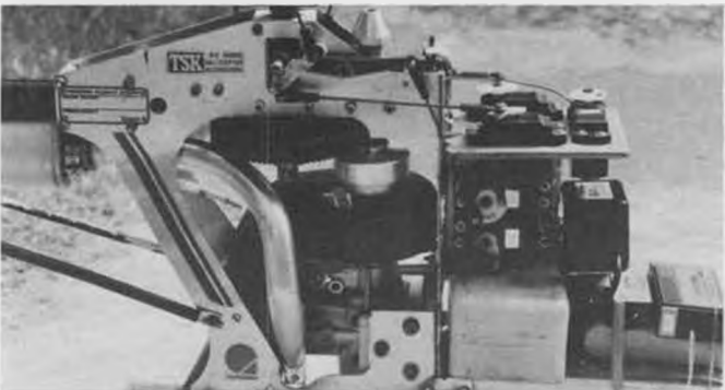
Complete Vanguard Installation, including 1991 narrow-band receiver. Special through-the-frame exhaust header designed by James, made by MACS.
