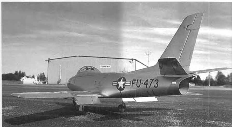
An outstanding feature of the BVM Sabre are the scale inlet and tail pipe openings. No "cheater" holes required to gulp sufficient air for proper operation.
