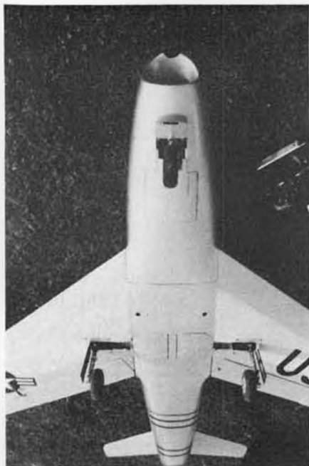
Three-step photos showing retract operation. In full down position, wheel doors are closed. During retraction, wheel doors open. Note nose gear rotating 90 degrees for flat storage of wheel. In final stage, gear is sucked up and doors are closed, all set for a smooth, belly landing. What are we saying! Just kidding, Bob!
