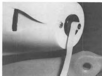
Wrap prop adaptor shaft tightly with masking tape to make snug fit with standard size hole in prop.
