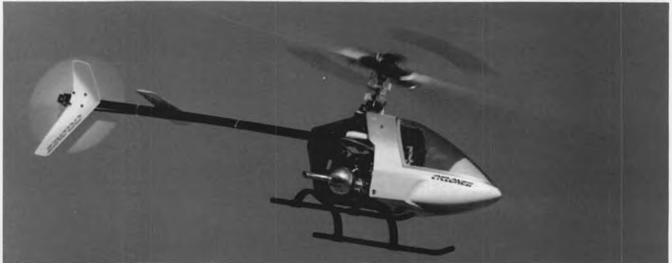
The author's Kalt Cyclone II test ship with pleasing paint job by Ray St. Onge. With OS 50H, it moves right along, does loops and rolls. At designer rotor speed of 1400 rpm control response is smooth, not quick enough for hot-dogging.
