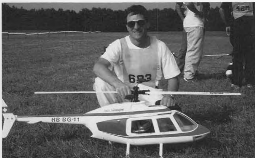
Two-time Swiss National Champion, Rudolf Linder, with his Heim Star Ranger. Had special shaped Sitar Hiller control paddles, parabolically shaped at tip to reduce profile drag.
