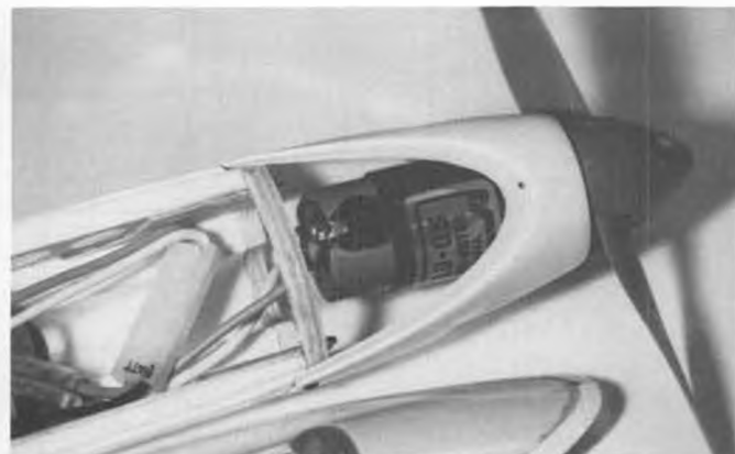
Completed installation. Note how spinner blends into fuselage. Prop is 8x6 Robbe. A Graupner folder would also work well.
