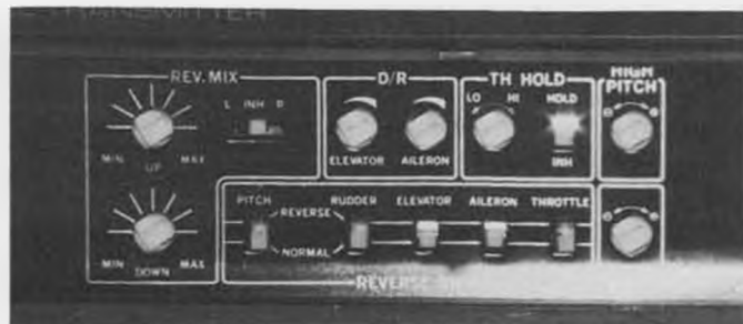
Under front cover are the helicopter functions. Here the 6H FM transmitter is shown. The PCM has failsafe in addition.
