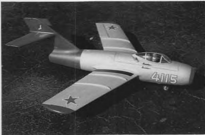
Dave Nicholson's modified Byron Mig-15. Uses BVM fan, duct, and KBV engine. Flies about 20 percent faster with this system.
