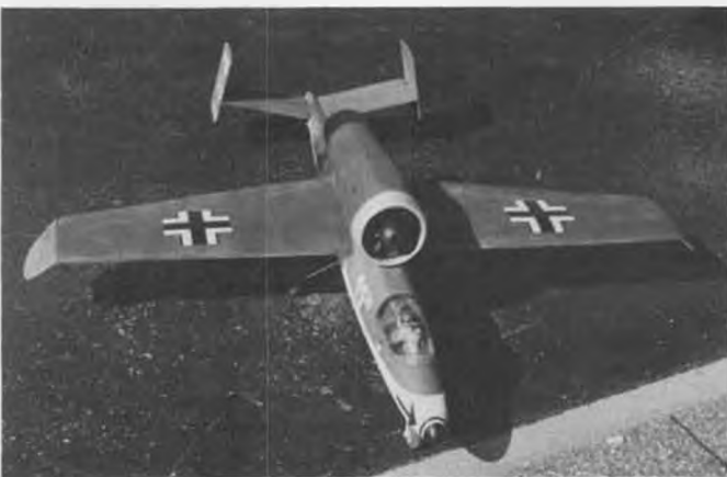
Dave Nicholson's Nick Zirolli designed Heinkel HE-162 unfortunately no longer kitted by Midwest. Modified to use BVM fan equipment and KBV engine, it flies fast and with authority.
