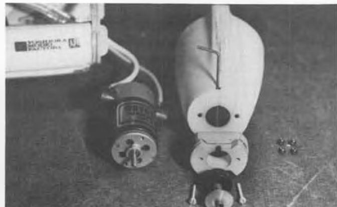
Whole assemblage from another angle. Note hole in cowl bottom to access Allen wrench to tighten set screw in prop adaptor.
