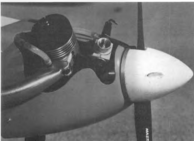
Business end of this month's ARF, with Rossi .40 and MACS Products header. Note heavy gauge fiberglass cowling.
