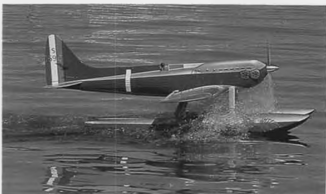
Ken Bundt's sleek 1931 Supermarine S6-B on a high-speed taxi. It is quarter-scale and powered by tandem-twin ST 6000.
