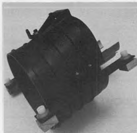
The Violett fan is double suspended in rubber mounts, for many good reasons.
