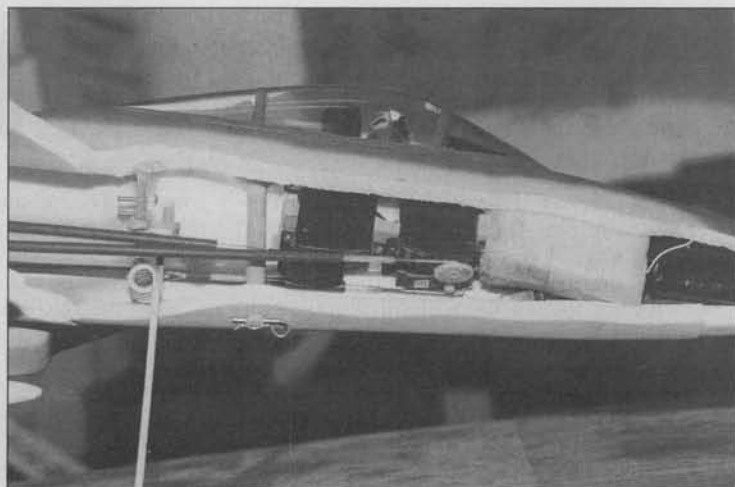
Factory cutaway demonstrates simple three-channel radio installation in forward area of fuselage.
