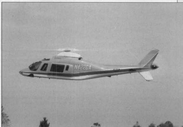
Dave Davidson's magnificent Agusta A-109 at the 1990 Raves Funfly in Virginia. Notice the windshield wipers and pitot tube near the front window screen. Has scale-like retractable landing gear. It is a Heim kit with Webra 61 engine. The full-size A-109 is made in Italy and has one of the lowest drag coefficient of any helicopter.
