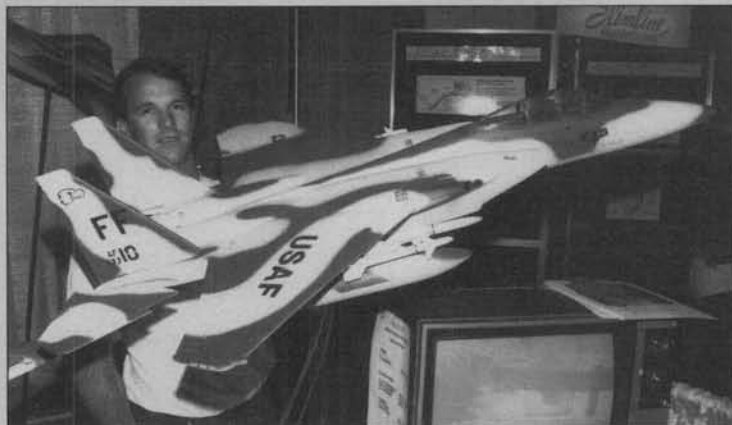
Byron Bruce of Combat Models with his molded high density foam F-15 Eagle warbird. Intended for .40-.50 power, can also be converted to slope soaring.
