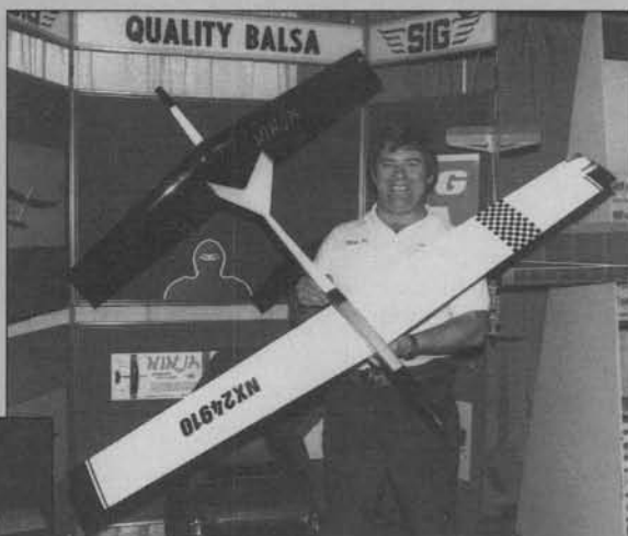
Mike Pratt in the Sig booth with the prototype, no-name-yet slope glider with pitcheron control and V-
