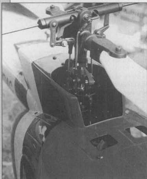
The two-bladed main rotor head on the Vario mechanics in the Peka MD-500 body. What a colorful rotorhead with pretty ball links! Superb German kit engineering by Uli Streich of Germany.
