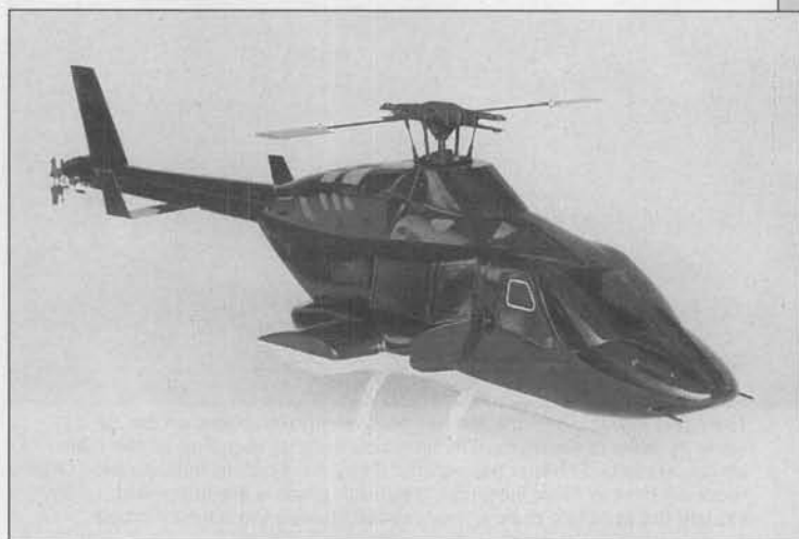
The 30-size Airwolf fuselage from Helicopter World Inc., $129.95. Optional retracts, $39.95. The fuselage is made from plastic similar to the Concept canopy, and it is pre-painted in black. The body will fit on Concept, Shuttle, Enforcer, and X-Cell 30. A
