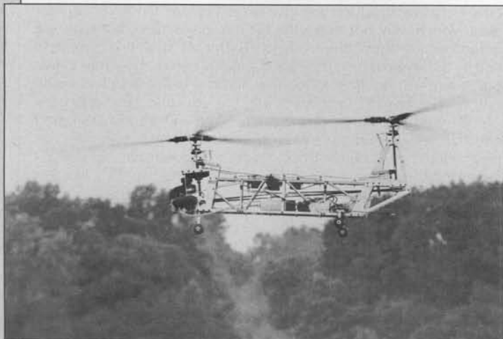
A scale Vertol tandem-rotor helicopter without the scale fiberglass fuselage. Quite stable in hover. The kit is manufactured by Hirobo in Japan. It is available from Hirobo's U.S. importer, Altech Marketing. Costs around $1500. It is powered by a single O.S. 32H engine.
