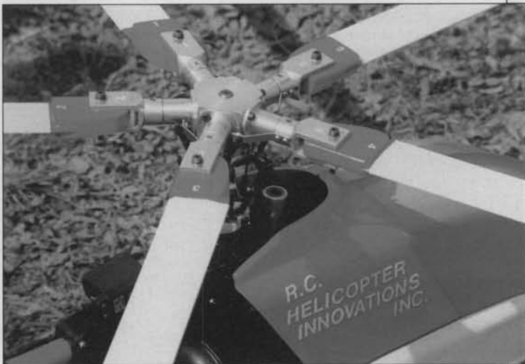
Another five bladed rigid main rotor head design. This one is made by Charlie Johnson in Virginia. His company name is on the canopy. Charlie sells this head for about $400. Call (703) 448-0876. I have flown this head. It is very responsive. Wood blades are used. It would fly better and less responsive if soft fiberglass blades were used. Rigid hub multi-blade rotors are easier to make than the articulated flapping head. But articulated heads fly better.
