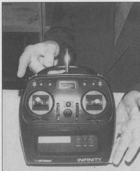
The new Infinity programmable helicopter radio from Airtronics. The shape, electronics and software are designed in the USA. Has LCD screen display. You can program the radio by touching the LCD screen. You can elect to operate on any one of the 50 available frequencies by touching the screen. Isn't this wonderful? This one transmitter will work with any Airtronics or JR FM receiver on any 72-band frequency.
