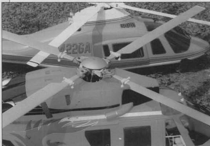
The scale looking four bladed hingeless main rotor head on the BK-117. Made by Wiks in Germany. The little bob weights dangling on the main blades are called "bifilar pendulum." They are used on full-size BK-117 to reduce 4-per-rev rotor vibration. If enough readers are interested, I will explain the principle of how they reduce vibration in a future article.
