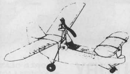
No. 776-O.T. RASSITOODUS $9.00 Novel canard design from '39 handbook. Span 60", 1/5 hp eng. By Herb Lozier.
