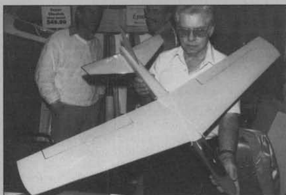
Robert Pettyjohn and the new Lynx from Cheetah Models. Features foam core wings, balsa fuselage and tails.
