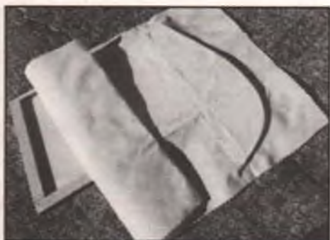
Bruce experimented with the F&M process on a Fleet biplane rudder. Here the lightweight Poly Fiber cloth is being applied to the framework with the Poly-Tak adhesive.
