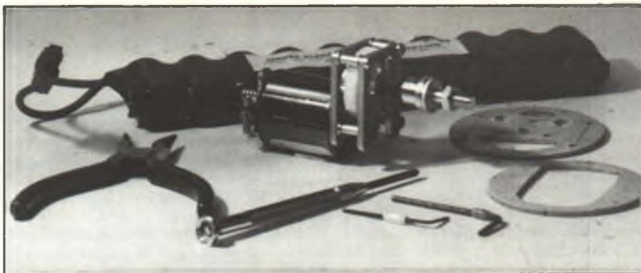
The latest in the War Emergency Power series from Model Electronics: the War Plus Turbo 10 motor, attached to a stock Super Box 6:1 gearbox. The plywood disk with the large hole is the firewall that is glued to the fuselage. The happy-face disk is the motor mount that carries the gearbox and screws to the firewall. A 10-cell Sanyo SCR pack provides very steady power output. Jim later shortened the prop shaft to reduce the large gap behind the spinner.
