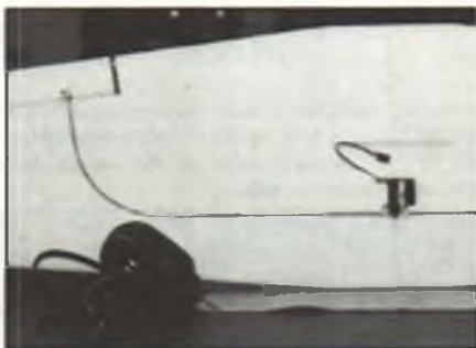
■ TOP LEFT: A soldering gun fitted with a couple of different homemade music wire tools cleanly cuts the aileron servo pocket and the plastic sheath groove. Jim says the one-piece cable from aileron to aileron is as smooth and precise as you could want—don't change it! ■ TOP RIGHT: This photo shows the original interior, but a case of nose-heaviness was solved by moving the elevator servo back and also opening the end of the foam battery chute; the battery now is farther back with its center of the balance point. The FX-35 speed control unit is mounted in the motor cavity. The motor, battery and speed control get very effective cooling.
