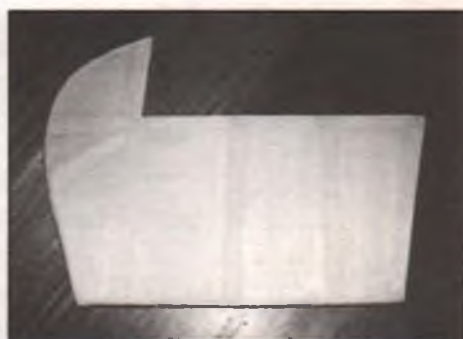
Here a coat of silver Poly-Spray has been added to the rudder to provide ultraviolet protection and provide the first sandable layer. Fiberglass parts such as wheel pants and cowls should have an epoxy primer coat or Feather Coat (FC-900) prior to painting with Poly-Tone.
