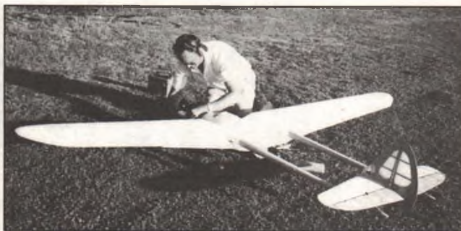
Photo No. 4. Airborne editor Merv Buckmaster recently finished this RC version of Ben Shereshaw's 10-foot XP-3, but mounted the engine in the nose to cure a bad case of tail-heaviness.
