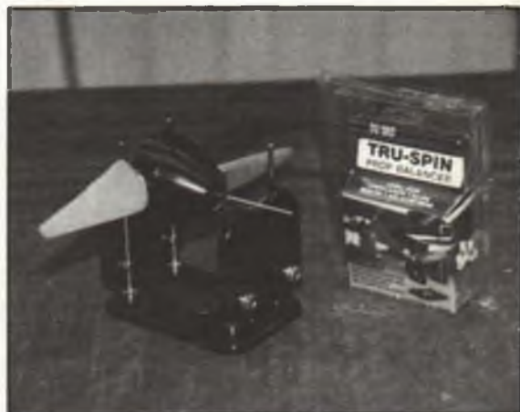
The supplied large spinner and Sonic-Tronics 13x7 landing prop require exclusive cutting for fit and for making air intake passages. De-Bro's Tru-Spin balancer was used to get it all back in excellent balance.
