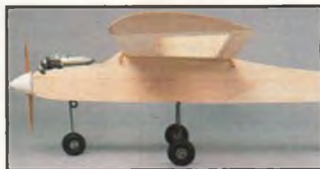
Wing dihedral and washout give PT series trainers uniquely stable, self-recovering flight.
