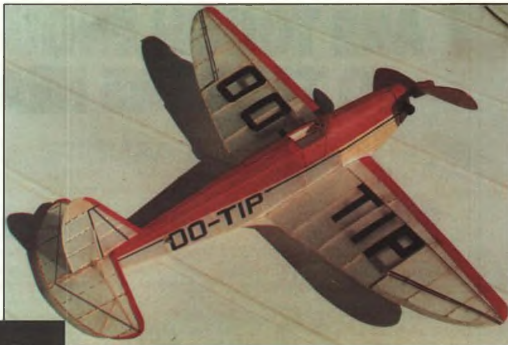
Another fine Topsy 52 as built by French scale expert Roger Alme from Siegfried Glockner's plans. Note that Roger employed translucent tissue covering, while Glockner's model is opaquely painted.
