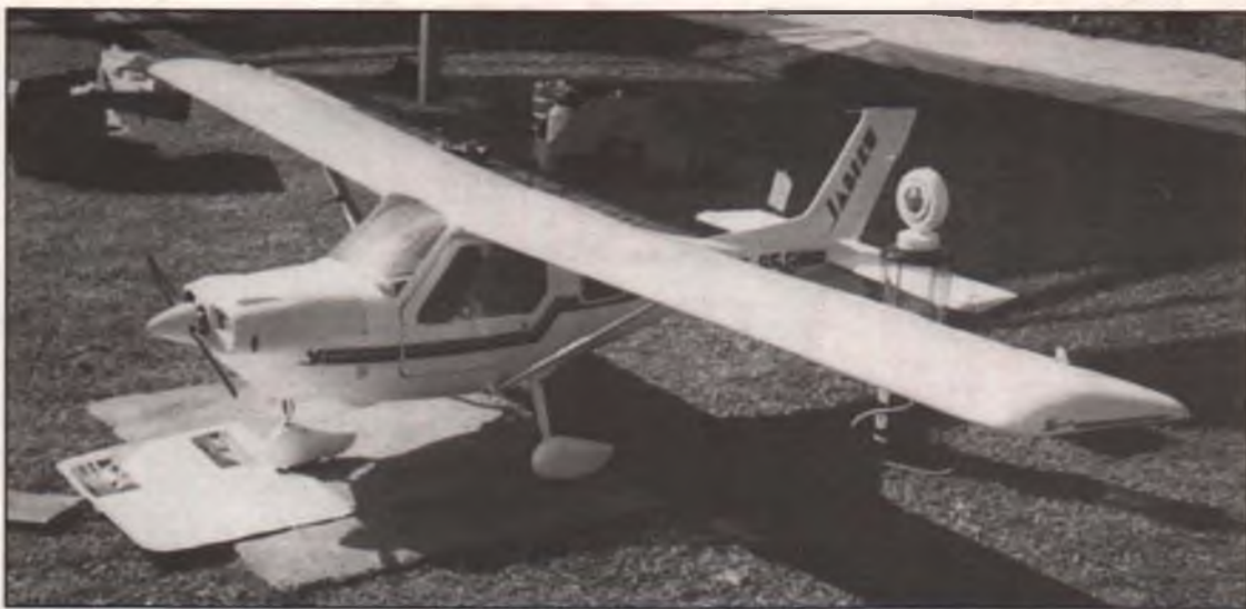
Many scale enthusiasts may not be familiar with the Jabiru, an all-composite two-place general aviation aircraft currently being produced in numbers in Australia. The 1/3-scale Jabiru pictured here was built from a molded, highly prefabricated kit offered by Noel Wilson; text has particulars.
