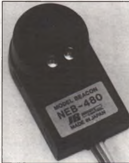
JR's Model Beacon is a small on-board device that gives both an audible and visible indication of your airborne NiCds' voltage status. Doubles as a model locator if your ship should go down in rough country.
