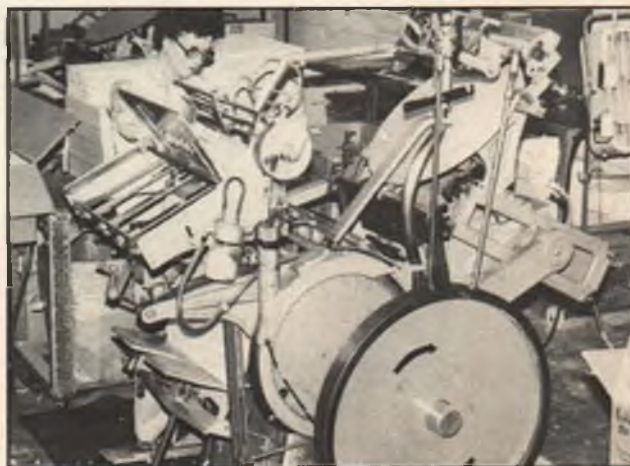
Like most other kit manufacturers, Sig uses a converted printing press to turn out die-cut parts for its kits. Last year, Sig entered the Laser Age by purchasing two double-headed laser cutting machines which can cut up to 24 balsa sheets at a time.
