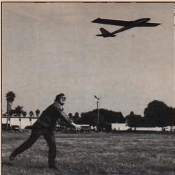
First test-glides should be performed over soft grass to prevent possible landing damage from being out of trim.
