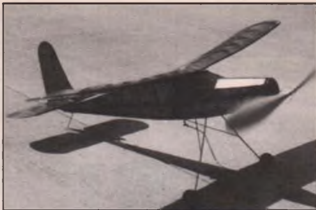
Photo No. 4. Ernie Wrisley turned out this good-flying example of the 32-inch Outdoor Cabin as originally designed by Virginia Sturiale and presented as full-size plans in Model Aircraft Engineer, May 1934. Model flies on 18 strands of 1/8-inch FAI tan rubber, and Ernie says the DT is absolutely necessary. Pond has plans.
