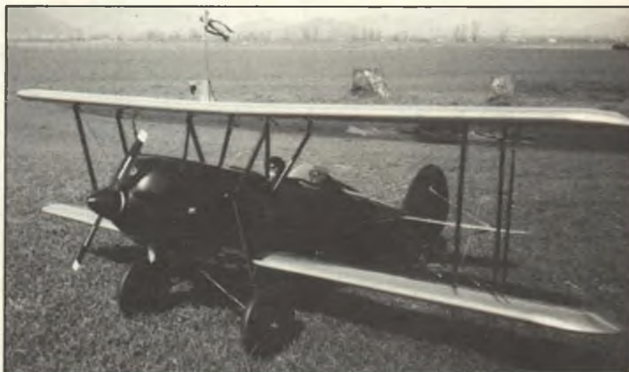
According to Bill Pottage, his Ikon N'west Travelaire 2000 biplane has been a real joy to fly. Wingspan is just over 5 feet, and Bill is using an O.S. .90 four-stroke for power.
