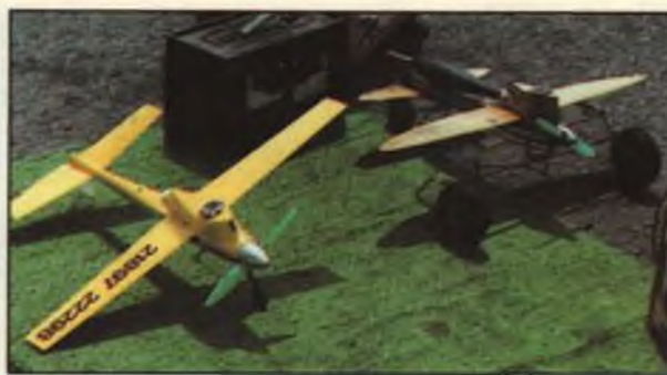
Speed planes are a triumph of functionality, with clean, sophisticated and sometimes exotic designs. Two examples seen at the 1995 Nats include a Formula 40 on the left (as a proto-style plane, it has a landing gear) and a conventional speed plane on the right (note takeoff dolly and tuned pipe exhaust).
