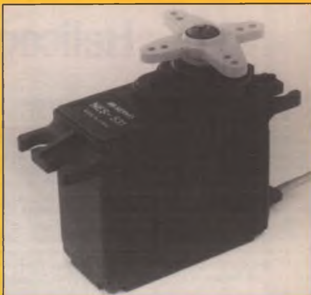
JR's new NES-531 could be considered a "high-performance sport servo," features a five-pole ferrite motor, ball bearing supported output shaft, and 51 inch-ounces of torque.
