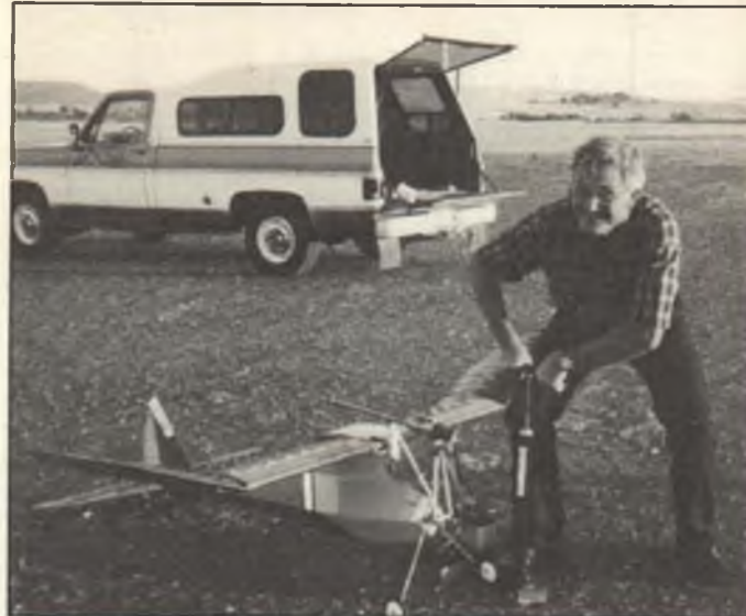
Photo No. 1. What the heck will these guys think of next? Stan Lane (pictured) and Jim Kyncy, both of SAM 30, teamed up to refit their RC Anderson Pylon with a Dyna-Jet, mounted above the wing. A new SAM event?
