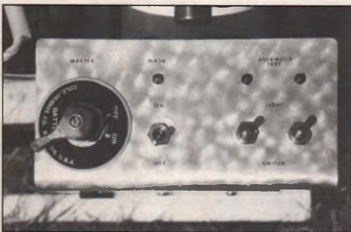
The control panel of the BAT winch is simple and effective. From left are the master on/off switch (mounted in the positive side of the battery cable), the standby switch, and the test lights for the two solenoids. Pressing the switch toward the winch tests the light itself; moving it toward the operator checks the solenoid. Each solenoid is tested individually. The switches should be in the middle position during launch.
