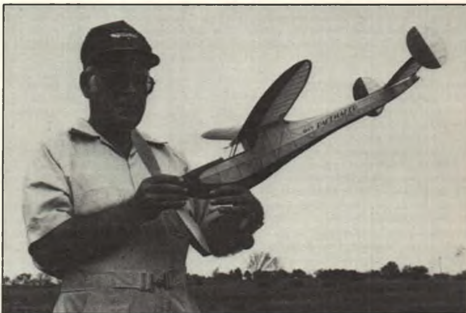
Jim Kutzka shows us his version of the Pacemaker decked out in yellow and black trim. The unusual lines of the model make it as attractive as well as an efficient platform. The huge 14-inch propeller is a decided advantage in SAM Commercial Rubber events. A dethermalizer system is an absolute necessity; Jim opted for a pop-up stabilizer. The Pacemaker might also be a good candidate for a pop-off wing DT.
