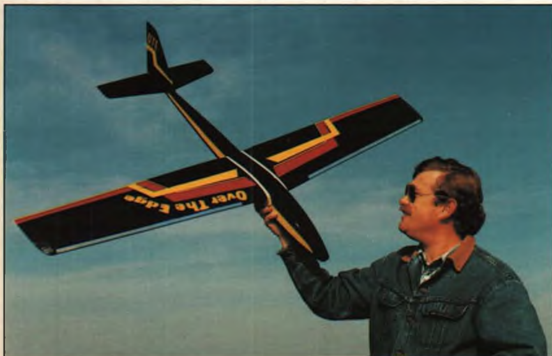
Bill looks pretty pleased with the way his Over The Edge came out. Model is covered entirely with black Solarkote, trimmed with Solartrim. Vinylwrite lettering and PEP's "Sky Sheen" reflective leading edge tape are nice, practical additions.
