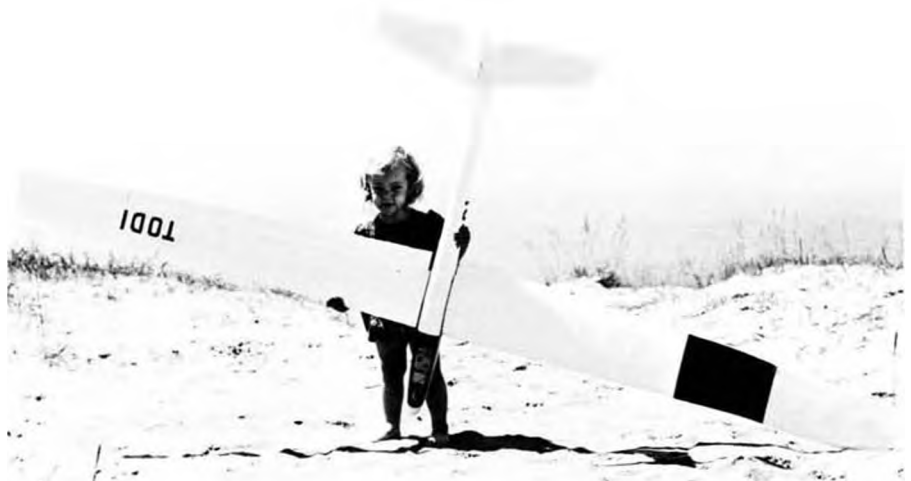
The "Todi" R/C glider by Dodgson Designs features flaperons that operate from minus 10° to plus 30°. Plane will fly fast, slow, inverted . . . or what have you . . . Ain't she cute?
