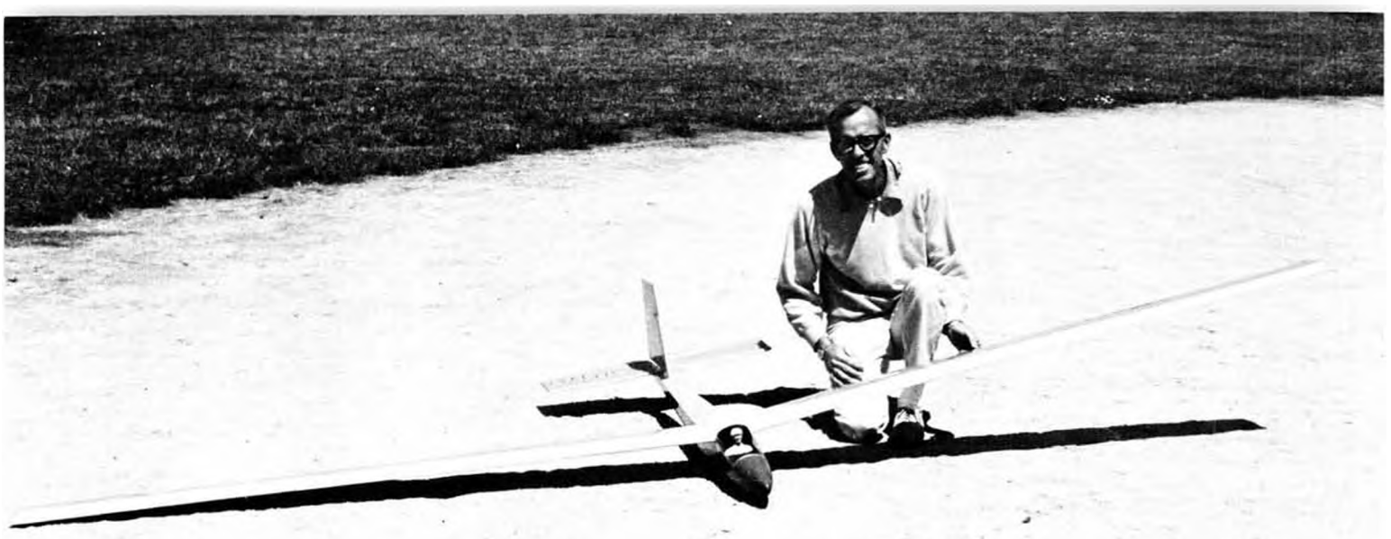
R/C Soaring editor's "Big Juan" had (radio interference) 12 foot span, 1060 sq. in., weighed 6 pounds (12.8 oz./sq. ft.), was fast clean, and efficient. Needed spoilers or flaps for landing. Airfoil was NACA 6412 at root, 6409 at mid-span and tip, 8" root chord.
