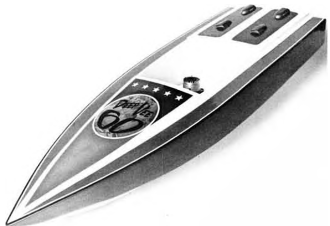
Dumas' DEEP VEE 60, a 38" long, 14" beam deep V boat for rough water racing. All wood construction.
