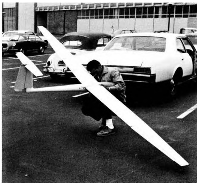
Bob Crumley's 13-1/2 foot scale AS-W12 has rudder, elevator, ailerons, flaps, retract gear, tail 'chute. Disposable water ballast next!
