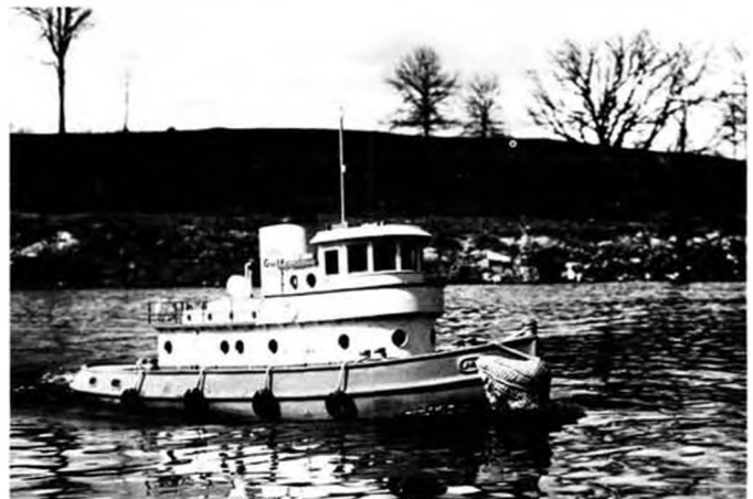
Boat is model of Harbor Tug "Douglas Greg." Length 42", beam 11-1/2", and displacement is 33 pounds. Electric or steam power.
