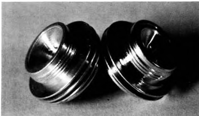
Which head has the 1973 Cox Tee Dee .049/.051? The one on the right, but don't go by part numbers . . . they're the same! See text.
