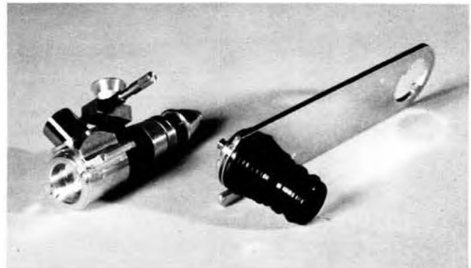
Proper way to remove Cox cylinder. DON'T stick wrench in exhaust slots or your piston will end up looking like a splined axle end!
