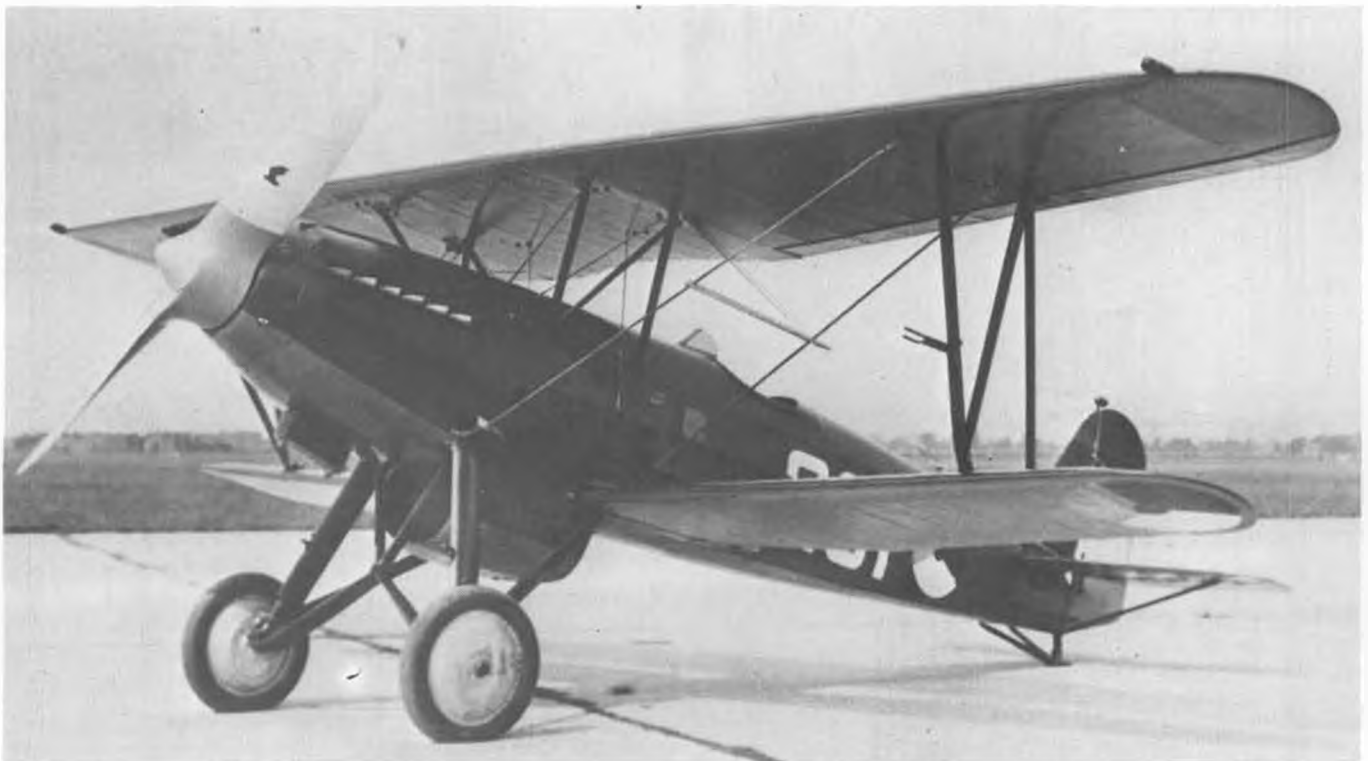
Production D-XVII had integral propeller and spinner hub, fixed tunnel type radiator, and 595 hp Rolls-Royce Kestrel IIS instead of the Curtiss Conqueror. Contemporary with the Hawker Fury and the Curtiss P-6E, the Fokker D-XVII had the same classic lines.
