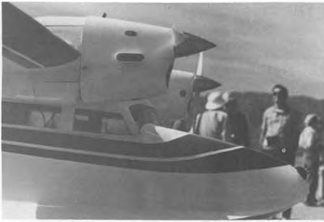
Twin front rotor K & B .40's power Irwin Ohlsson's modified Grumman Widgeon. One and a half pounds of lead in the nose!
