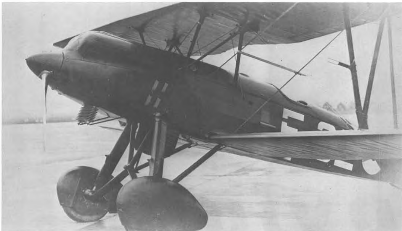
Close up of the prototype Fokker D-XVII with radiator partially extended. A Potts oil cooler has been installed, and wheel pants added. Venturi for turn and bank indicator just ahead of "F". Neat and snug fit on cowling around Curtiss Conqueror engine.
