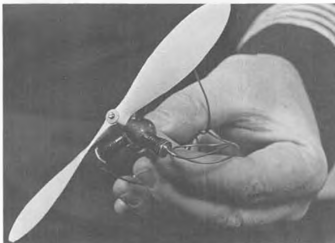
Fantastic 3 cylinder "Anzani" CO 2 engine by Capt. Ed Toner, Boeing 747 pilot for TWA. Photo by George Evans.
