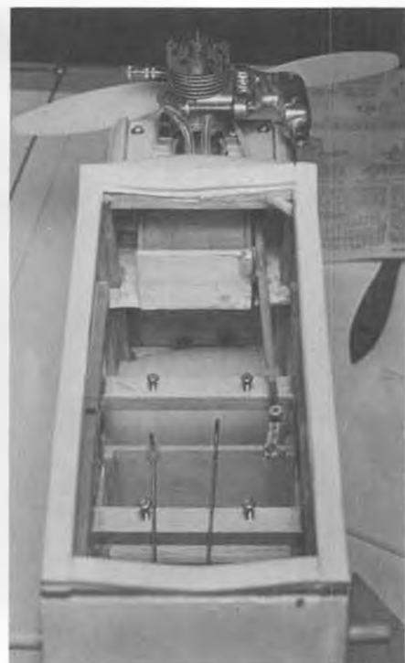
Because you always had to do a lot of fiddlin', the fuselages were designed with plenty of elbow room. Three-across servo tray fits easy.
