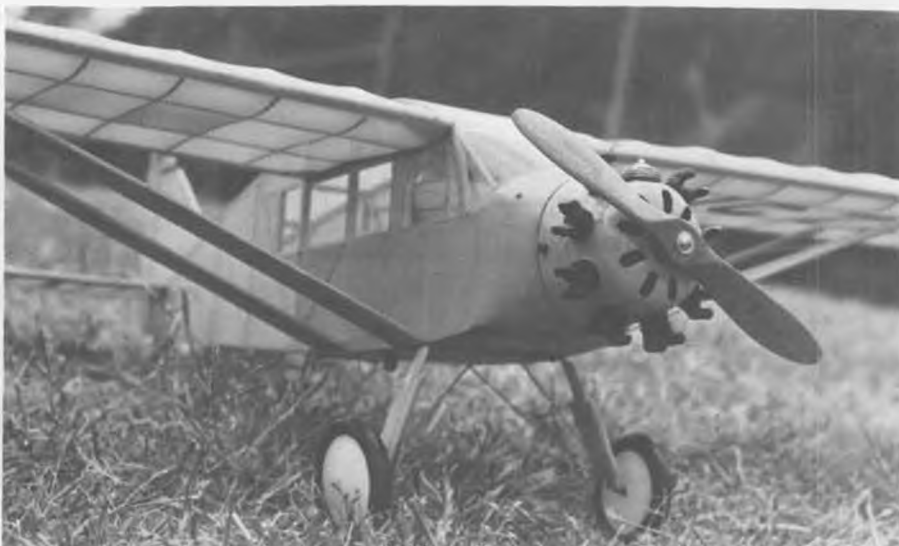
Two shots of Fernando's Flyline Bellanca "Skyrocket." Powered with a Cox .020 Pee Wee, and controlled by Ace radio on pulse rudder, the ship is a slow and realistic flyer.
