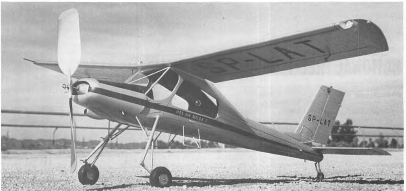
Don Typond's Wilga. Note the modified hubs on the Trexlers, as described in the text.
