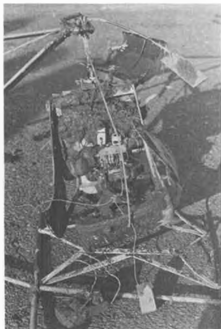
Radio problem resulted in high engine, no control. Ship dove in from 400 ft.! What a mess! Smashed bubble, split fuselage, bent tail boom.
