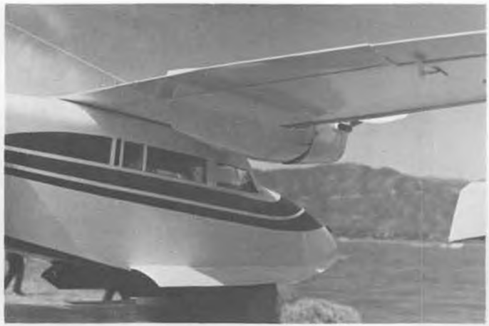
Wide sponsons are most obvious modification Irwin made on the Widgeon. Water handling was excellent.
