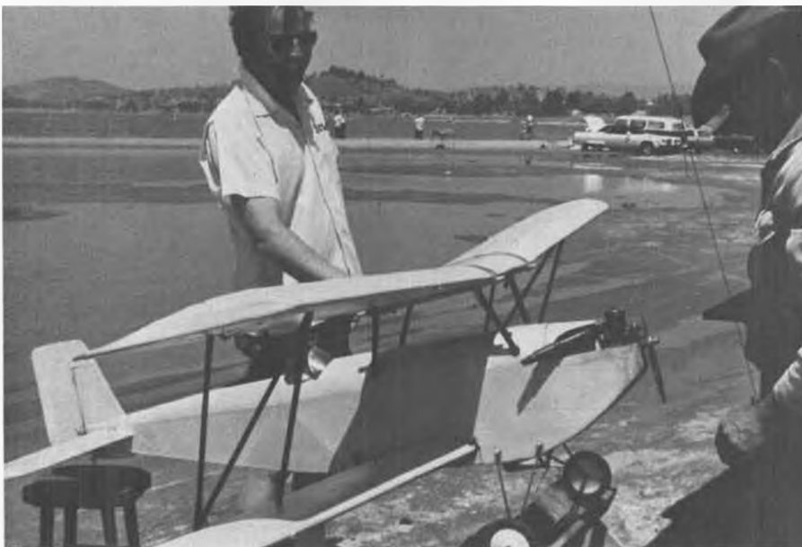
Artie, on the right, flies the big biplane with a Kraft radio. Power is an Enya 60 swinging a 13x5-1/2 and that exhaust pipe is from Lord knows what! Size can be judged by those 5" Wms. Bros. wheels. Flying speed is a honkin' 30-35 mph, and it seems to land at about minus 2 mph!
