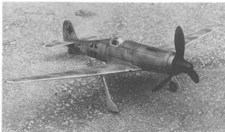
Rubber powered Foché Wulf TA 152 H1, by Lev Pazdera of Czechoslovakia. It has rubber actuated retractable landing gear. Span is 27-1/2 inches.
