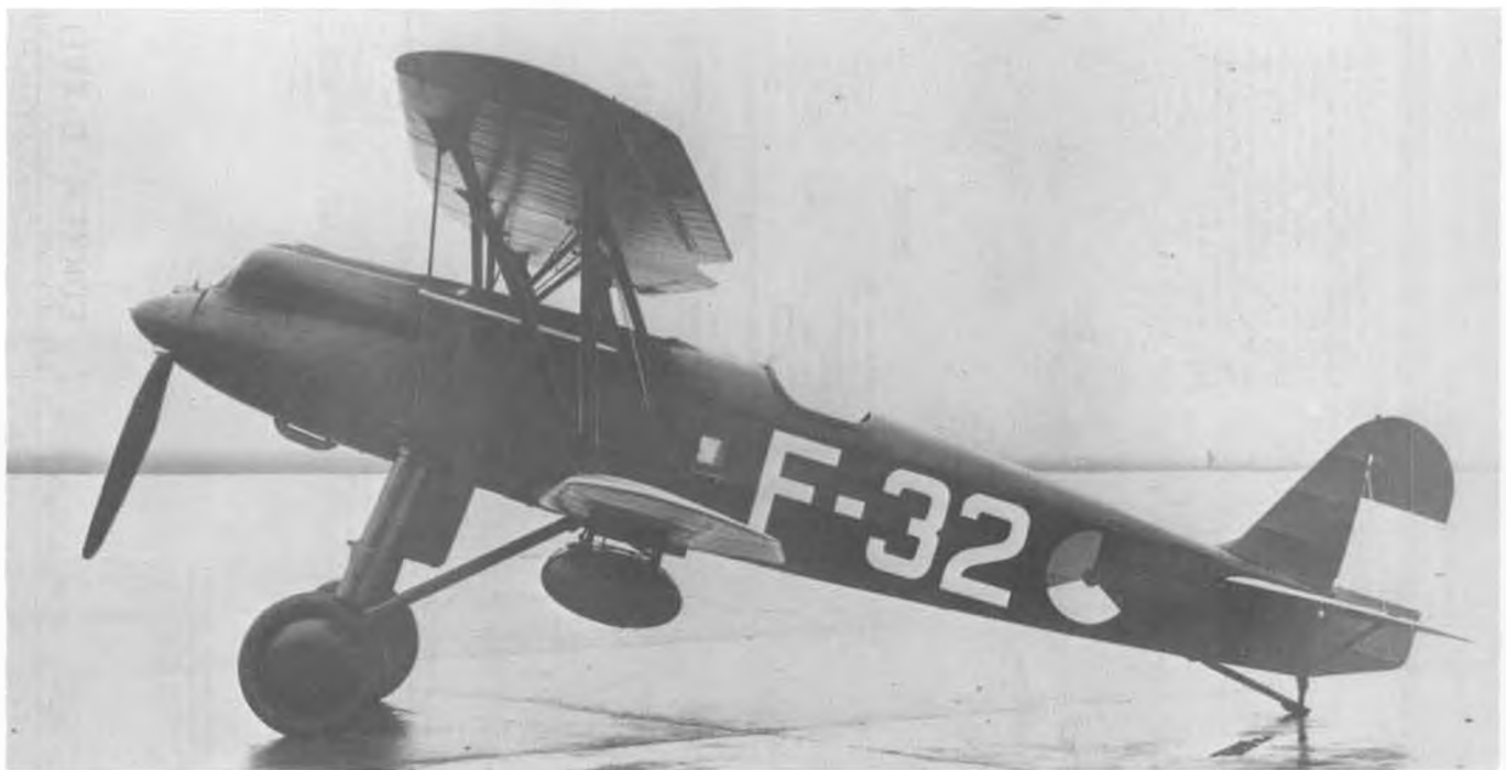
The prototype Fokker D-XVII with retractable radiator extended and jettisonable auxiliary fuel tank installed. Beautiful cowling job.
