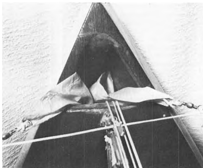
Close-up of bow "tunnel" with spinnaker clews partially extended. Halyard and bungee are running down the tunnel; also jib halyard.
