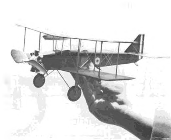
The extremely wide landing gear tread shows up well when seen from this angle. Williams Bros. cylinders used to make the engine.
