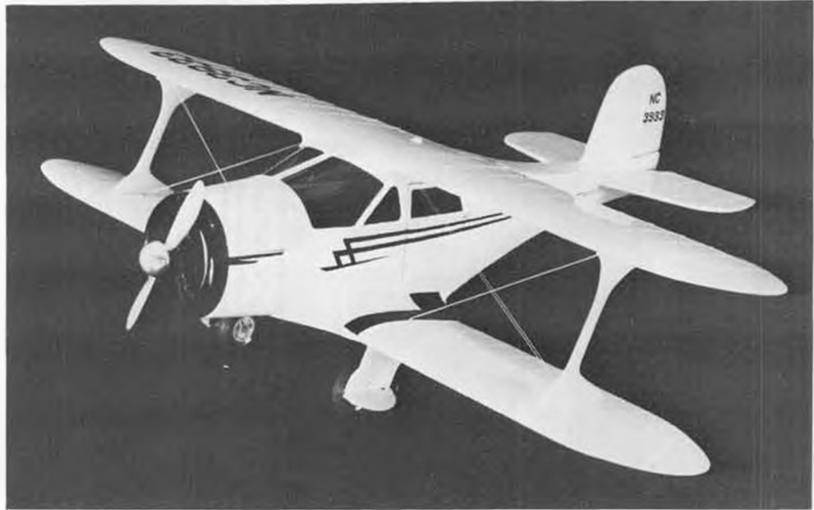
R/C scale Staggerwing Beechcraft, by Lenco. Scale is 1-5/8", span 55 inches.
