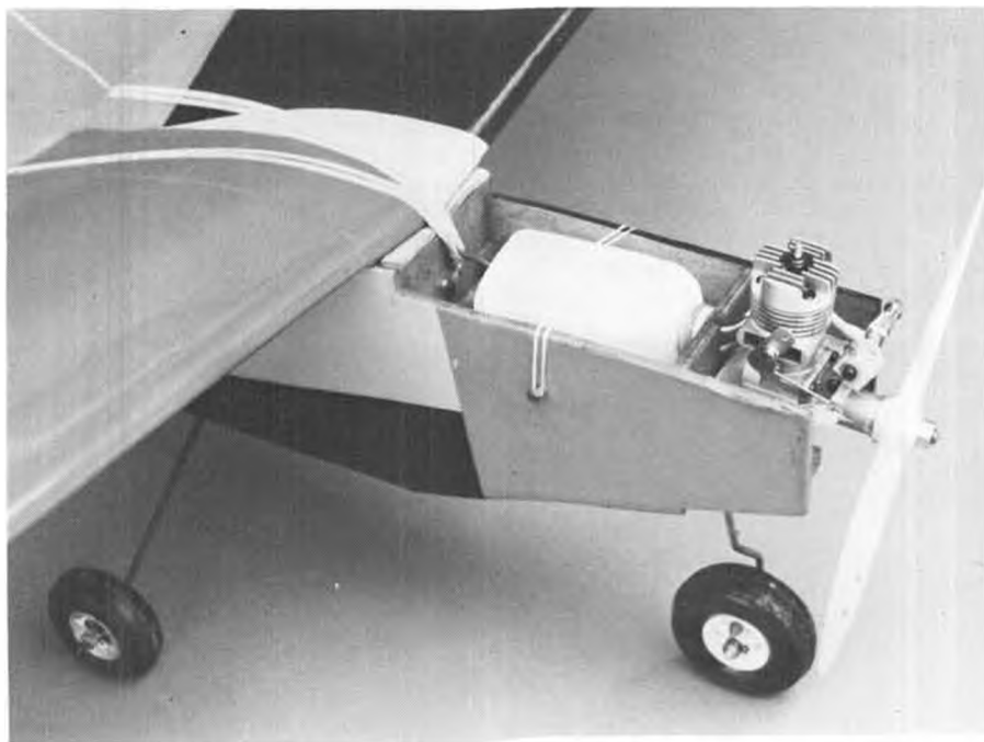
How's that for an accessible fuel tank? Enya .19 is more than adequate power for the "Boxy Bunny." Ground control is sufficient without the need to rig a steerable nose wheel.
