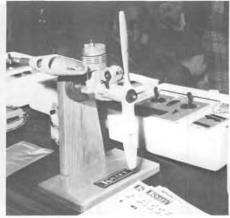
The new Kraft Schnuerle ported R/C 60 engine. Double ball bearings.
