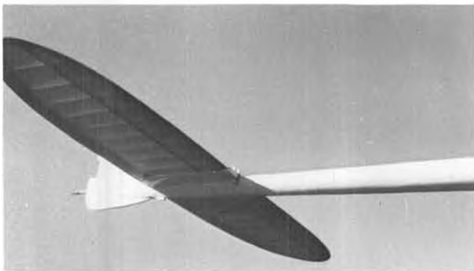
Tail feathers. VTO peg facilitates takeoff and eliminates possibility of damage or detrimming of rudder tab during launch.
