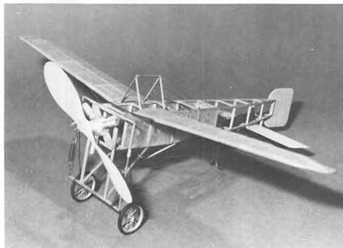
Dave Acker's Bleriot, constructed from Henry Struck plans. Bamboo struts, covering from Cleveland kit, flies on paddleball rubber!
