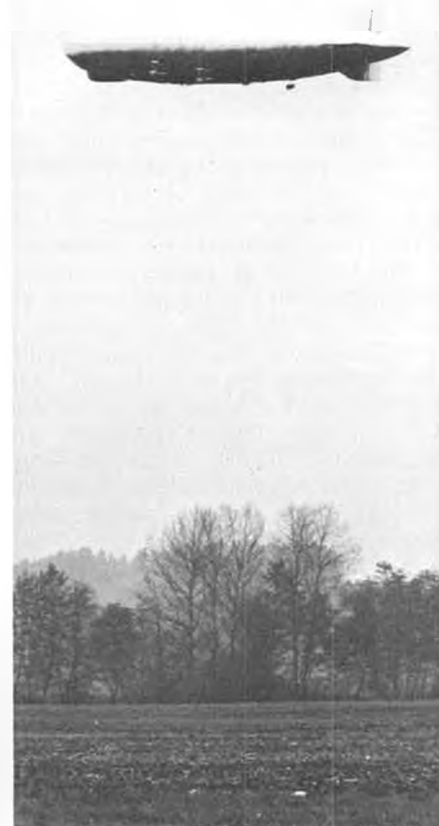
With nothing to produce scale effect, the huge model looks absolutely full size in this flight photo. It's covered with metalized plastic.
