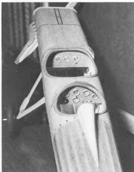
Instrument panels in Salvatore Alu's Eaglerock. Just enough detail for effect without weight.
