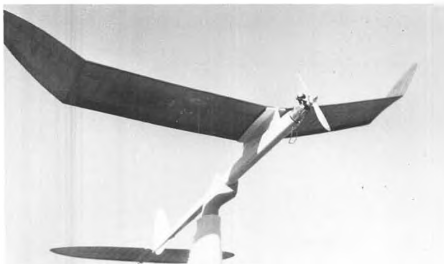
Earlier version of the Shrike with forward fin. Aft fin provides more consistent power pattern. Design has been well tested in all kinds of air.
