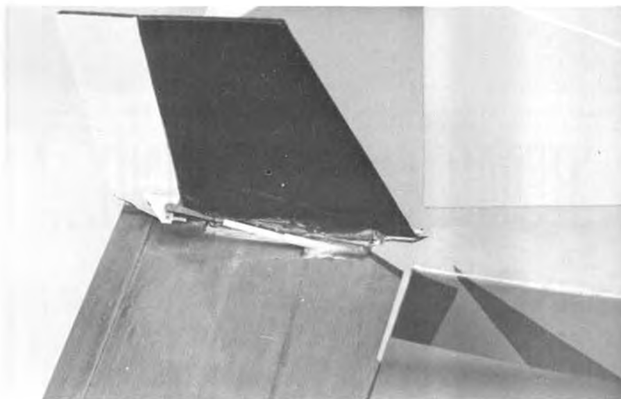
All-sheet tail surfaces glue directly onto fuselage. Run control tubing before final assembly. Considering usual nose-heaviness before trimming, 3/16 rather than 1/8 sheet could be used for tail.
