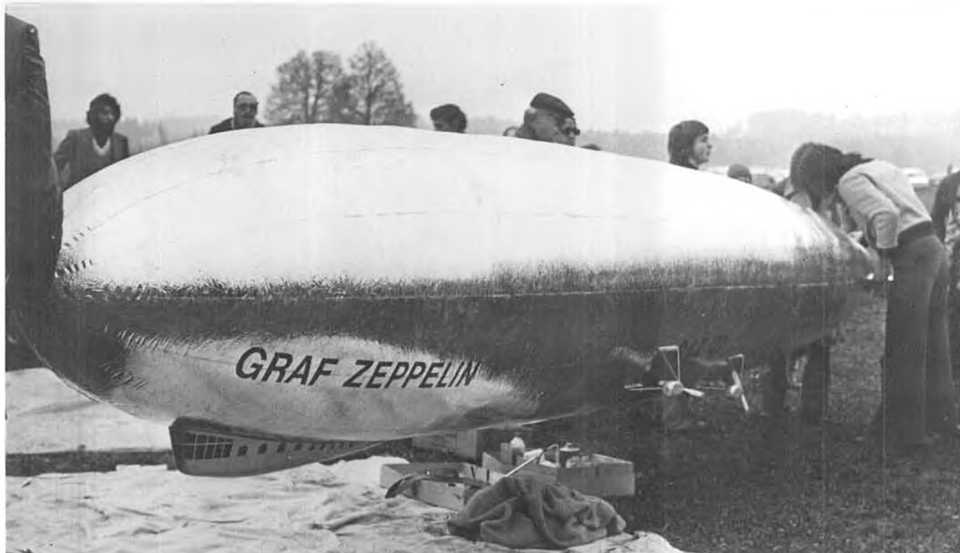
Fantastic flying scale (1:35) model of the Graf Zeppelin, is 22 feet long, 3 feet in diameter, powered by 5 electric motors, and flies at about 12 mph. Photos and information sent to us by Emil Giezendanner, Switzerland, where the dirigible was built and is flown.
