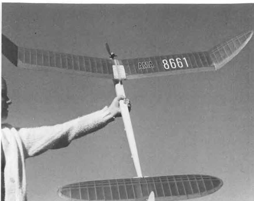
The Shrike's long tail moment controls power. The generous dihedral is also helpful in gusty weather. Closely spaced ribs assure a more consistent airfoil.
