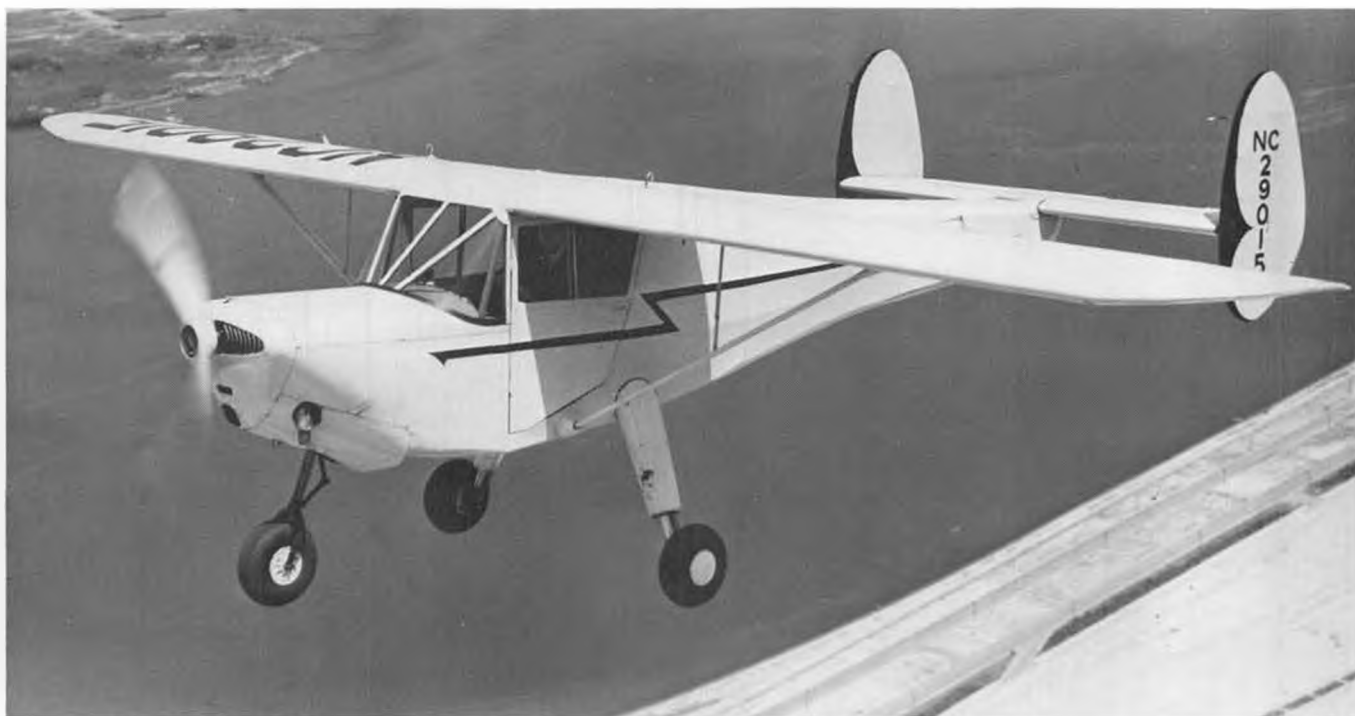
Air-to-air photo of the Skyfarer, taken by famous aviation photographer Rudy Arnold. Fins were fixed, and like the "Ercup", the plane could not be over-controlled. The opening of World War II put an end to its career.
