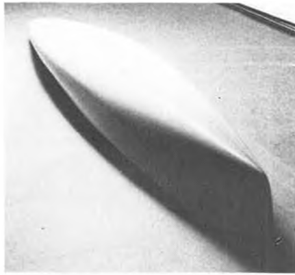
Chip Bullen's "Liberty 76" shows narrow bow sections for minimum wave resistance on wind.
