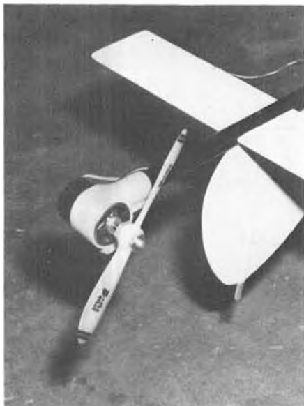
Separate tail drive motor on Gilbert's electric chopper solved underpowered problem.
