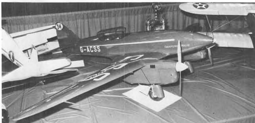
Col. Bob Thacker's DH Comet "Grosvenor House" Golden Era racer. Opposite rotating Veco 60 "pumpers", 13 pounds, and about 640 squares Yipes!
