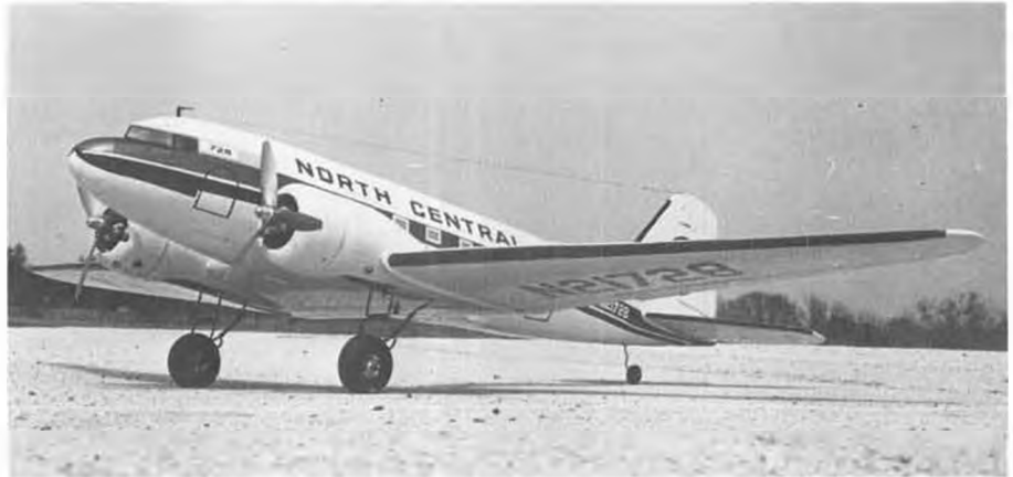
Jim's DC-3 with a more suitable background. What a difference a little planning can make! Ship has homebuilt retracts, Freon operated, and Wankel engines. Neato!
