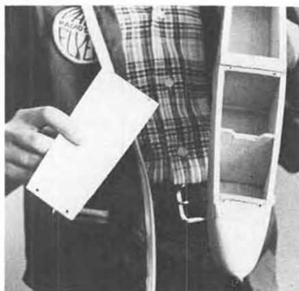
No pop-off canopy here! Hatch cover is firmly held in place by four screws.
