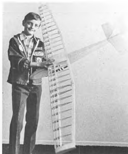
Completed framework, ready for covering. An excellent beginner's built-up model.
