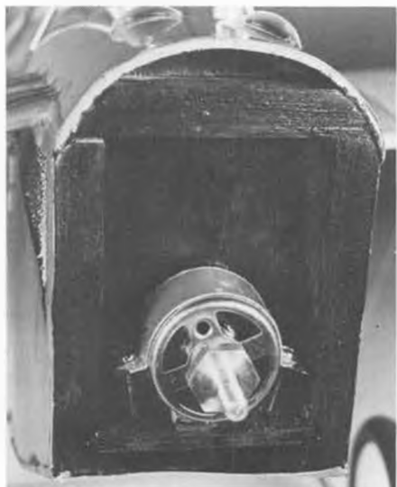
The Astro Flight 020 electric motor is simply strapped to the mounting plate.
