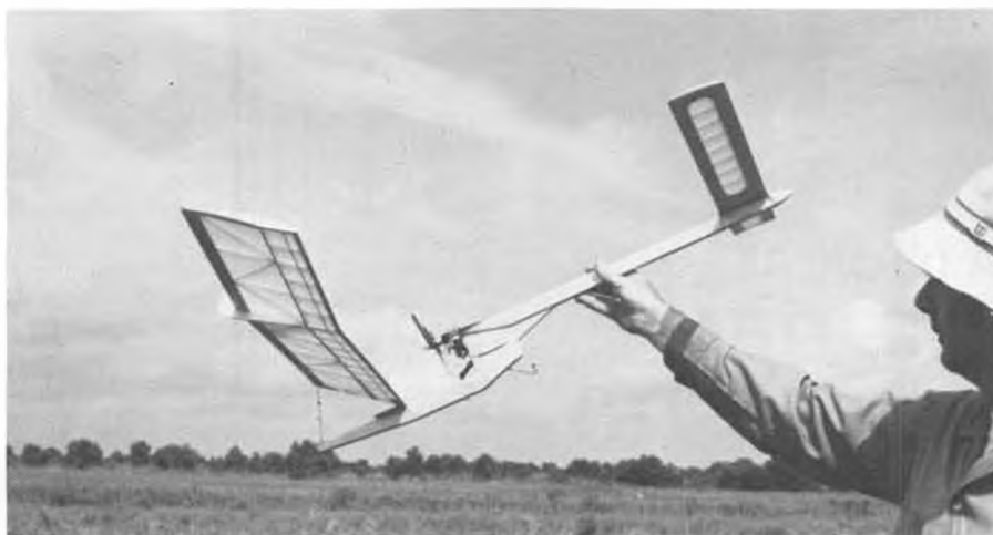
That's right, it's the main wing that pops up for the DT. The twin .010 Tee Dee version took first in Cargo.
