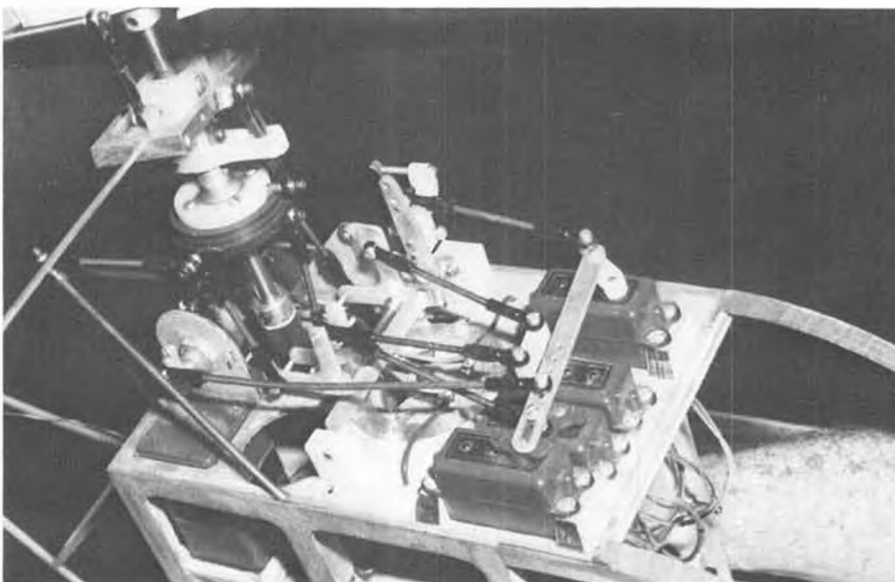
Control system on Charlie Gilbert's electric chopper appears Rube Goldbergish, but everything has a purpose. Main purpose is to keep weight to a minimum. Power-to-weight is excellent now!
