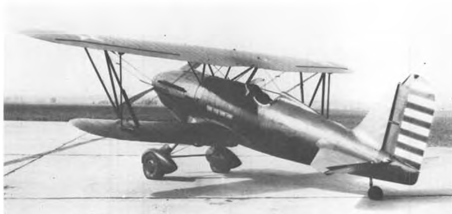
Adjustable horizontal stab moved in cutouts covered with sliding plates. Landing gear of YP was beefed up with streamlined cross-strut and wires.
