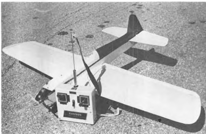
Jim Houston's Junior Nobler, converted to R/C with Cannon Mini-Twin, and Cox .051 Tee Dee. Fuselage length unmodified.
