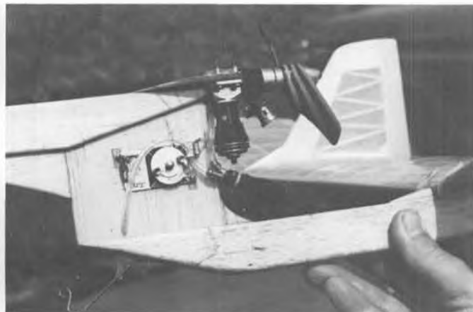
To cut down on messiness, fuel is dumped for cut-off, rather than flooding. Hand carved prop is best, but it lasts forever.
