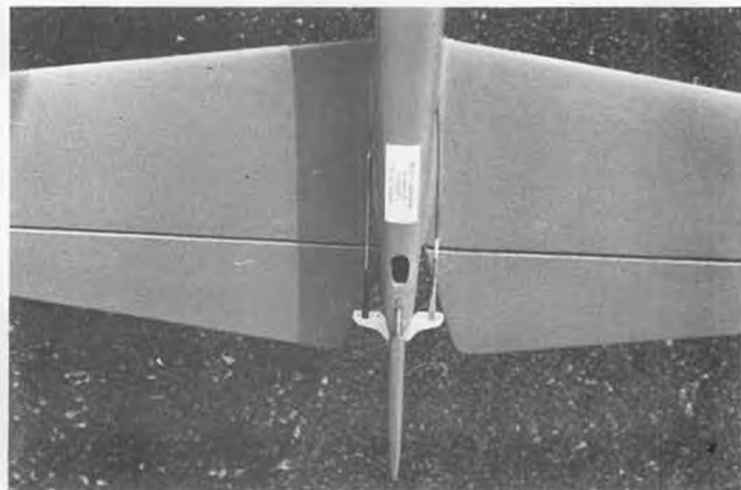
The end! Note dual rudder linkages which eliminate slop, also wire skid to protect rudder during nose-high landings, identification tag.
