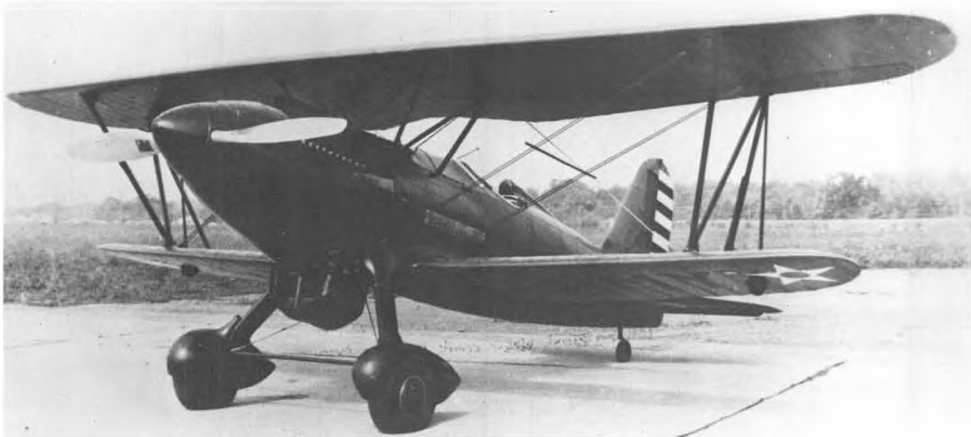
Standard PR photo of the 1930's shows that the YP-23 was in the same class as the Hawker Fury, Avia B-534 and Fokker D-XVII. With supercharger removed, it had classic lines, but speed was reduced to 200 mph at 15,000 feet.
