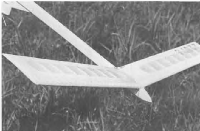
Turbulator on the front wing works well in the subcritical Reynolds number range in which it operates. Note high aspect ratio.
