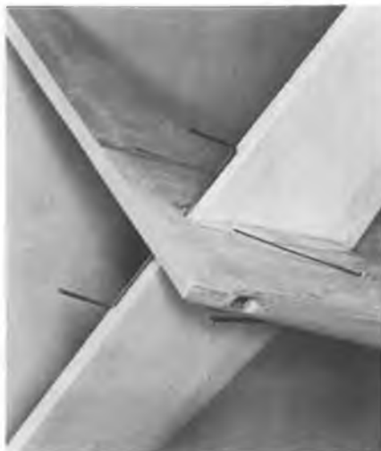
Tail section prior to attaching control surfaces. Note elevator linkage inspection hole.
