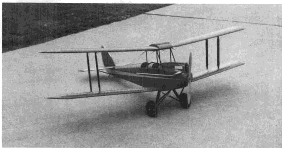
Another just-completed photo. Forster .99 was unable to get the plane off of a close-cut grass field . . . was later replaced by Fox .59 that powered very first "Big John".
