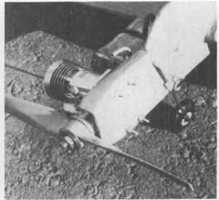
Instantly detachable landing gear has shock absorbing coil for smooth landing in grass.
