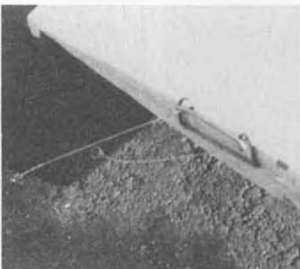
Leadout guide. Leadouts can be threaded through when changing wing.
