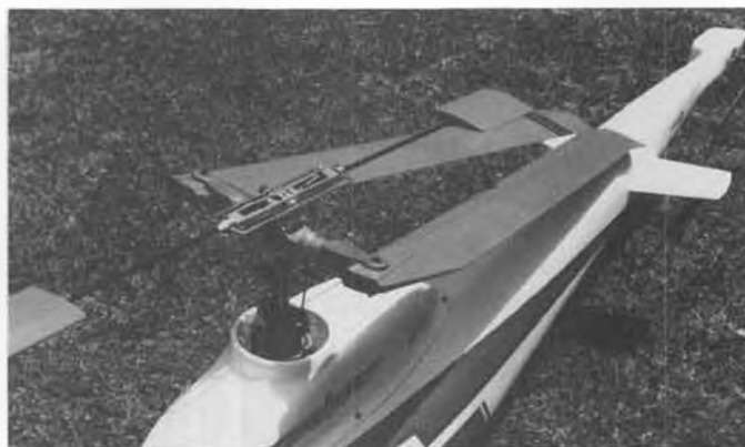
Close-up show single-bolt attachment of blades on Kavan head. Big improvement without any apparent disadvantages.
