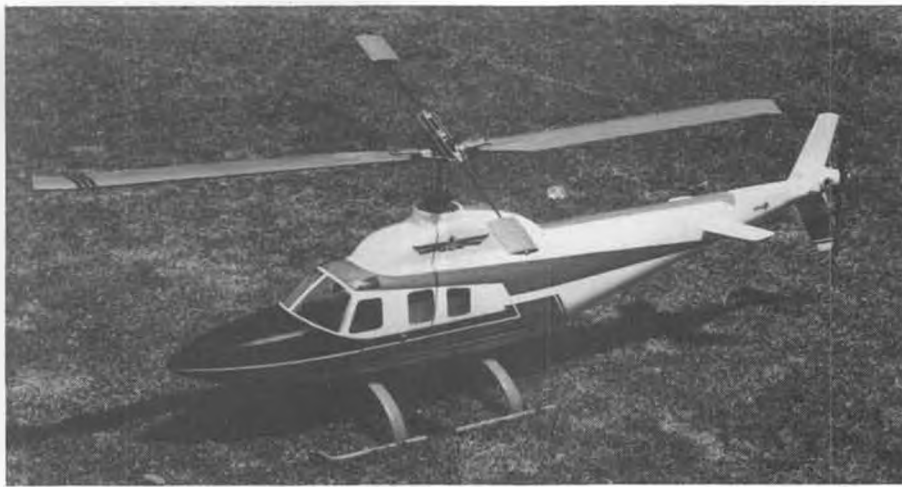
John Tucker's Shrike Commander/Kavan/Ranger/What-have-you, as described in April issue. Latest modification is single-bolt blade attachment, which has several advantages. See text.
