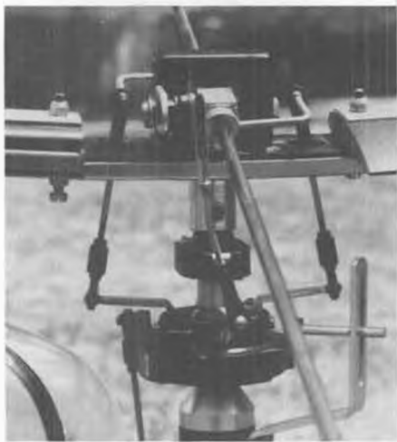
Smoother Alouette flight from installing two cranks on stabilizer bar. See text for more.
