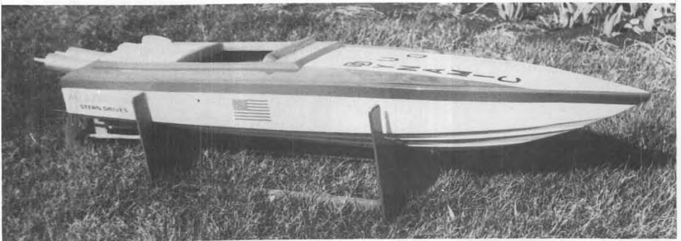
The completed Dumas Deep-Vee with twin OPS 60 engines. Fibreglas hull was specially reinforced by factory to handle twins. Hull is designed for single 60's, not twins, in its stock form. Watch for future report on running tests.
