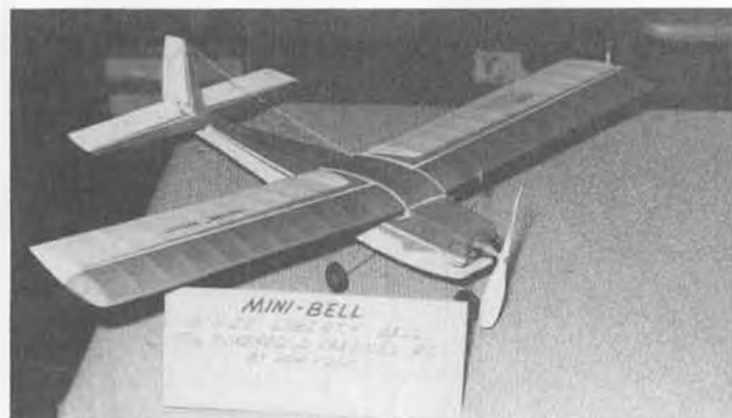
This CO 2 Brown twin powered 1/3 size Liberty Bell (Goldberg Sr. Falcon) "Mini-Bell" is controlled by Cannon mini 2-channel radio.
