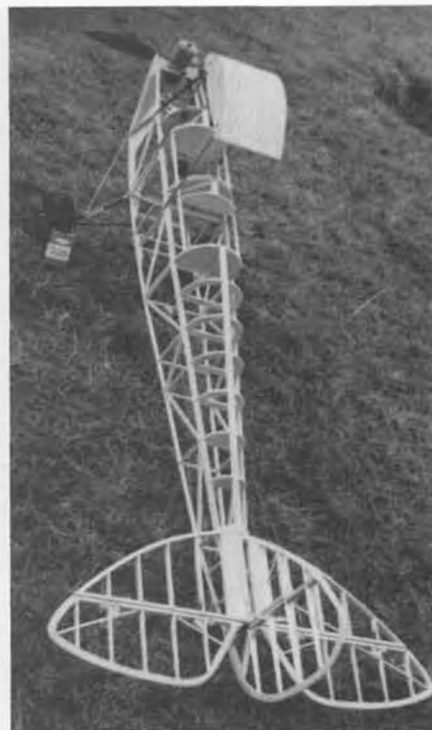
Fuselage and tail framework. Fuselage sheathed with 3/32 balsa. Nylon covering over all.
