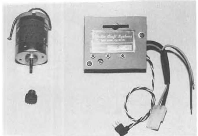
Electric R/C car speed control, by Electro Craft Systems, shown with Astro Flight Astro 05 motor.
