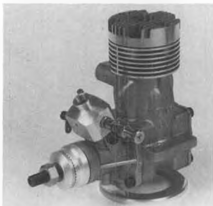
MRC-Enya's Schnuerle-port 60XF-TV develops 1.7 hp at 16,000!
