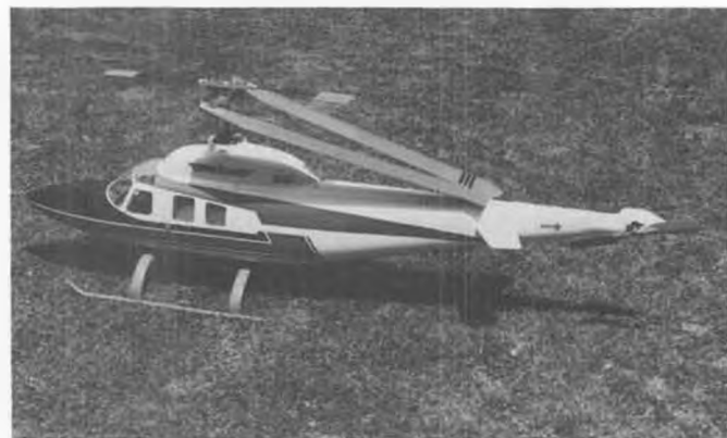
With blades folded and vertical fin removed, chopper is easier to transport. Single bolt also improves balance, avoids splitting.
