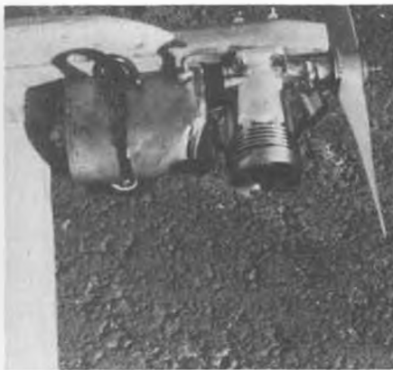
Tank is uniflow vented for consistent runs. Engine is home-brew "McFox" 34.
