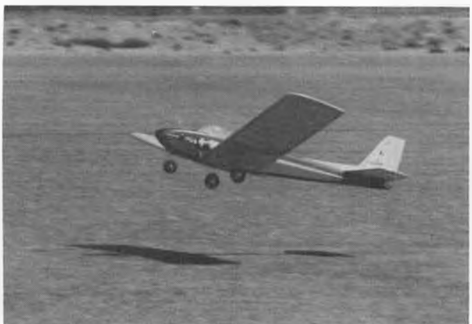
Bob Simon also went the electric route, with 2 Astro 05's in his Goldberg Skylark. Nose gear linked to rudder for "ground driving".
