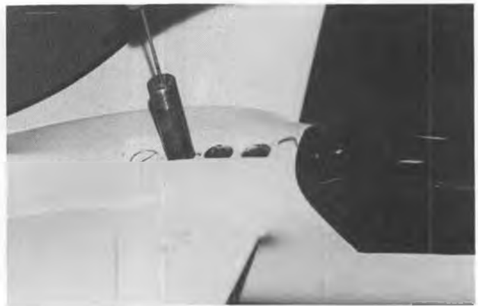
Ballast can be added to Ken Bates' flying wing sailplane for increasing speed and/or varying wind conditions.
