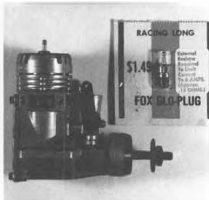
Fox .15 Schnurle-ported R/C engine, with ball bearings.
