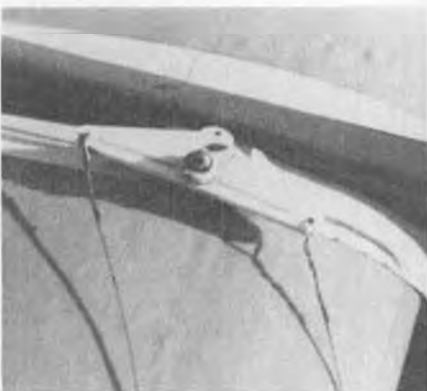
Extremely simple outside bellcrank mount.
