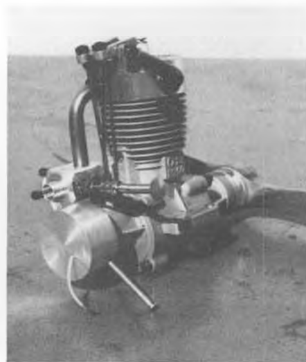
Ignition conversion of the OS 60 four-cycle engine by the SCAMPS' Jim Dean. Rear timer geared to fire every other crank revolution.
