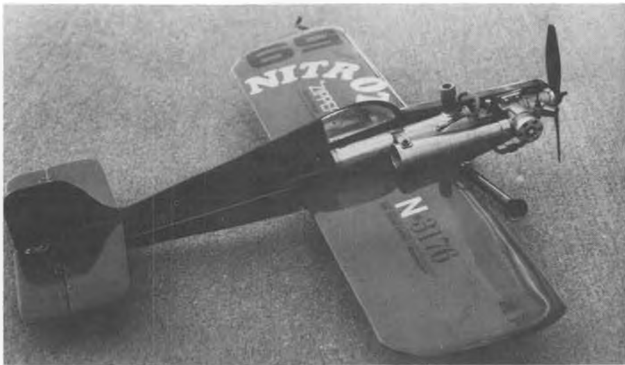
Bill "Moose" Allen's "Badyear" . . . a Kilsdonk designed "Zipper". FV Rossi with megaphone, Rat tank, titanium gear, Kilsdonk shut-off, Kelly glass prop, Hobby epoxy paint and deco by Bill.
