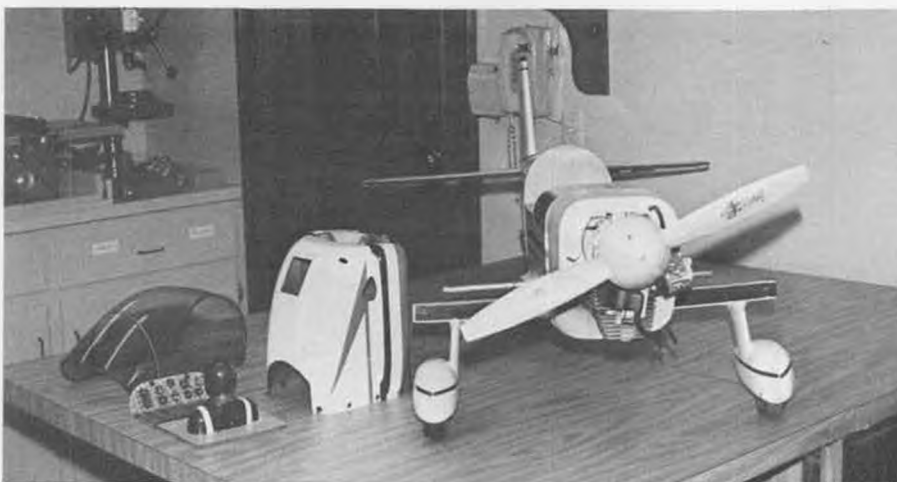
The combination wing beam and landing gear mount takes all flight and landing loads. It's eight laminations of 1/8 spruce laid up with epoxy. Canopy is molded plexiglass.
