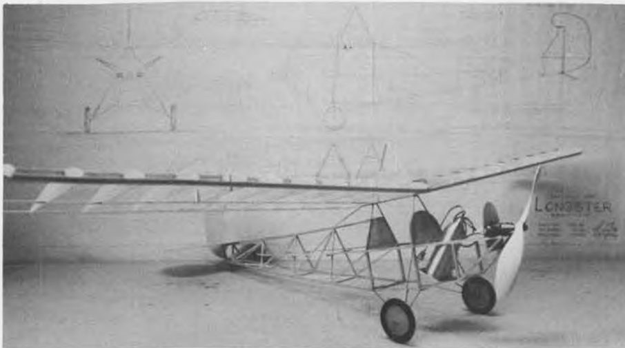
Completed basic structure is quite light, closely follows the construction of the full-size Longster. The flying wires are functional, so don't leave 'em off.
