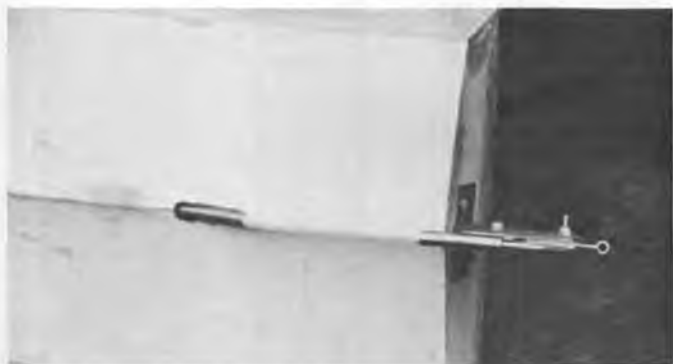
The flex drive cable and tube installation. Make the hole in the hull oversize, then fill with epoxy and micro balloons.
