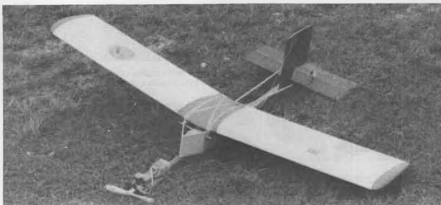
The "Knock-About", knocked together by Charles Ricci, Pompano Beach, Florida. Could call it "R/C on a Stick". Fuselage (?) is a piece of 1/2 x 3/4 x 37-inch hardwood. More info in text.
