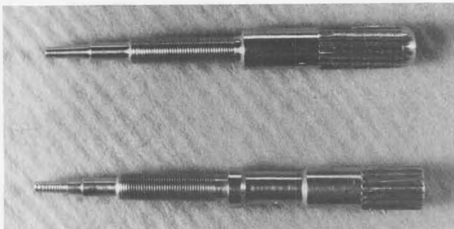
All needle valves are not created equal! Look closely at the taper and see text for details.
