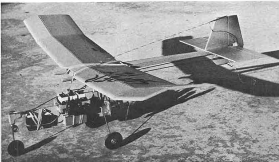
LIAHO (July '73 MB) featured an open-air radio installation. Layout subsequently copied by European kit manufacturer, though radio was enclosed in built-up fuselage.
