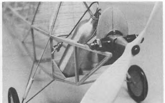
Closeup of the motor and tank installation. Model uses a 10cc main tank and 1-3/4cc condenser tank (hidden behind firewall).
