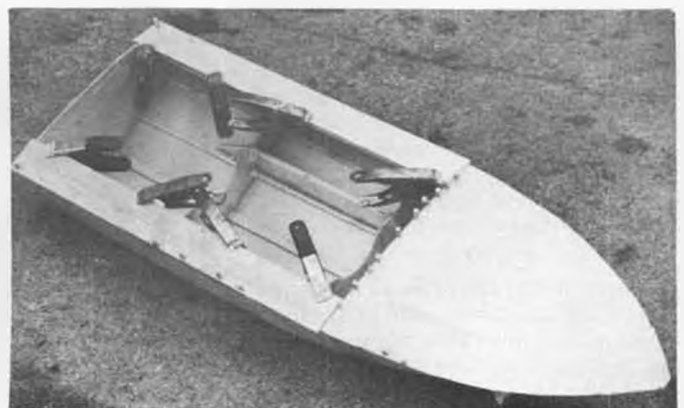
Masking tape, map tacks, and clamps are used to hold the deck sheeting in place.
