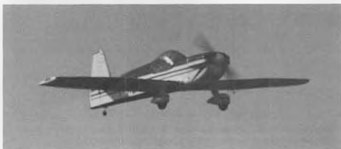
Jeff's CAP 20L in a fly-by at Las Vegas. Ship is an exceptionally smooth, stable flier, yet performs the snap maneuvers without difficulty. Sharp leading edge at outer end of wing panels, as detailed on plans, helps to stall the tips.
