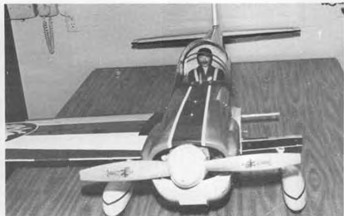
Another view of partially assembled CAP 20L. Wing and horizontal stabilizer are sheet balsa epoxied over foam cores.
