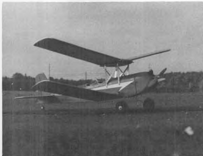
MB editor's second R/C ship, and first of many bipes, the Barnstormer, designed by Jack Luck. Pulse rudder, Arden .09 glow.
