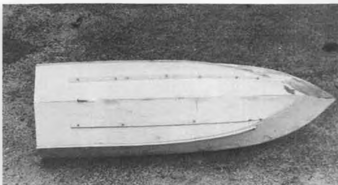
The bottom and side ride strakes are pinned in place while the glue dries.
