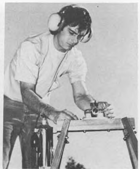
Mike Hoffelt adjusts his Fox the "proper" way. . . from behind the engine. Note ear protection and pressure bottle.
