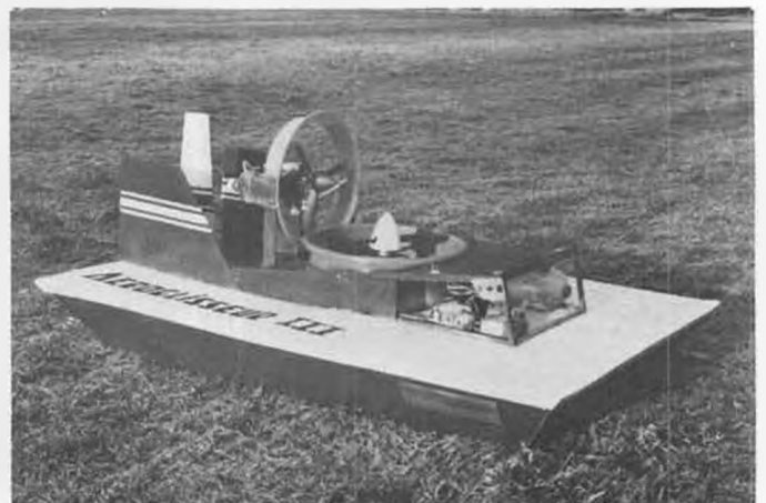
Georges Chaulet sent in this photo of his R/C hovercraft, which features two engines: one for lift, the other for propulsion.
