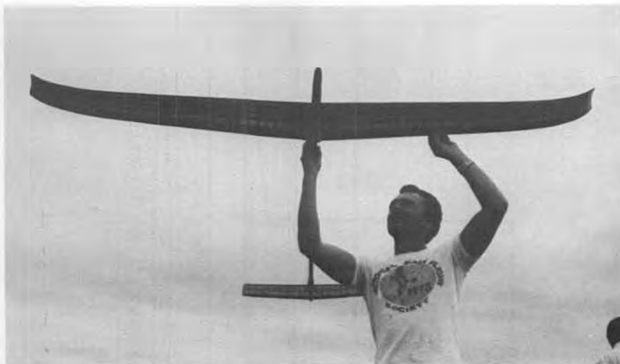
Two photos of Merv Buckmaster and his "Eldia 2 DC" original design A/2 Nordic. Elliptical tip dihedral is quite rare on F/F designs, but is sometimes seen on R/C sailplanes.
