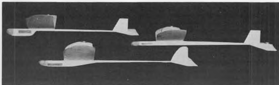
Three variations on fuselage profile shape have been experimented with over the years, but no significant performance differences have been noted.
