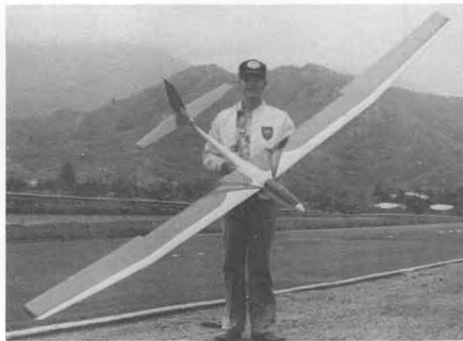
Ben Clerx shows off his "Kalihe". Ship spans 133 inches, weighs 5 lbs. empty, and features spring-loaded flaps.
