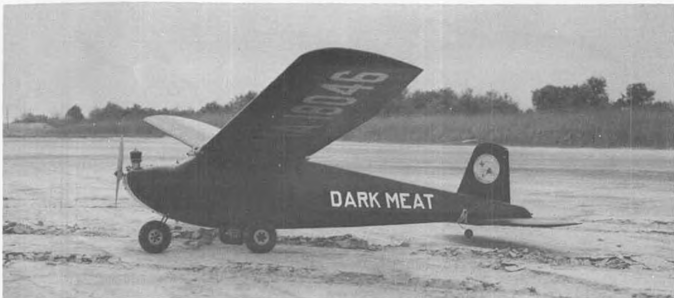
MB Editor's first ever R/C model, a Berkeley Royal Rudder Bug, with Babcock 3-tube radio and compound escapement, built in 1954. The five-pound ship was no ball of fire with the little K&B "Green Head" .15, but it flew successfully.
