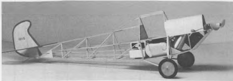
Fuselage ready for covering. Nose section covered with card stock prior to adding tissue. If you want a longer motor run and can stand the noise, a Cox .010 would be just right.
