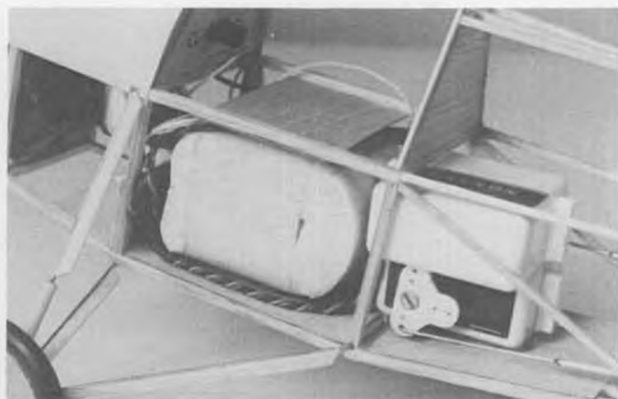
A lightweight, super-small radio is a must for this model. Prototype uses a Cannon rig, 100 ma. battery mounted in the nose.
