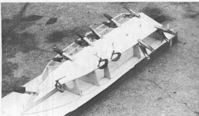
Clamping the bottom ply sheeting in place. Map tacks are used to hold middle of sheeting against frames.
