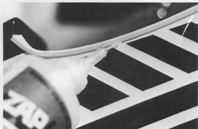
Application of cyanoacrylate to all accessible seams and joints prolongs the life of the model. Use care to prevent runs.
