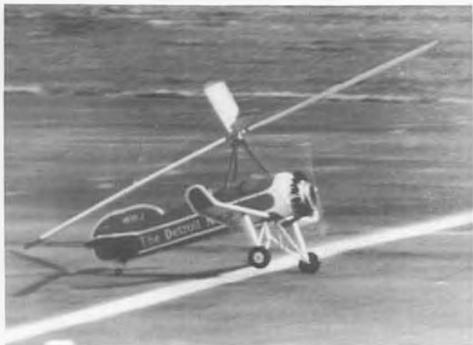
Model during latest tests, just before ground loop. Note flatter coning angle with more blade weight.
