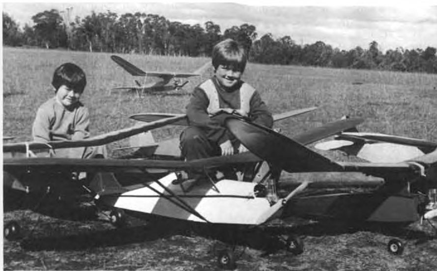
Wayne Hadkin's sons and the old time models at the UMAC contest. Playboy on the right was covered with brown kraft paper, water-shrunk and doped. Plenty tough and economical too!
