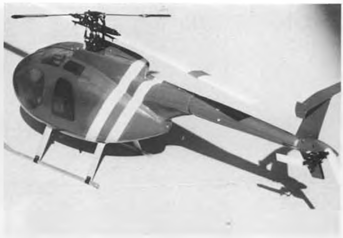
Modified tail and new landing gear change chopper to realistic 500D.
