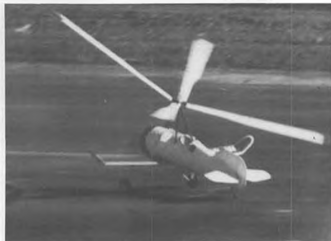
Continued test with heavier blades with reflex. Note forward blade is still rising too far up.
