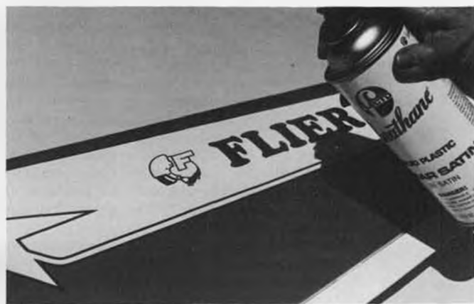
The quick and dirty method: give the whole model a spray coat of your favorite clear fuelproofers.
