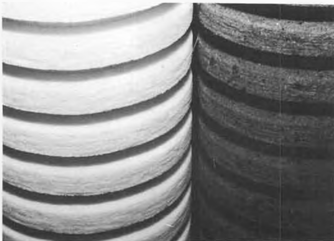
Five micron filter cartridges make the Magnum fuel appear crystal clear. New and used filters are pictured. Yecch!
