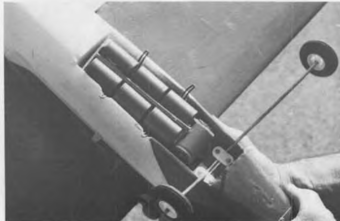
The 900 cells are slightly shorter and lighter than the regular sub-C cells, but deliver nearly the same power and duration as sub-Cs.
