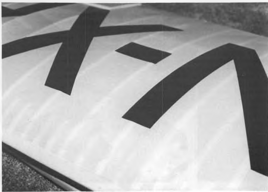
Rib stitching was done with Solartex and R/C 56 glue. See text for details.
