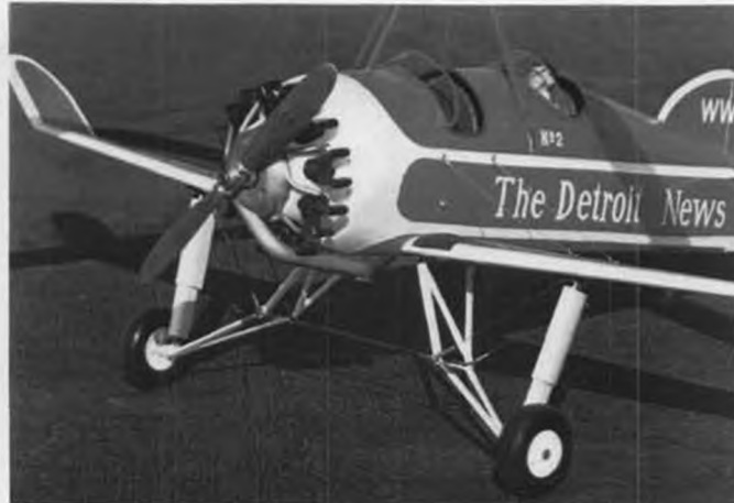
Fine scale detail on author's autogiro reflects his patient hand; all lettering and numbering is handpainted. When it comes to flight testing, the author's patience was really put to the test! A lot of critical adjustments to the rotors, cables, and center of gravity are most important.
