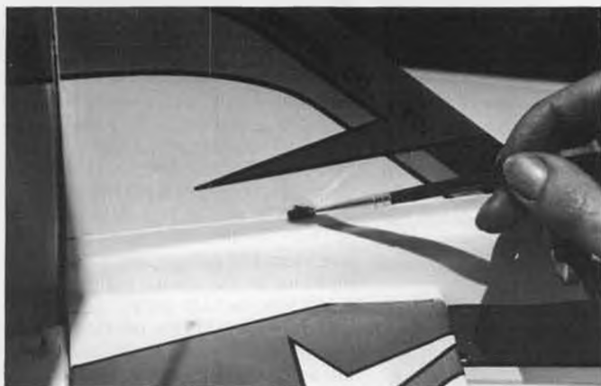
An alternate method of fuelproofing is to seal seams with polyurethane, using a fine brush.
