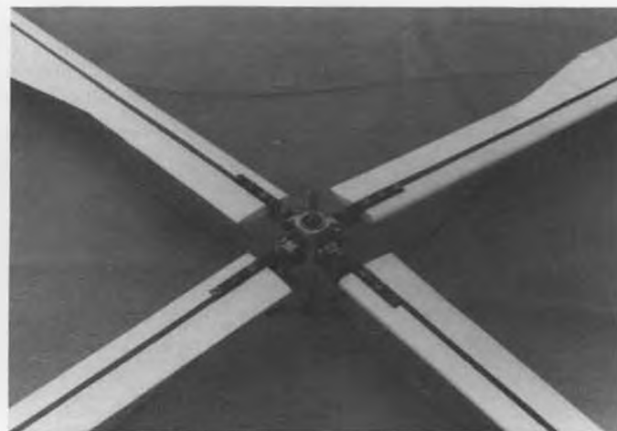
Bottom of rotor. Note ball bearings and set screw flat on shaft.
