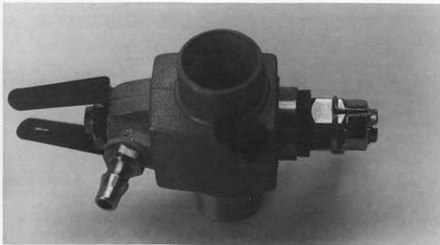
A dual sheet metal spring ratchet(left) maintains the setting for the high speed needle valve. A clever tiny wire spring dual ratchet(right) does the same for the idle needle whose screw/slot is visible at the extreme right.
