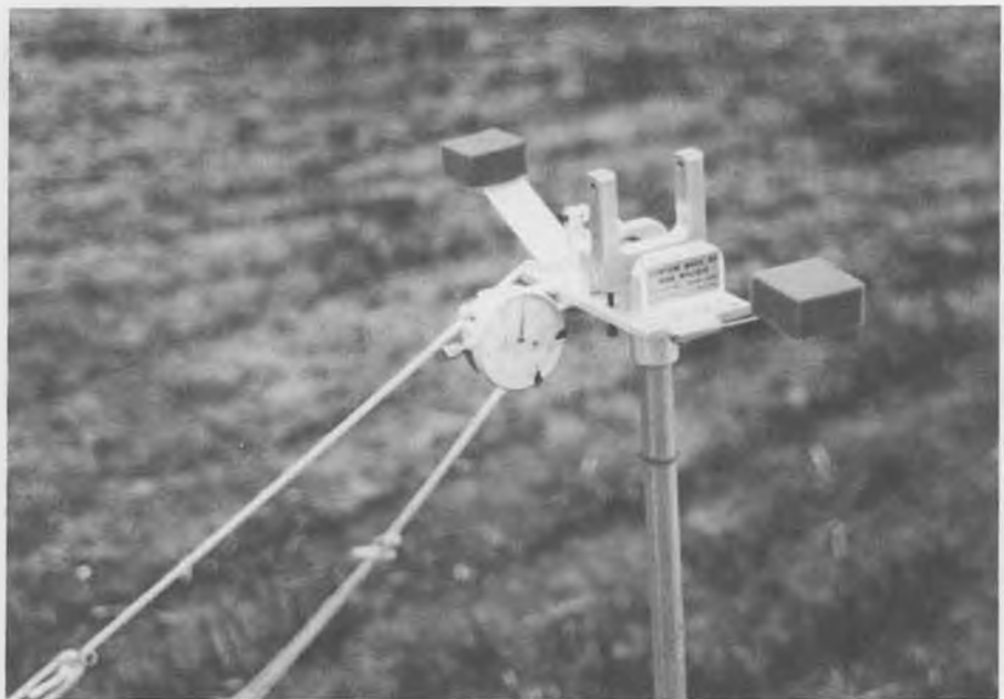
Text identifies Bob Wilder's products as one of the award winners in the NFFS Top Ten categories. Here is a picture of one of Bob's custom Wakefield Torque Meters.
