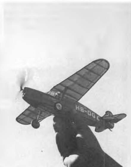
Prototype had inline four-cylinder air-cooled engine, which makes for a long nose moment that aids model's flight characteristics.
