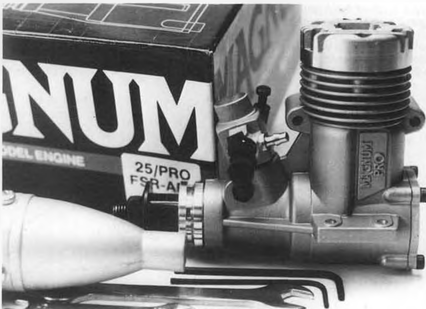
Magnum 25/Pro offers unusually fine options of dual ball bearings and an aluminum piston with a chromed brass cylinder, at attractive pricing.
