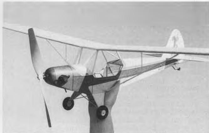
Jumbo Scale Crackerjack, also by Kruse, features plug-in wing panels and adjustable control surfaces. Struts pop on and off via Robart hinge point connectors. Model spans 36 inches, weighs 3.75 oz.
