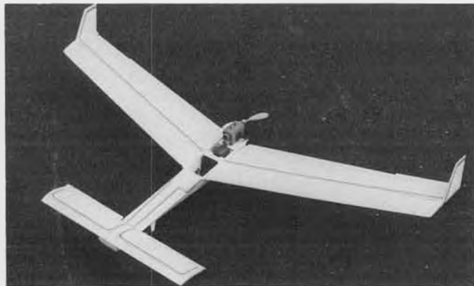
Unusual Goldwing ultralight canard by Larry Kruse is powered by the tiny Brown A-23 motor. Ship features movable control surfaces and a canard surface trimmable by way of a concealed nylon set screw. Model spans 26 inches.
