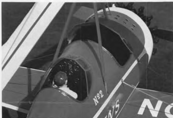
Fine scale detail on author's autogiro reflects his patient hand; all lettering and numbering is handpainted. When it comes to flight testing, the author's patience was really put to the test! A lot of critical adjustments to the rotors, cables, and center of gravity are most important.
