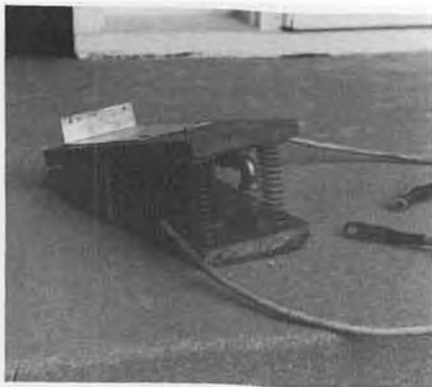
Fred Fredrickson of S.O.A.R. club in Illinois sends this photo of a footswitch which is itself the solenoid switch.
