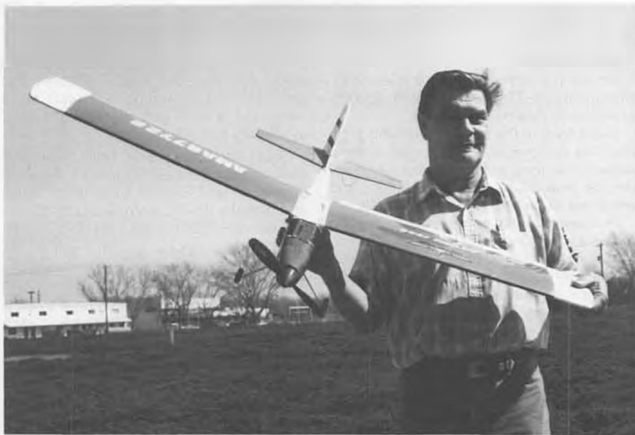
Ken Martin with his modified Etude. The RTF Etude is an easy ship to modify, as it is very versatile. Ken added one more rib panel to each side and set the dihedral at 3-1/2 inches.
