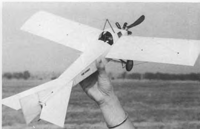
The '87 Nats winning Cessna Comet by Kruse is powered by a Telco Turbo CO2. Model is tissue covered with an airbrushed dope finish. Weight is 59 grams, wingspan is 22-1/2 inches.
