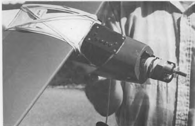
Ken uses an Astro cobalt 05 to the Etude, geared with the Kyosho Etude prop.
