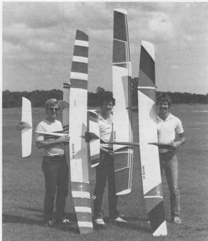
Above: The Mistral is a high-performance thermal duration ship, kit-ed up in Canada by ASTECH Models. Big ten-footer is of all-wood construction. See text for kit availability, and also for the interesting results of experiments using this sailplane to test various airfoil sections.
