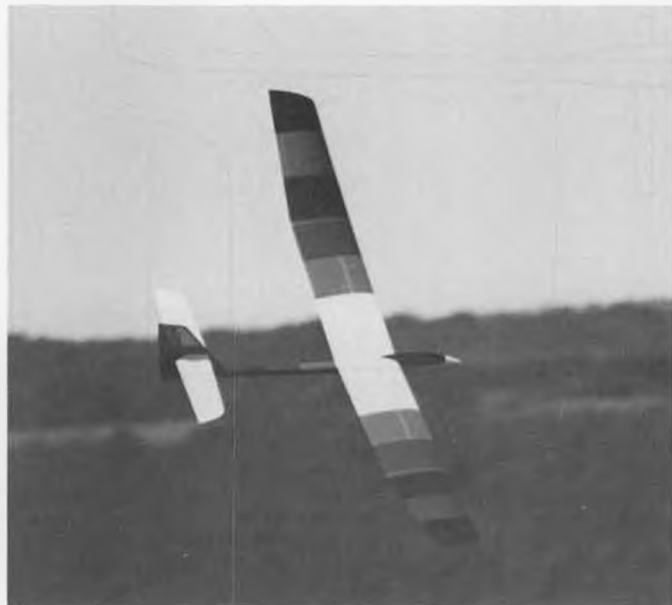
Above: The Mistral is a high-performance thermal duration ship, kit-ed up in Canada by ASTECH Models. Big ten-footer is of all-wood construction. See text for kit availability, and also for the interesting results of experiments using this sailplane to test various airfoil sections.
