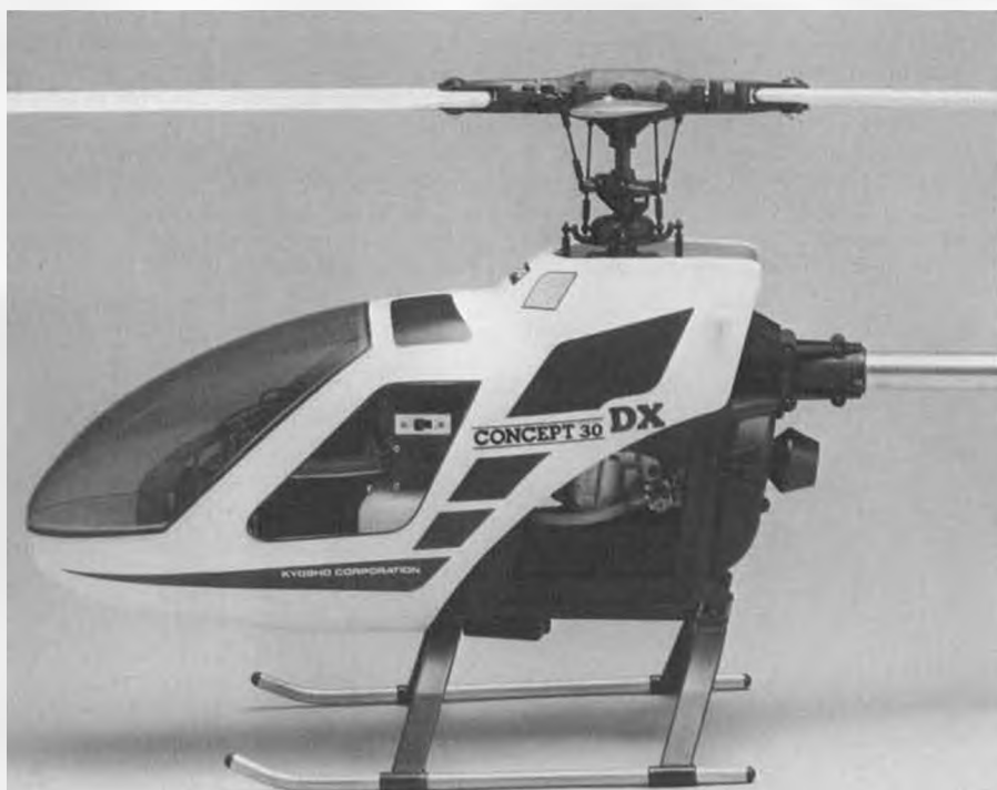
For traveling, the tail boom can be removed quickly and easily by loosening four screws and unsnapping the tail rotor pushrod at the point where the boom joins the fuselage. This photo shows the ingenious washin/washout scissor unit with 95% Bell-Hiller mixing ratio.
