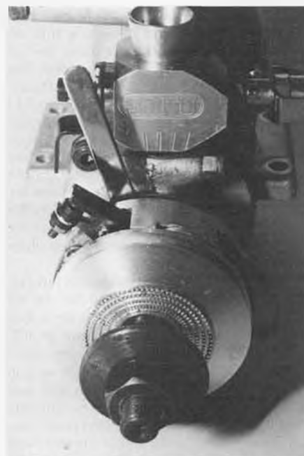
The Saito G60F is a modern spark ignition engine with exposed points and enclosed timing cam and follower. Note timer arm position marks on carb.
