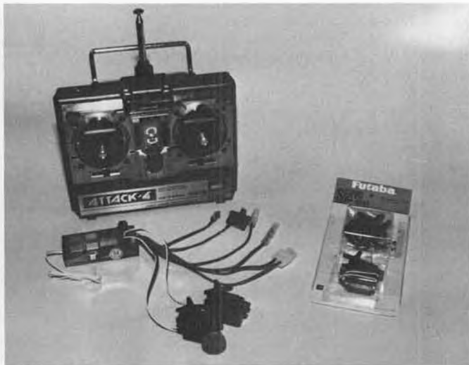
The Futaba Attack-4 radio comes with two servos; you'll need an extra for the Chipmunk. MCR-4A receiver has built-in speed control.
