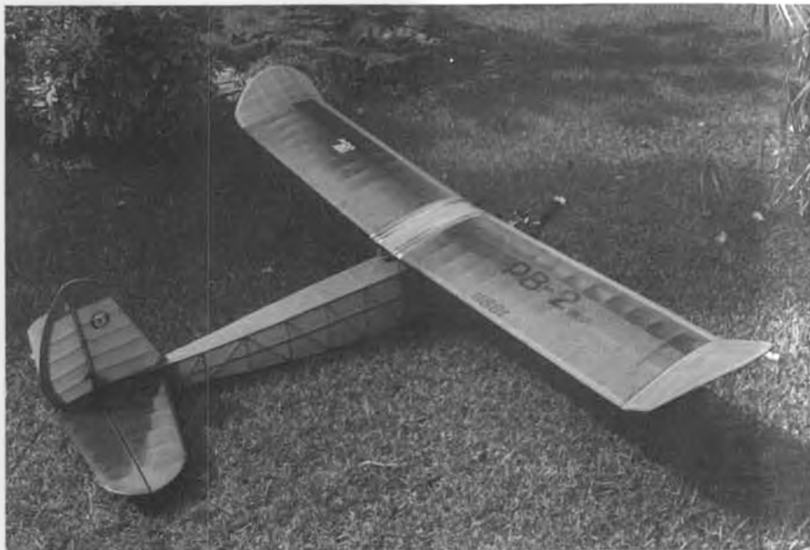
12. Another Aussie modeler, Dave Hipperson, sent in this photo of his Petrides PB-2, an excellent flier and good choice for R/C Texaco. Dave's uses an O.S. .60 four-stroke.
