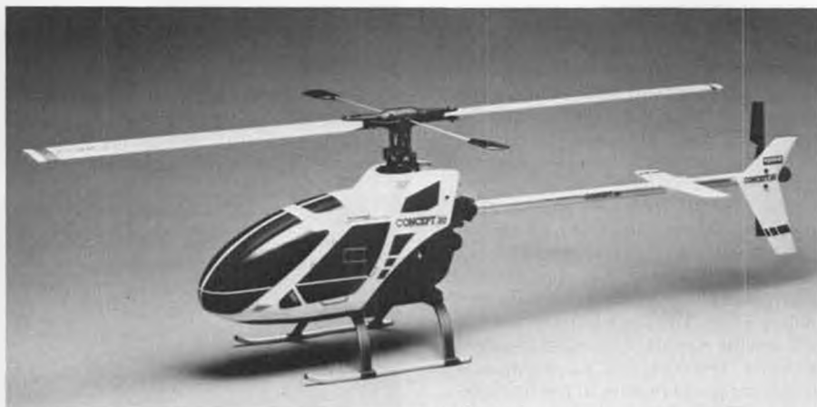
An excellent example of two-bladed main rotor design is the Kyosho Concept 30, reviewed in this issue on page 32. Model features an articulated rotor with mild flap hinge offset.
