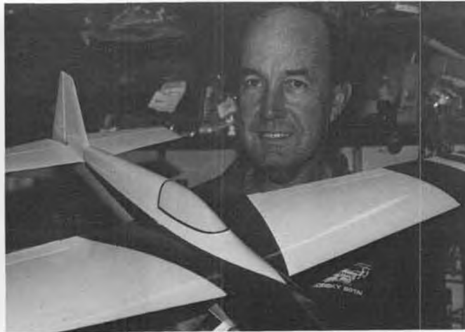
Keith won the Aussie Quarter Midget Nats in 1987 with this Nelson-powered racer. Uses Mac pipe, Kraft wheels and a 7x4 Taipan prop.
