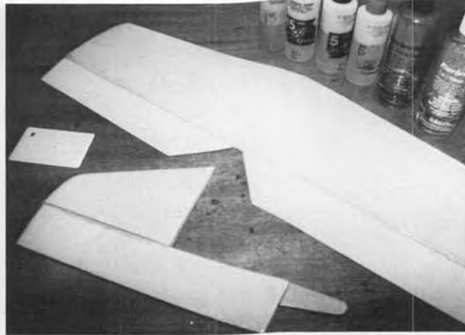
Tail surfaces are also of foam/fiberglass construction. Use a plastic wallet card to squeegee the epoxy into the glass cloth.
