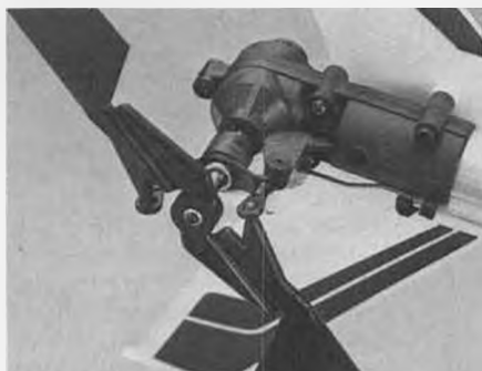
This is the one-piece molded bearingless tail rotor that is available in Japan, but not here in the U.S. Our author is nuts about it. Appears to work on the "live hinge" principle.
