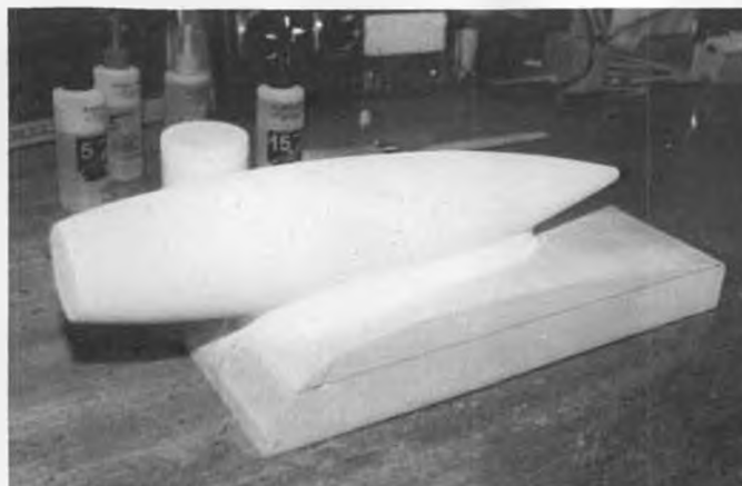
Nacelle core is made of blue foam, turned on a lathe. Airfoil-shaped base guarantees proper fit to wing. After glassing, the foam is dissolved with paint thinner, leaving a finished part (right).
