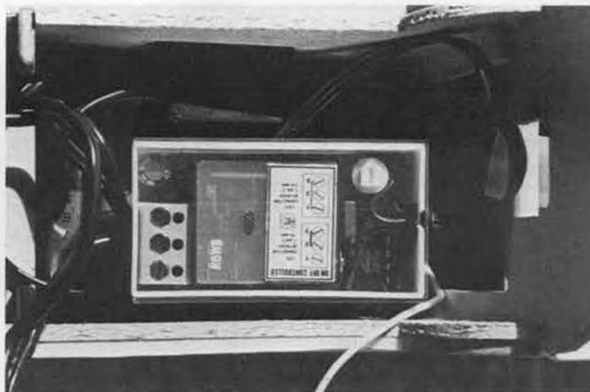
Electronic on/off controller from High Sky nestles on top of the receiver. Compact unit does away with a third servo and switch.
