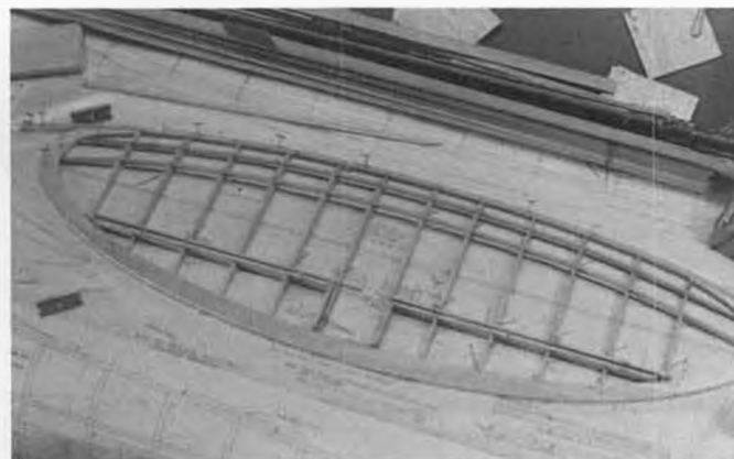
3. The addition of elevators to the Playboy's horizontal stab for R/C flying is a fairly easy job.
