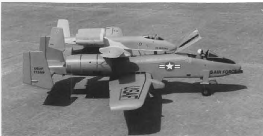
The larger of the two A-10's belongs to Ron Appleton, was built from Radio Modeller plans, uses a single integral silencer for both engines and is also equipped with an electric fuel pump. The little guy perched on top is Alex Cornish Trestrail's twin Cox .051 ship.
