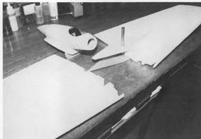
Tapered plywood joiners provide structural integrity for the wing center section. Tube extends up through nacelle for access to single wing attachment screw.
