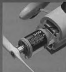
A standard 6 or 7 cell pack powers the shock-mounted Turbo 550 motor.
