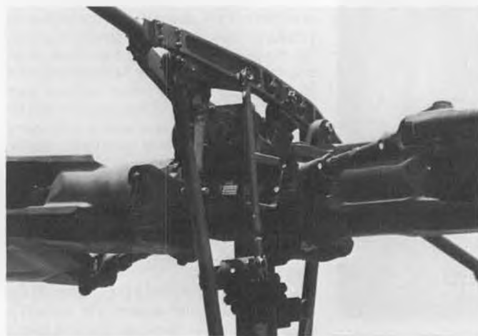
FIGURE 7. Close-up of the main rotor on a full-size Bell UH-1 Huey. An example of a two-blade teetering rotor.
