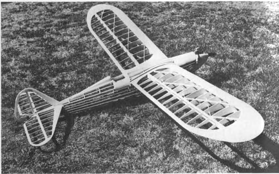
11. Bare bones Cumulus shows typical Ben Shereshaw construction. Model is being built as an R/C ship by Australian O.T. modeler Martin Simons.
