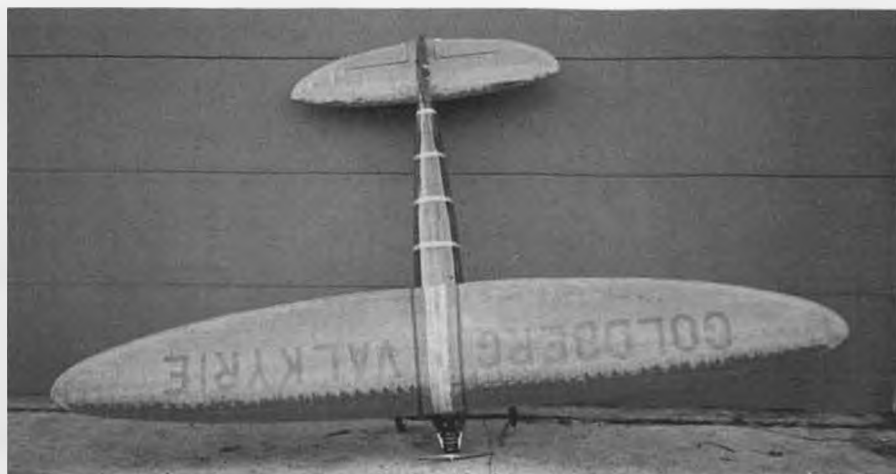
Old Timers make great subjects for all sizes of electric power systems. Colin McKinley built this big ten-foot Carl Goldberg Valkyrie for an Astro 60 cobalt with 24 cells.
