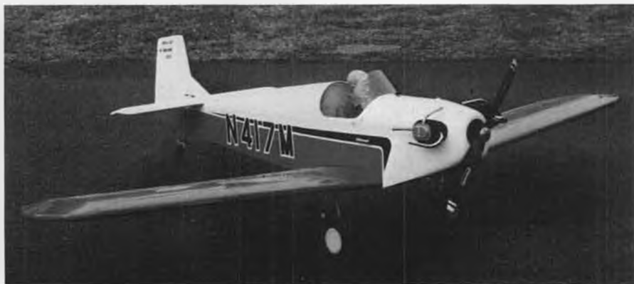
Sporting a new fuselage, right wing and horizontal stab, Doug MacBrien's favorite, the Druine Turbulent, flies again after a three-year hiatus. Scratch built from his own plans.
