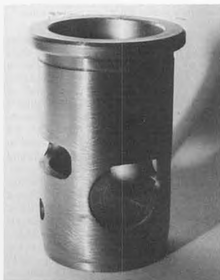
The Fox "Q" brass cylinder has round recessed areas machined at the front and rear fuel/air inlet ports. Engine is designed for all-out Quickee 500 racing.
