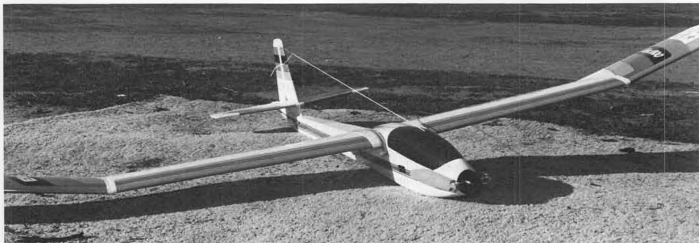
An example of modern ARF design at its best, the Elec. 1800 really turned our columnist on to electric power. Model is imported and marketed by Global Hobby Distributors. Note high horizontal stab for good ground clearance. It's our featured ARF of the month.
