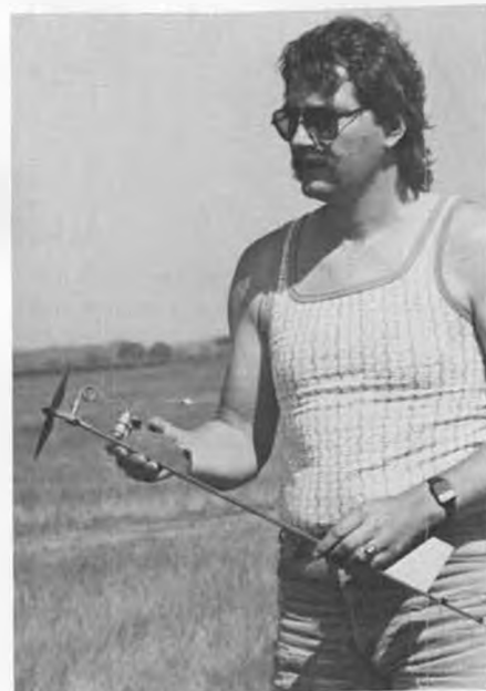
Czech flier Kucera displays the fuselage for his high-tech CO 2 ship. Tank is mounted on pylon for easy access and cooling.
