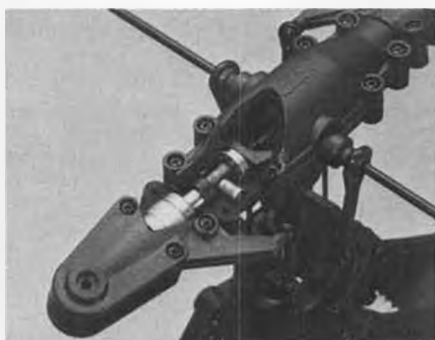
Cutaway of the main rotor hub reveals the inside of the Concept 30's articulated, 5% flap hinge offset rotor design. Soft flap stiffness gives very smooth flight characteristics.
