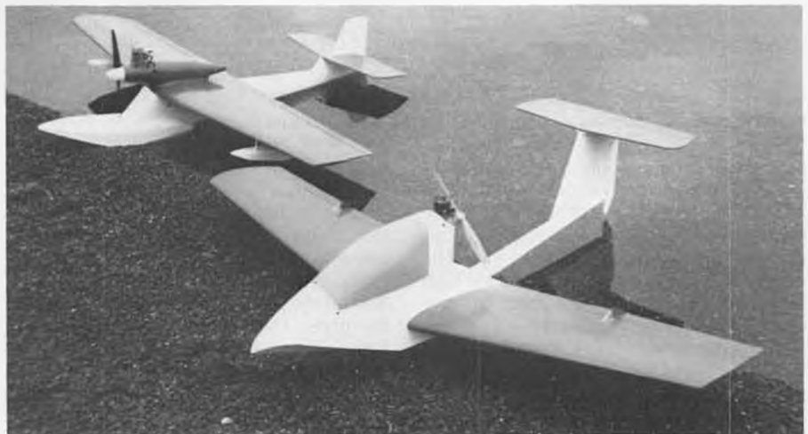
Author's Sea Fli X (foreground) and XI, placed side by side for direct comparison. Besides the obvious differences in configuration, they differ structurally in that the X uses a lot of balsa and a plywood covered wing, while the XI is 100% foam and fiberglass construction.
