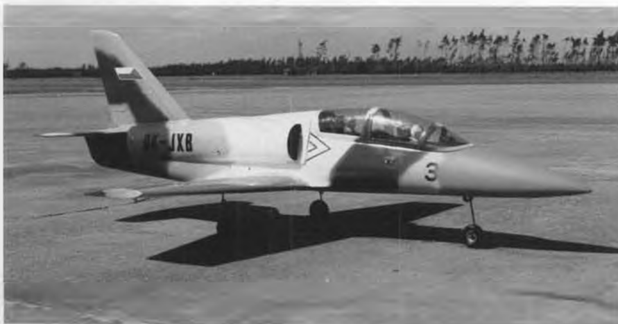
The L-39 Albatross is a popular ducted fan subject in England. This one by Reg Smith is from a Peter Nye kit and uses a Rossi .65/Turbax fan combination.
