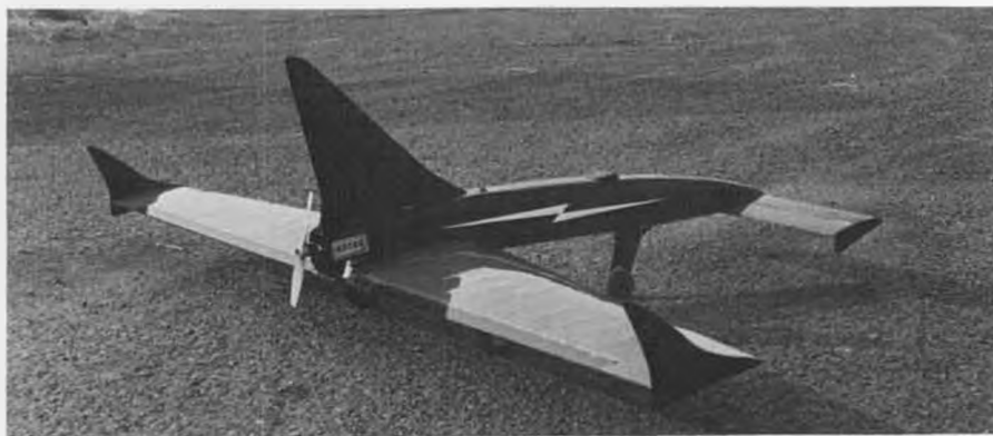
Mean looking "Diablo" is a German design, built by John Foley from Hobby Horn plans. A five-footer, it really moves out with an Astro 15 cobalt on 12 cells.
