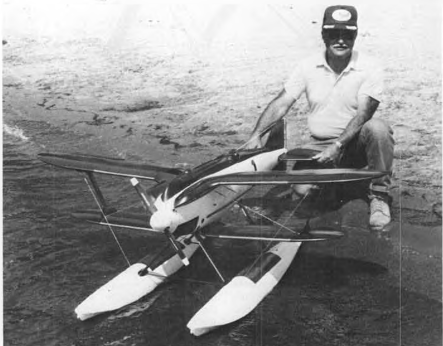
Absolutely gorgeous Gloster IV B Schneider Cup racer by master builder Leo Mariani was also featured in last month's "Brimfield Float Fly" article. At 1/4 scale the model spans 66 inches, weighs in at 14 pounds, and is powered by an O.S. 1.08. No flight reports yet, but stay tuned.
