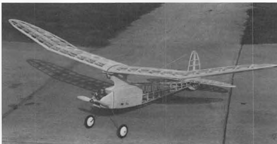
1. The framework of the prototype Tyro Models Playboy Sr. as built by John Pond himself. This month's column contains a lengthy and very interesting letter from Playboy designer Joe Elgin regarding the origin of this and other Cleveland Models designs.
