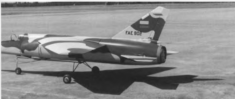
Sleek K&B powered Mirage F-1, built by D. Lings from Thorpe plans, is at least four years old and still going strong. Note takeoff dolly.
