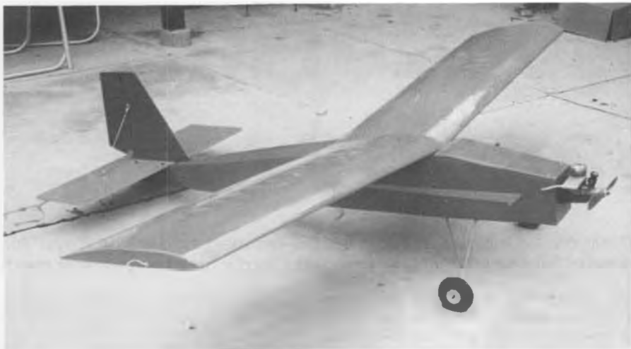
The first of five camera planes built by John Drouillard for UCLA. Original engine was a K&B .61 (shown here), but when cameras and strobe lights were added a Quadra 35 was installed. Still flying after years of trouble-free service. Story in text.
