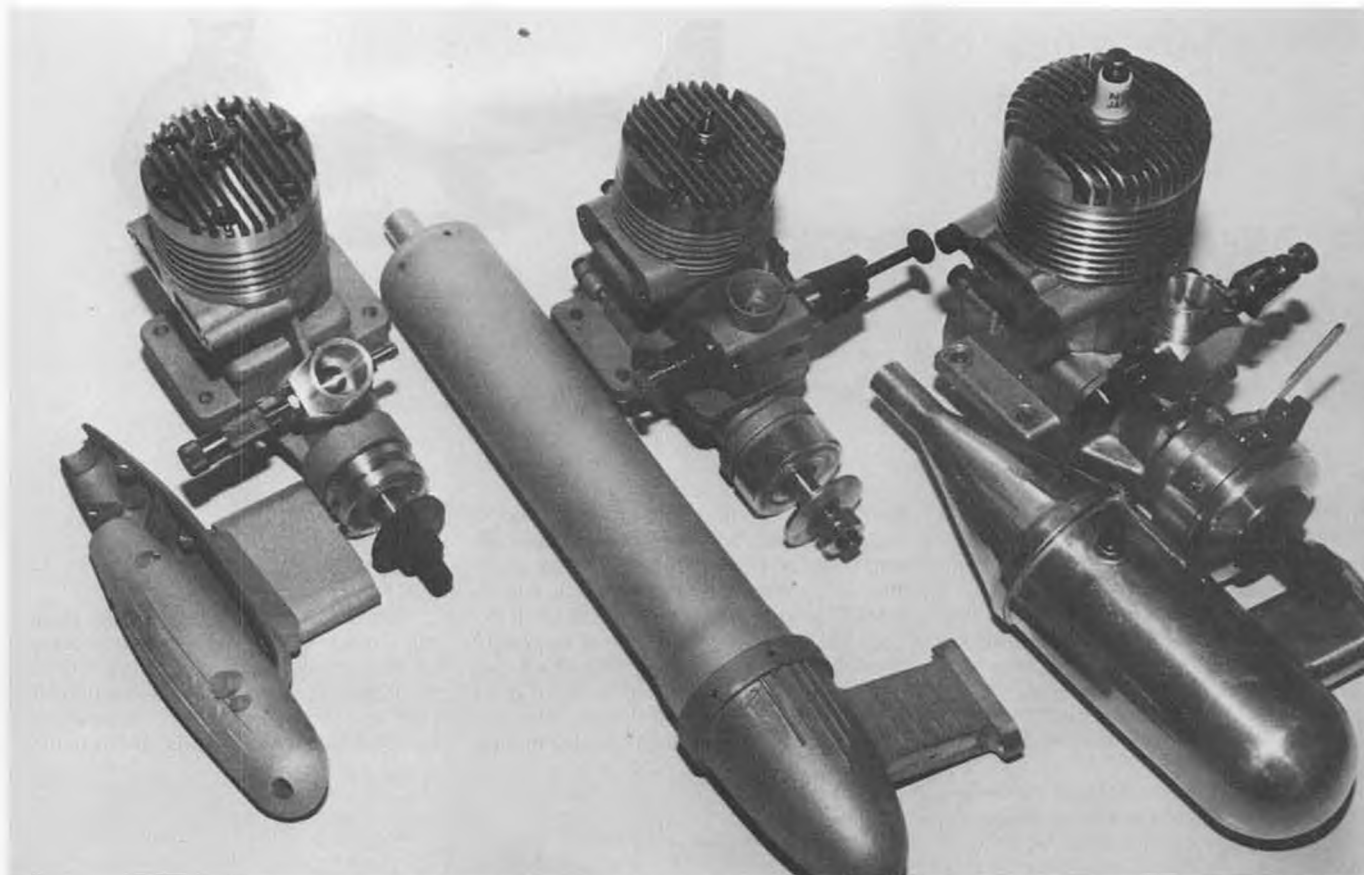
Even the matching mufflers are unique. The Merco .61SS has a three-part cast silencer (left), the Fox "Q" has a nine-inch muffled tuned pipe (center), and the Saito G60F has a beautifully spun and polished welded sheet aluminum muffler with pressure tap (right).
