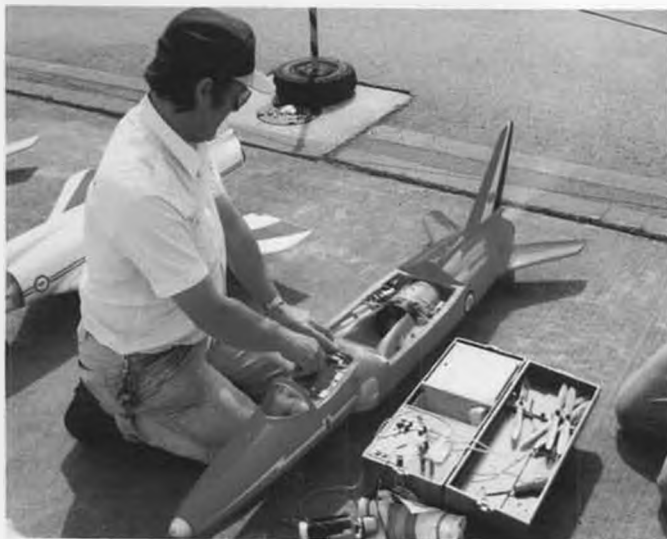
The L-39 Albatross is a popular ducted fan subject in England. This one by Reg Smith is from a Peter Nye kit and uses a Rossi .65/Turbax fan combination.
