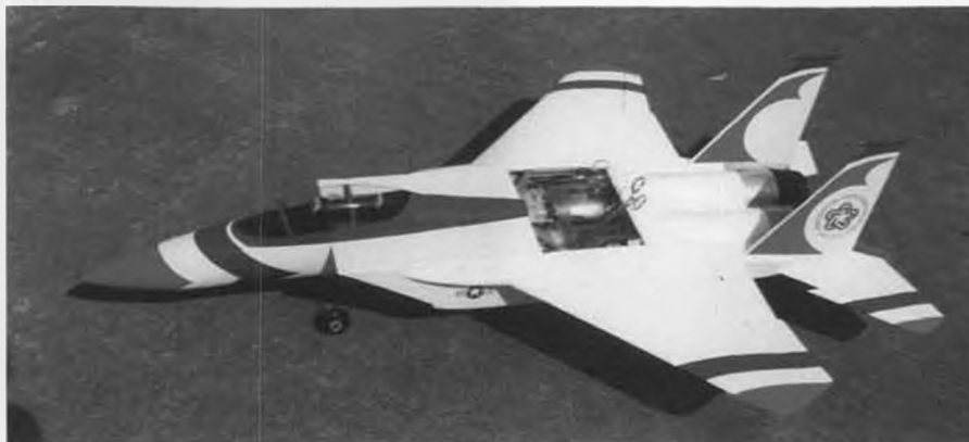
Scratch built F-15 by Alex Cornish Trestrail is powered by two O.S. 25 VR's with Kress 720 fans. Takes off from a steerable dolly and lands on a belly skid — a common setup in England.
