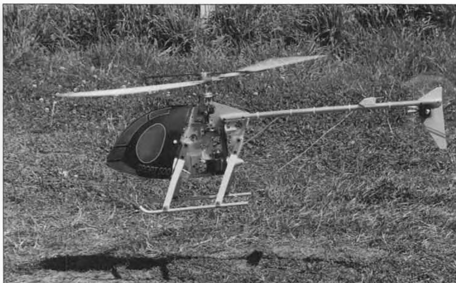
The first successful hover of Al's Sport 500 helicopter from Hobby Lobby Intl., after discovering incorrect installation of gyro that made it go crazy! See text.
