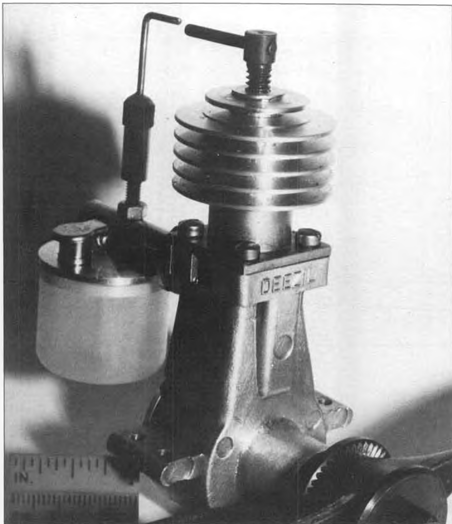
Engine design from the 1940s combines with ultra-modern metallurgy and precision machining of today in this SAM approved Repro DEEZIL.
