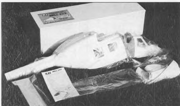
EZ Brand Bell 222 distributed by Global Hobby. Has more detail than Kyosho, is lighter, but a little more fragile. EZ fuselages are the only ones that come with windows pre-cut.
