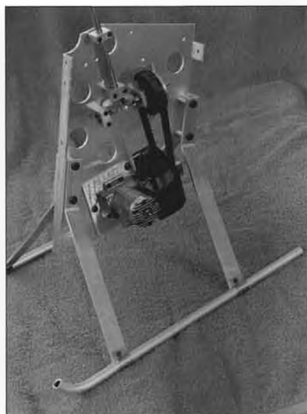
The Sport 500's chassis, with engine, cooling shroud, and main gears. Very simple and very rugged machine. Perfect for beginners.
