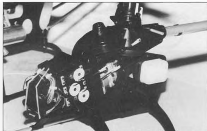
All pushrods on Hobby Dynamics/Kalt Enforcer are straight, to prevent buckling. Cone start from top. Frames and struts are glass-filled nylon. Plastic swashplate. Hingeless main rotor head with steel flexbeam.
