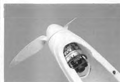
The LeMans AP36L motor delivers plenty of power for climbouts while a scimitar-shaped folding prop reduces drag.
