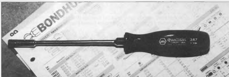
Here's a real useful tool available from Bondhus. High quality metric socket wrenches and Allen drivers from Wiha of Germany. We need 5.5 and 7mm. The 8mm is also good for accessing glow plug on Schluter and other helis.
