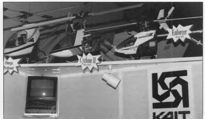
Hobby Dynamics' Kalt Omega Professor, Cyclone II, and new .30-size Enforcer that will be out this summer. Enforcer has 46-1/2 inch rotor dia., weighs 5-1/2 lbs.
