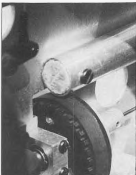
Al bushed the forward end of the tailboom tube with a wood dowel to prevent distortion when tightening the mounting bolts.
