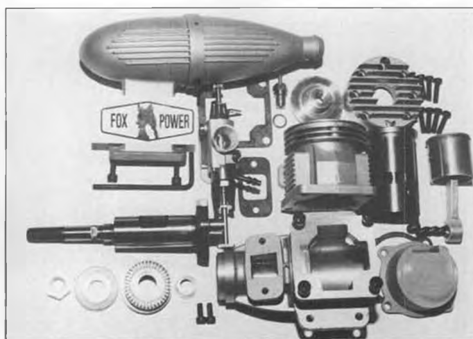
Teardown shows three paper gaskets. Text tells about bolt "snugging" when machine screws pass through paper gaskets.
