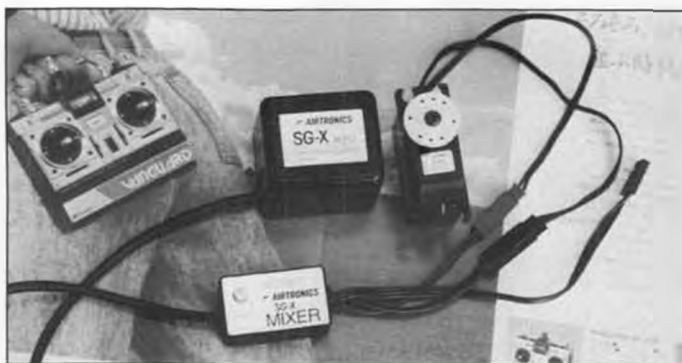
Airtronic's new SG-X gyro. It even includes a special tail rotor control servo. One of the least expensive electronic yaw rate gyros on the market.
