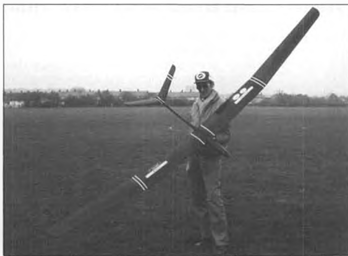
Saving the wing center sections of a crashed 12-foot BOT, Les Sparkes built this modern-looking V-tail, pod-and-boom soarer.
