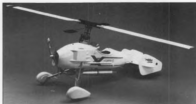
Robbe/Schluter .60-size autogyro. Uses Scout rotor head and a unique spin-up mechanism for jump takeoffs. Uses helicopter-style Bell and Hiller control system.
