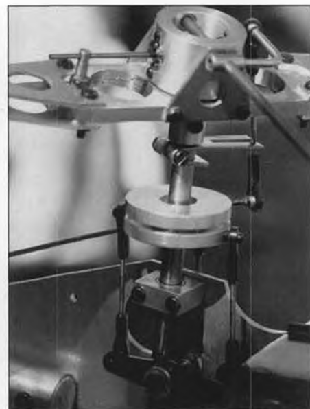
Main rotor head and control hookups are kept simple as a result of its being a fixed pitch helicopter.
