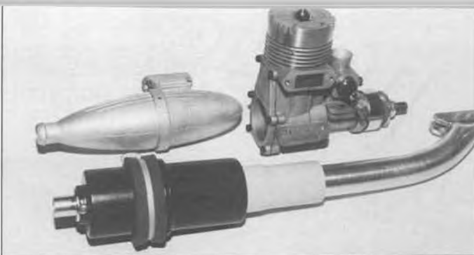
The rear outlet of all FOX mufflers is flared to accept a hose and clamp. You can see how easily this prototype FOX after-muffler fits behind this FOX .40 engine. Unit is supplied with two solder-in-place straps/clamps that are then bolted to the model's side. These prototype after-mufflers are simply sweat-soldered together and need airflow on all surfaces to keep seams from melting open from exhaust temperatures. Some after-mufflers use internal swirling actions to absorb the energy of sound... some use flow reversals to dissipate the energy... some use a series of holes to decelerate the exhaust velocity and dissipate energies. The muffler supplied with the K&B SPORTSTER engines uses a combination of these actions.
