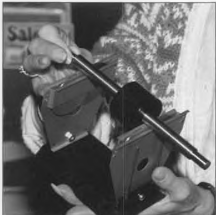
New flywheel and 10mm steel shaft from Hobby Hutch for balancing rotor head and blades on High Point or similar balancers.
