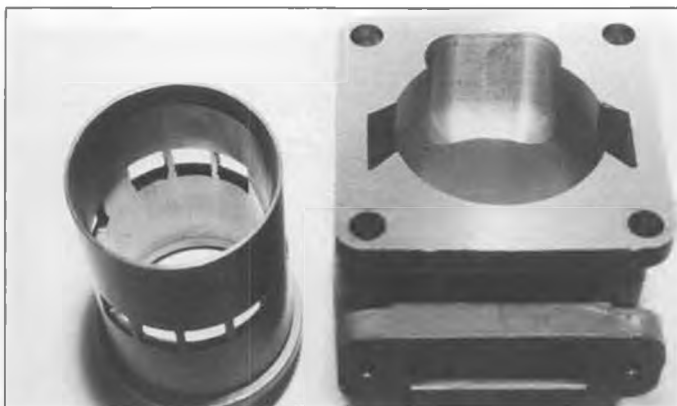
Bottom view of cylinder and its finned casting gives a good look at porting intricacies for modern Schnuerle engines.
