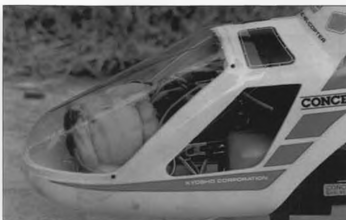
If you should break the tinted windscreen on your Concept, a quick substitute can be cut from a two-liter soda bottle. Each bottle will make two. Tim Lampe suggests using double-sided tape for mounting, so it will pop off in crash. Think positive, Tim!
