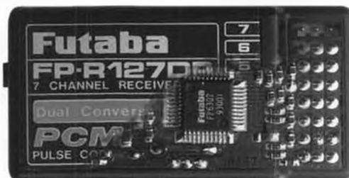
The heart of the new R124DP/R127DP PCM receivers is Futaba's custom microprocessor circuitry.
