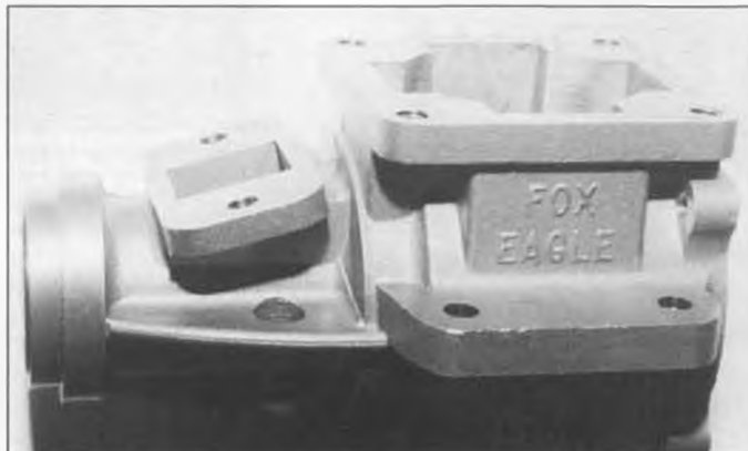
Parts for Fox engines, like this lower crankcase section, just a phone call away. Flange mounting of carb being copied by "Fangine 100."
