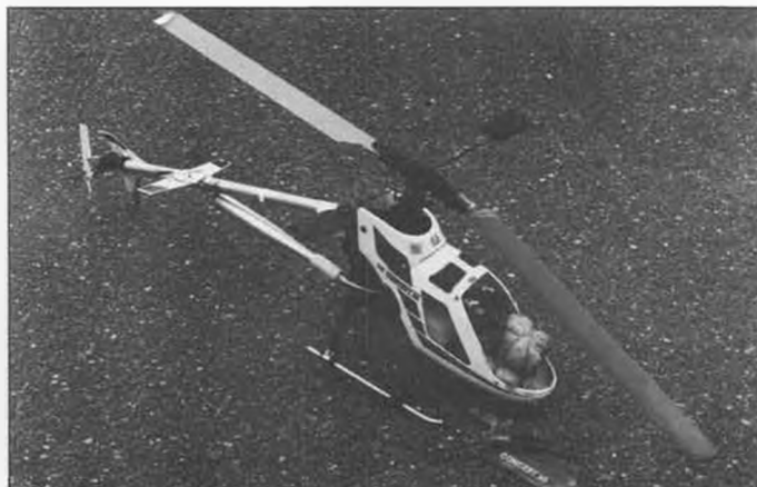
Author's Concept 30 after crash from inverted flight because of insufficient negative pitch. But it does fly great inverted! Note MACS 30-size aircraft tuned pipe system. Works better than MACS 30 hell pipe system.
