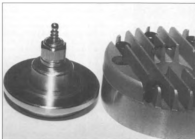
The glow plug threads into the machined button head (left)... casting on right clamps the button head in position.
