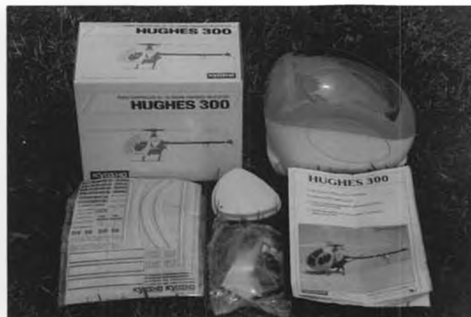
Hughes 300 kit is quickest way to convert Concept 30 into a scale ship. Not very scale close up, but looks very good in the air. Flies well, but big canopy slows forward speed a little.
