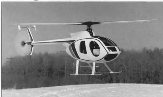
Concept 30 with Hughes 500 body. Aerodynamic shape of fuselage tends to pitch the model's nose up in forward flight. Note tiny GMP base-loaded antenna on landing strut.
